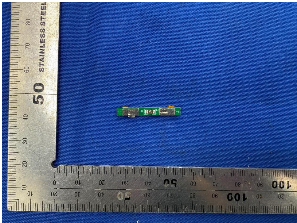
Picture 7. Front view of the PCB D (only for mounting PTC) (10095 & 10020)
