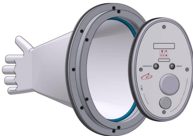
Figure 3: Insert Glove Test Device into the port.
