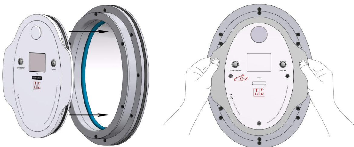
Figure 5: Inserting the Glove Test Device into the port.
