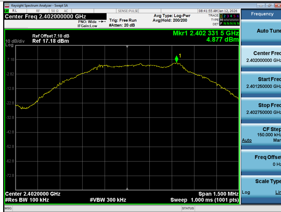
Tx. Spurious NVNT 2.4G 2402MHz Ant1 Emission
