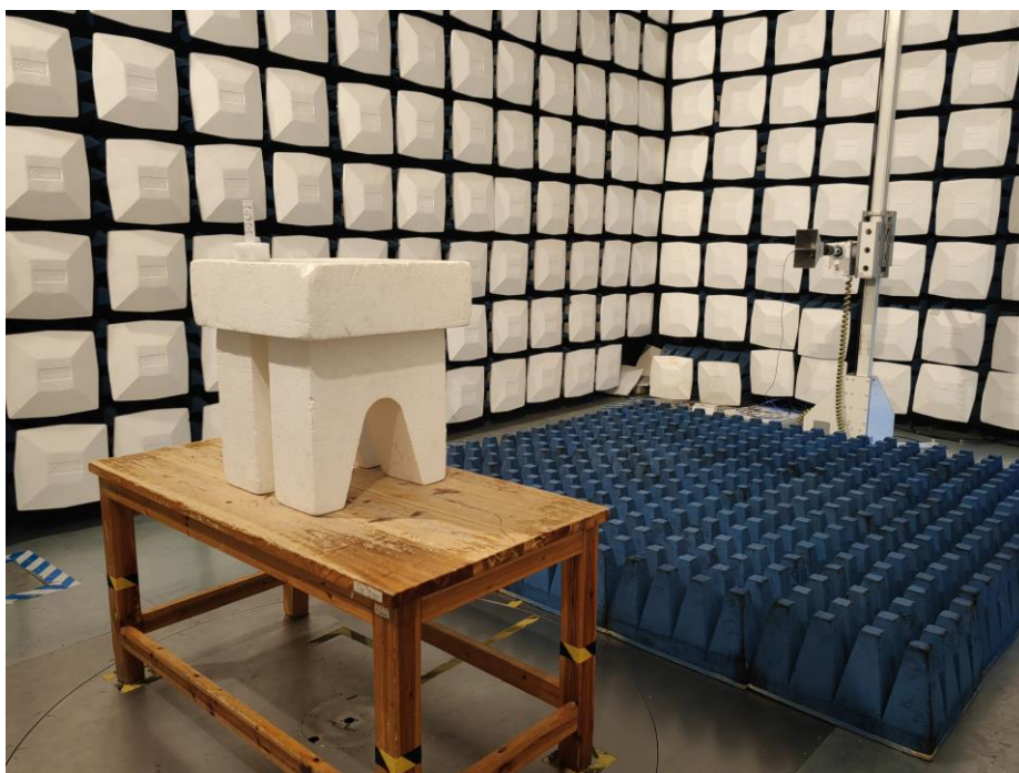
Test Setup For Radiated Emission (Above 1GHz)
