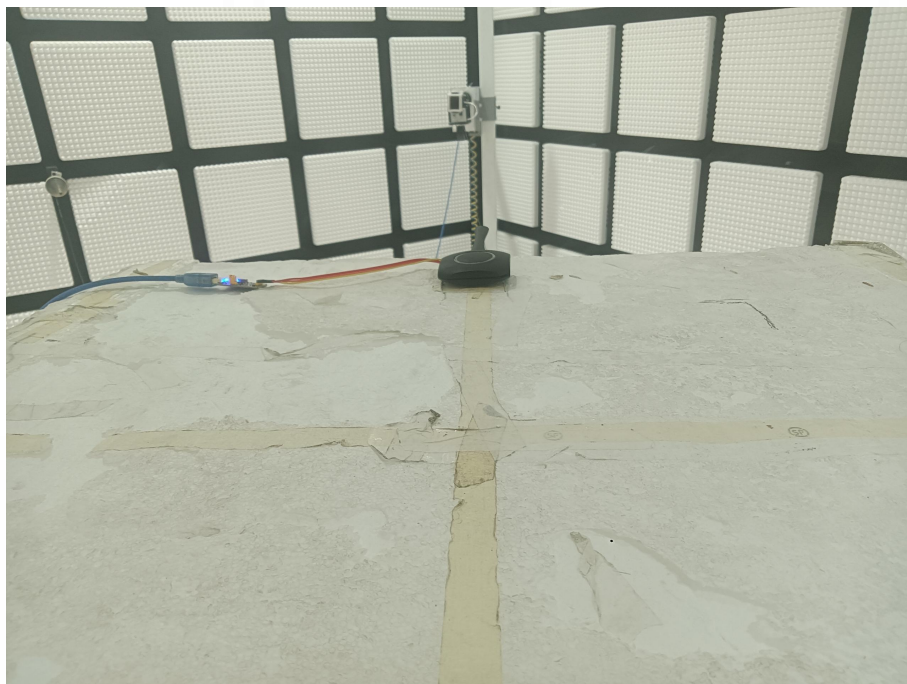
Radiated spurious emission Test Setup-3(Above 18GHz)
