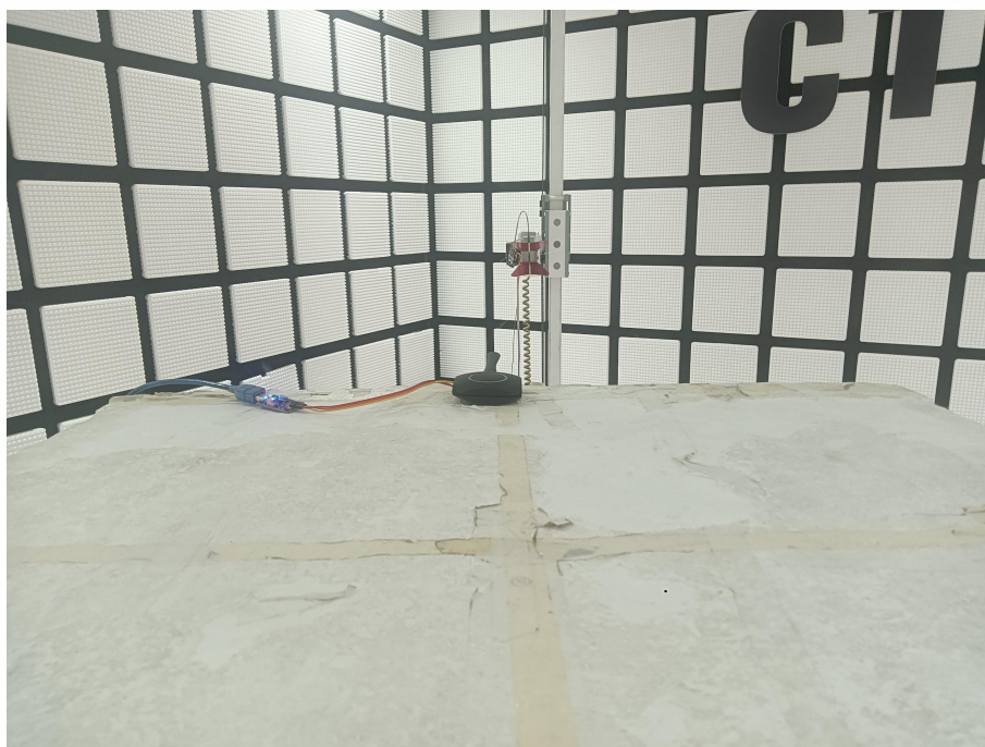
Radiated spurious emission Test Setup-2(1GHz to 18GHz)
