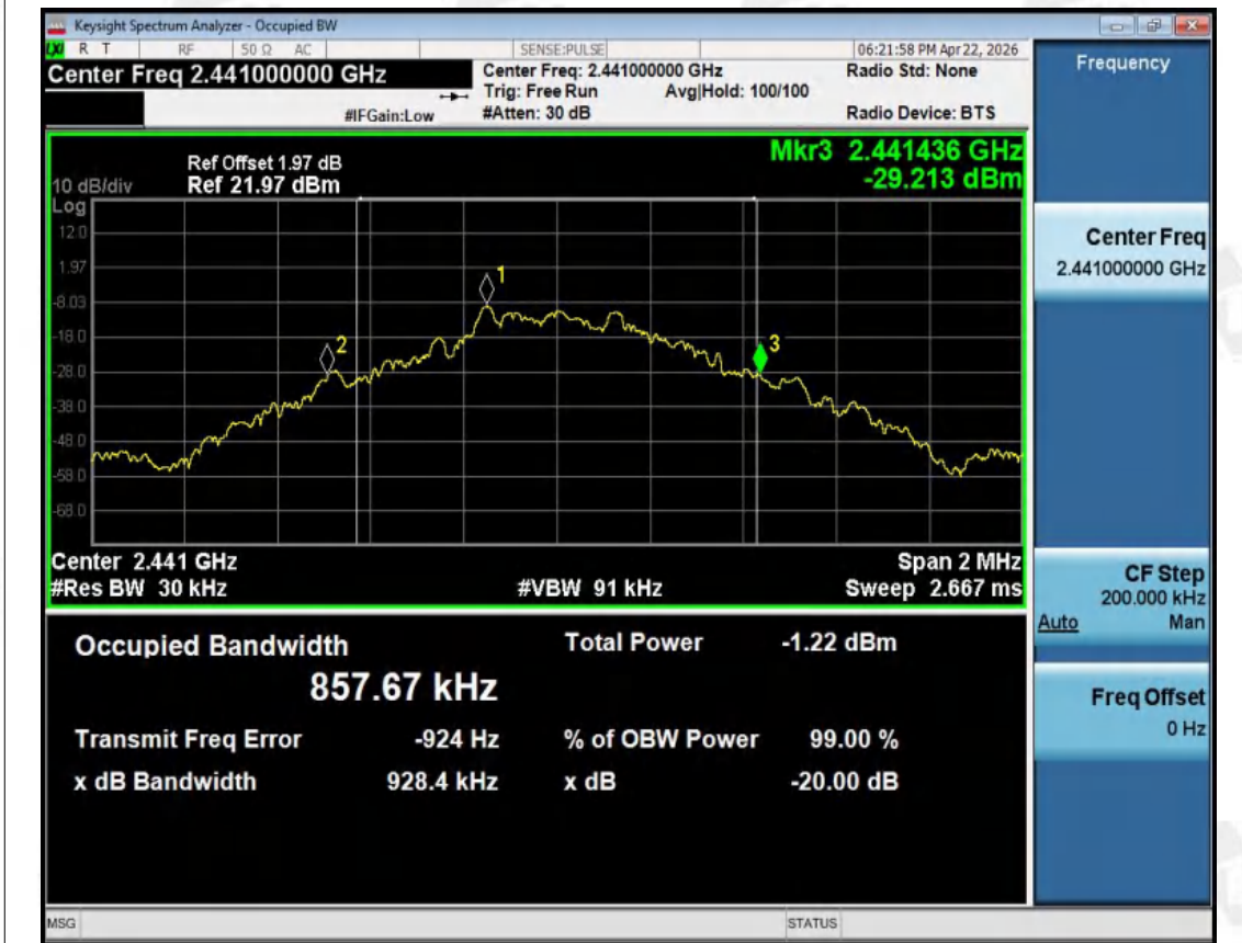
-20dB Bandwidth NVNT 1-DH1 2441MHz Ant1
