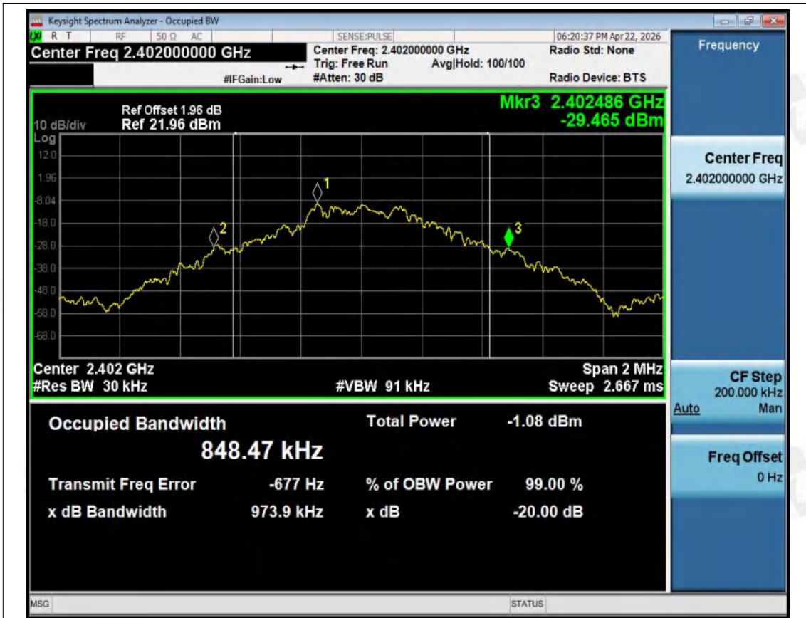
-20dB Bandwidth NVNT 1-DH1 2402MHz Ant1
