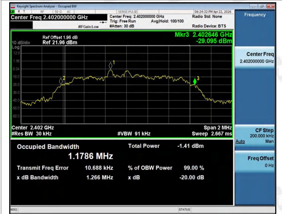
-20dB Bandwidth NVNT 2-DH1 2402MHz Ant1
