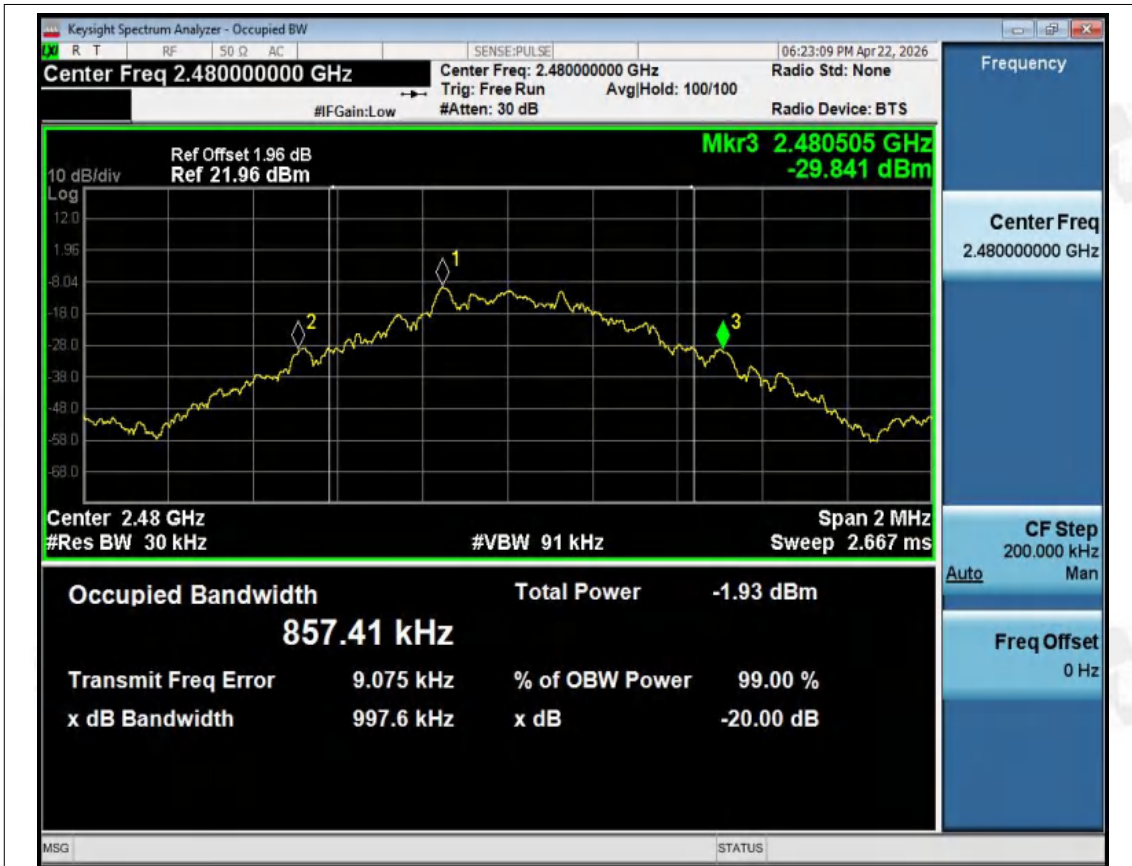
-20dB Bandwidth NVNT 1-DH1 2480MHz Ant1
