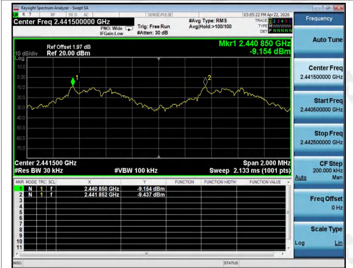
CFS NVNT 1-DH1 2441MHz Ant1
