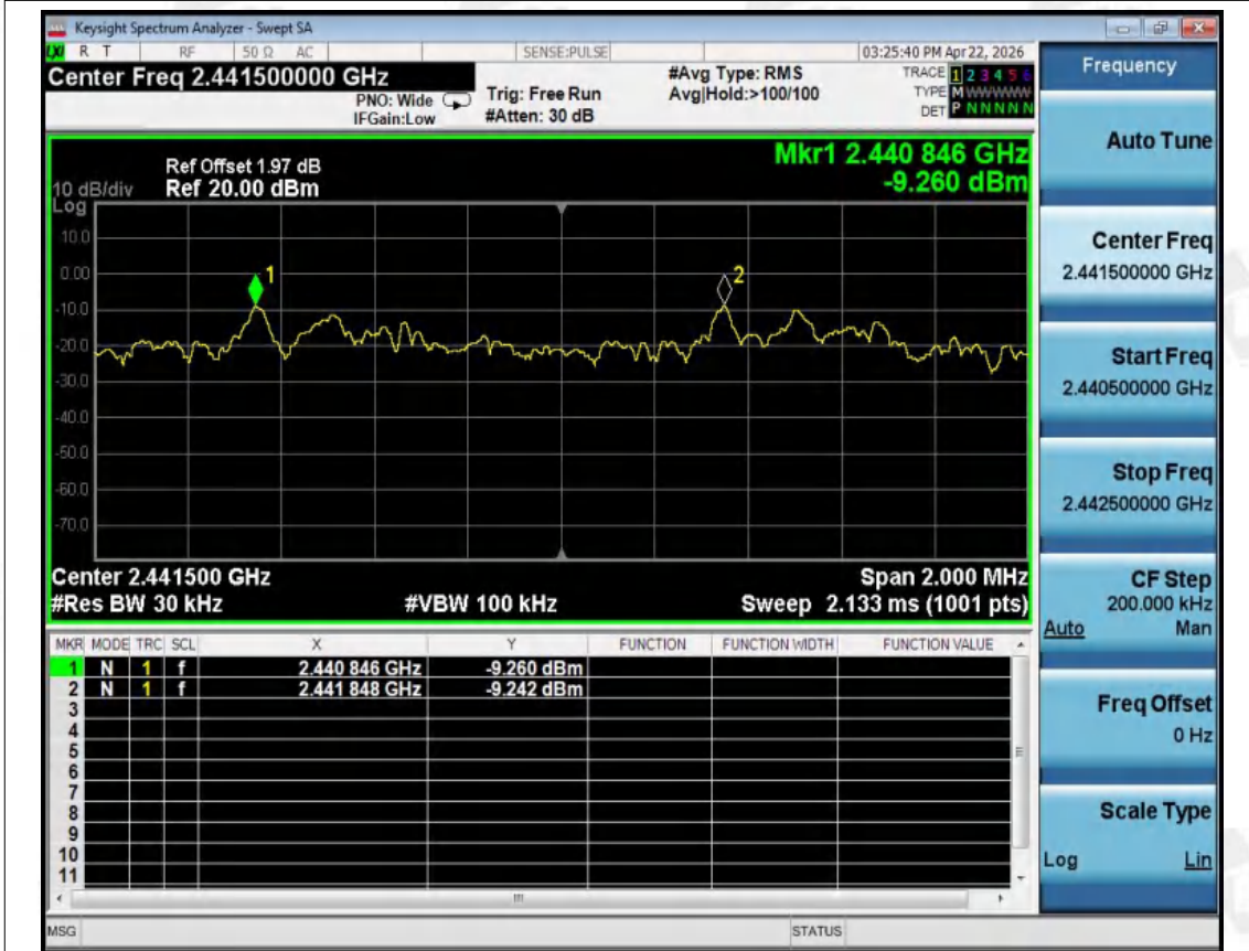
CFS NVNT 3-DH1 2441MHz Ant1
