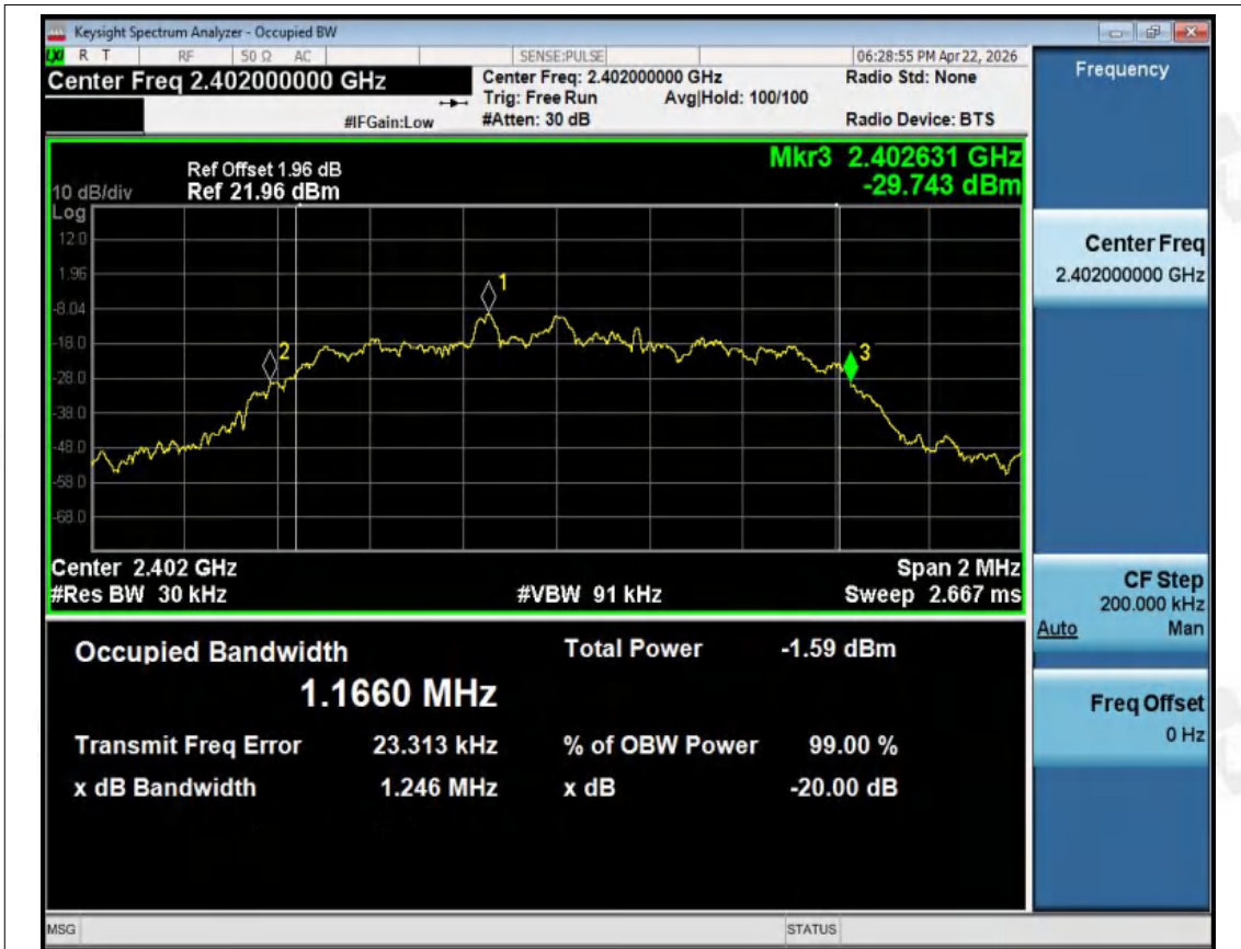
-20dB Bandwidth NVNT 3-DH1 2402MHz Ant1
