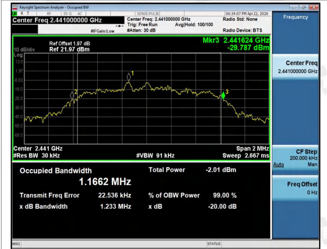
-20dB Bandwidth NVNT 3-DH1 2441MHz Ant1
