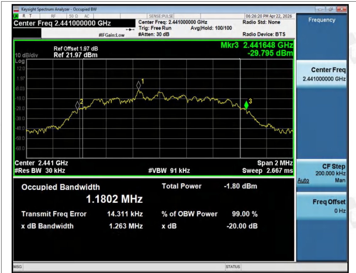
-20dB Bandwidth NVNT 2-DH1 2441MHz Ant1
