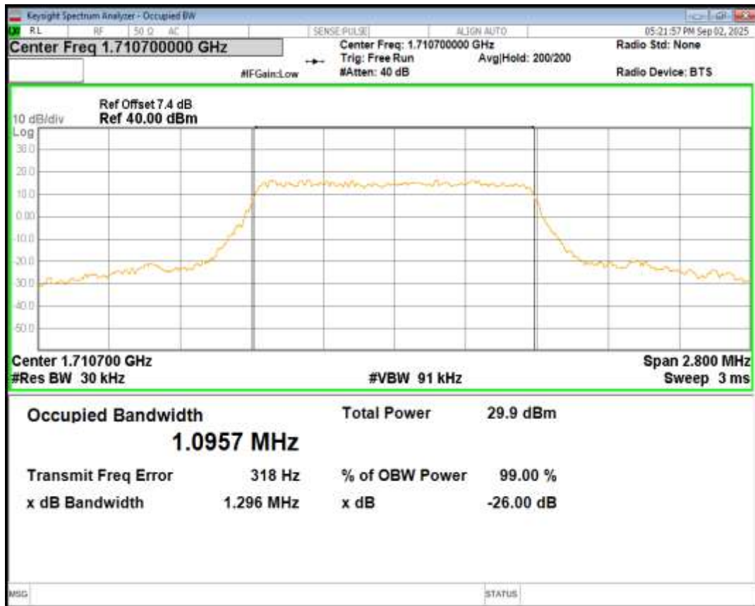
Band66 QPSK BW=1.4MHz Channel=132322 RB Size=6 Position=#0
