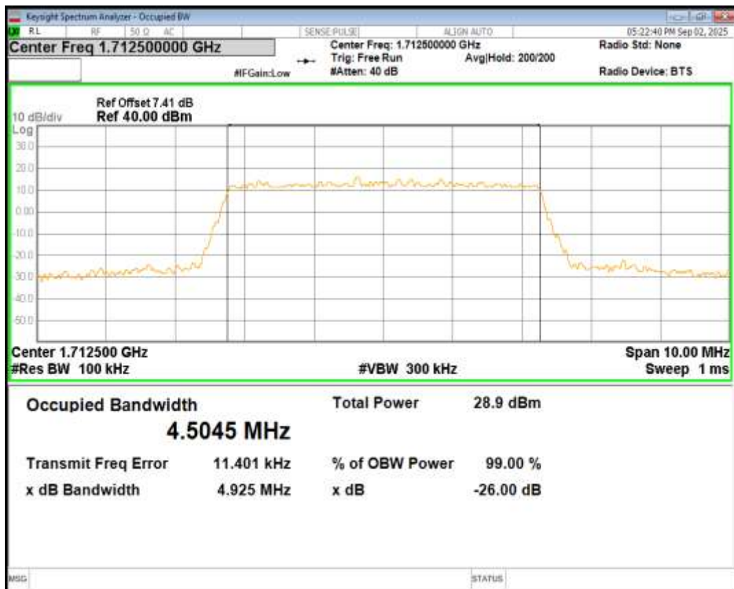
Band66 16QAM BW=5MHz Channel=132322 RB Size=25 Position=#0
