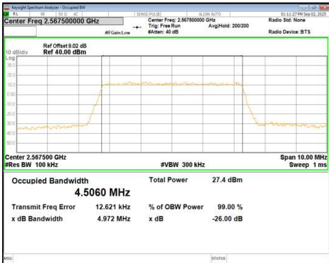
Band7 16QAM BW=20MHz Channel=21100 RB Size=100 Position=#0
