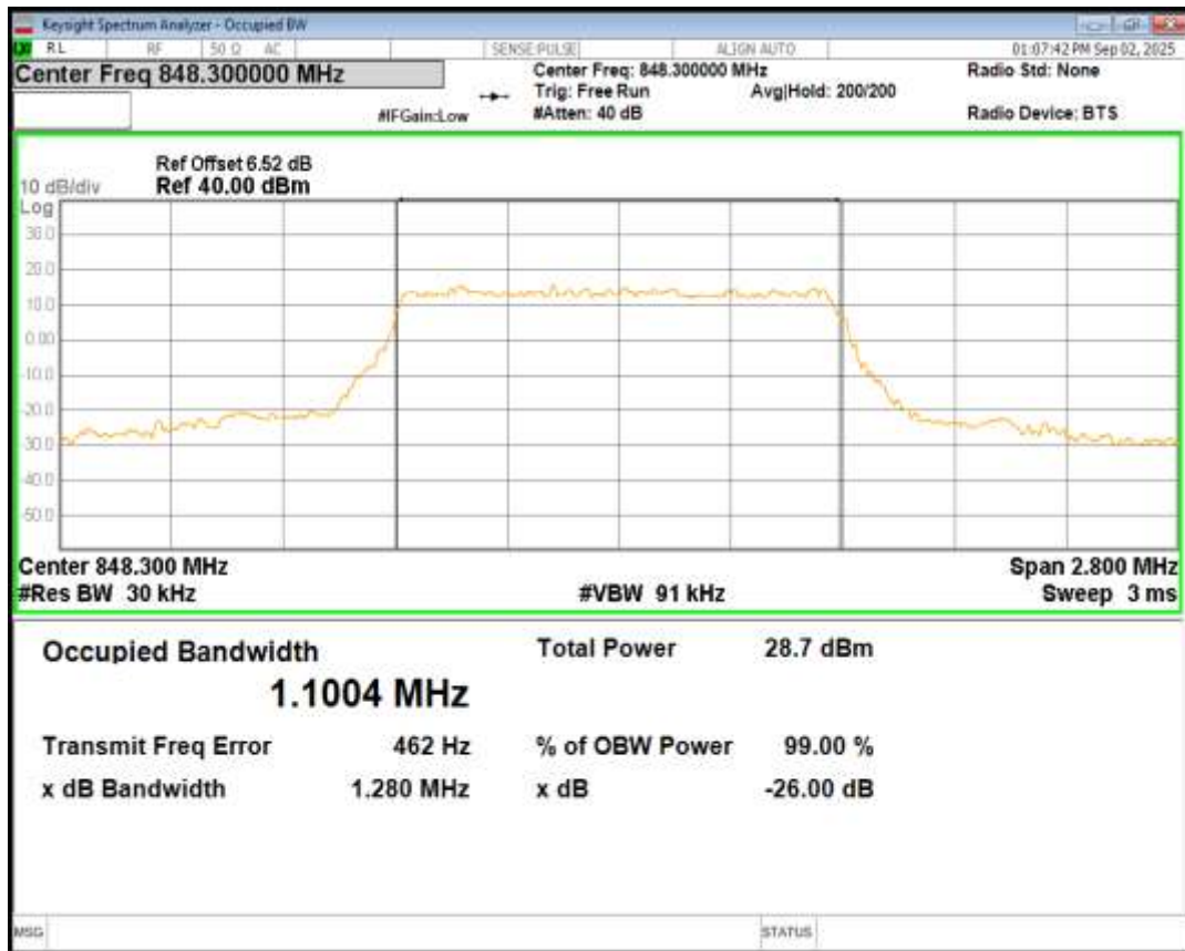
Band5 16QAM BW=10MHz Channel=20450 RB Size=50 Position=#0
