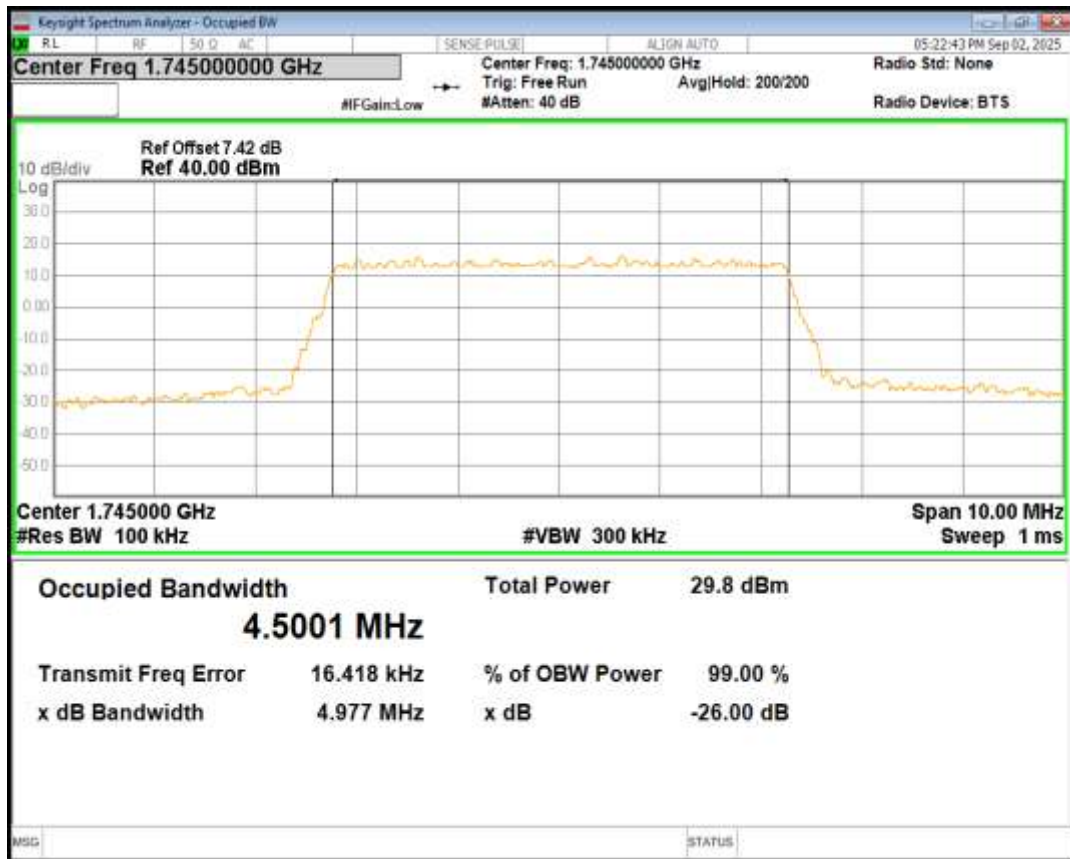
Band66 QPSK BW=3MHz Channel=132657 RB Size=15 Position=#0
