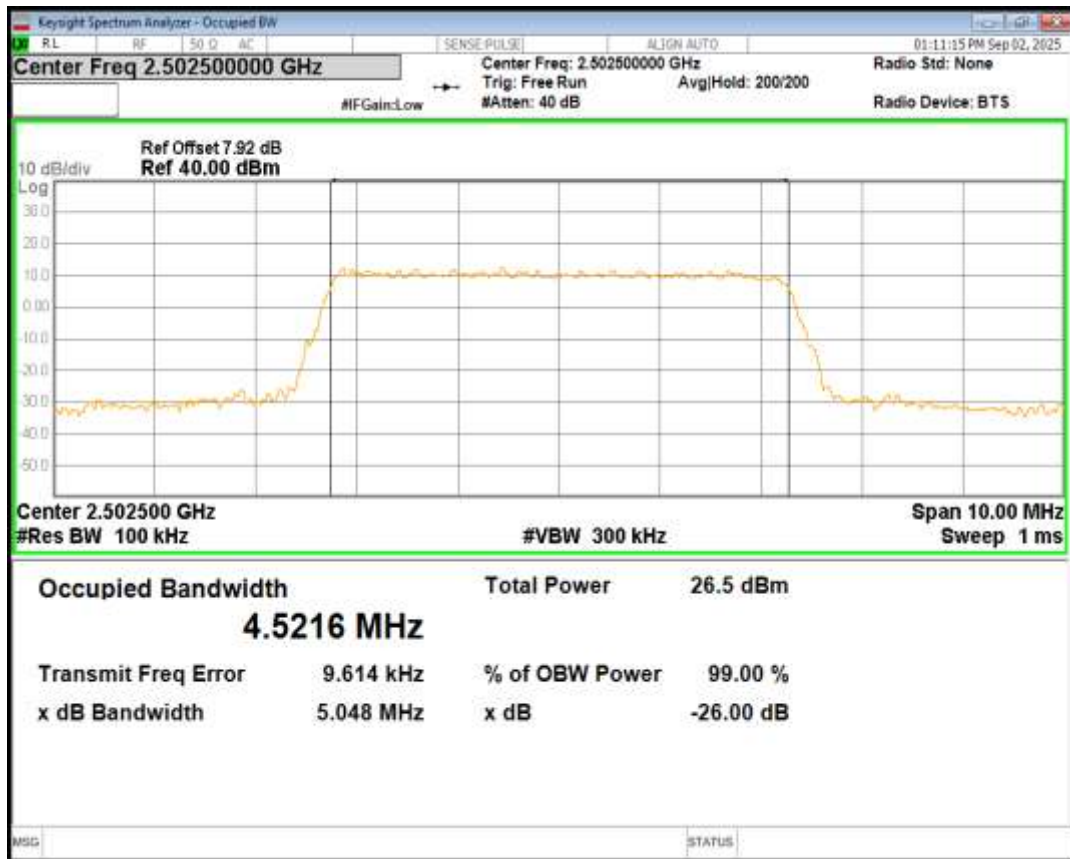
Band7 16QAM BW=5MHz Channel=21425 RB Size=25 Position=#0
