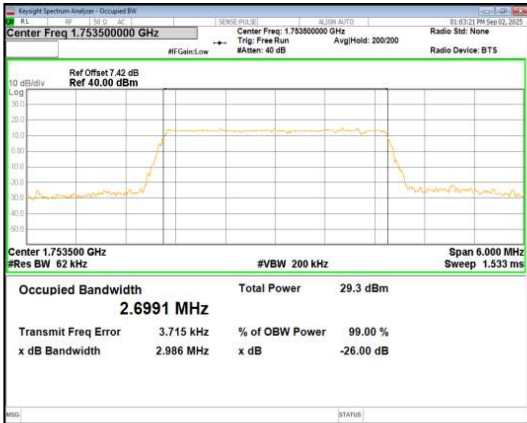
Band4 16QAM BW=5MHz Channel=19975 RB Size=25 Position=#0
