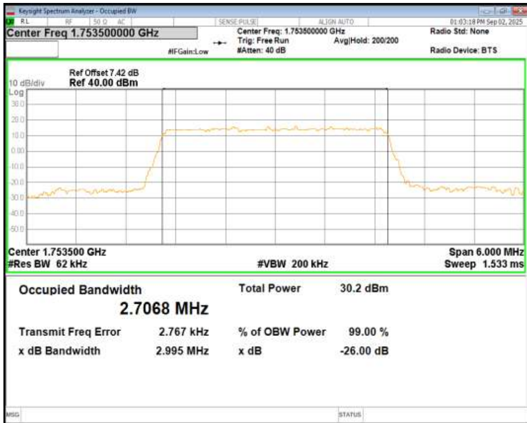
Band4 QPSK BW=5MHz Channel=19975 RB Size=25 Position=#0
