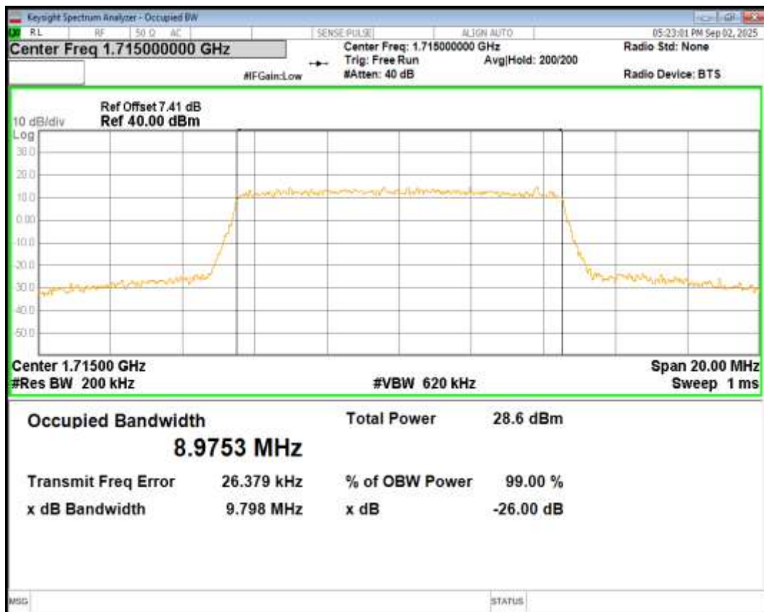
Band66 16QAM BW=10MHz Channel=132322 RB Size=50 Position=#0
