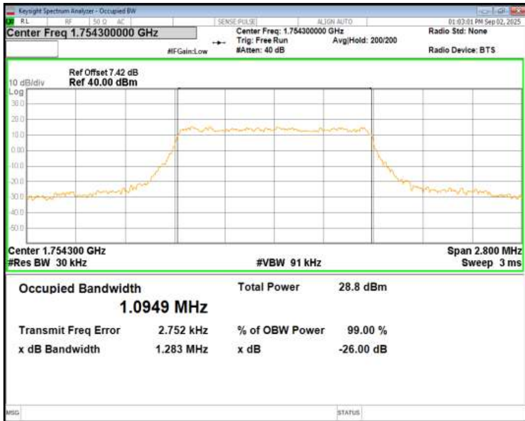
Band4 16QAM BW=10MHz Channel=20000 RB Size=50 Position=#0
