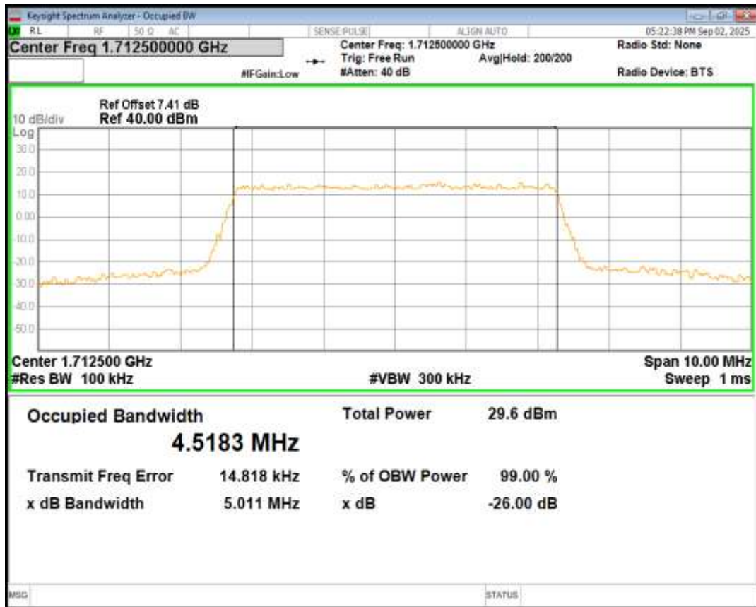
Band66 QPSK BW=5MHz Channel=132647 RB Size=25 Position=#0
