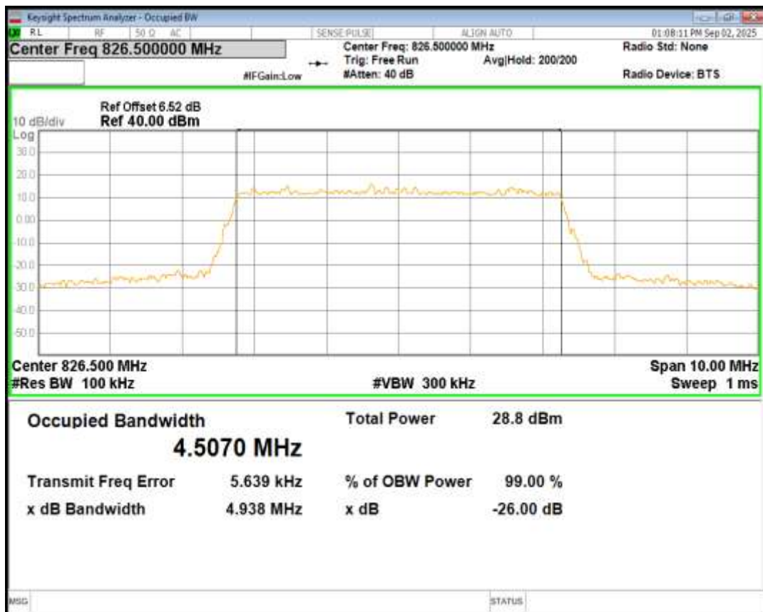
Band5 16QAM BW=5MHz Channel=20525 RB Size=25 Position=#0
