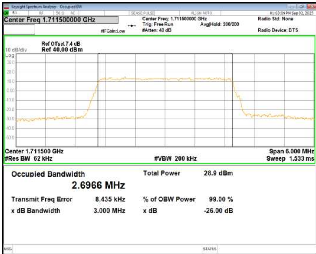
Band4 16QAM BW=3MHz Channel=20175 RB Size=15 Position=#0
