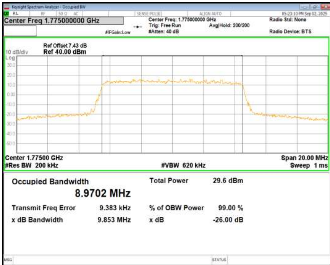
Band66 QPSK BW=20MHz Channel=132072 RB Size=100 Position=#0
