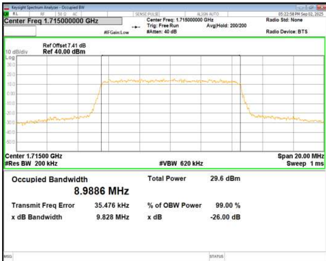
Band66 QPSK BW=15MHz Channel=132322 RB Size=75 Position=#0
