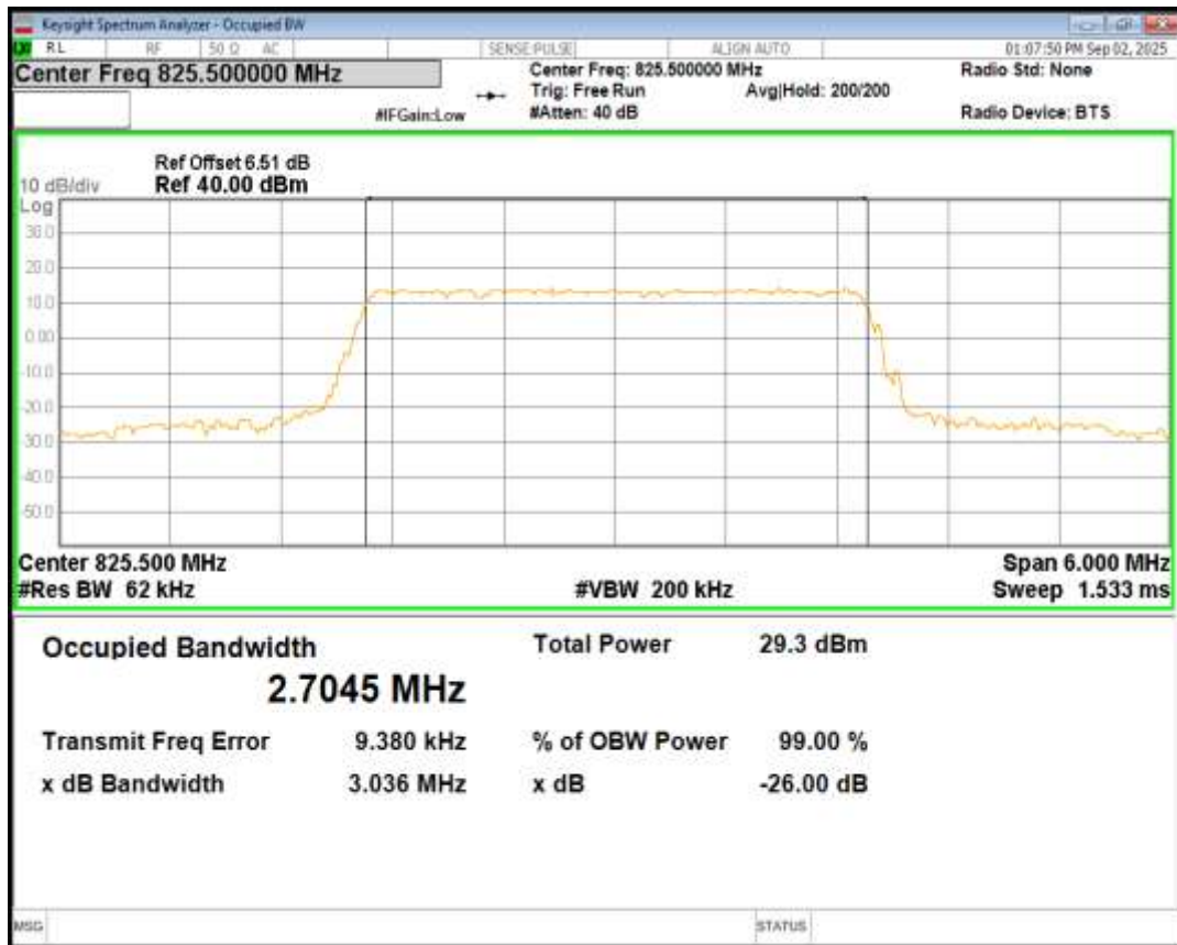
Band5 16QAM BW=3MHz Channel=20525 RB Size=15 Position=#0
