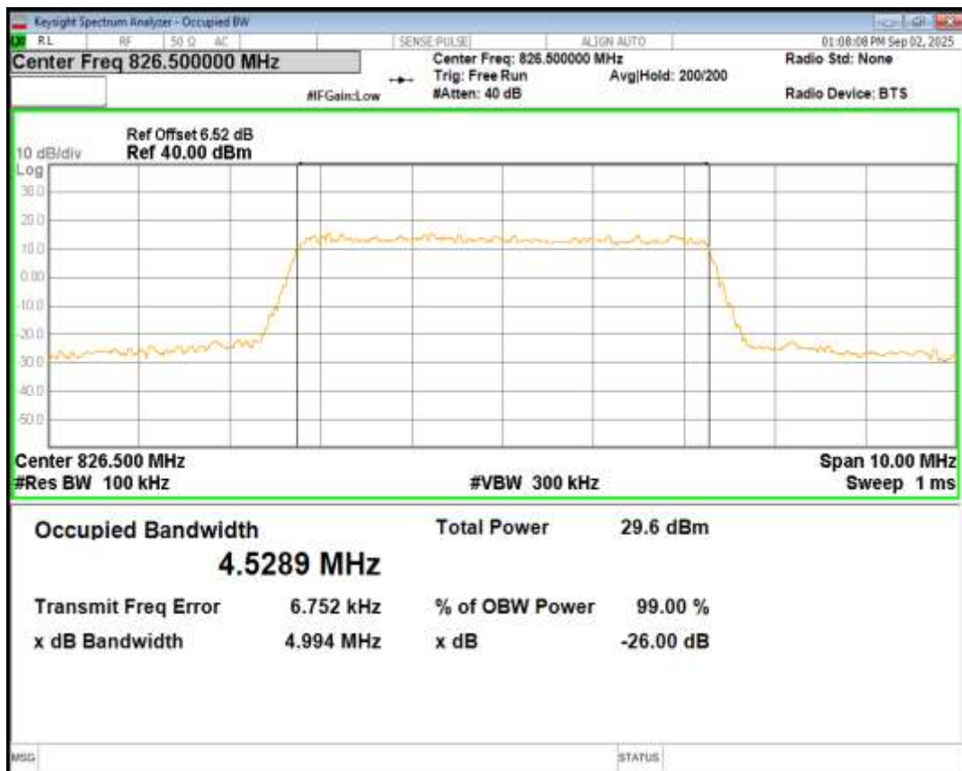
Band5 QPSK BW=5MHz Channel=20525 RB Size=25 Position=#0
