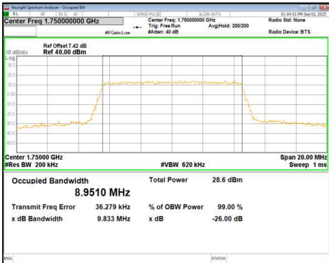
Band4 16QAM BW=15MHz Channel=20025 RB Size=75 Position=#0
