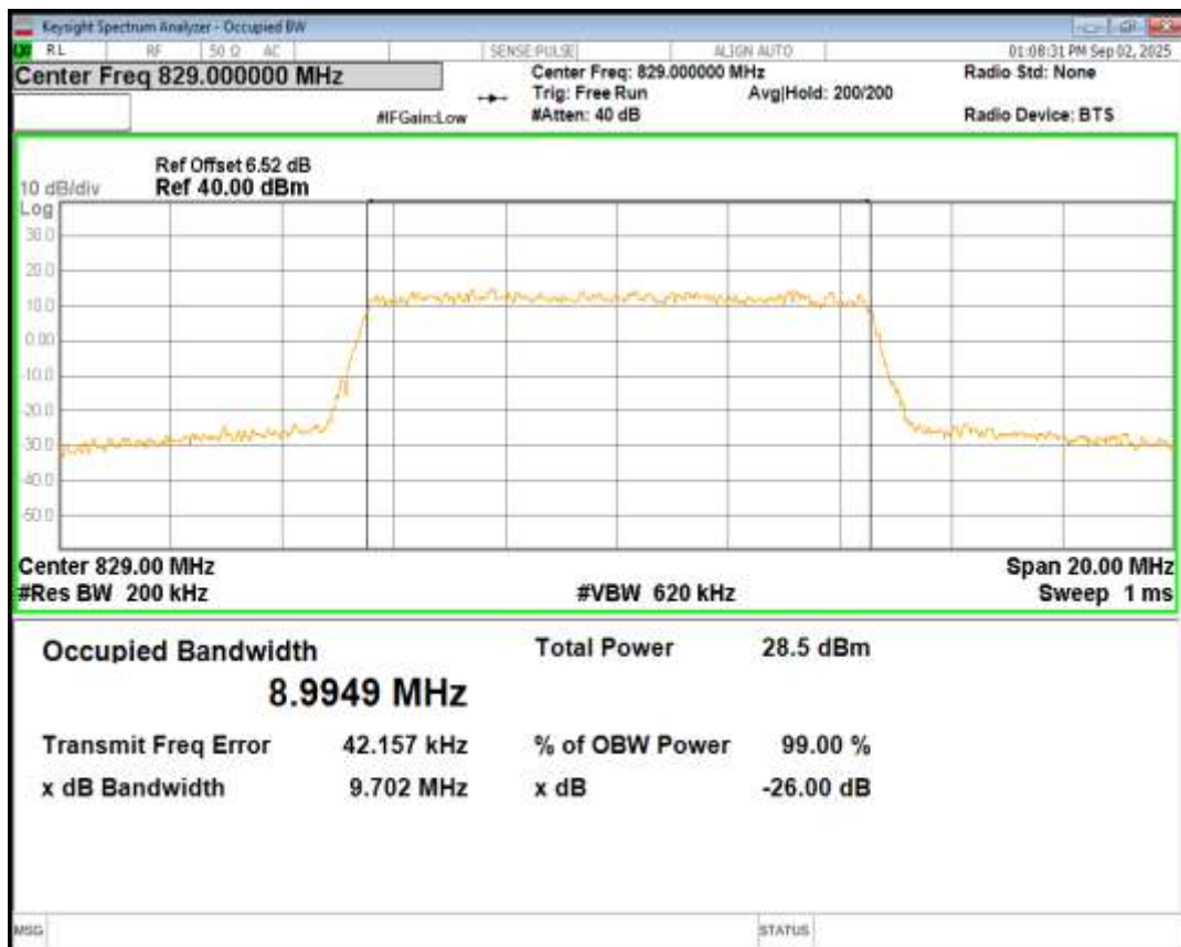
Band5 16QAM BW=10MHz Channel=20525 RB Size=50 Position=#0
