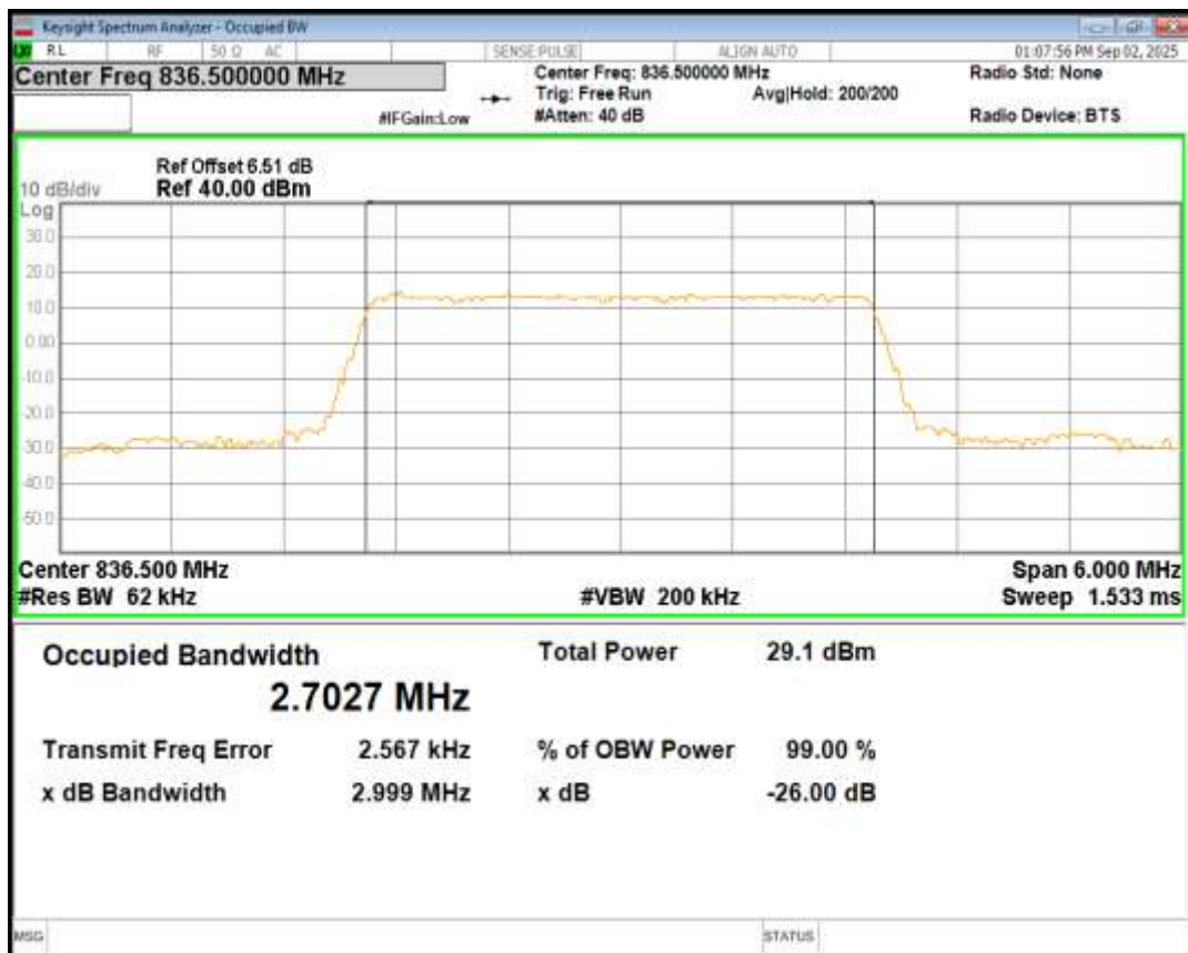
Band5 16QAM BW=3MHz Channel=20635 RB Size=15 Position=#0
