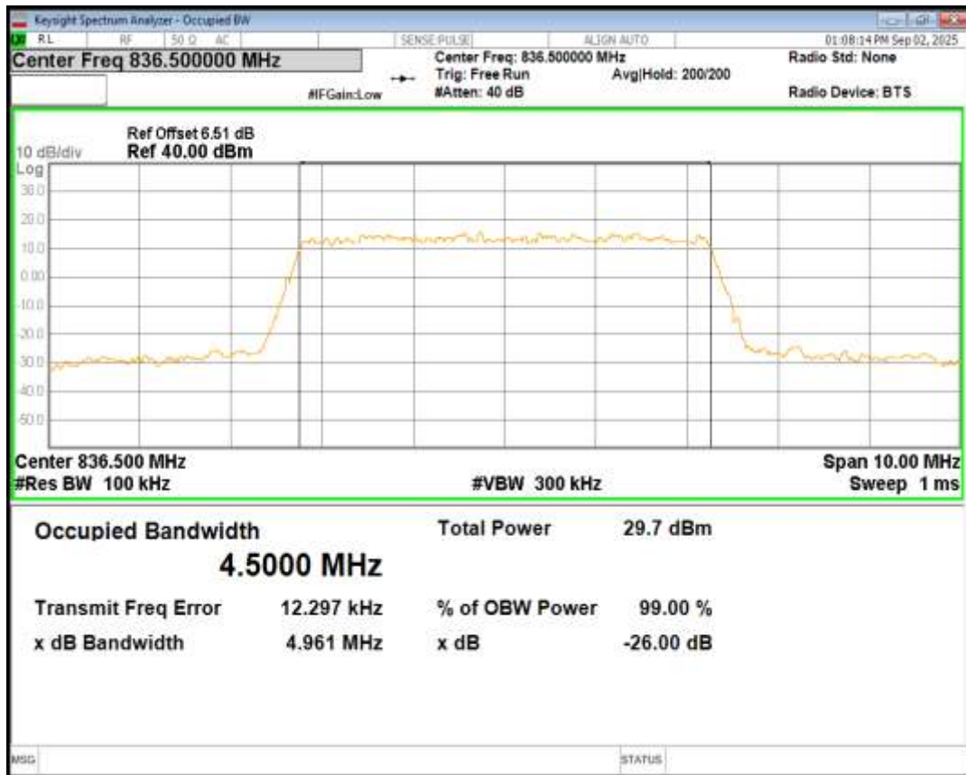
Band5 QPSK BW=5MHz Channel=20625 RB Size=25 Position=#0
