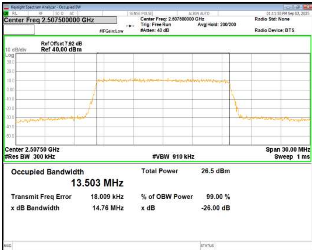
Band7 16QAM BW=15MHz Channel=21100 RB Size=75 Position=#0
