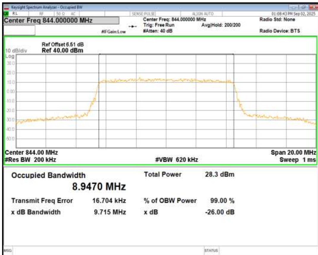
Band5 16QAM BW=3MHz Channel=20415 RB Size=15 Position=#0
