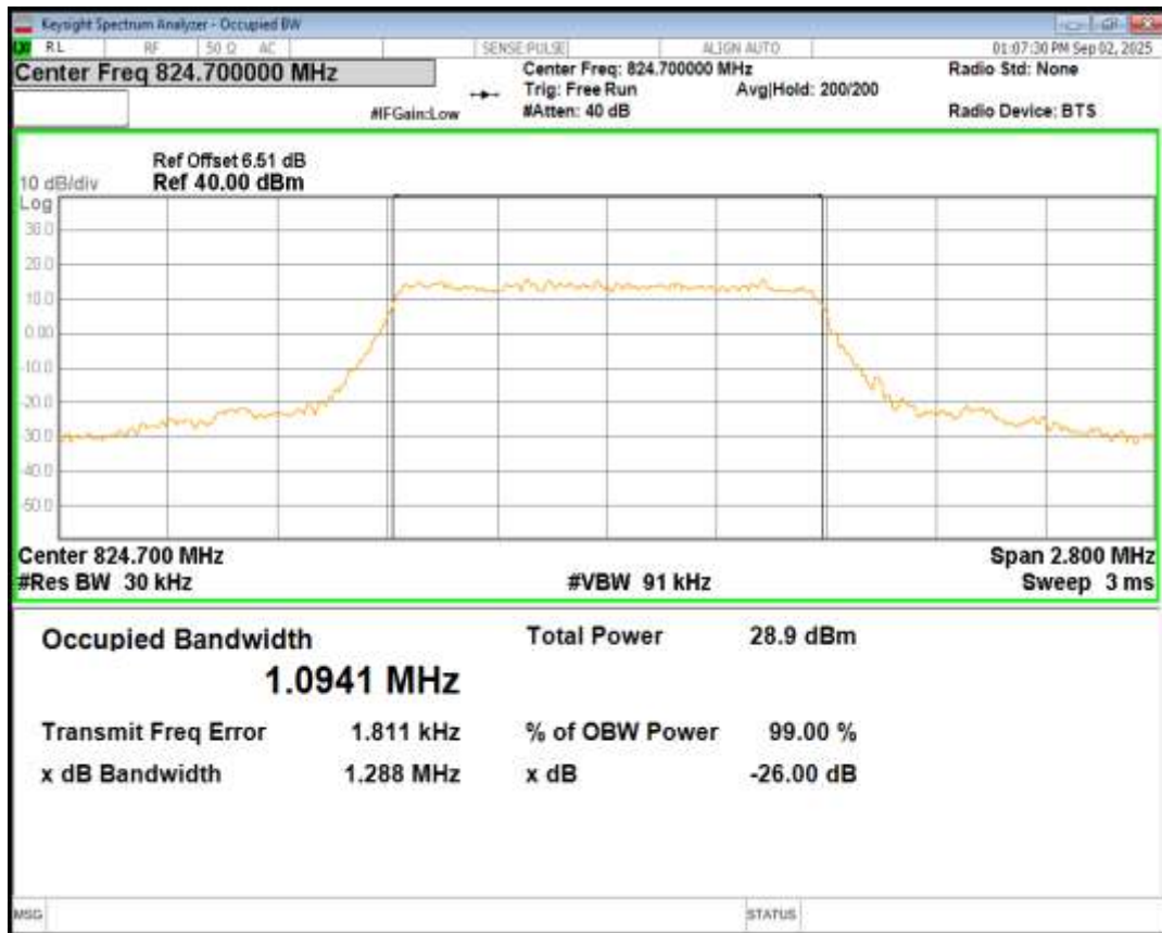
Band5 16QAM BW=1.4MHz Channel=20525 RB Size=6 Position=#0
