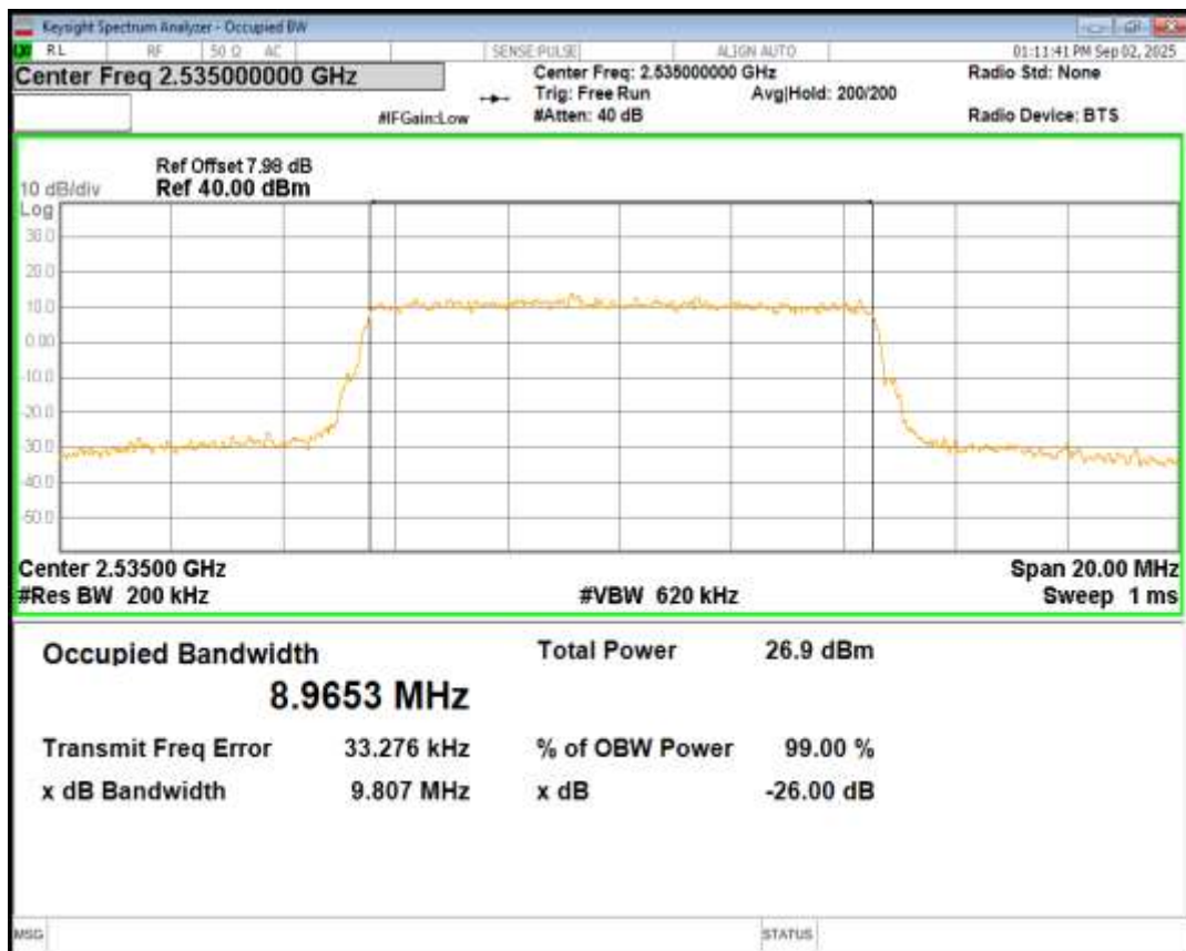
Band7 16QAM BW=10MHz Channel=21400 RB Size=50 Position=#0
