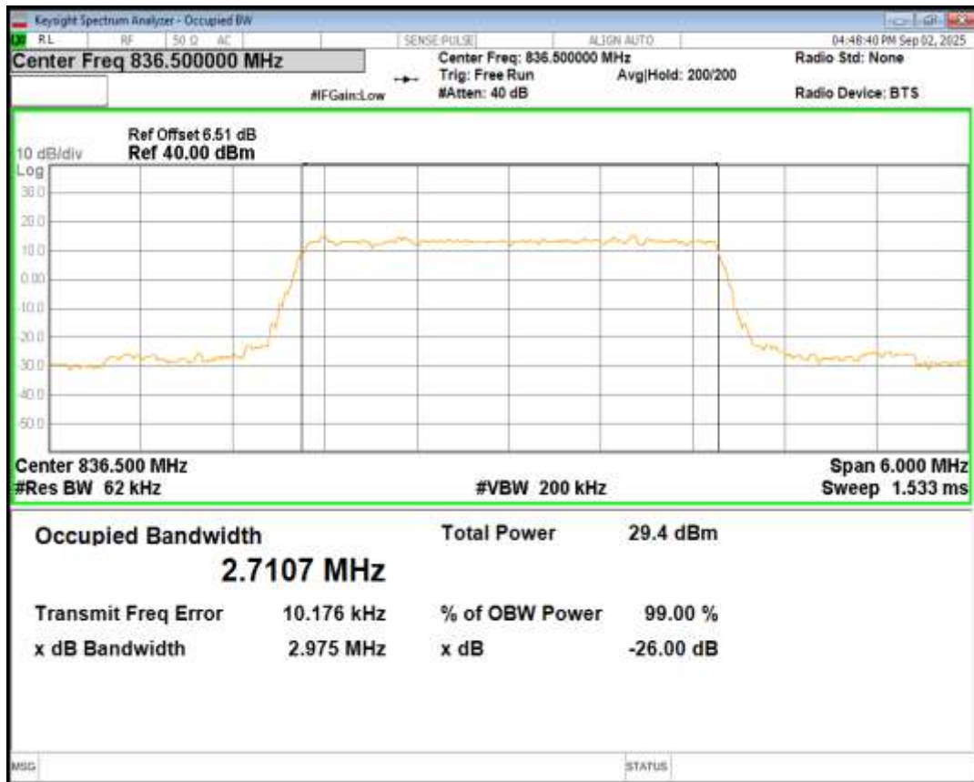
Band26(824-849) QPSK BW=3MHz Channel=27025 RB Size=15 Position=#0
