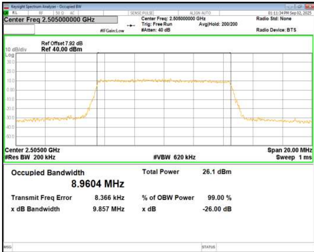
Band7 16QAM BW=10MHz Channel=21100 RB Size=50 Position=#0
