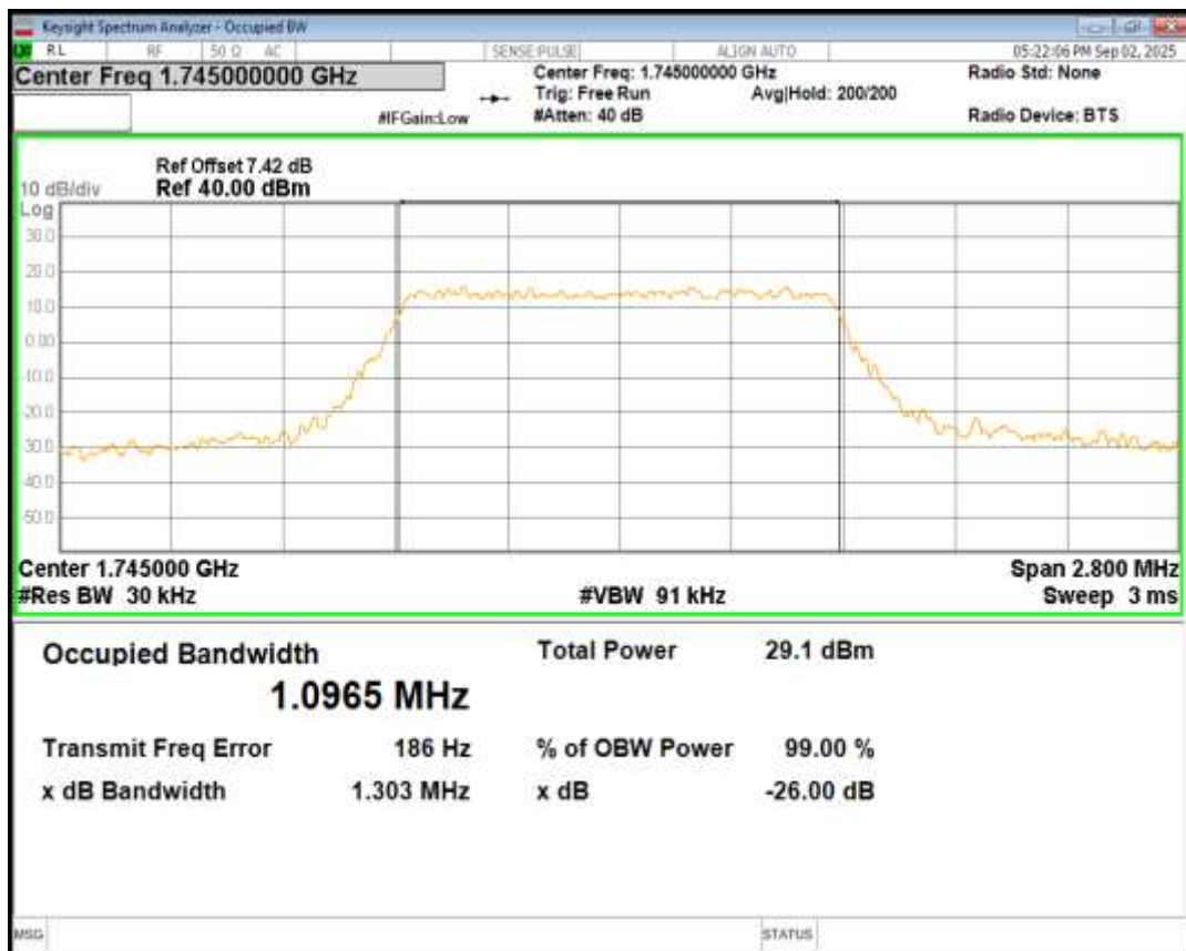
Band66 16QAM BW=1.4MHz Channel=132665 RB Size=6 Position=#0
