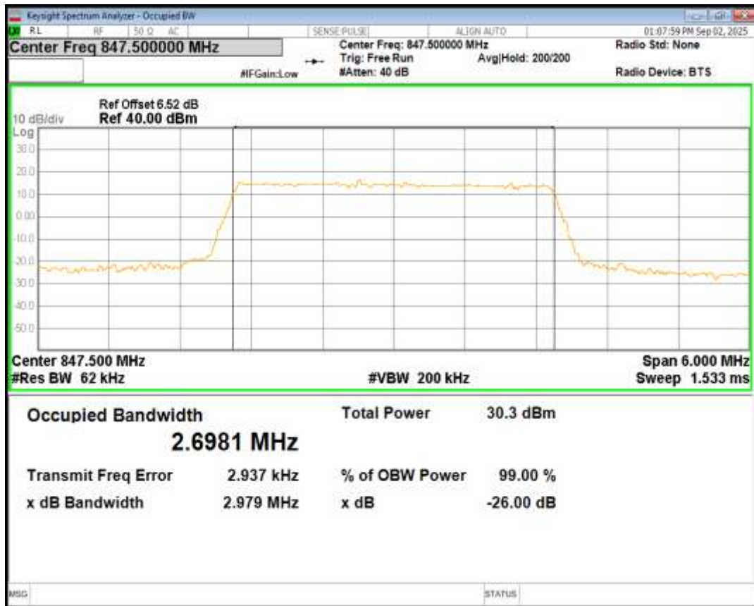
Band5 QPSK BW=5MHz Channel=20425 RB Size=25 Position=#0
