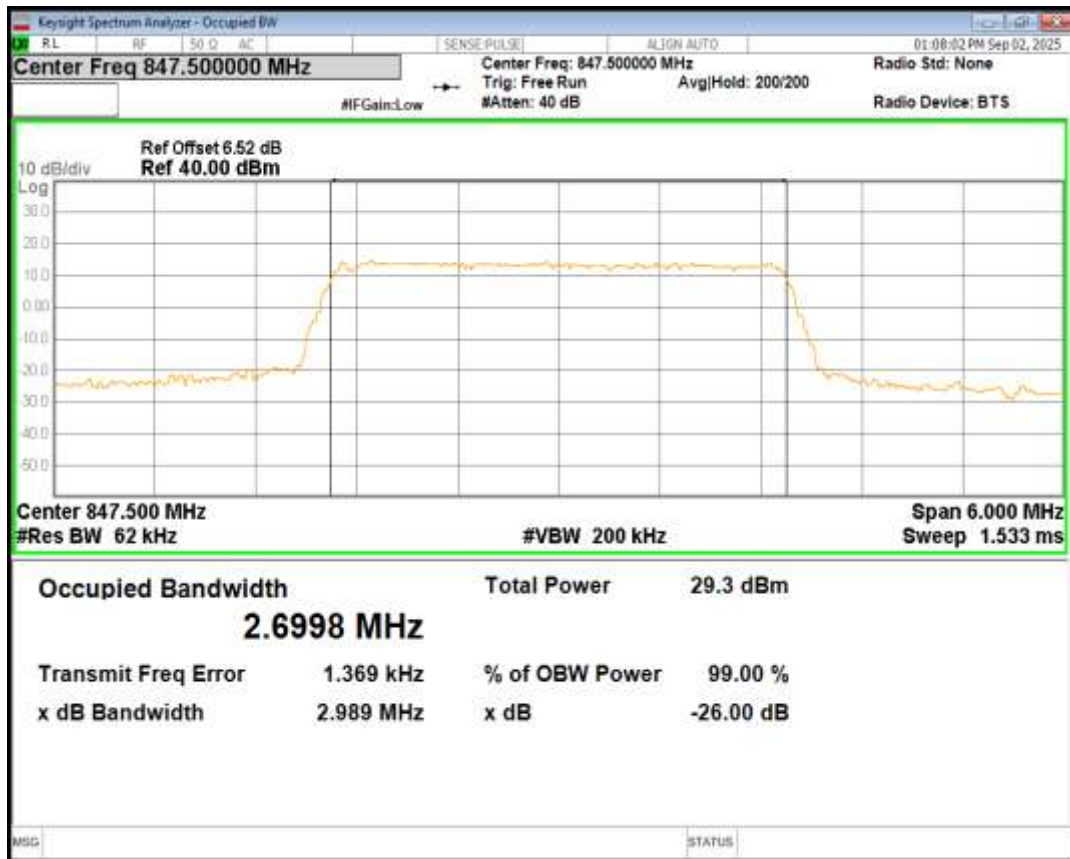
Band5 16QAM BW=5MHz Channel=20425 RB Size=25 Position=#0
