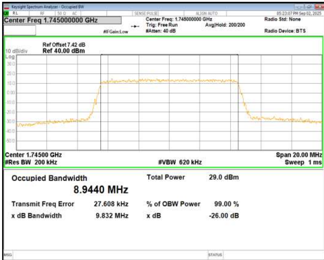
Band66 16QAM BW=10MHz Channel=132622 RB Size=50 Position=#0
