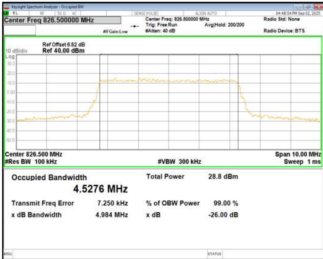
Band26(824-849) QPSK BW=5MHz Channel=27015 RB Size=25 Position=#0
