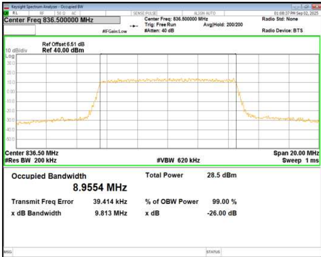
Band5 16QAM BW=10MHz Channel=20600 RB Size=50 Position=#0
