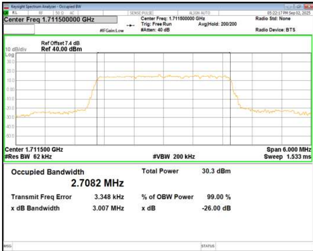
Band66 QPSK BW=3MHz Channel=132322 RB Size=15 Position=#0
