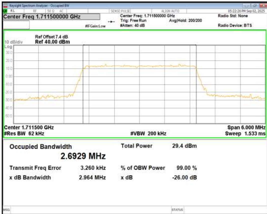
Band66 16QAM BW=3MHz Channel=132322 RB Size=15 Position=#0
