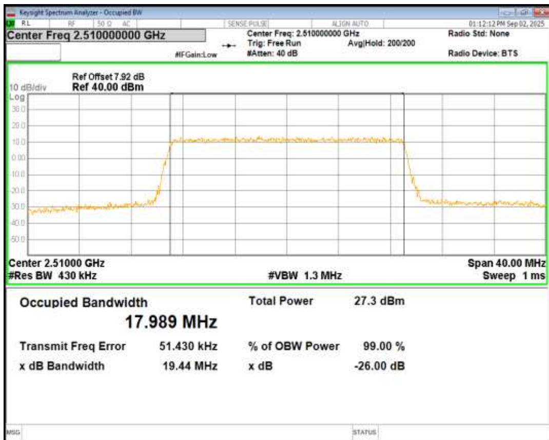
Band7 QPSK BW=20MHz Channel=21100 RB Size=100 Position=#0
