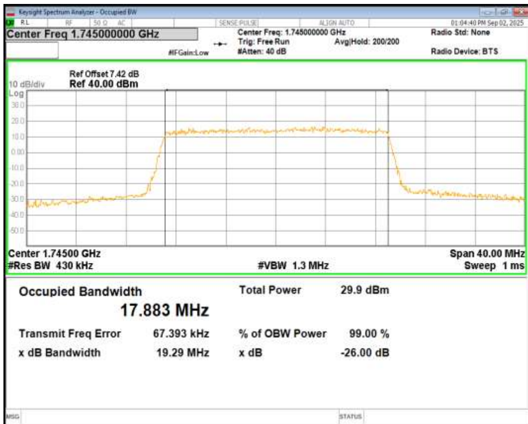
Band4 QPSK BW=3MHz Channel=19965 RB Size=15 Position=#0
