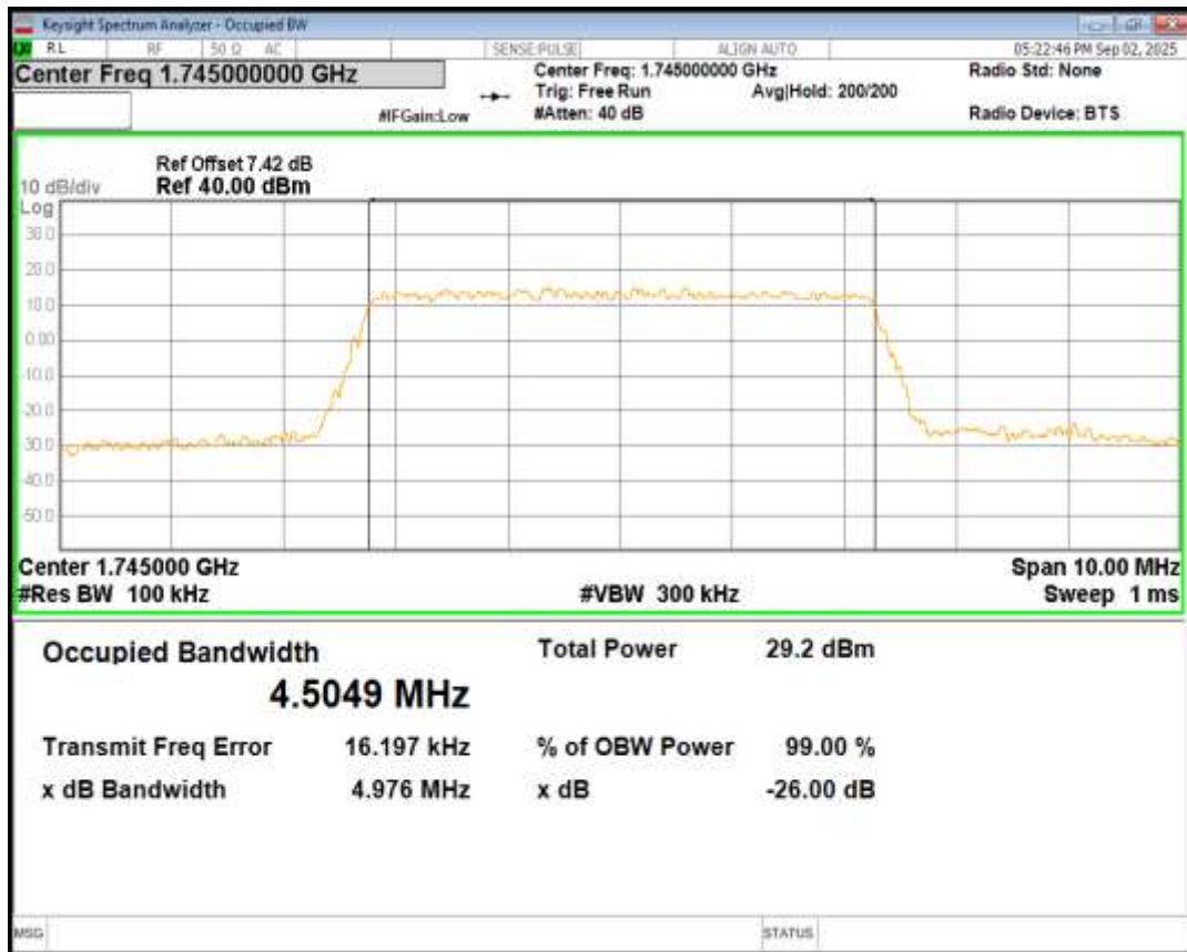
Band66 16QAM BW=5MHz Channel=132647 RB Size=25 Position=#0
