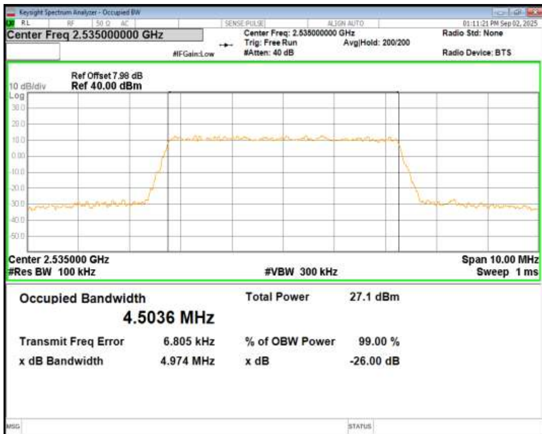
Band7 16QAM BW=5MHz Channel=20775 RB Size=25 Position=#0
