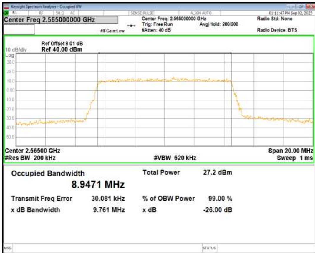
Band7 16QAM BW=15MHz Channel=20825 RB Size=75 Position=#0
