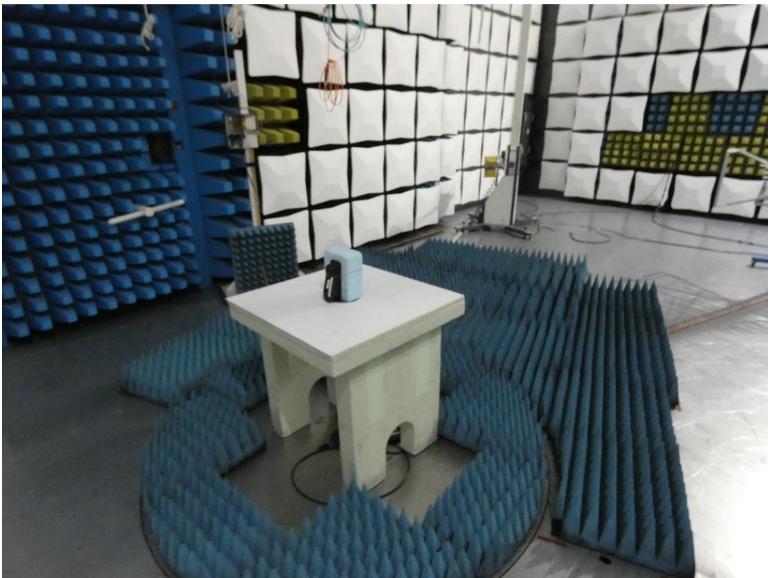
Photo 2: Test setup (stand alone setup) for radiated emissions measurements - above 1 GHz in the semi anechoic room (SAR)
