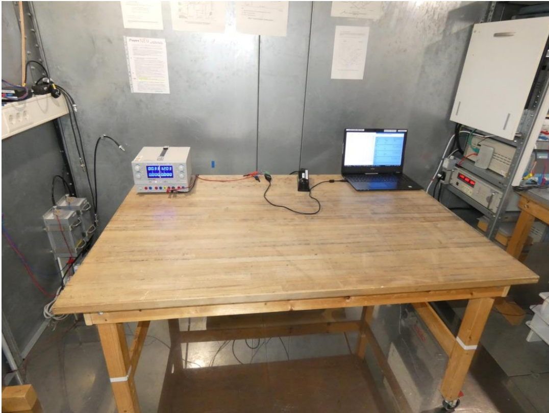
Photo 3: Test setup with Setup S01_AB01 for conducted emissions measurements below 30 MHz
