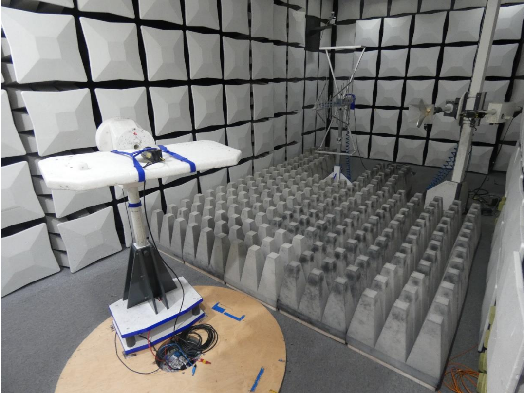
Photo 5: Test setup for radiated emissions measurements up to 26 GHz in the fully anechoic room (FAR)
