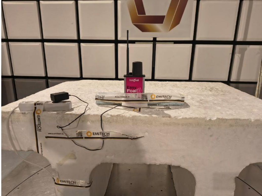
Test setup with charger
