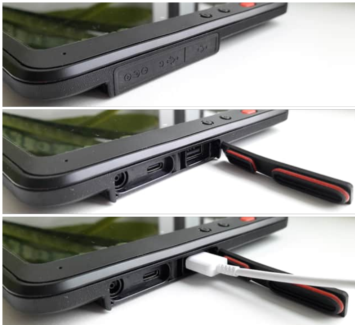
Figure 4.16: Connecting EASEE® Connect to EASEE® Set – Hardware: The USB port of EASEE® Set is located behind a lateral cover on the left side of the housing.
