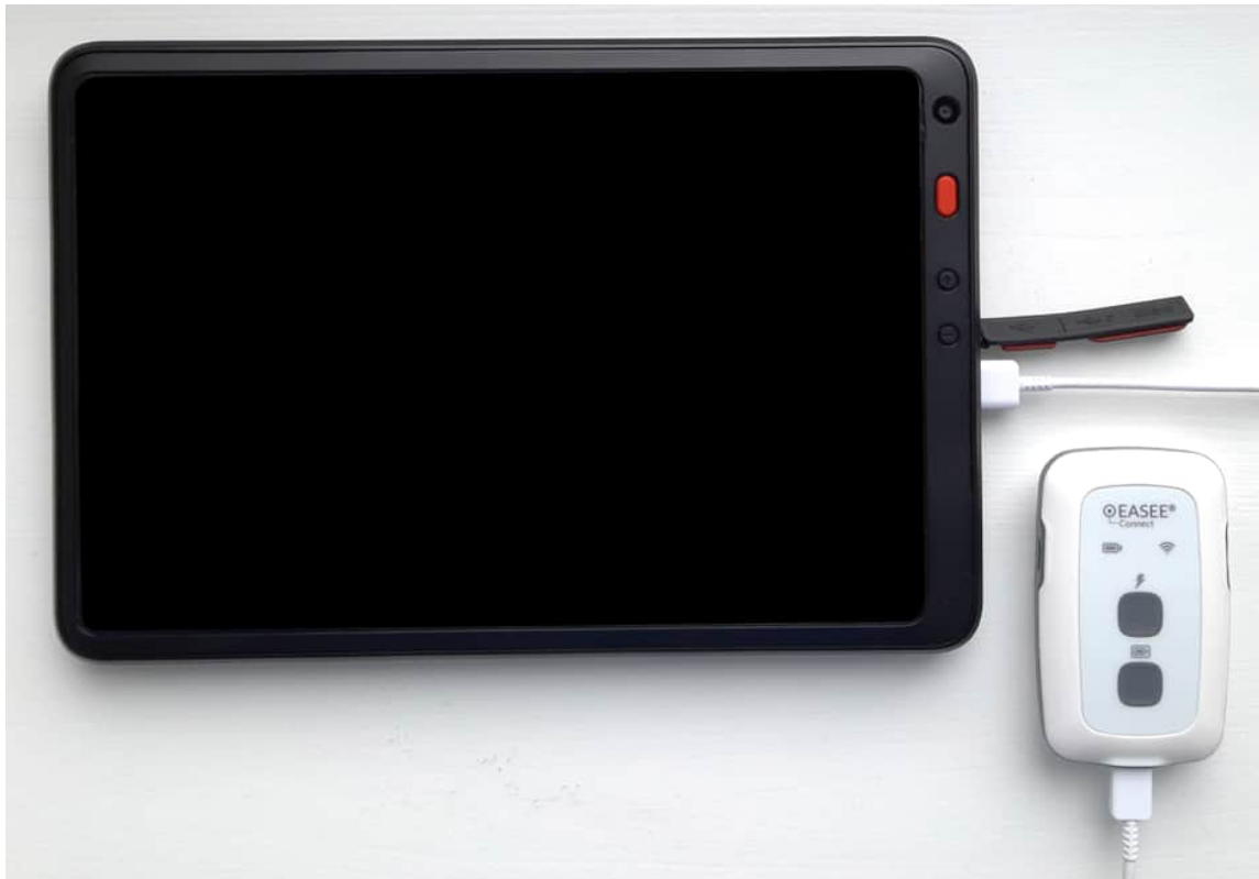
Figure 2.10: EASEE® Set / EASEE® Connect is the combination of EASEE® Set (left) and EASEE® Connect (right).
