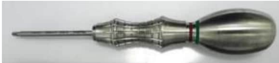
Figure 2.6: Screwdriver used for fixation of EASEE® Lead via bone screws (example for illustration only).
