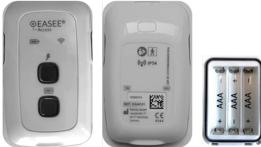
Figure 2.11: Front view (left) and rear view (middle) of EASEE® Access. Right side: Battery compartment open.
