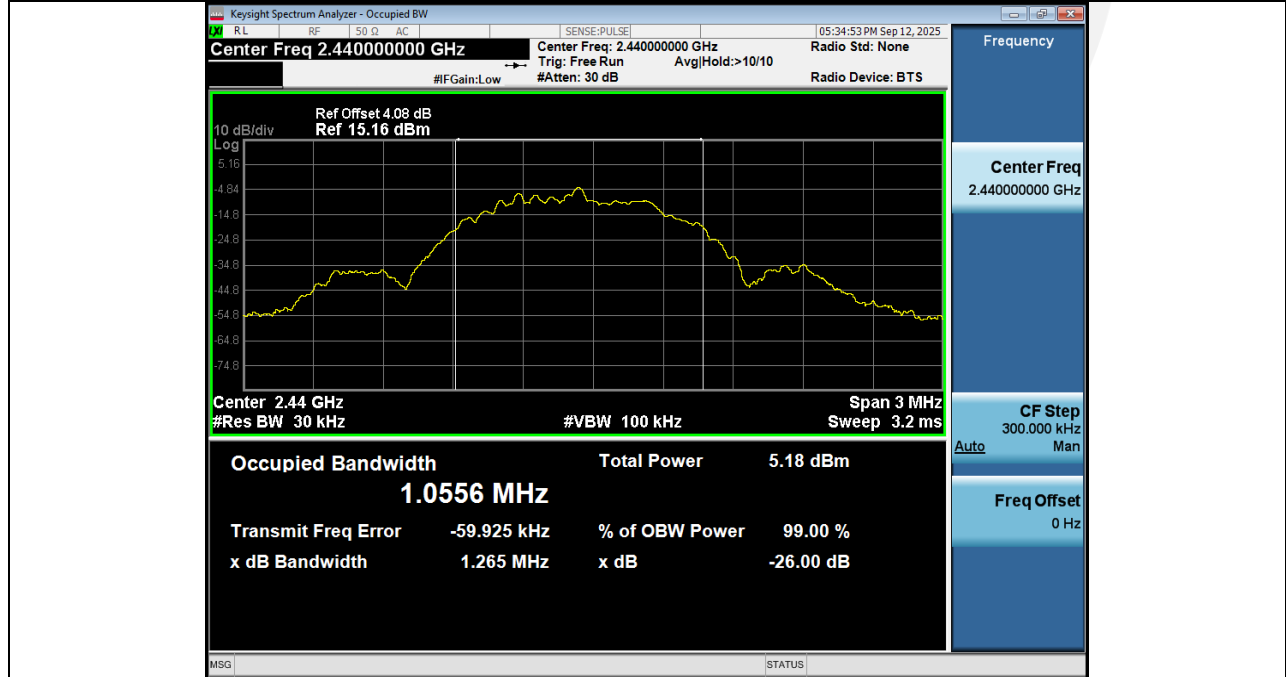
99% Occupied Bandwidth NVNT ANT1 1Mbps 2440
