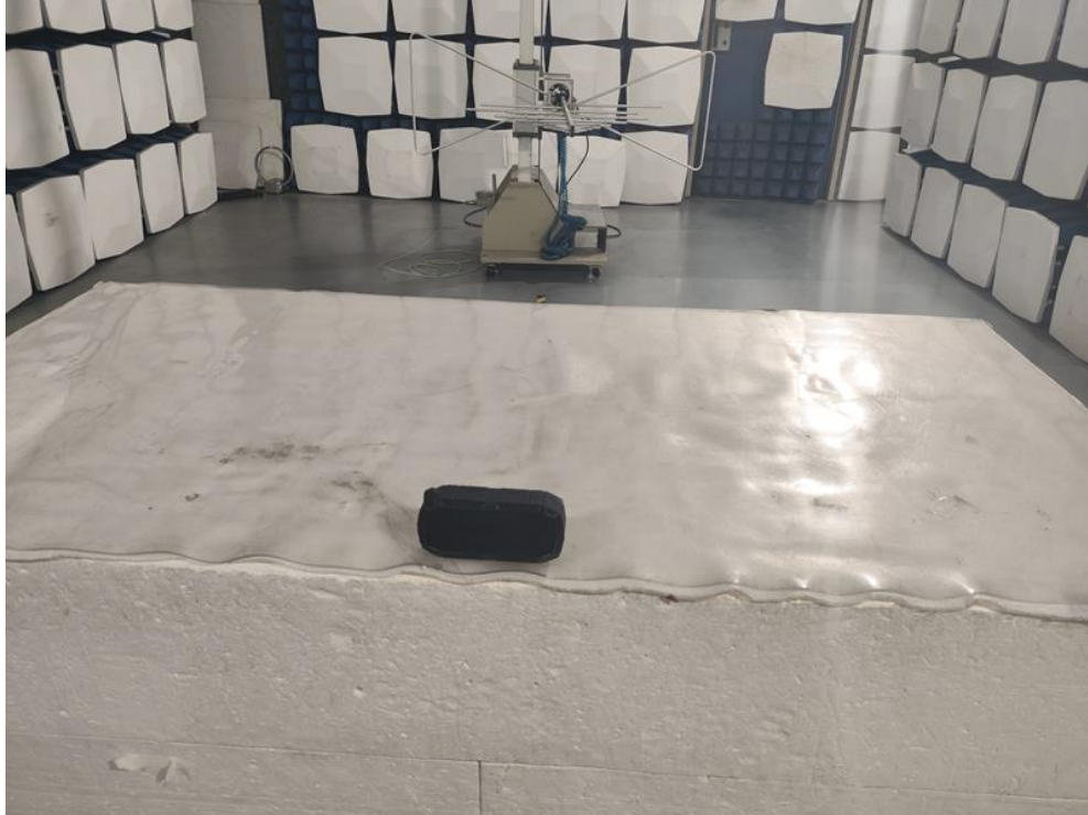
Radiated Emission Test Setup:
