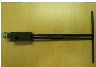
Figure 1 – MVG COMOSAR Validation Dipole
