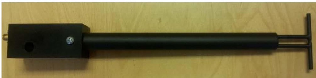
Figure 1 – MVG COMOSAR Validation Dipole
