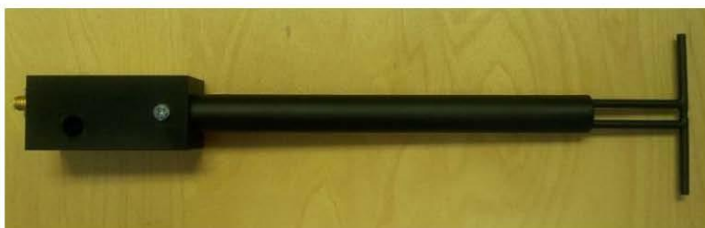
Figure 1 – MVG COMOSAR Validation Dipole
