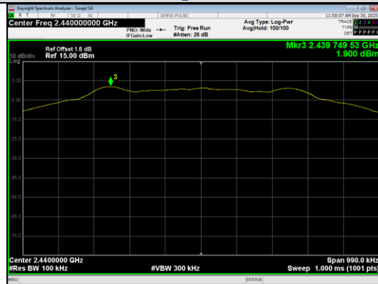
In-Band Reference Level BLE 1M_Channel 19
