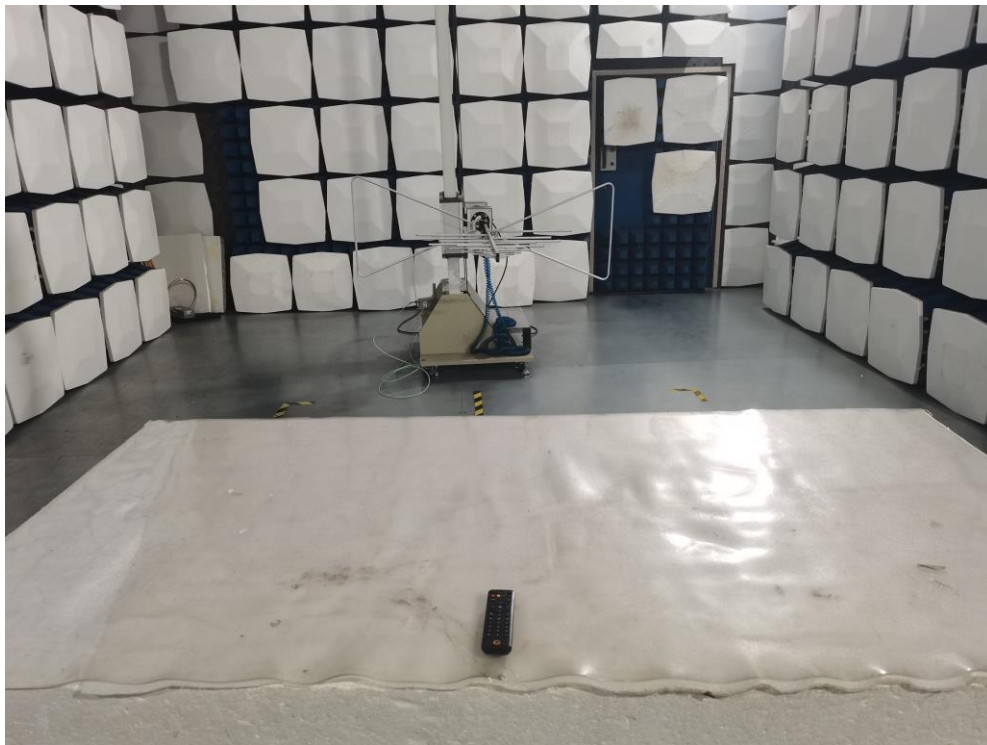
Radiated Emission Test Setup:
