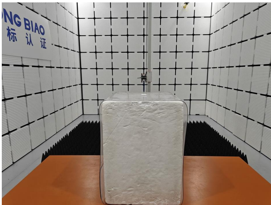
Radiated Emission Above 1GHz
