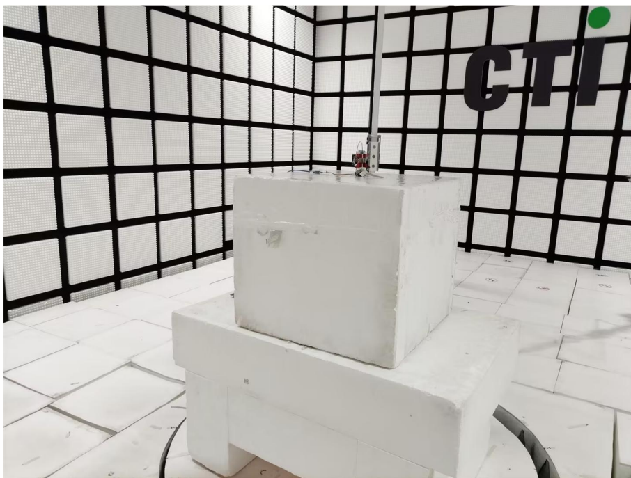
Radiated spurious emission Test Setup-3(Above 1GHz)
