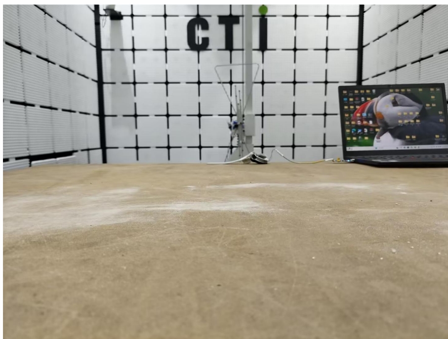
Radiated spurious emission Test Setup-2(Below 1GHz)
