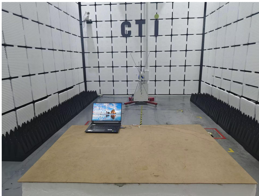
Radiated spurious emission Test Setup-1(Below 1GHz)
