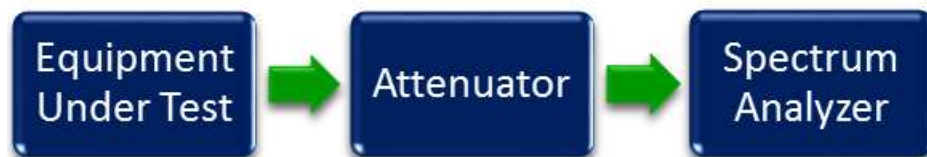
Figure 4. Conducted Spurious Emissions Test Setup
