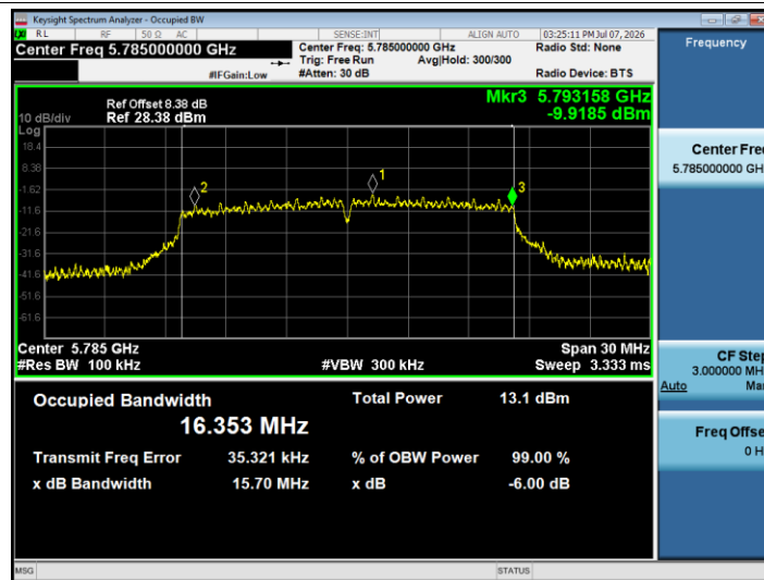
-6dB Bandwidth NVNT a 5785MHz Ant1
