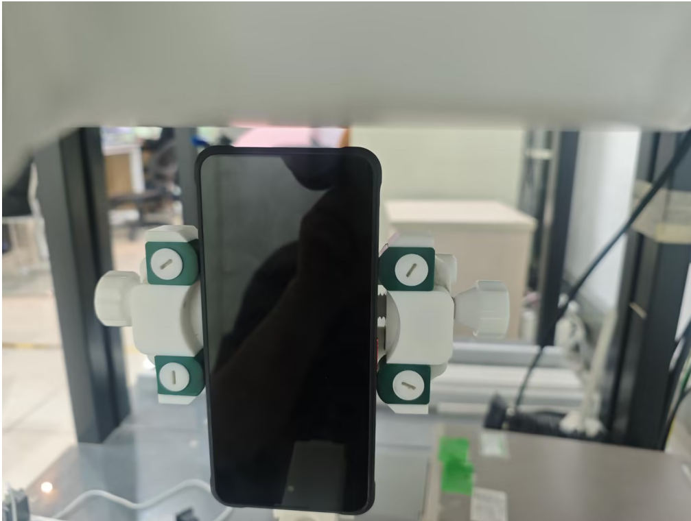
Body Bottom side(separation distance is 10mm)
