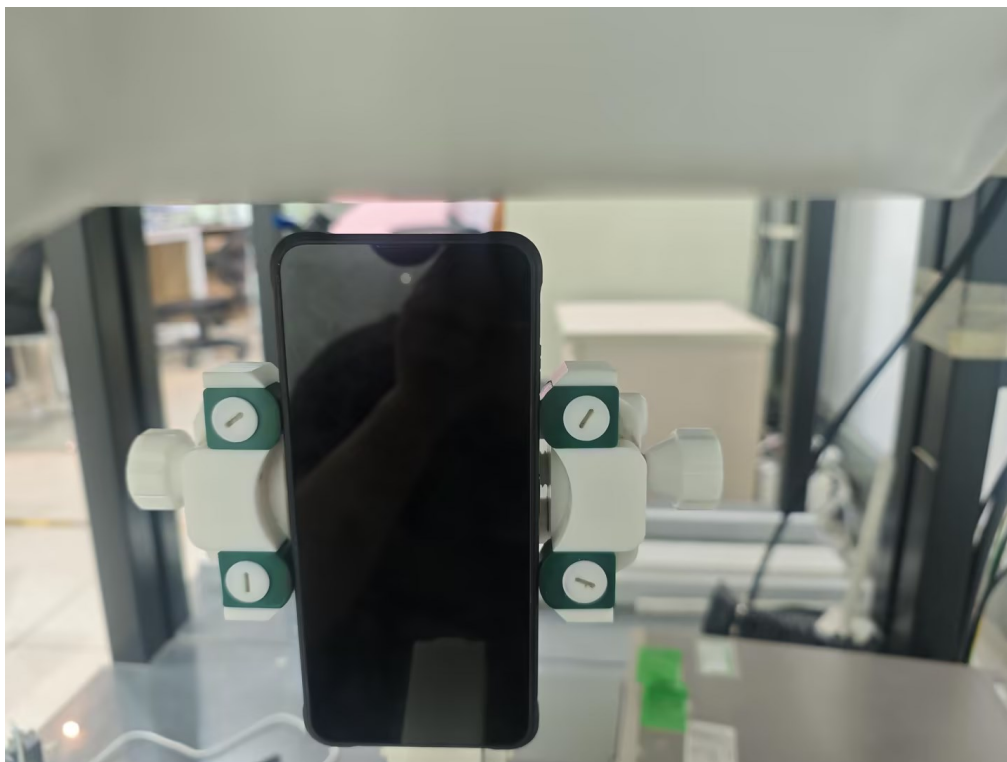
Body Top side(separation distance is 10mm)
