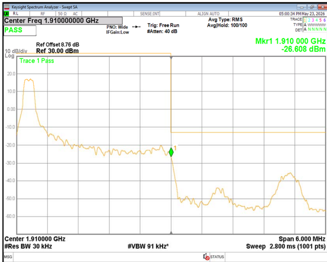
Band2 16QAM BW=3MHz Channel=19185 RB Size=1 Position=#Max
