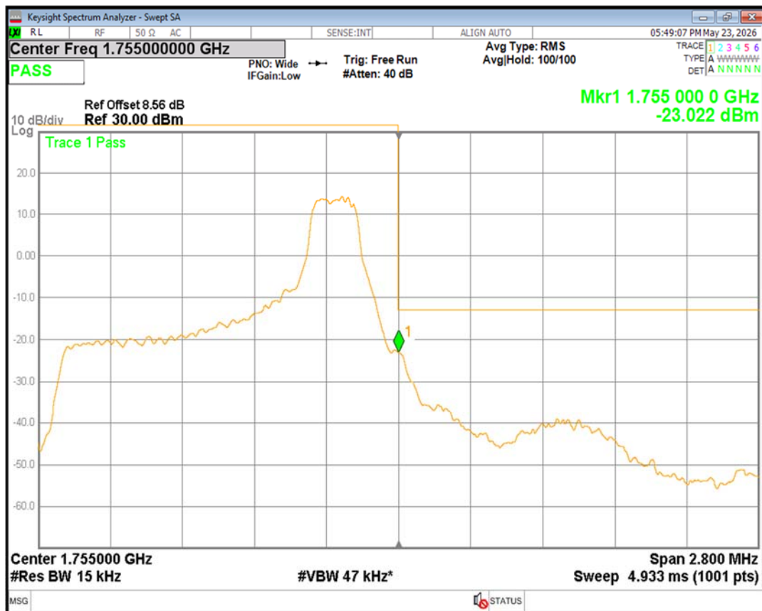
Band4 QPSK BW=1.4MHz Channel=20393 RB Size=6 Position=#0
