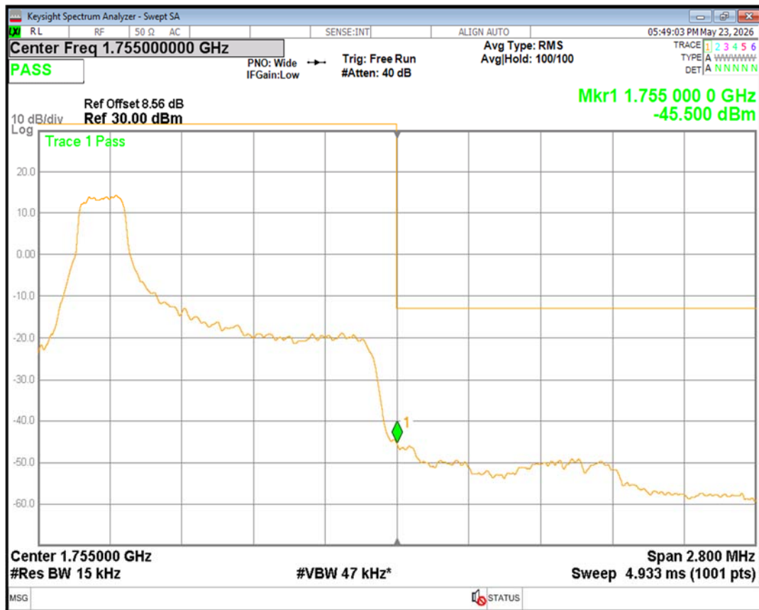
Band4 QPSK BW=1.4MHz Channel=20393 RB Size=1 Position=#Max
