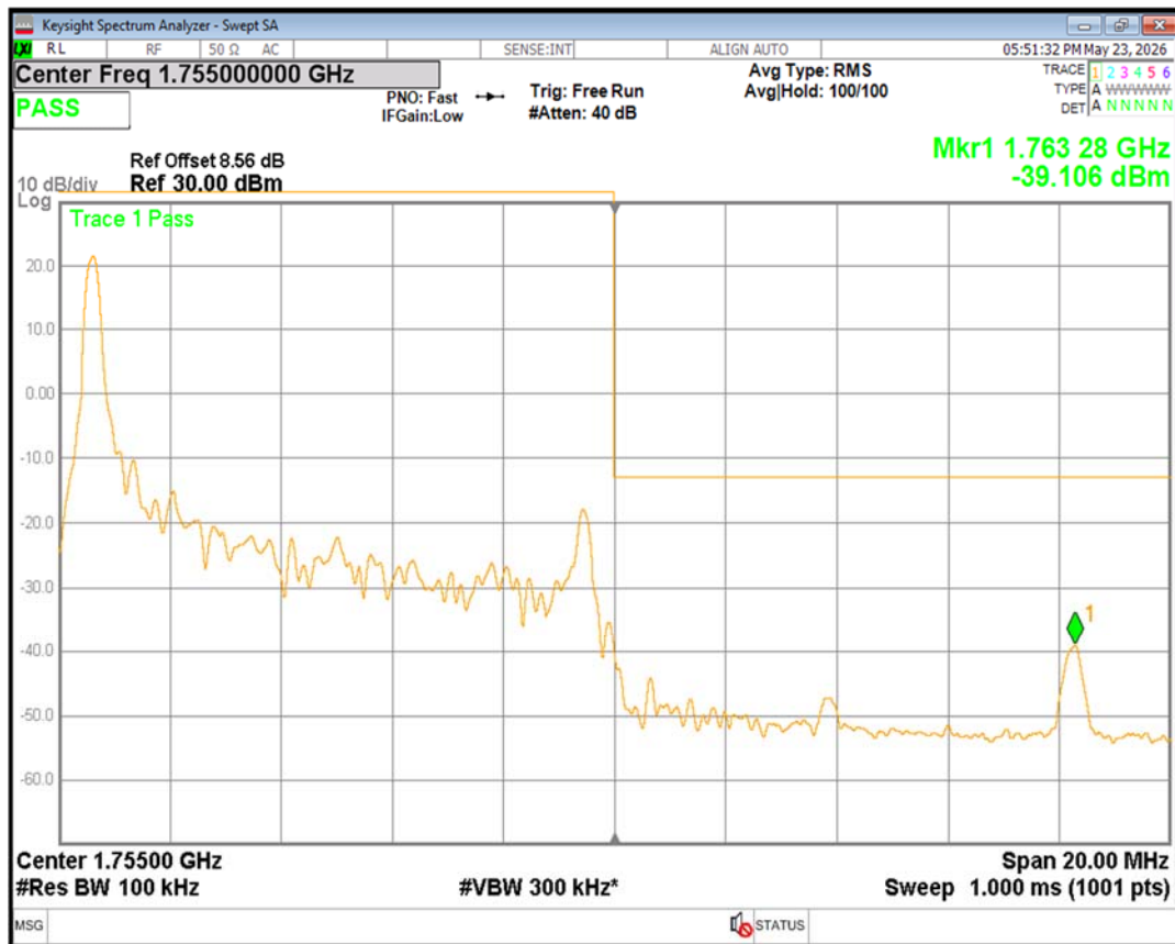
Band4 16QAM BW=10MHz Channel=20350 RB Size=1 Position=#Max
