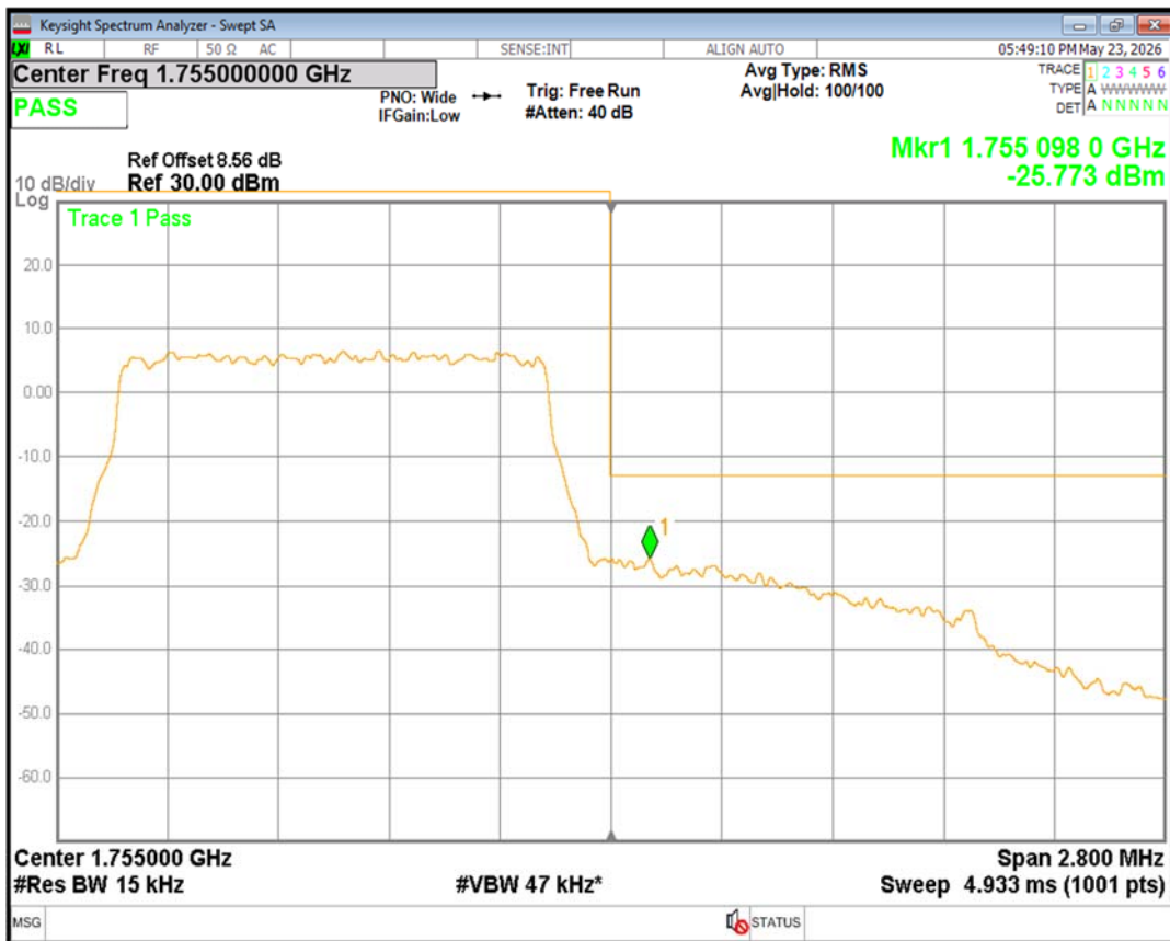
Band4 QPSK BW=10MHz Channel=20000 RB Size=1 Position=#0
