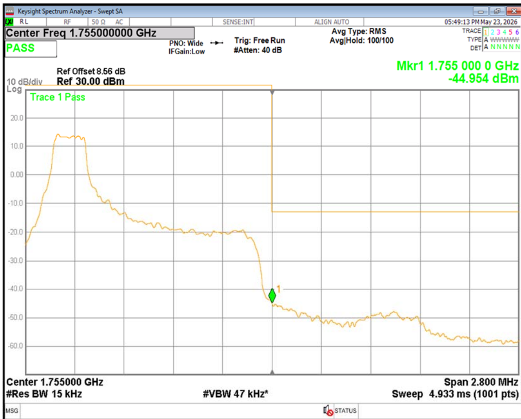
Band4 16QAM BW=1.4MHz Channel=20393 RB Size=1 Position=#Max
