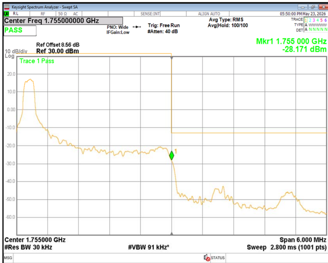
Band4 16QAM BW=3MHz Channel=20385 RB Size=1 Position=#Max
