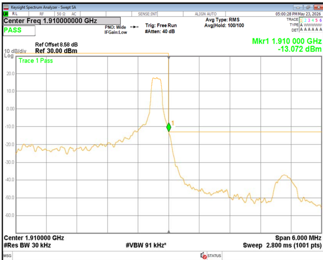
Band2 QPSK BW=3MHz Channel=19185 RB Size=15 Position=#0
