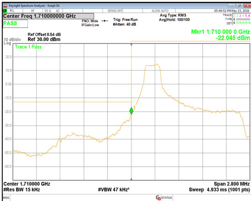
Band4 16QAM BW=1.4MHz Channel=19957 RB Size=1 Position=#Max
