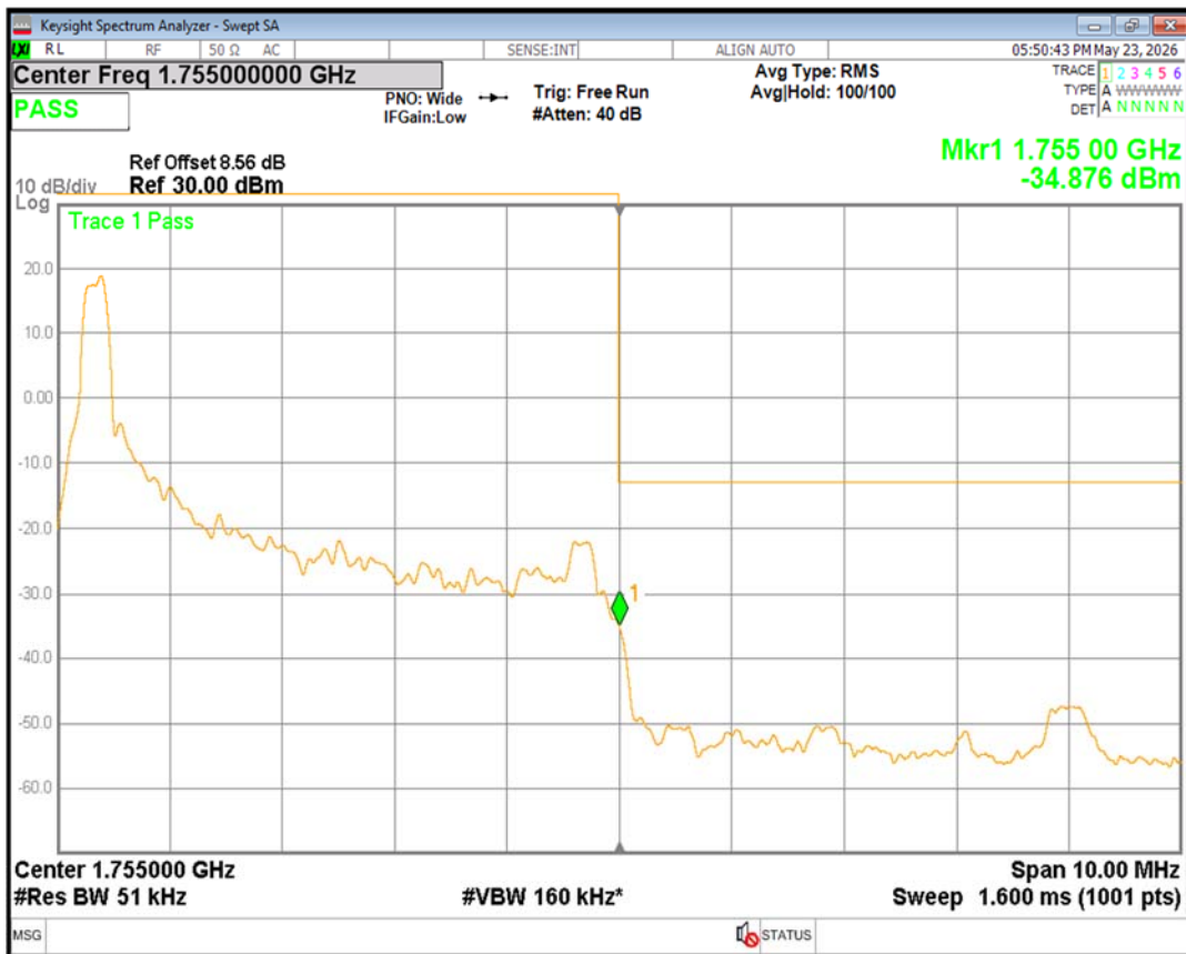
Band4 16QAM BW=5MHz Channel=20375 RB Size=25 Position=#0
