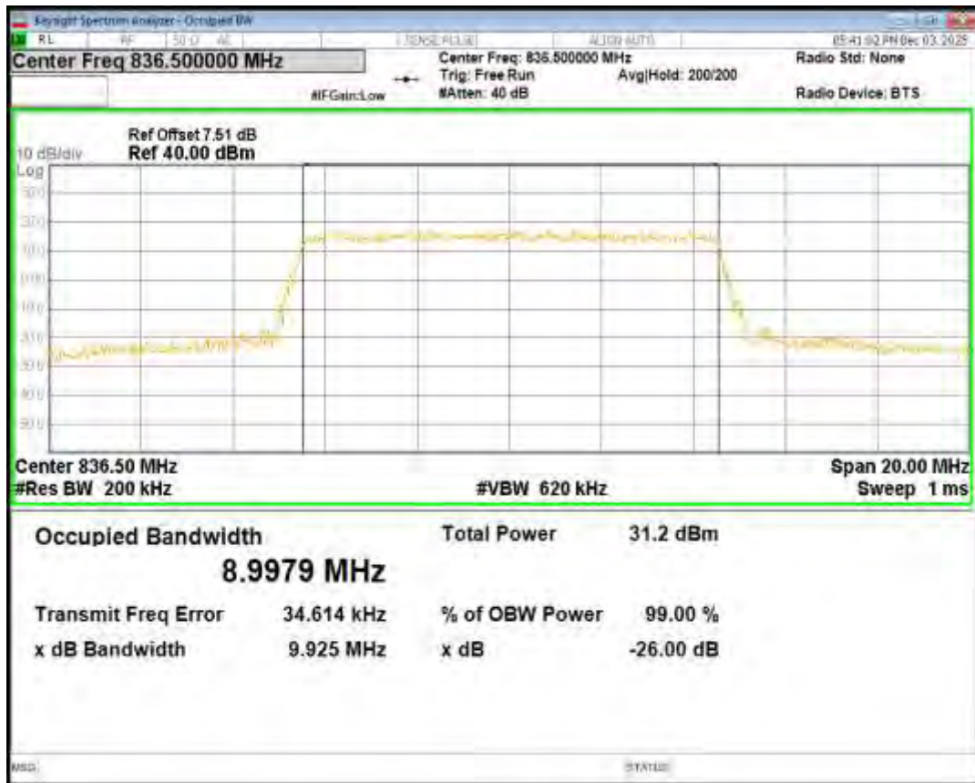
Band5 16QAM BW=10MHz Channel=20600 RB Size=50 Position=#0
