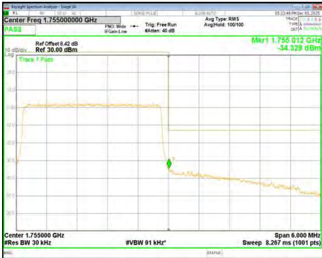
Band4 16QAM BW=5MHz Channel=19975 RB Size=25 Position=#0
