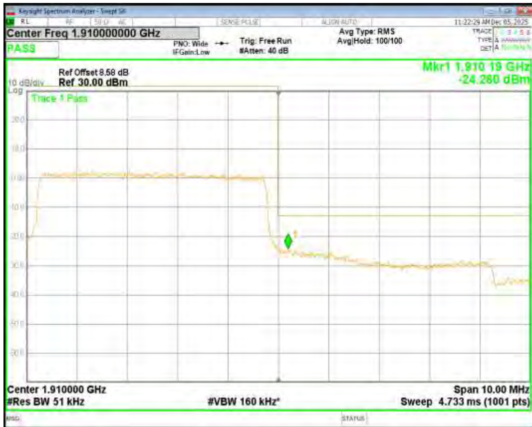
Band4 16QAM BW=1.4MHz Channel=19957 RB Size=6 Position=#0
