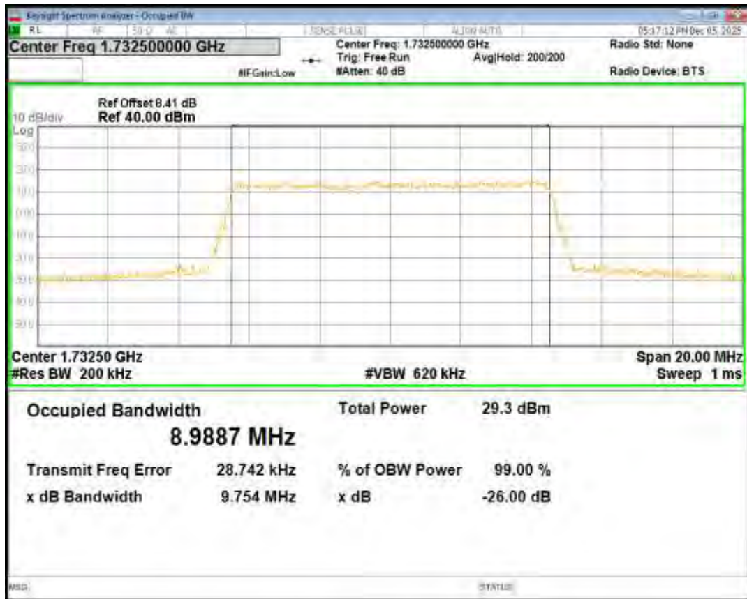
Band4 QPSK BW=10MHz Channel=20350 RB Size=50 Position=#0
