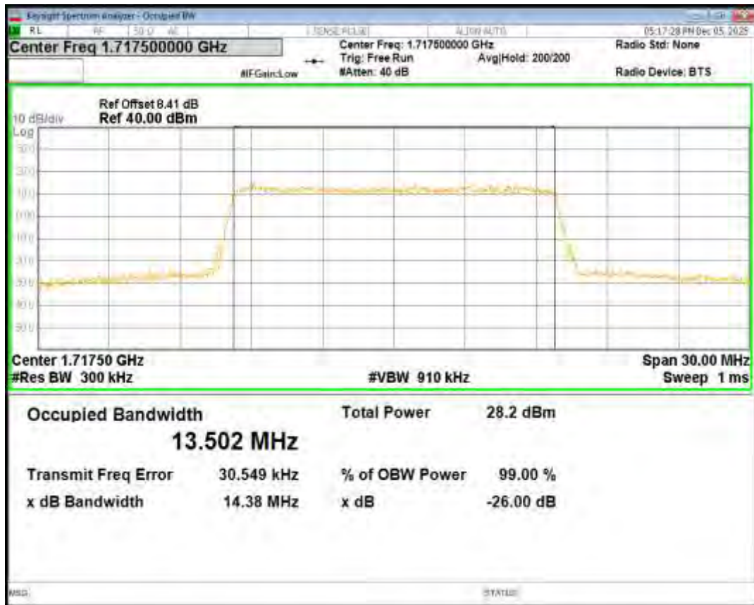
Band4 16QAM BW=15MHz Channel=20175 RB Size=75 Position=#0
