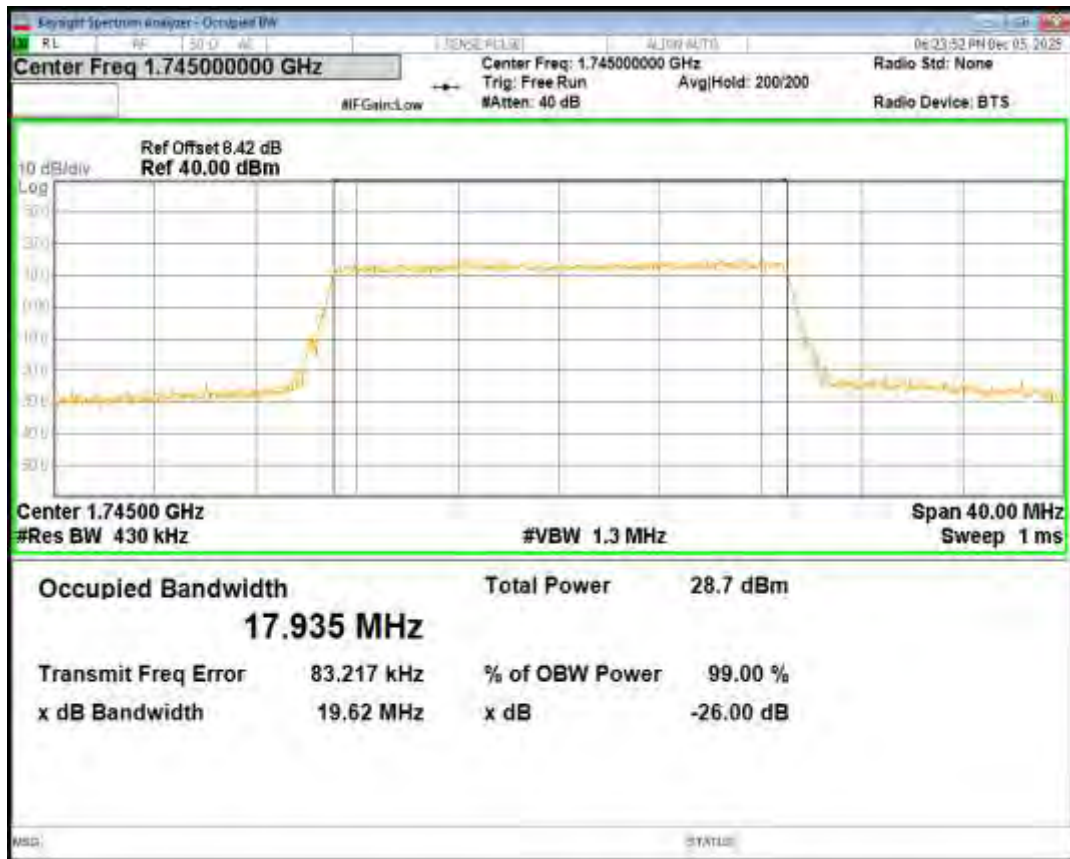
Band66 16QAM BW=20MHz Channel=132572 RB Size=100 Position=#0
