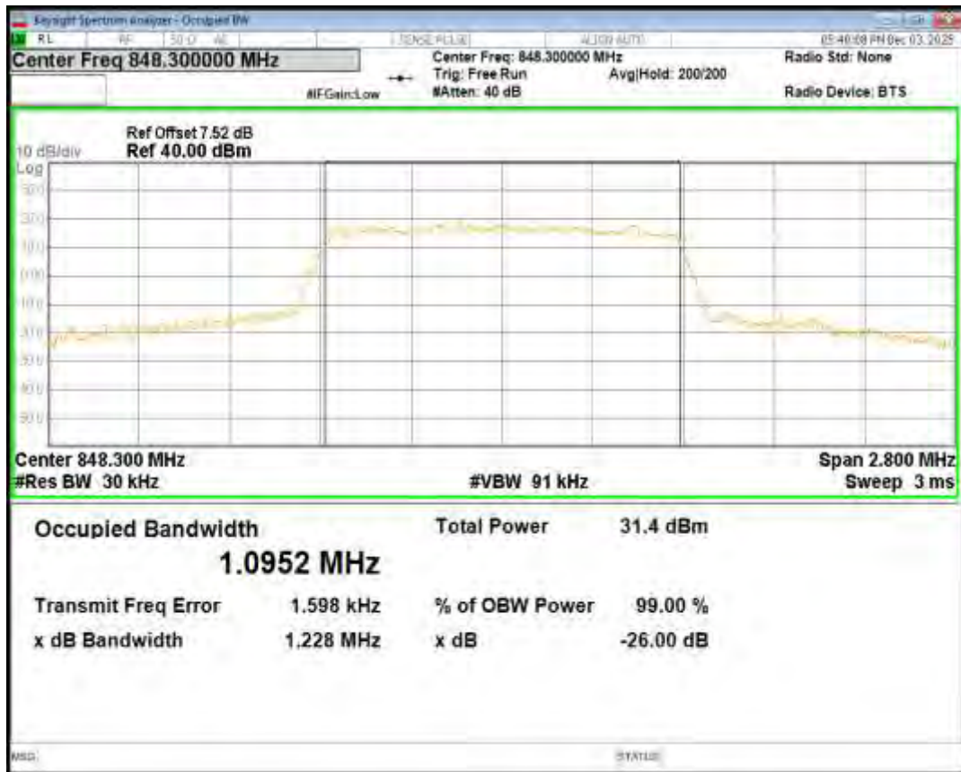
Band5 16QAM BW=10MHz Channel=20450 RB Size=50 Position=#0
