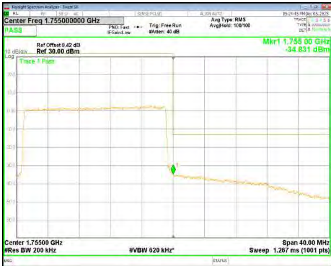
Band4 16QAM BW=3MHz Channel=19965 RB Size=15 Position=#0
