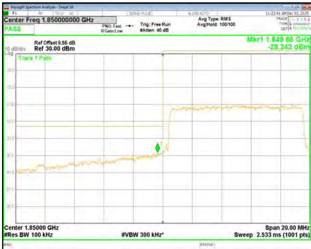
Band2 16QAM BW=10MHz Channel=19150 RB Size=50 Position=#0
