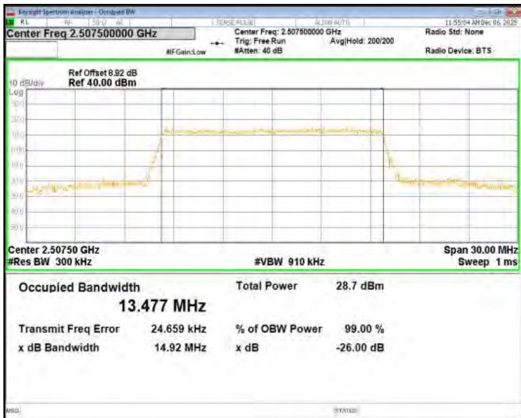
Band7 16QAM BW=15MHz Channel=21100 RB Size=75 Position=#0
