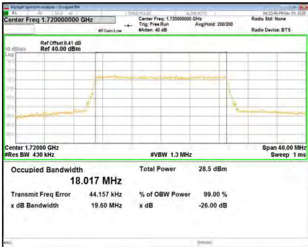
Band66 16QAM BW=20MHz Channel=132322 RB Size=100 Position=#0
