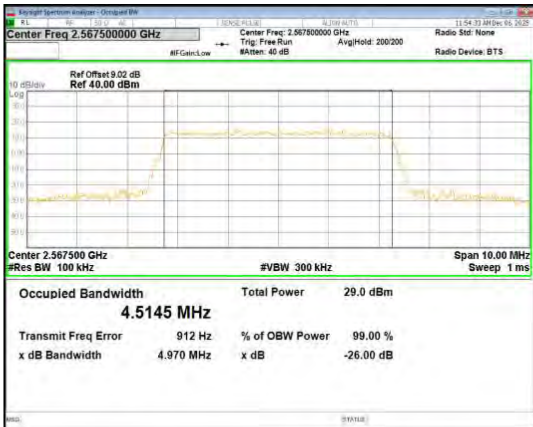
Band7 QPSK BW=10MHz Channel=20800 RB Size=50 Position=#0
