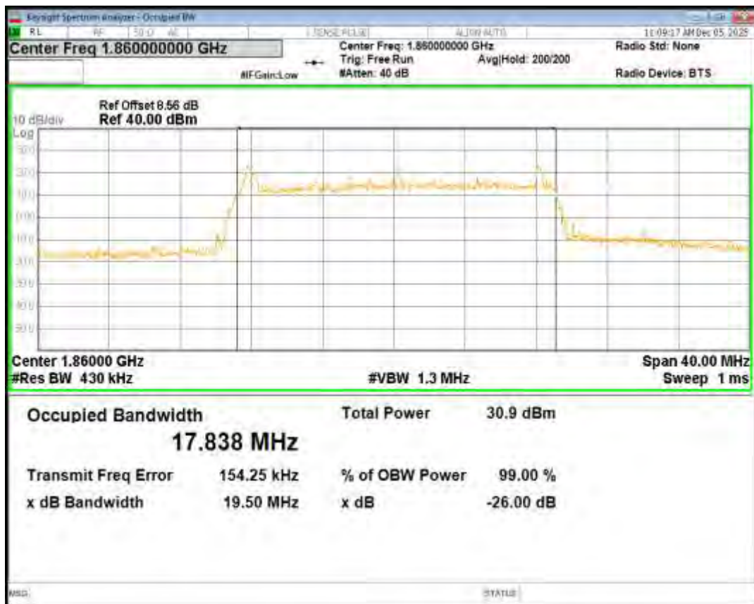
Band2 QPSK BW=20MHz Channel=18900 RB Size=100 Position=#0
