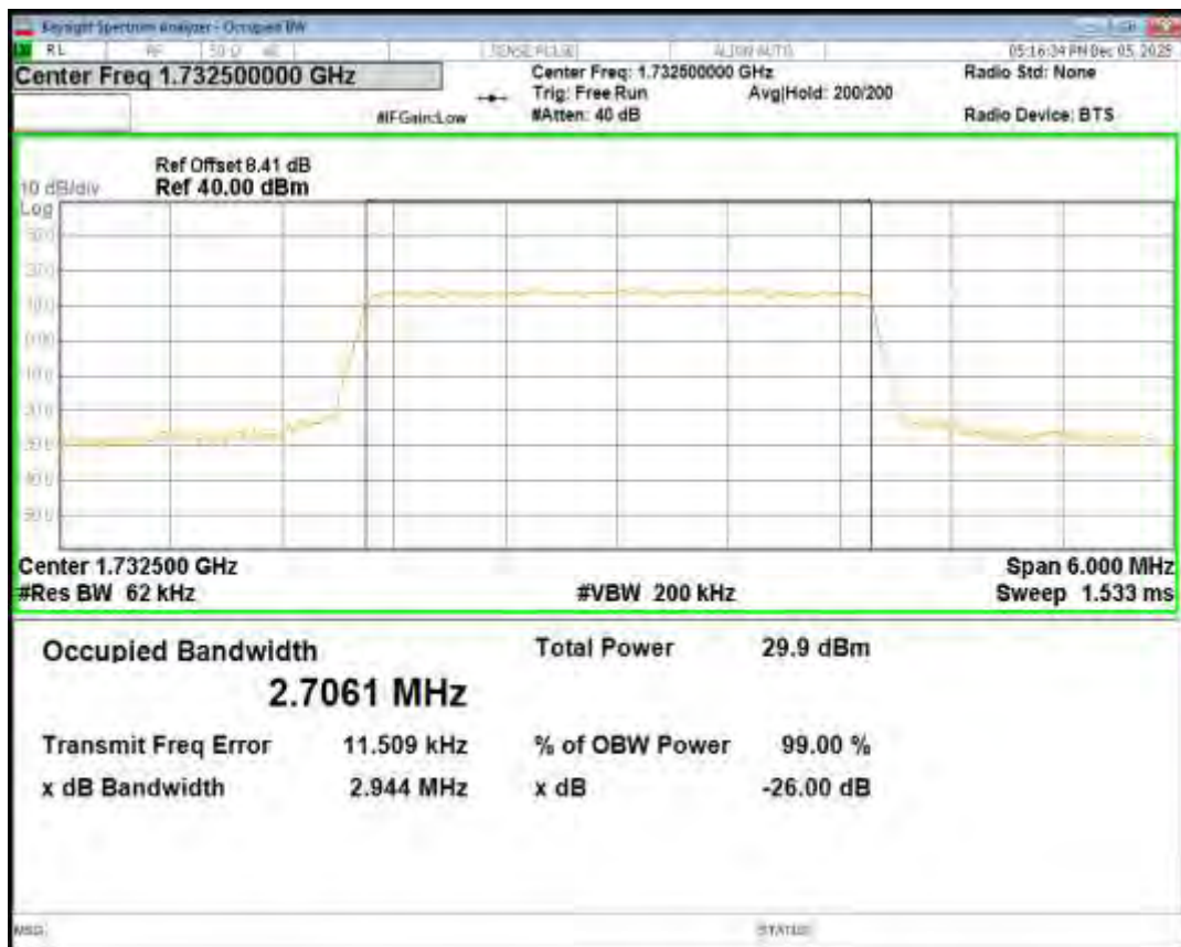
Band4 QPSK BW=3MHz Channel=20385 RB Size=15 Position=#0
