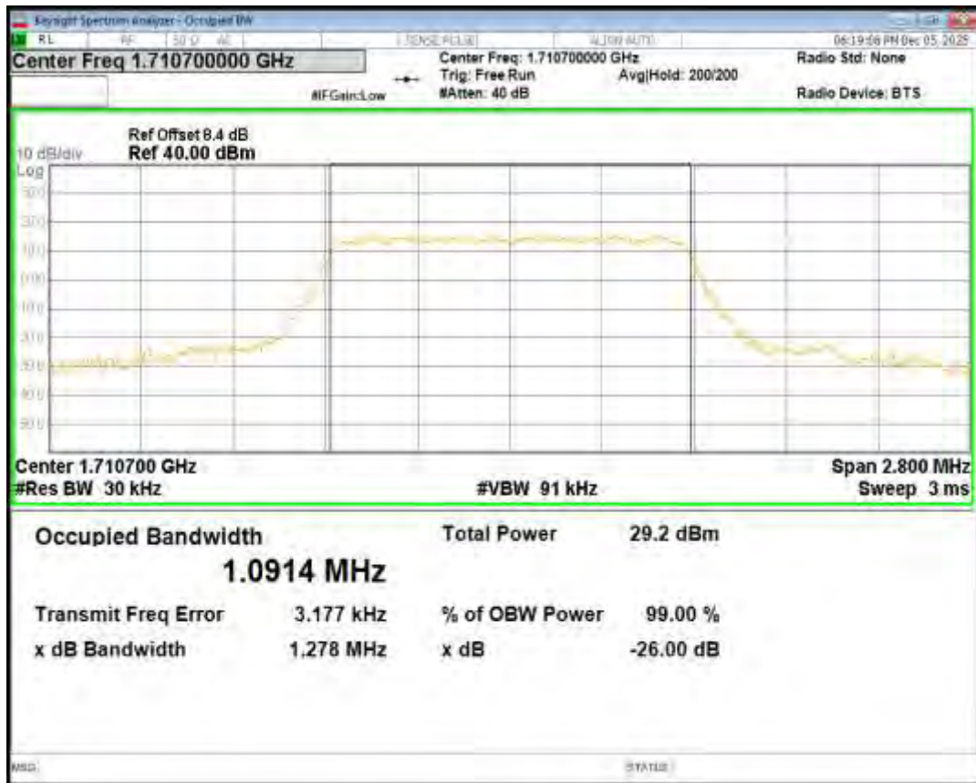
Band66 QPSK BW=1.4MHz Channel=132322 RB Size=6 Position=#0
