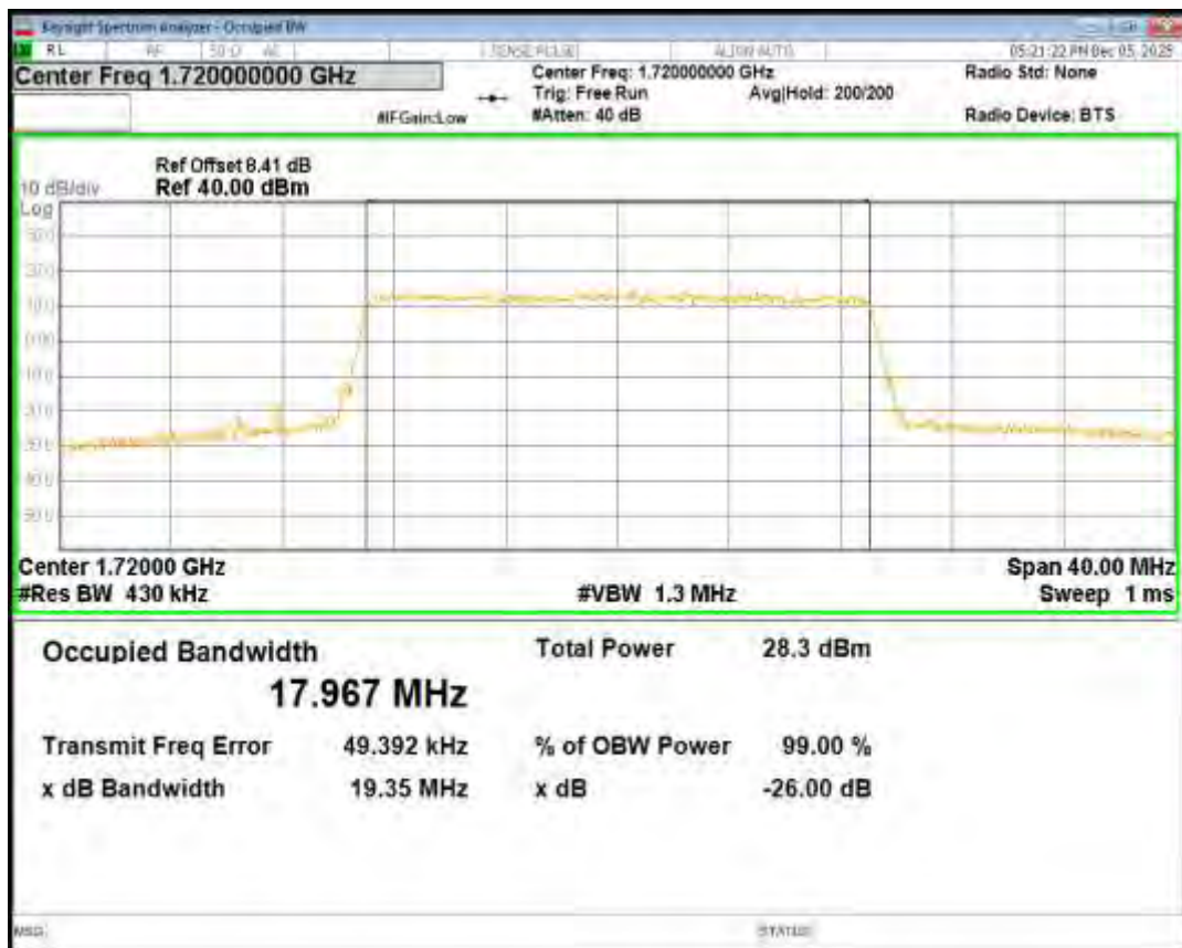
Band4 16QAM BW=20MHz Channel=20175 RB Size=100 Position=#0
