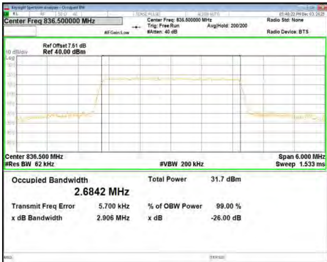
Band5 16QAM BW=3MHz Channel=20635 RB Size=15 Position=#0
