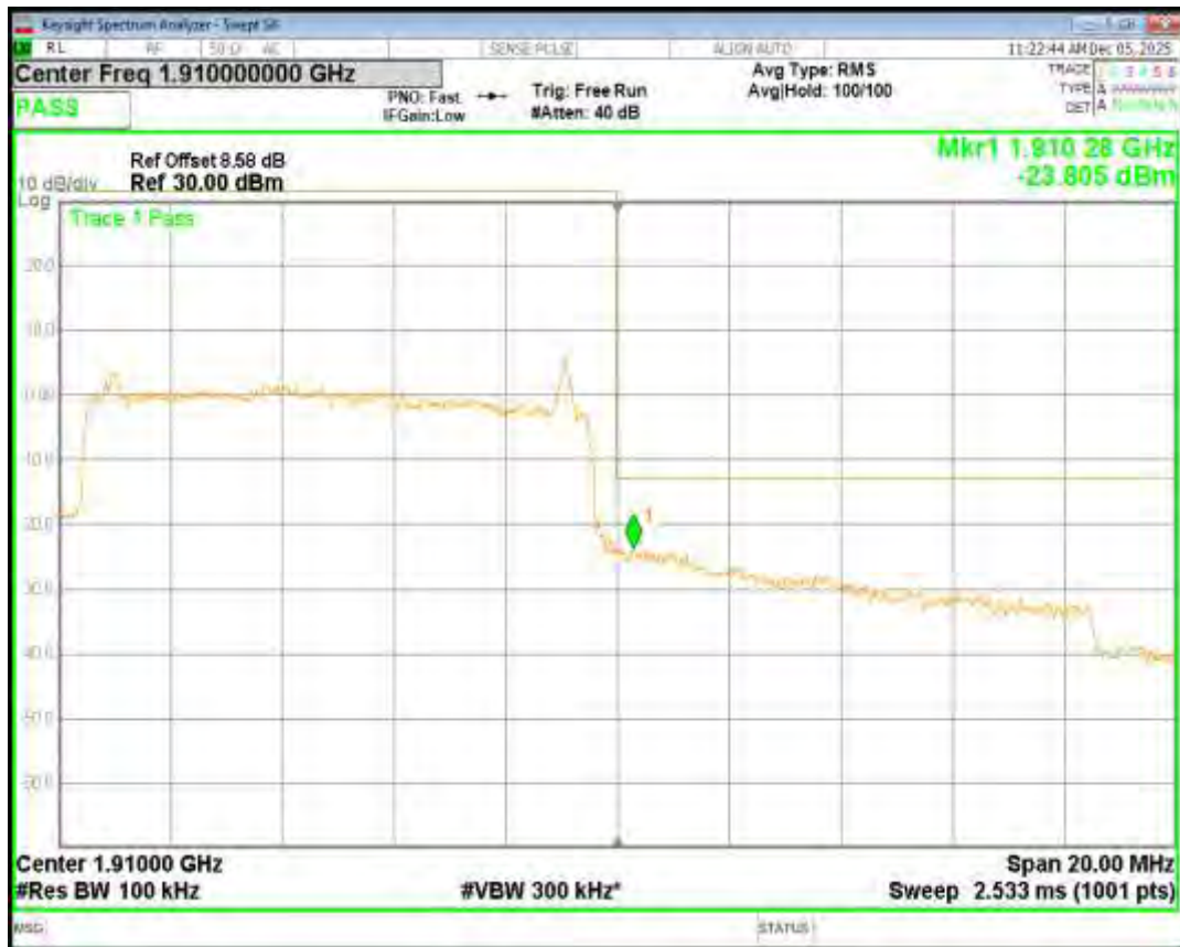
Band2 QPSK BW=15MHz Channel=18675 RB Size=75 Position=#0
