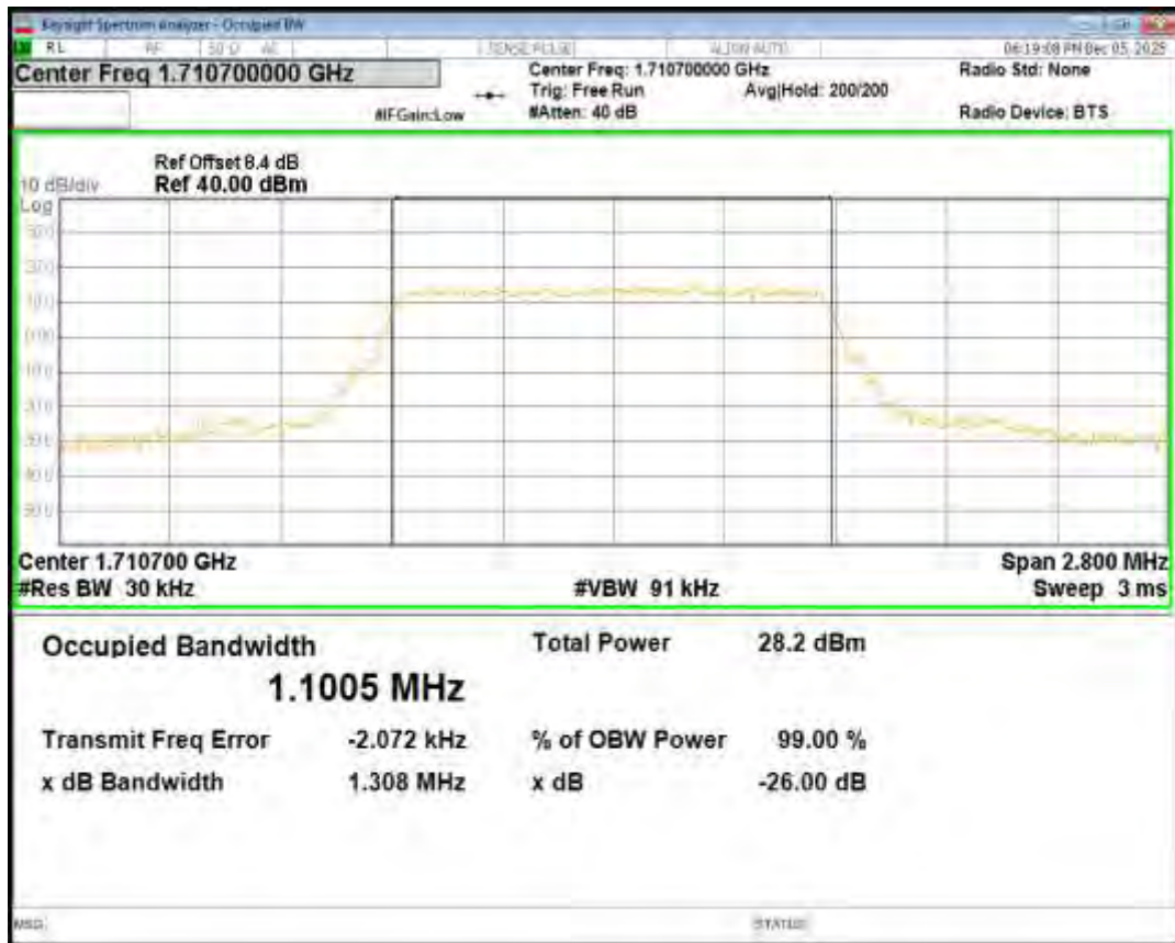
Band66 16QAM BW=1.4MHz Channel=132322 RB Size=6 Position=#0
