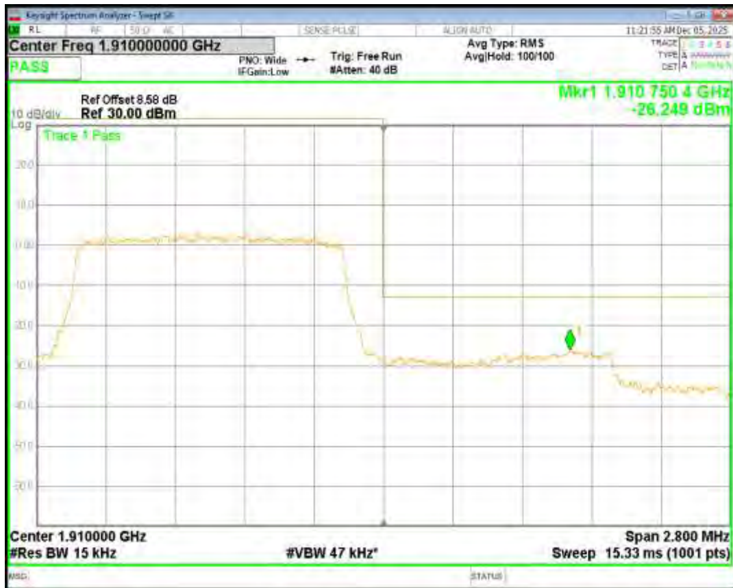
Band2 QPSK BW=10MHz Channel=18650 RB Size=50 Position=#0
