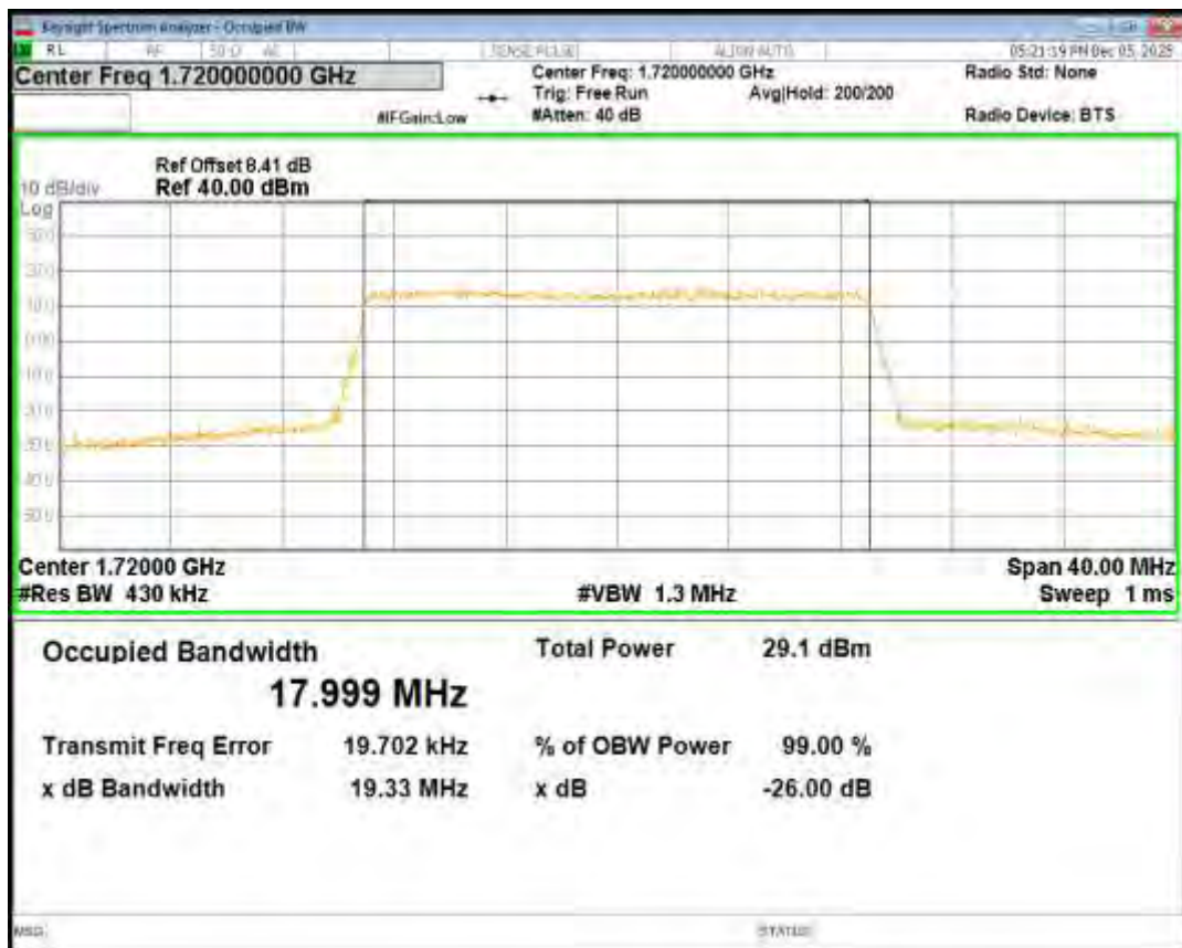
Band4 QPSK BW=20MHz Channel=20175 RB Size=100 Position=#0
