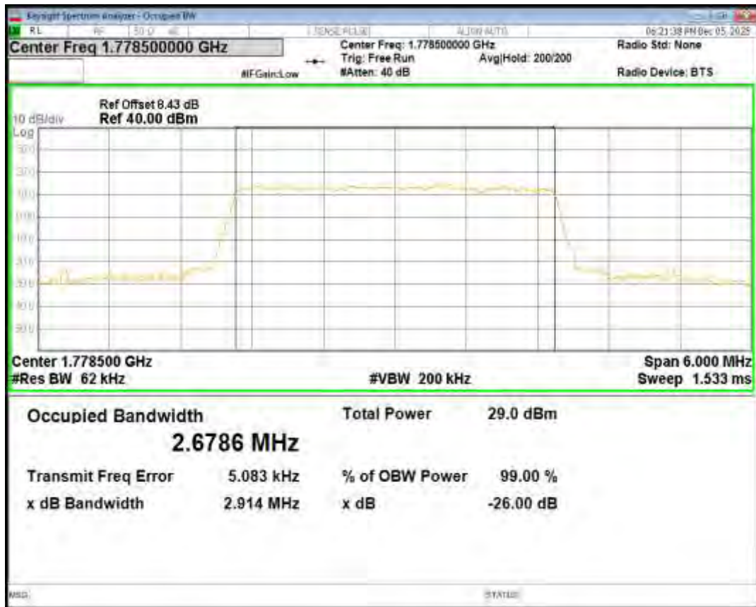
Band66 16QAM BW=5MHz Channel=131997 RB Size=25 Position=#0
