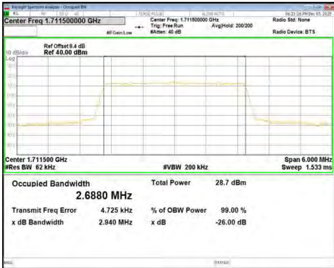
Band66 16QAM BW=3MHz Channel=132322 RB Size=15 Position=#0
