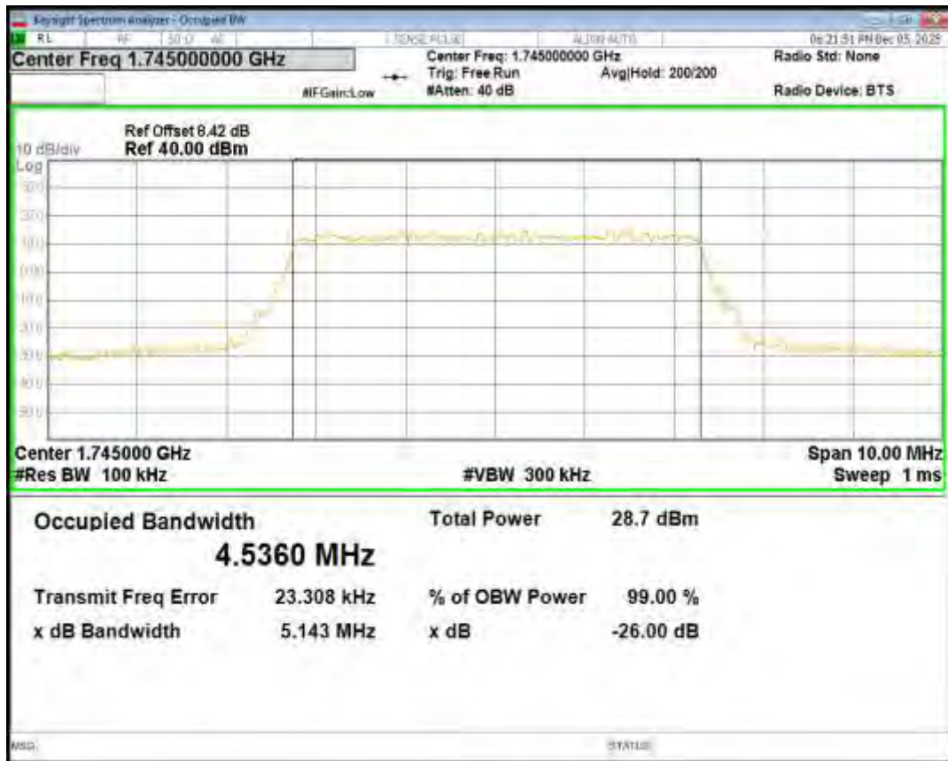
Band66 16QAM BW=5MHz Channel=132647 RB Size=25 Position=#0
