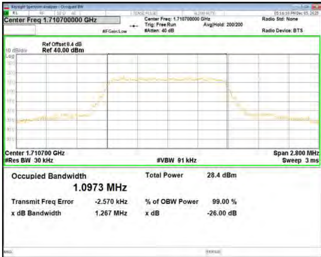
Band4 16QAM BW=1.4MHz Channel=20175 RB Size=6 Position=#0
