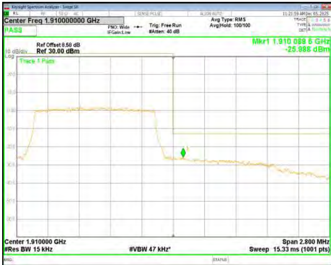
Band2 16QAM BW=10MHz Channel=18650 RB Size=50 Position=#0
