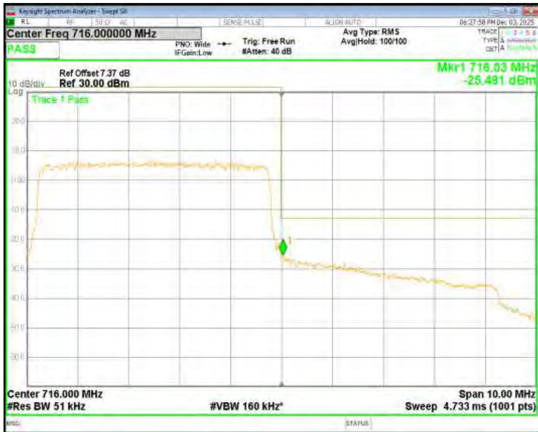
Band2 16QAM BW=1.4MHz Channel=18607 RB Size=6 Position=#0
