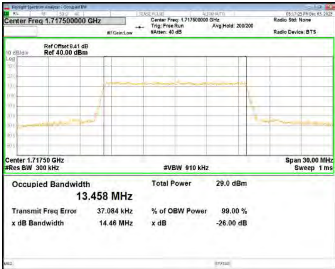
Band4 QPSK BW=15MHz Channel=20175 RB Size=75 Position=#0
