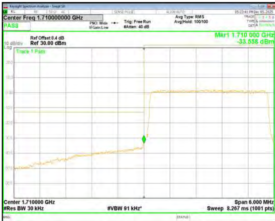
Band4 16QAM BW=3MHz Channel=20385 RB Size=15 Position=#0
