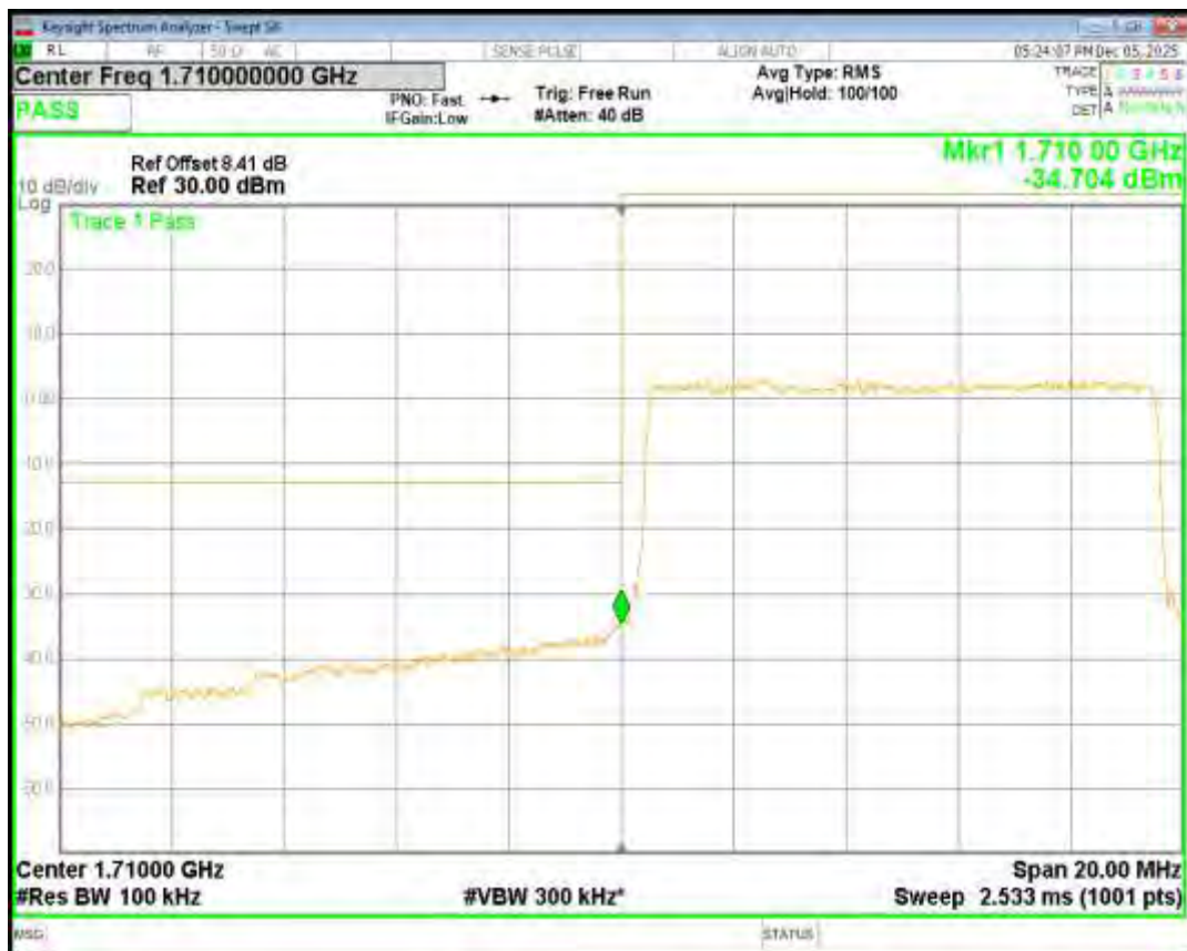
Band4 QPSK BW=10MHz Channel=20350 RB Size=50 Position=#0
