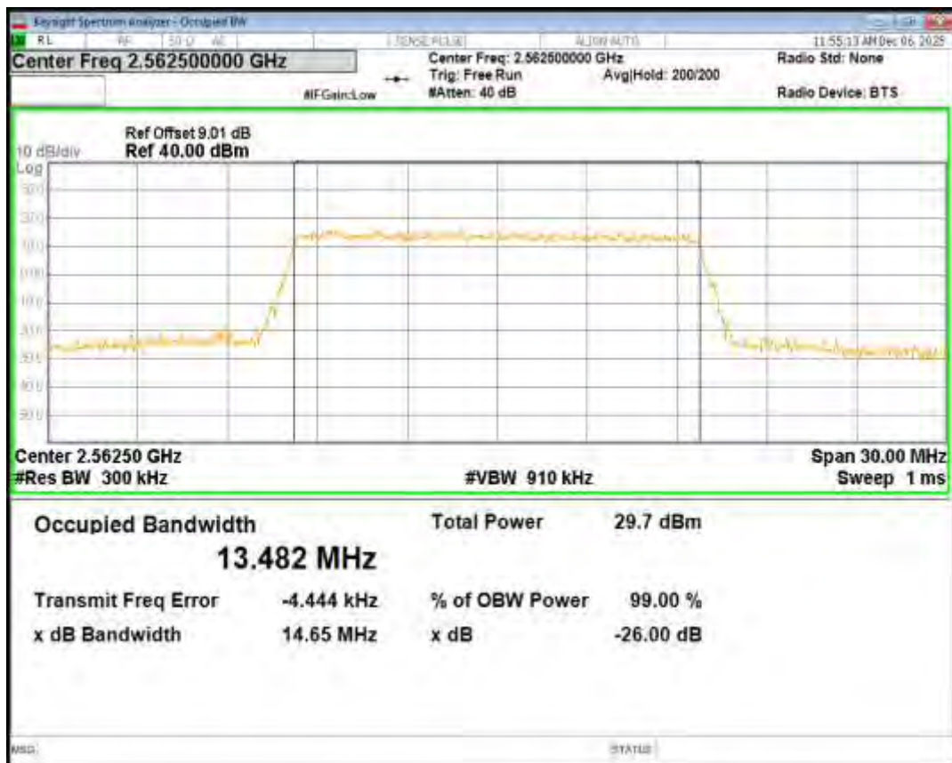
Band7 QPSK BW=20MHz Channel=20850 RB Size=100 Position=#0
