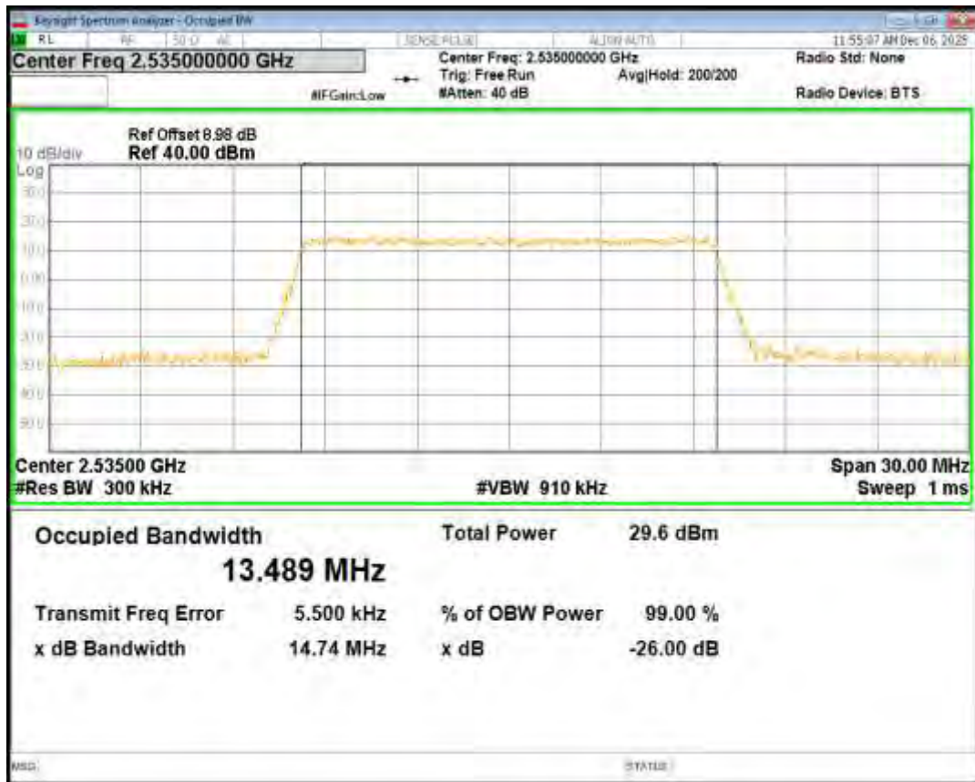
Band7 QPSK BW=15MHz Channel=21375 RB Size=75 Position=#0
