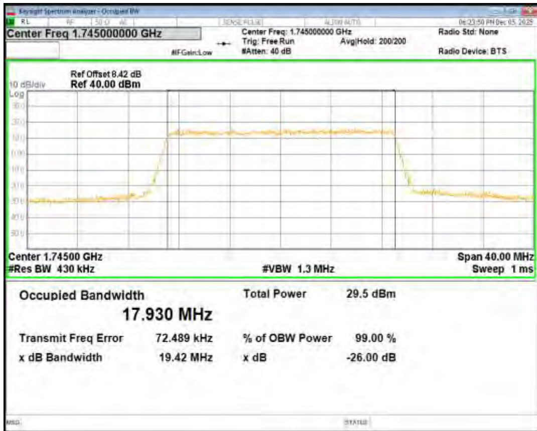
Band66 QPSK BW=20MHz Channel=132572 RB Size=100 Position=#0
