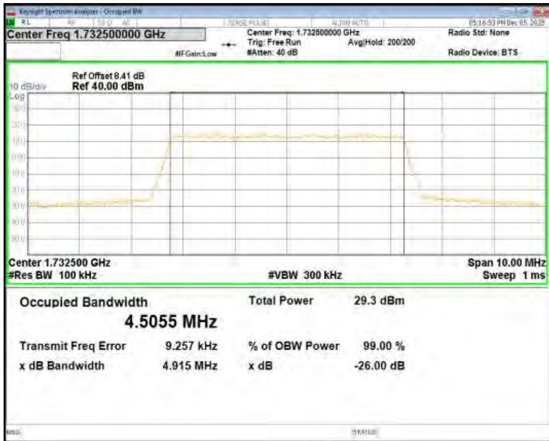
Band4 QPSK BW=5MHz Channel=20375 RB Size=25 Position=#0
