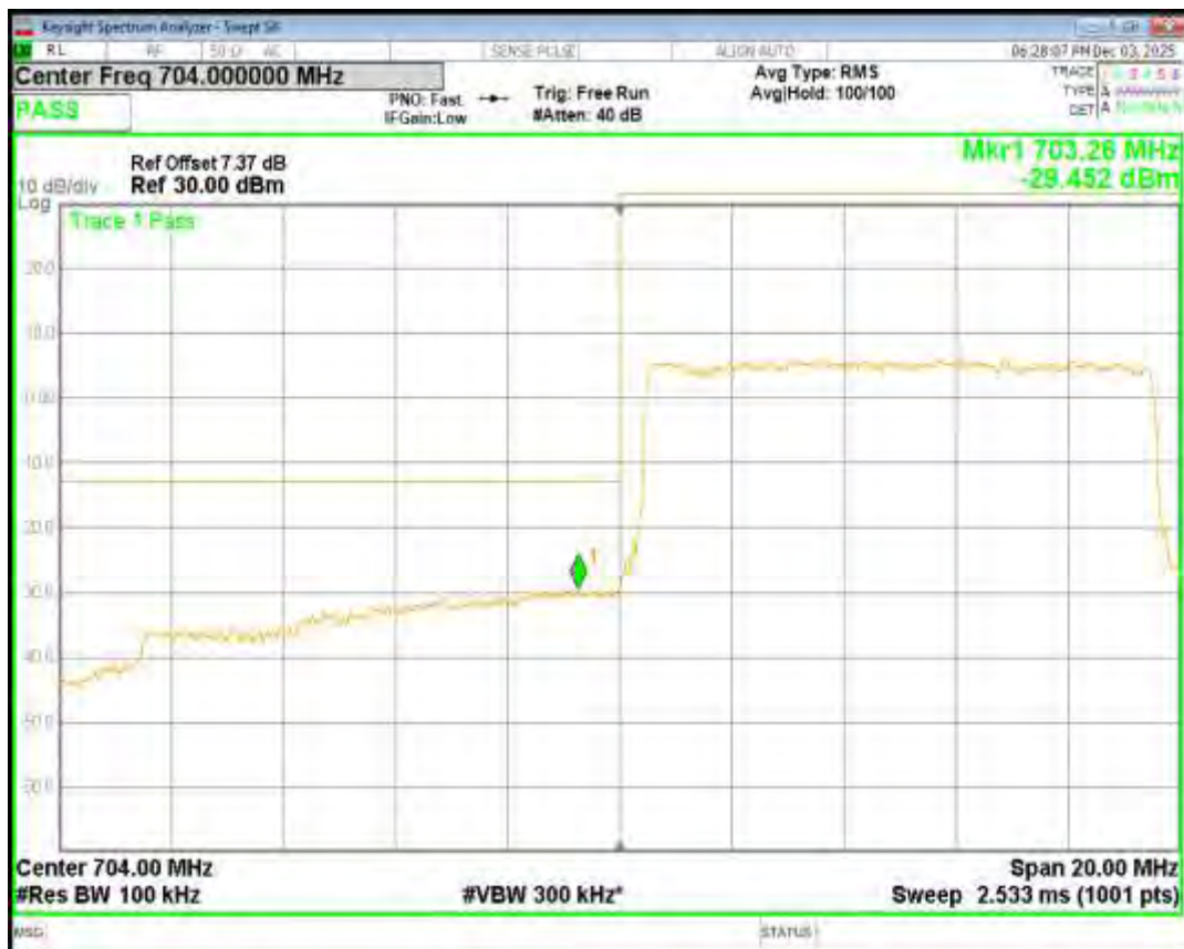
Band17 QPSK BW=10MHz Channel=23800 RB Size=50 Position=#0
