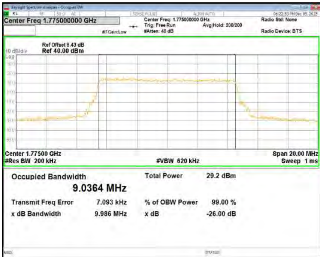
Band66 QPSK BW=15MHz Channel=132047 RB Size=75 Position=#0
