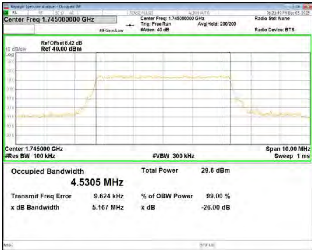
Band66 QPSK BW=5MHz Channel=132647 RB Size=25 Position=#0
