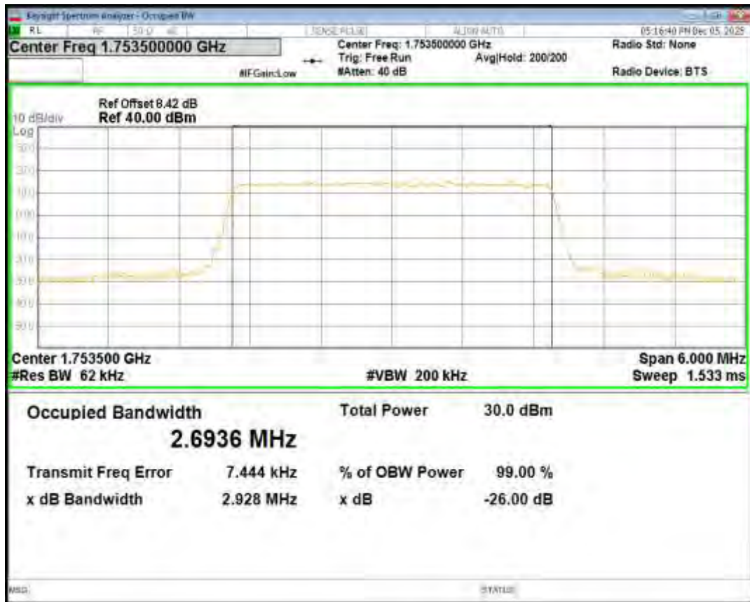
Band4 QPSK BW=5MHz Channel=19975 RB Size=25 Position=#0
