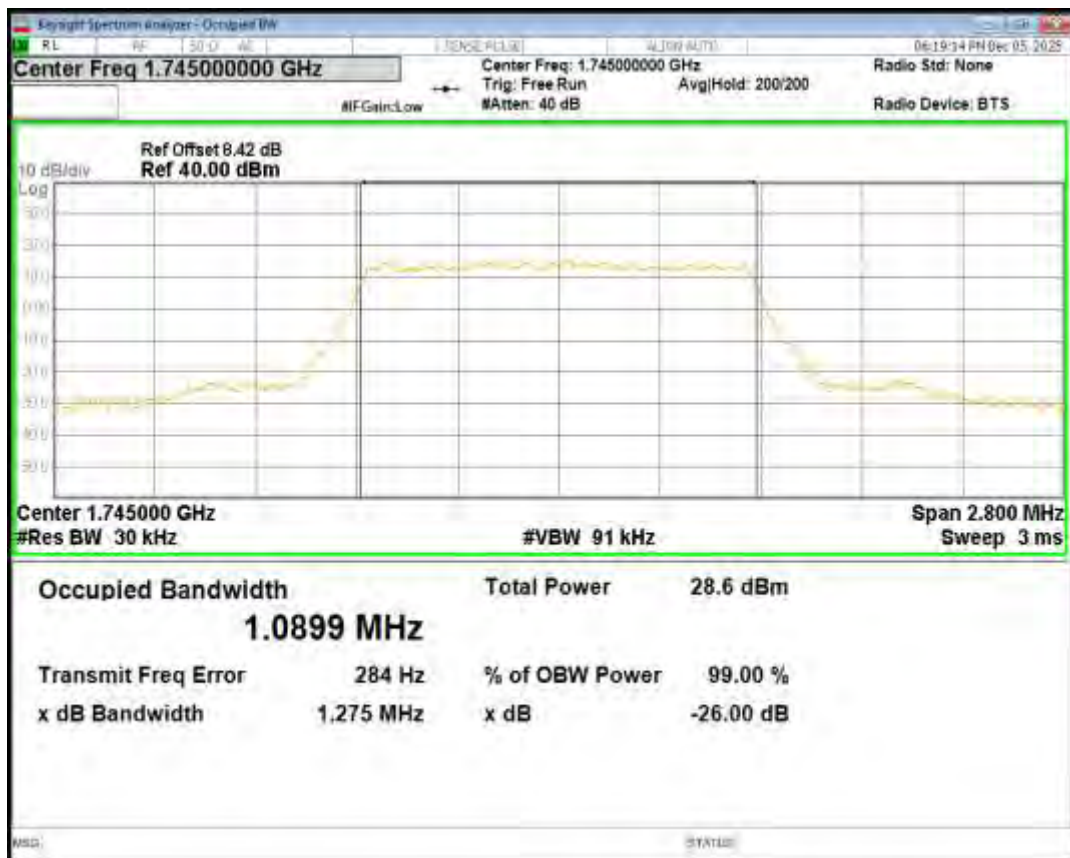
Band66 16QAM BW=1.4MHz Channel=132665 RB Size=6 Position=#0
