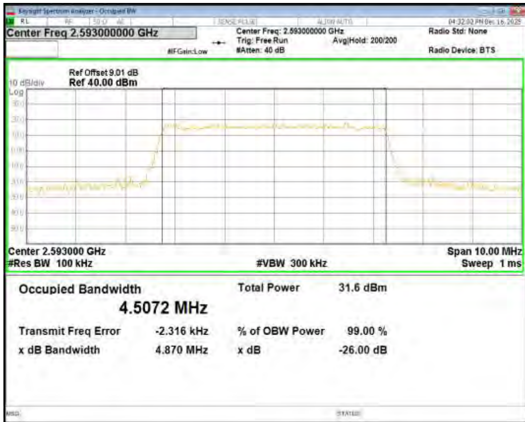
Band41 QPSK BW=5MHz Channel=41565 RB Size=25 Position=#0
