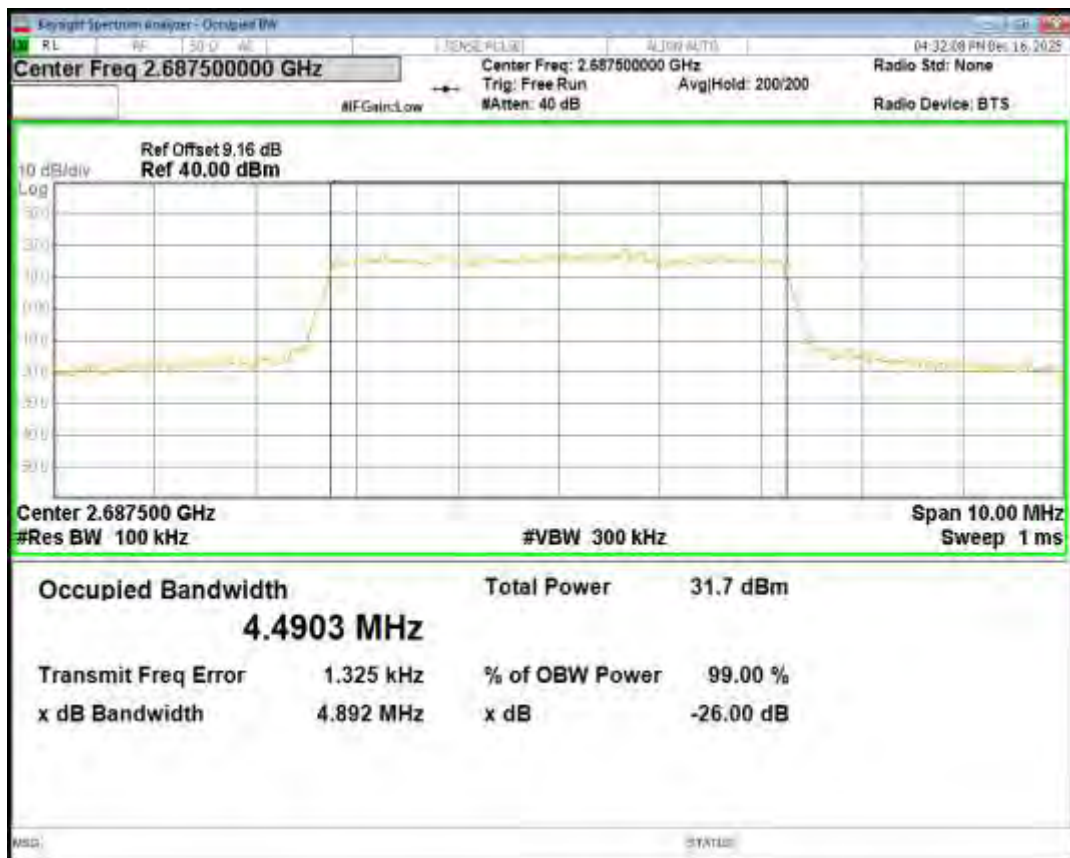
Band5 16QAM BW=1.4MHz Channel=20407 RB Size=6 Position=#0
