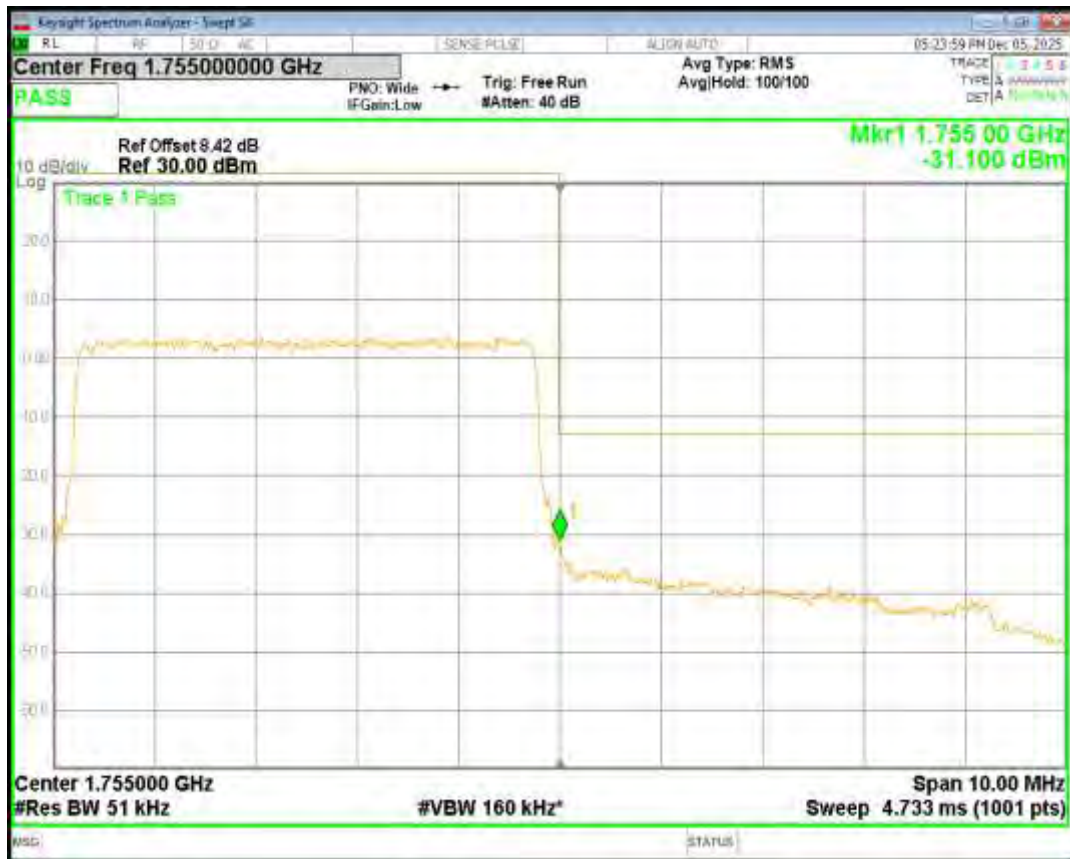
Band41 16QAM BW=10MHz Channel=39700 RB Size=50 Position=#0
