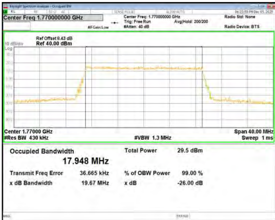
Band66 QPSK BW=3MHz Channel=131987 RB Size=15 Position=#0
