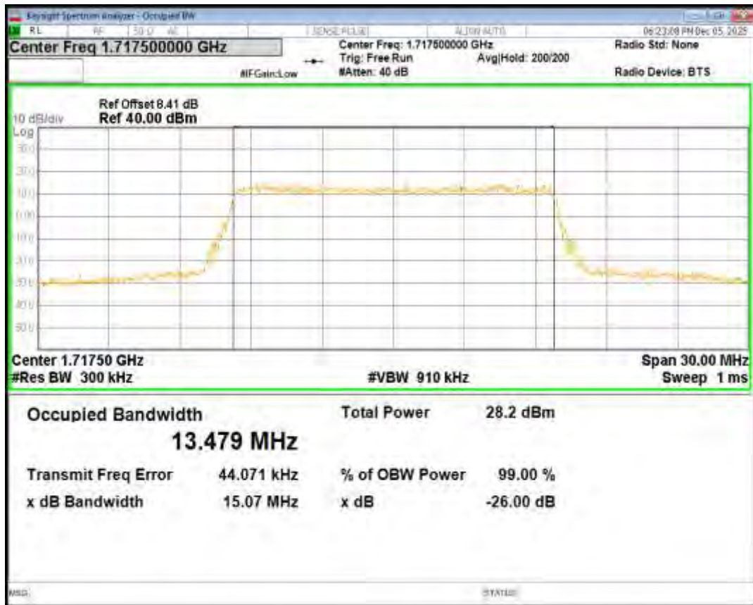
Band66 16QAM BW=15MHz Channel=132322 RB Size=75 Position=#0
