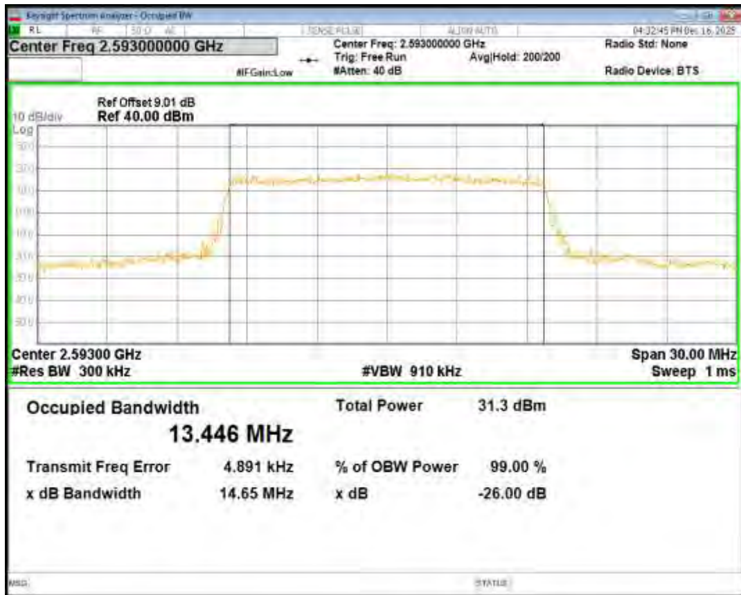
Band41 QPSK BW=15MHz Channel=41515 RB Size=75 Position=#0
