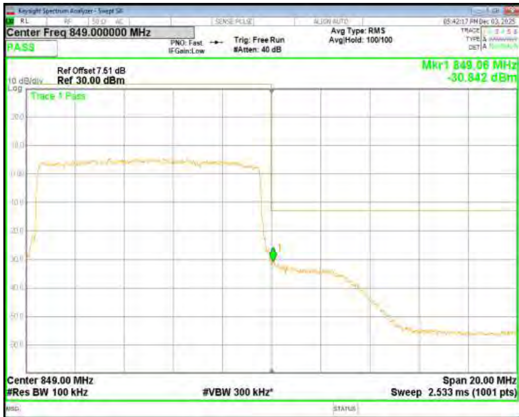
Band5 16QAM BW=3MHz Channel=20415 RB Size=15 Position=#0
