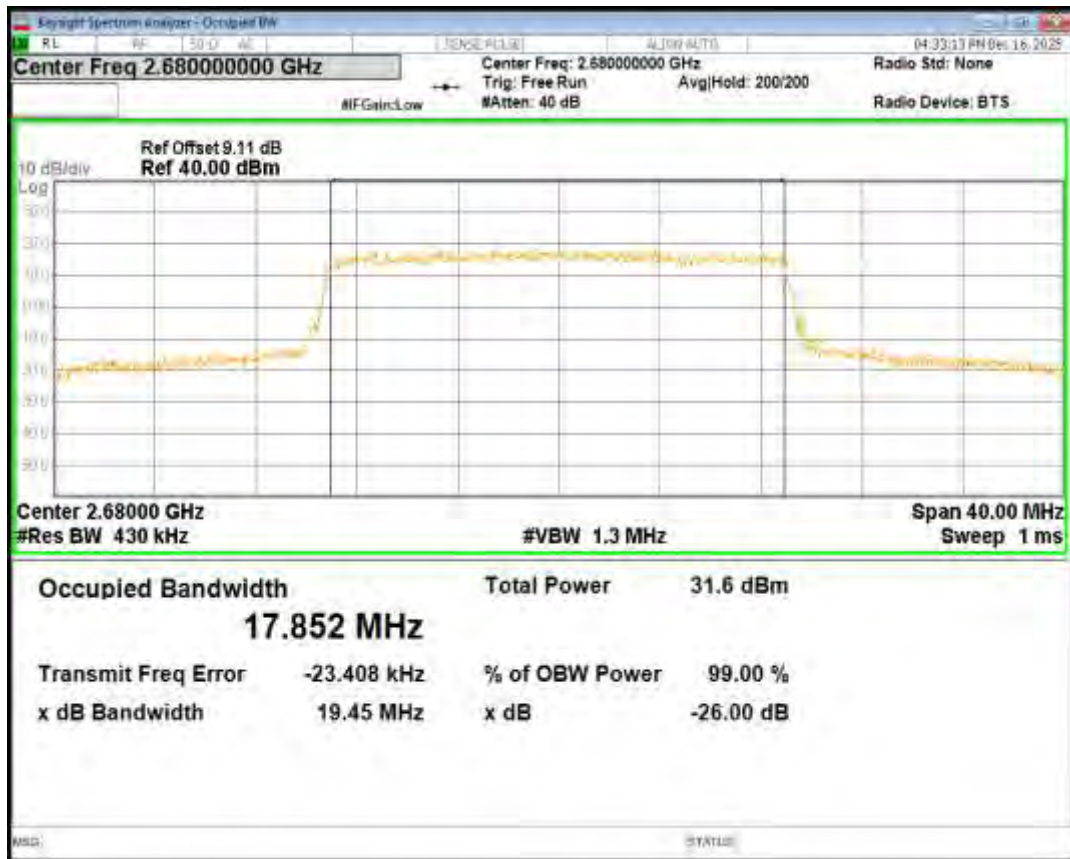
Band41 QPSK BW=5MHz Channel=39675 RB Size=25 Position=#0
