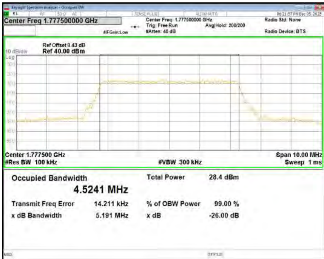
Band66 QPSK BW=1.4MHz Channel=131979 RB Size=6 Position=#0
