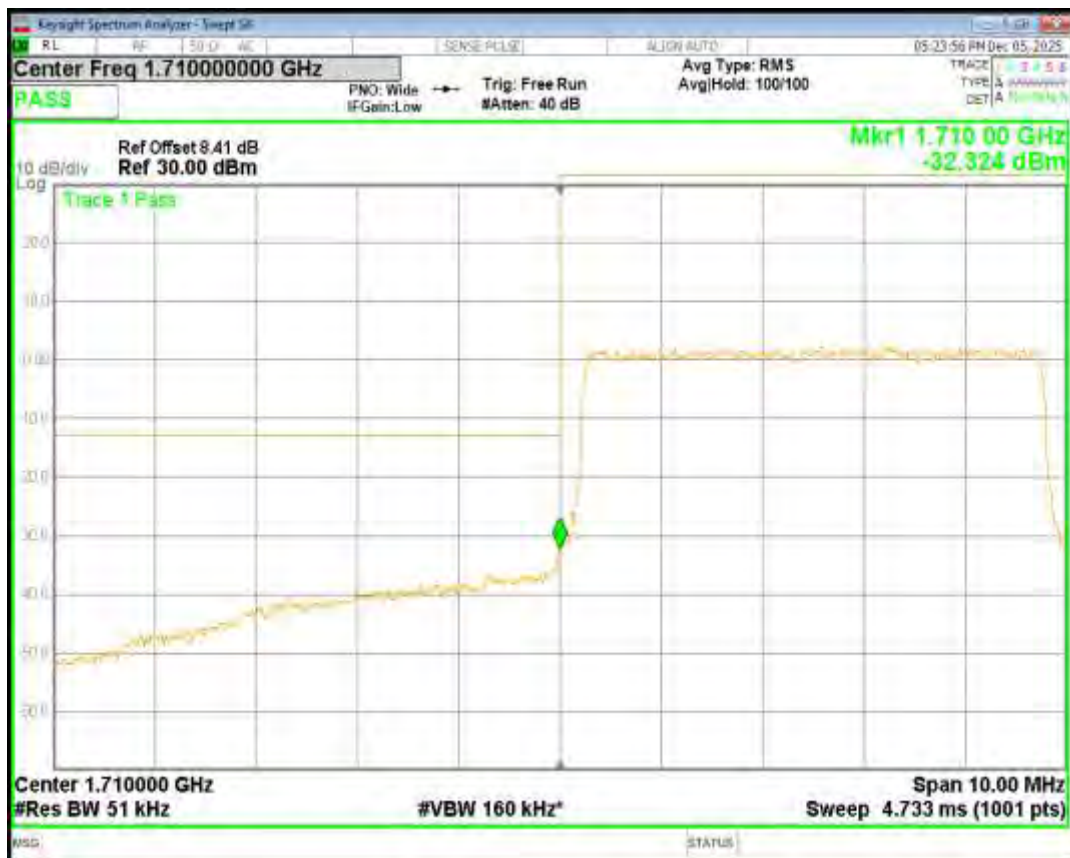
Band4 16QAM BW=5MHz Channel=20375 RB Size=25 Position=#0
