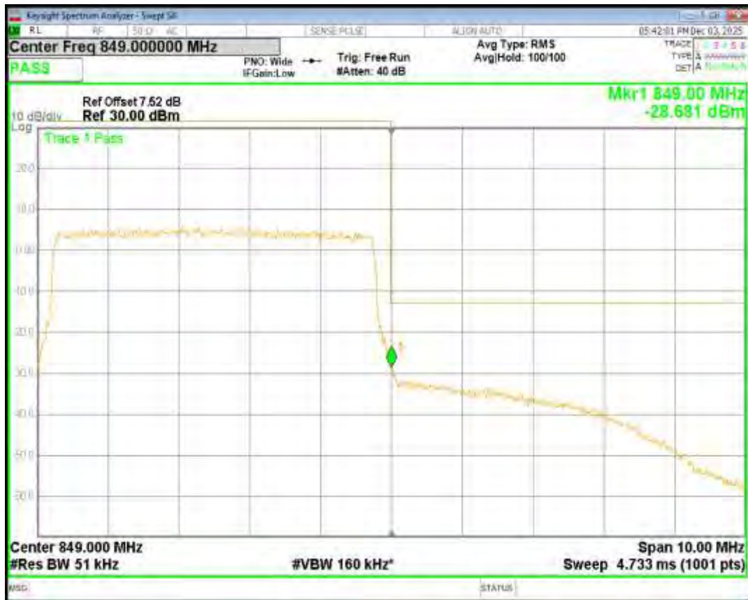
Band5 QPSK BW=1.4MHz Channel=20407 RB Size=6 Position=#0
