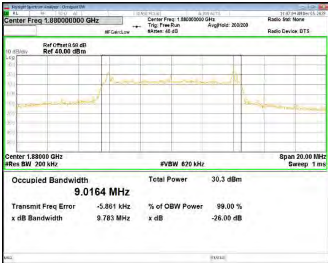
Band2 QPSK BW=10MHz Channel=19150 RB Size=50 Position=#0
