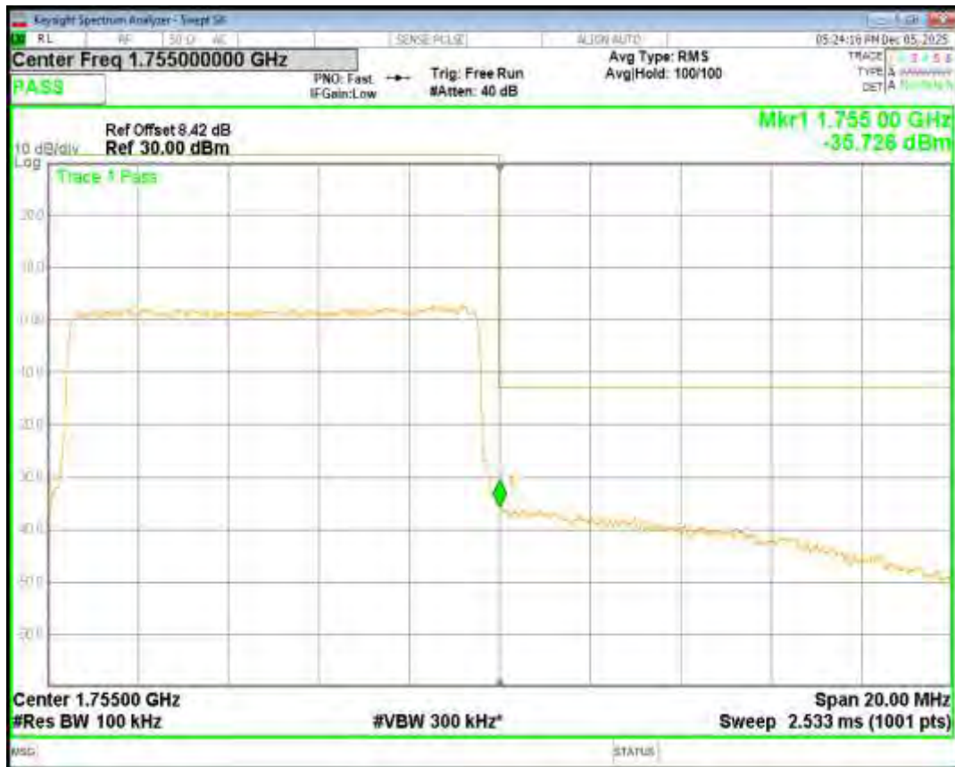
Band4 16QAM BW=15MHz Channel=20025 RB Size=75 Position=#0
