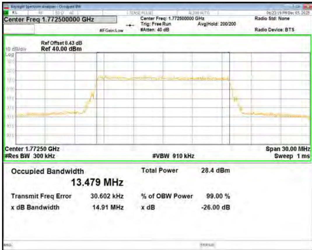
Band66 16QAM BW=20MHz Channel=132072 RB Size=100 Position=#0
