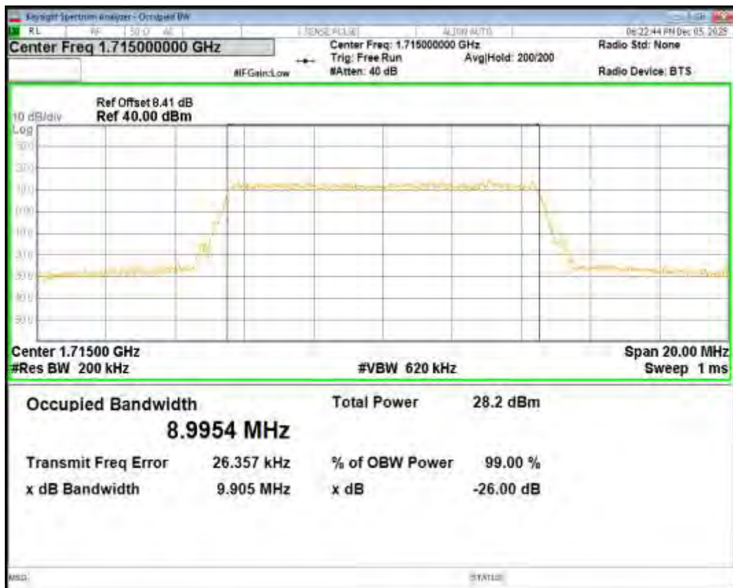
Band66 16QAM BW=10MHz Channel=132322 RB Size=50 Position=#0
