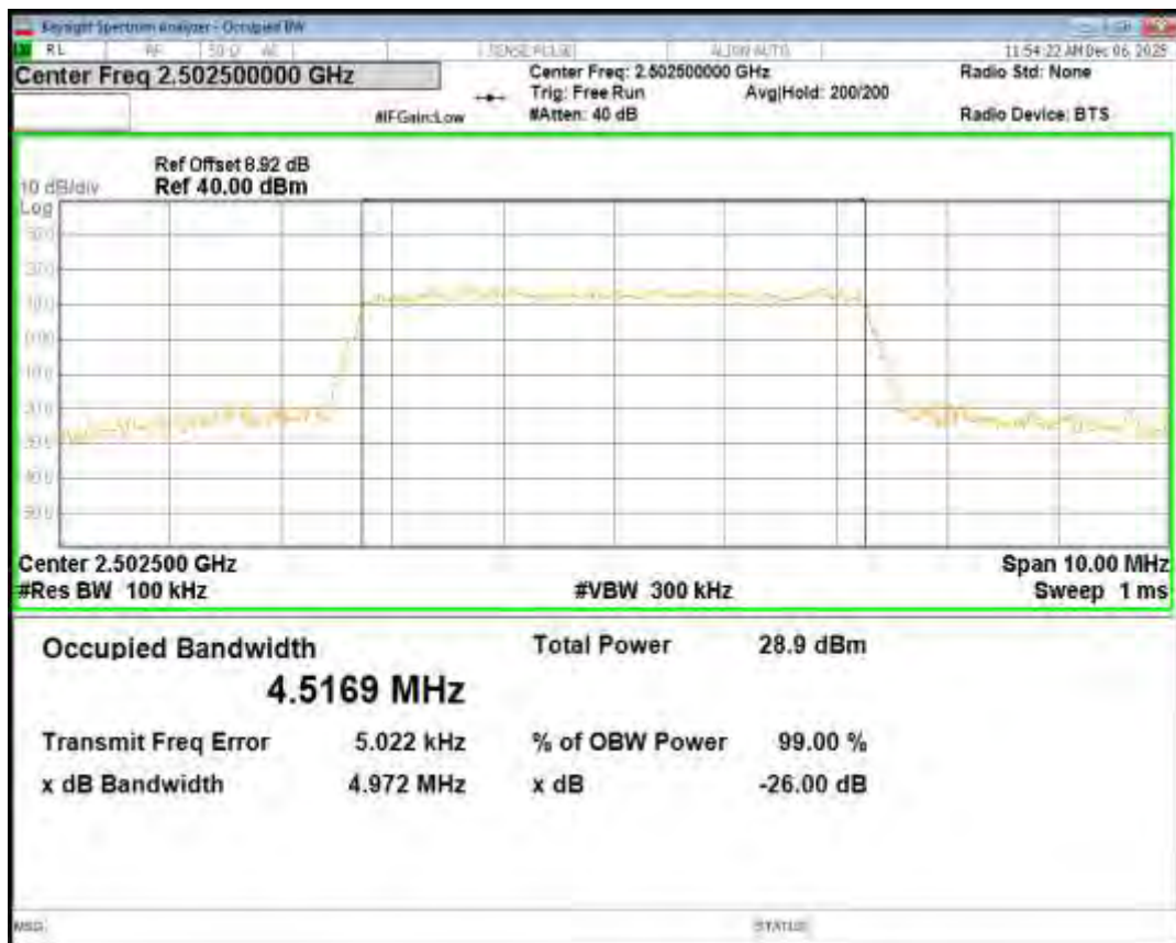
Band7 16QAM BW=5MHz Channel=21100 RB Size=25 Position=#0
