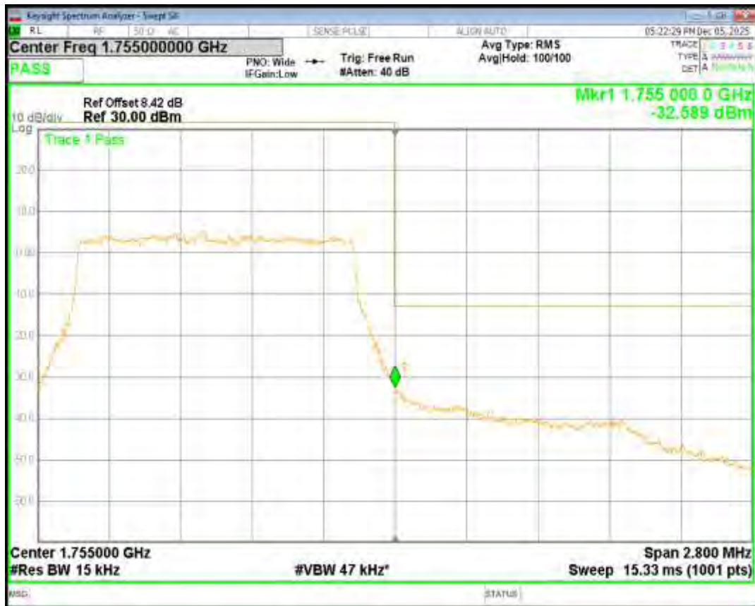
Band4 QPSK BW=10MHz Channel=20000 RB Size=50 Position=#0
