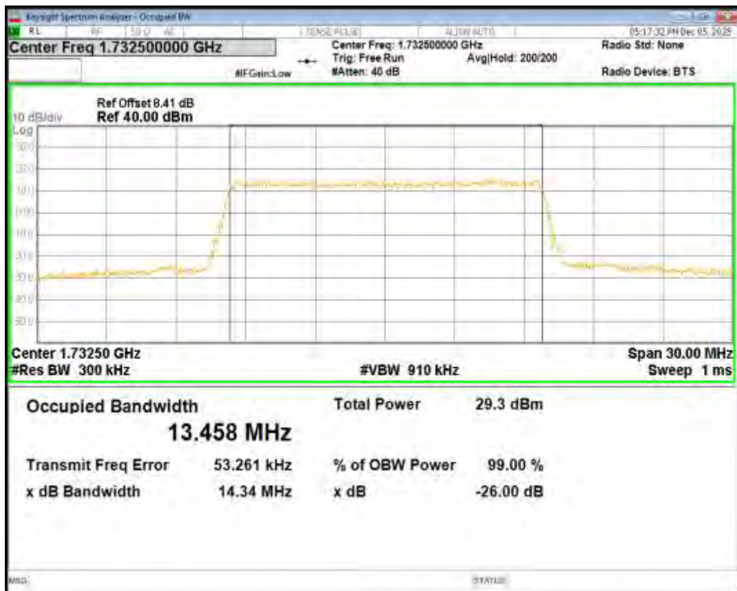
Band4 QPSK BW=15MHz Channel=20325 RB Size=75 Position=#0
