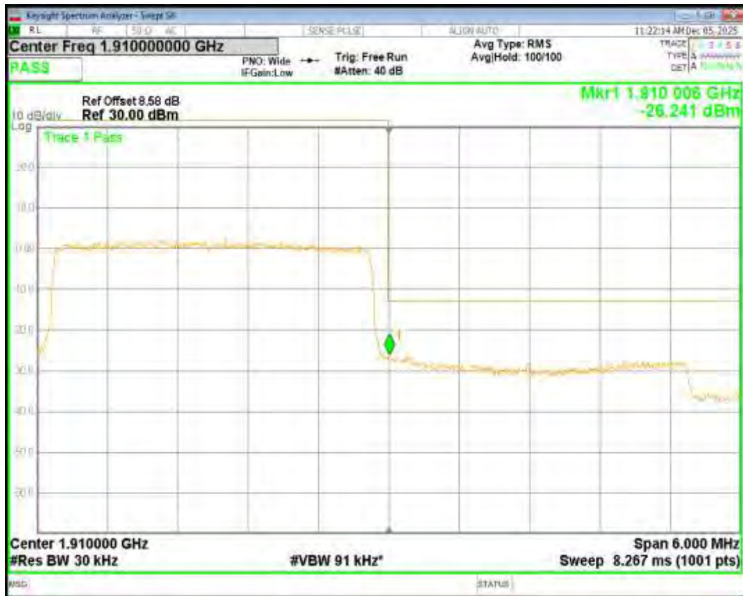
Band2 QPSK BW=5MHz Channel=18625 RB Size=25 Position=#0
