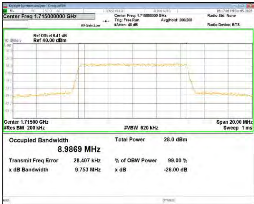
Band4 16QAM BW=10MHz Channel=20175 RB Size=50 Position=#0
