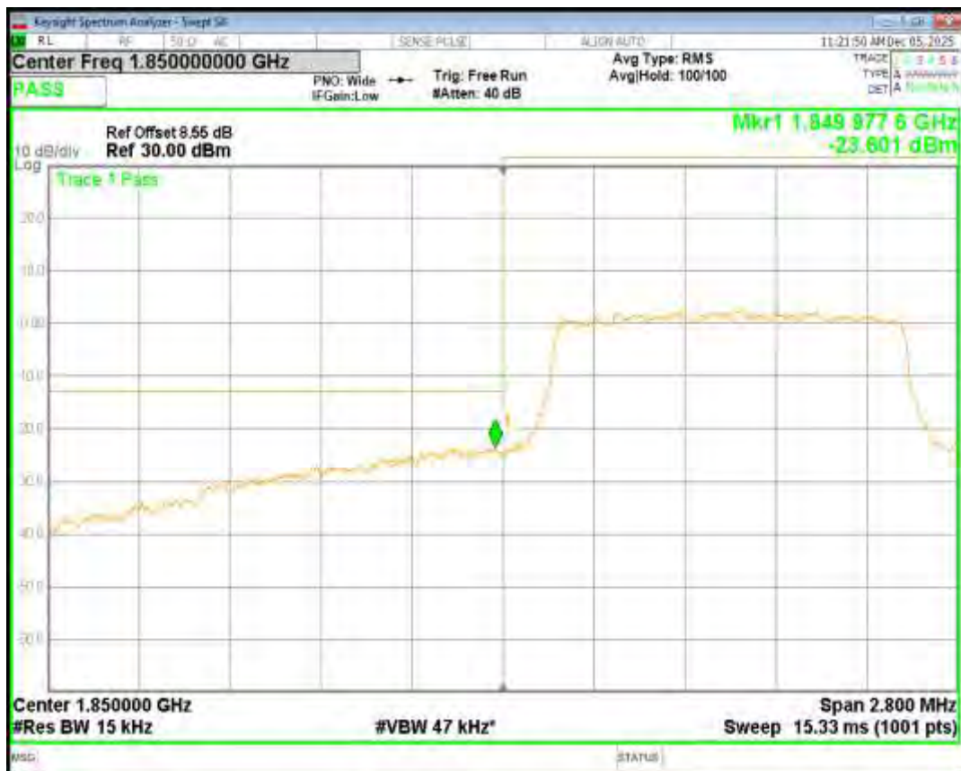
Band2 16QAM BW=1.4MHz Channel=19193 RB Size=6 Position=#0
