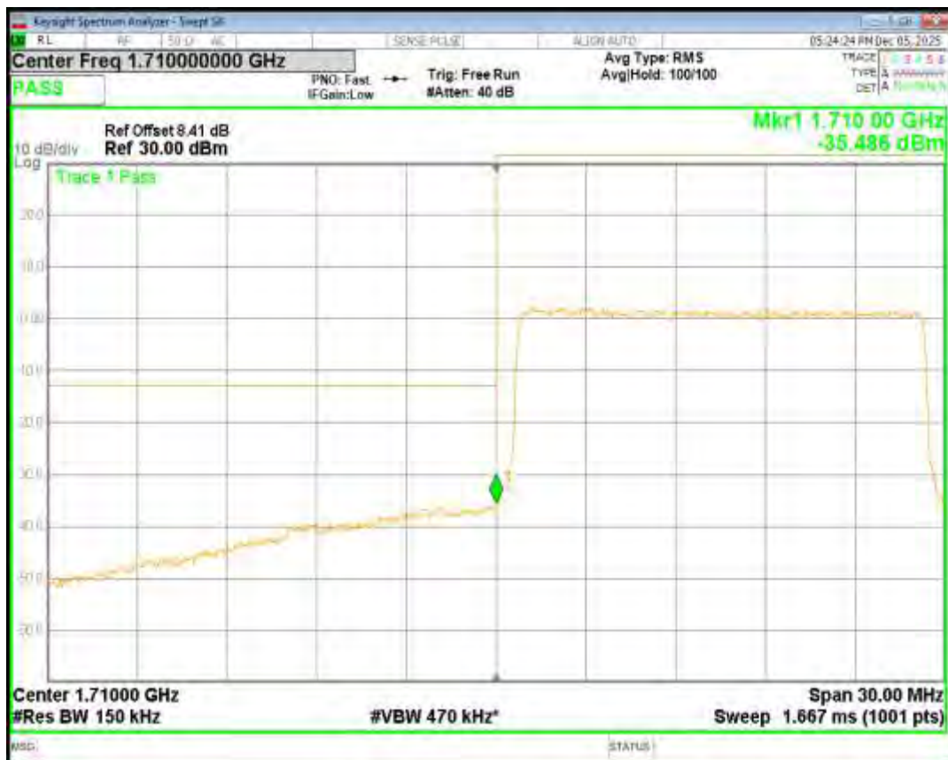
Band4 16QAM BW=15MHz Channel=20325 RB Size=75 Position=#0
