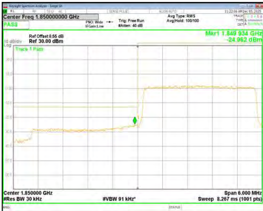
Band2 QPSK BW=3MHz Channel=19185 RB Size=15 Position=#0
