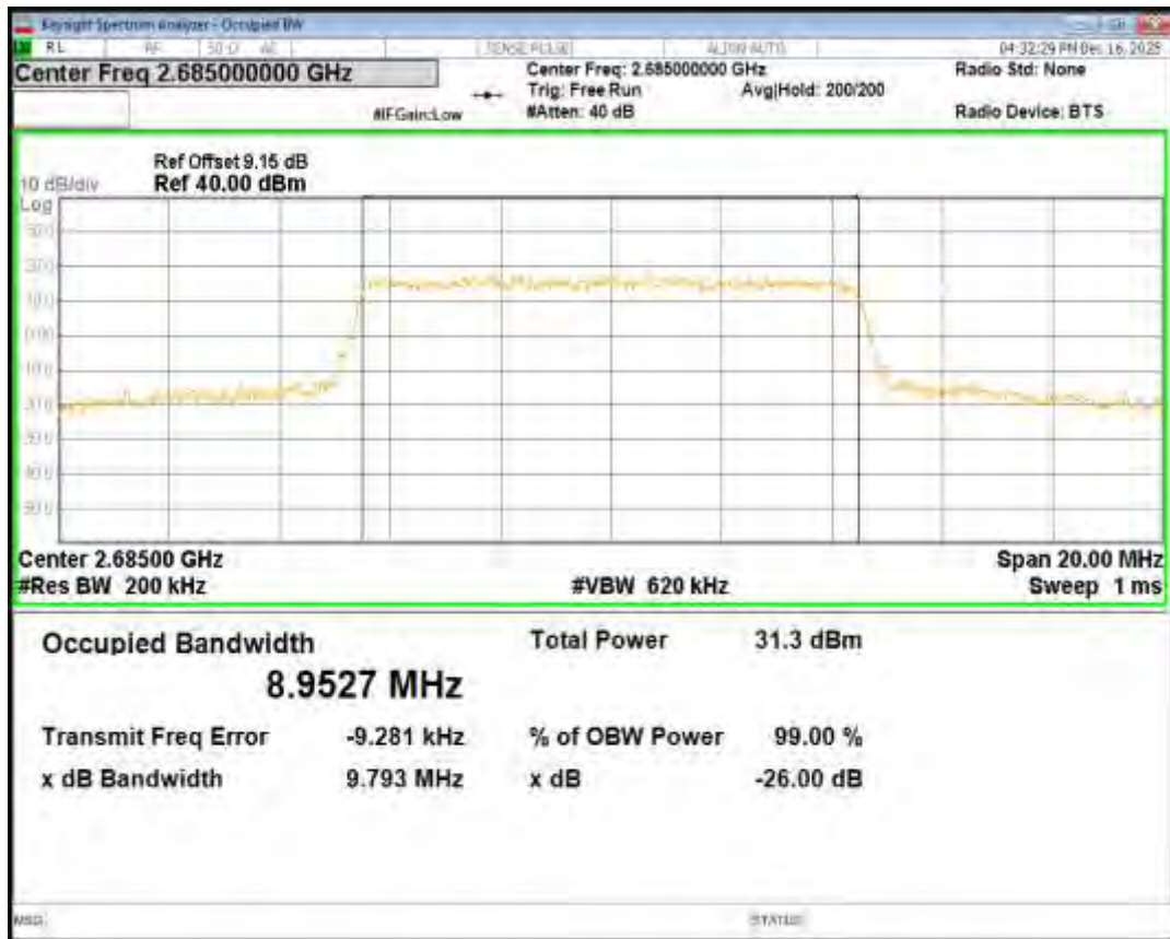
Band41 QPSK BW=15MHz Channel=39725 RB Size=75 Position=#0
