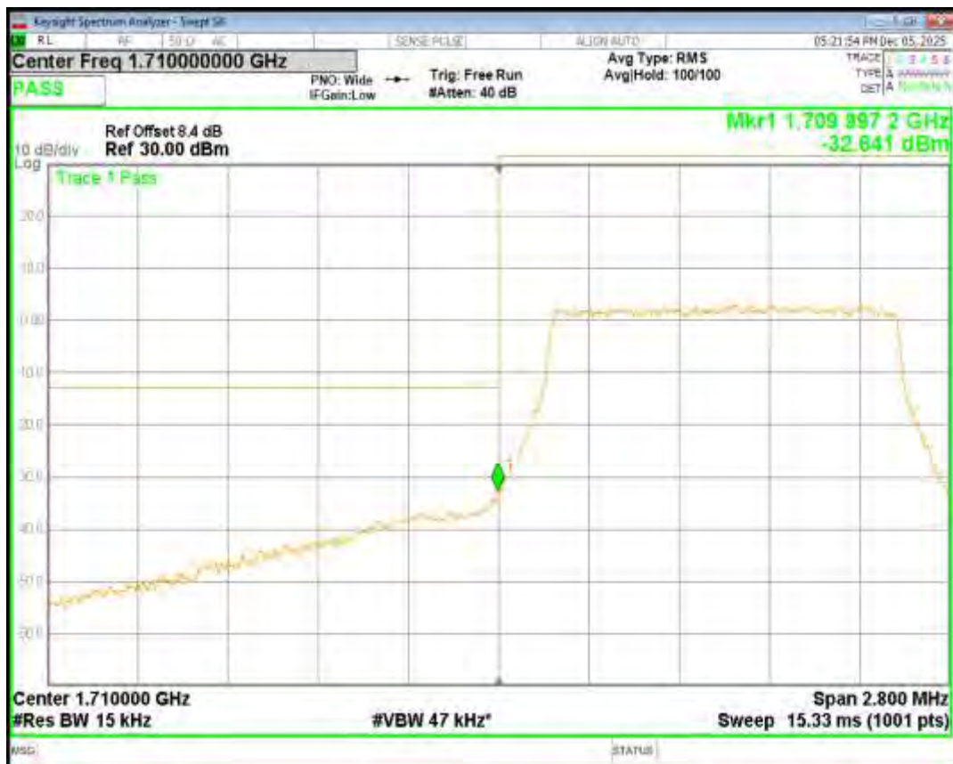
Band4 16QAM BW=1.4MHz Channel=20393 RB Size=6 Position=#0
