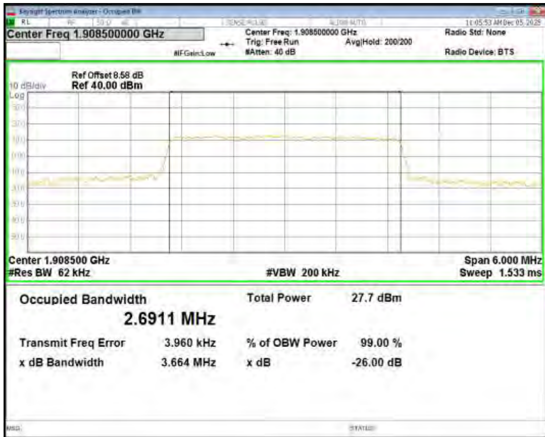
Band2 16QAM BW=5MHz Channel=18625 RB Size=25 Position=#0
