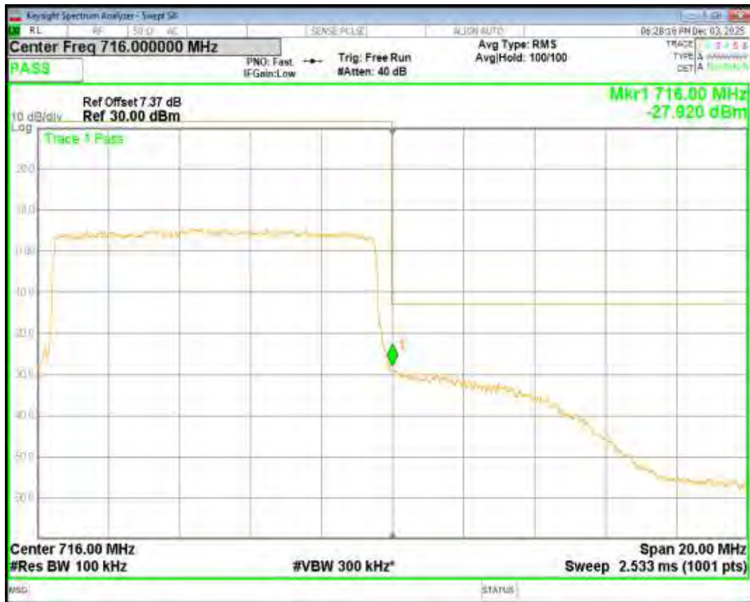
Band17 16QAM BW=5MHz Channel=23755 RB Size=25 Position=#0
