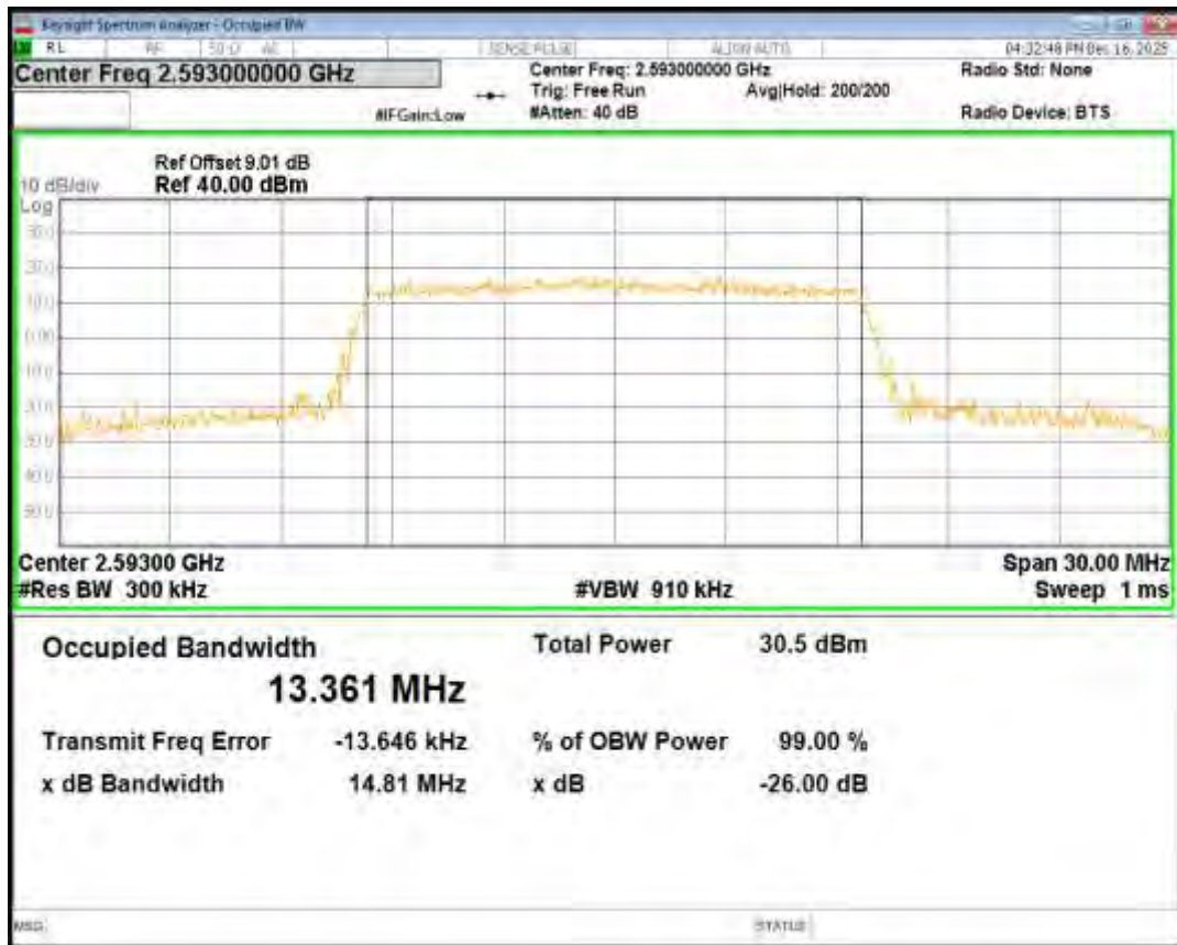
Band41 16QAM BW=15MHz Channel=41515 RB Size=75 Position=#0
