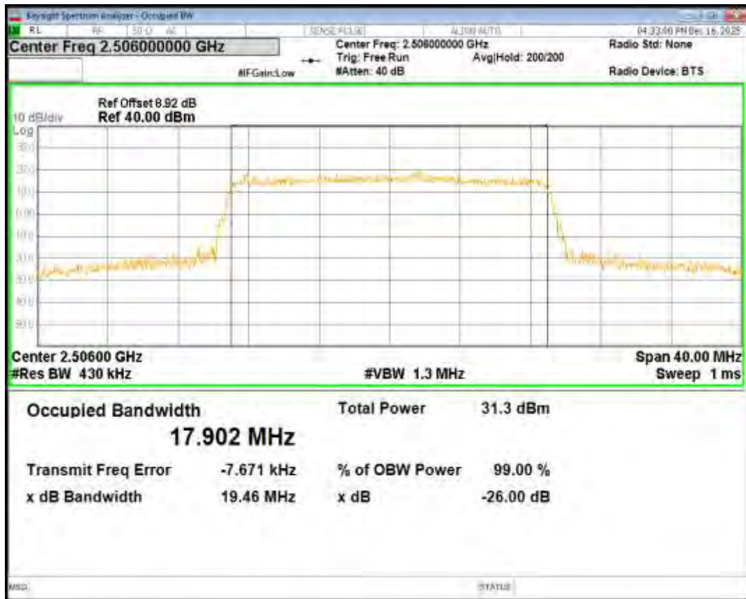
Band41 QPSK BW=20MHz Channel=40620 RB Size=100 Position=#0
