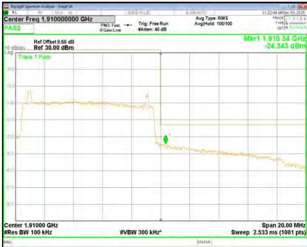
Band2 16QAM BW=15MHz Channel=18675 RB Size=75 Position=#0
