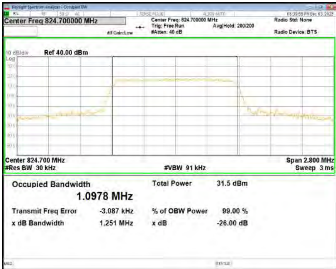
Band5 16QAM BW=1.4MHz Channel=20525 RB Size=6 Position=#0
