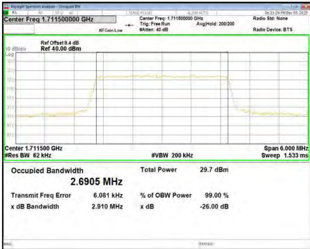
Band66 QPSK BW=3MHz Channel=132322 RB Size=15 Position=#0
