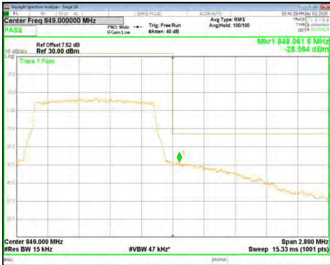
Band5 16QAM BW=10MHz Channel=20450 RB Size=50 Position=#0
