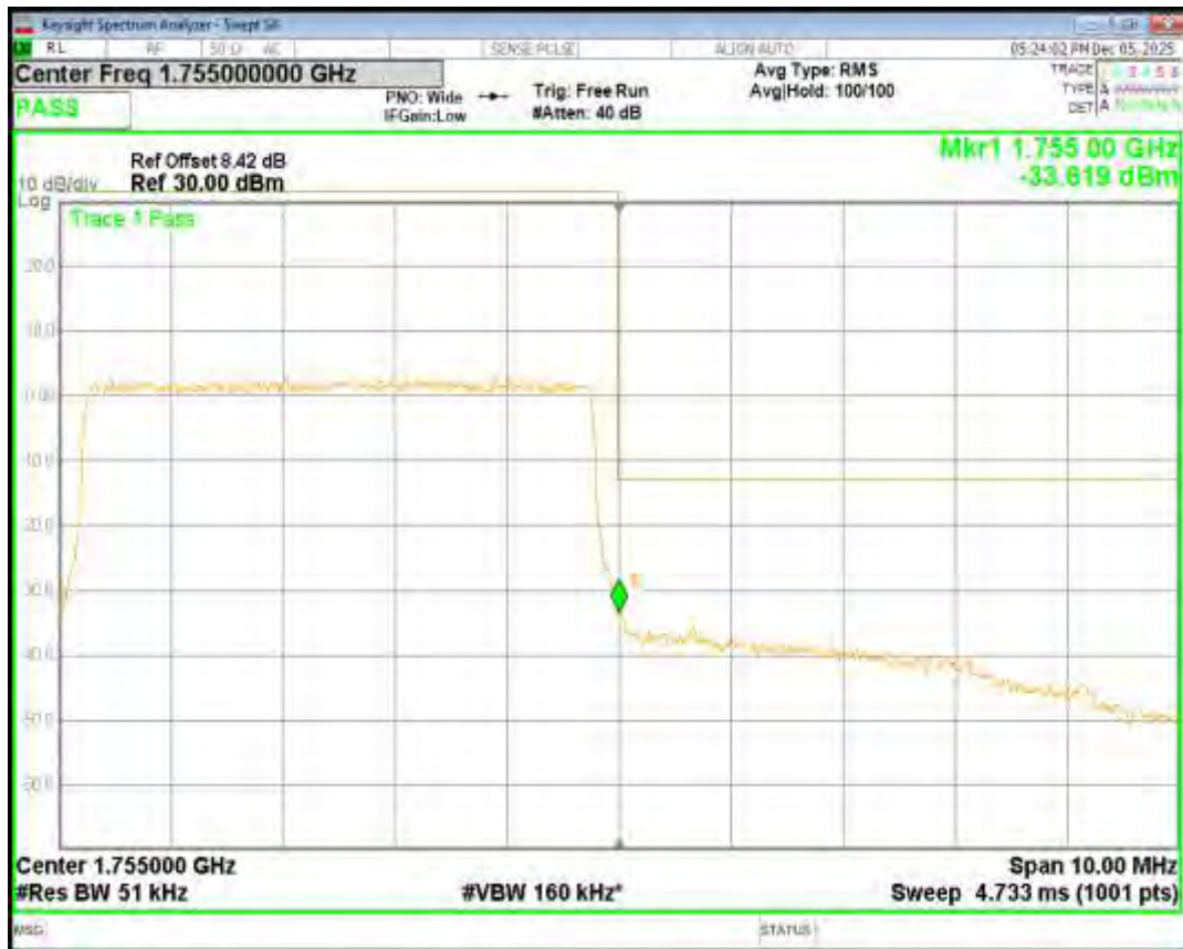
Band4 QPSK BW=1.4MHz Channel=19957 RB Size=6 Position=#0
