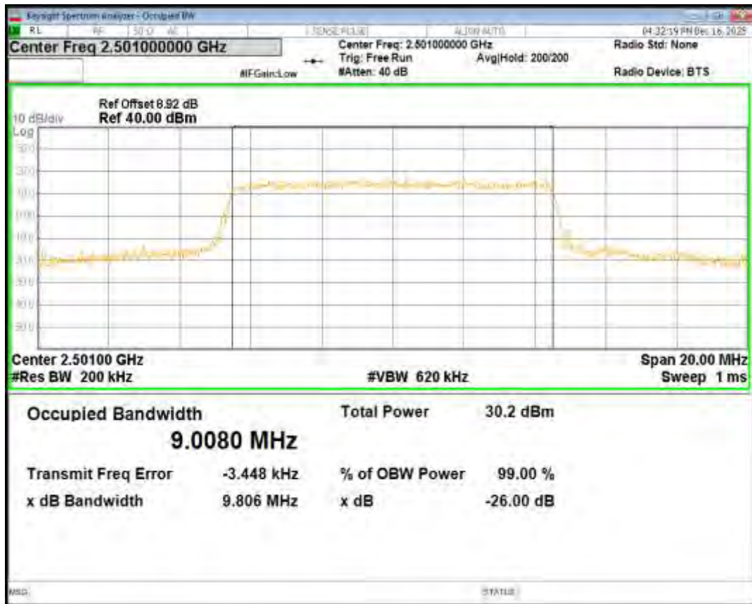
Band41 16QAM BW=10MHz Channel=40620 RB Size=50 Position=#0
