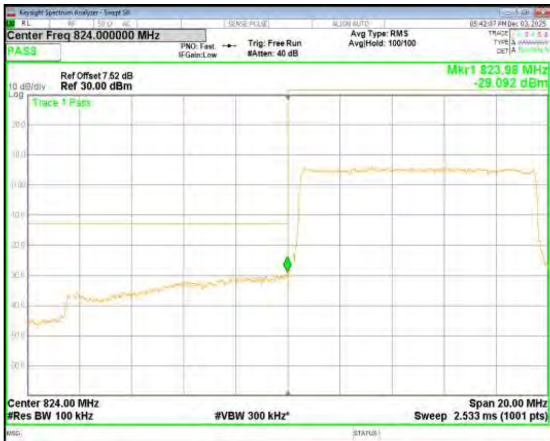
Band5 QPSK BW=10MHz Channel=20600 RB Size=50 Position=#0
