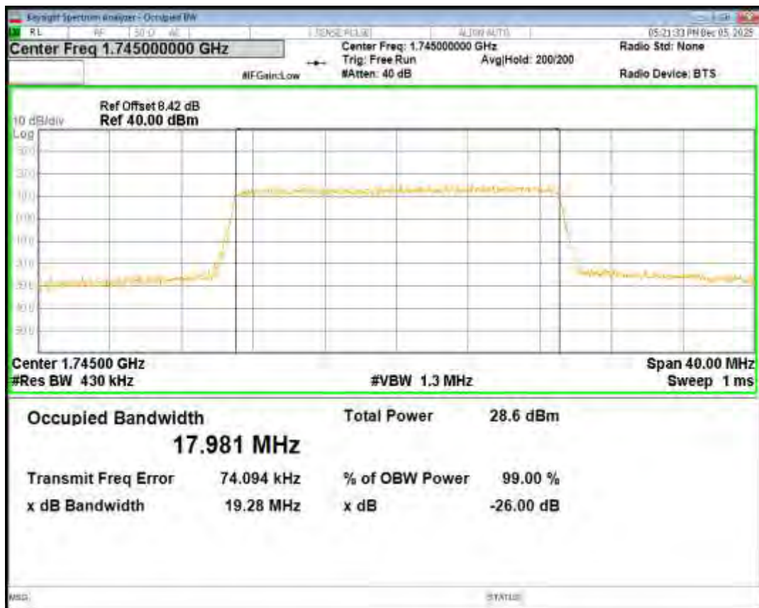
Band4 16QAM BW=3MHz Channel=19965 RB Size=15 Position=#0
