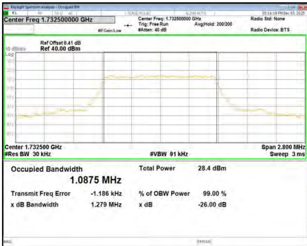
Band4 16QAM BW=1.4MHz Channel=20393 RB Size=6 Position=#0
