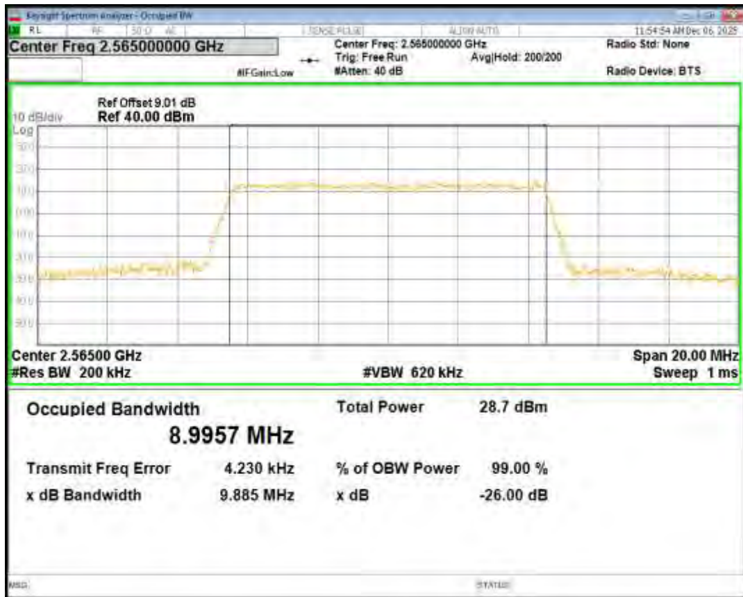
Band7 16QAM BW=15MHz Channel=20825 RB Size=75 Position=#0
