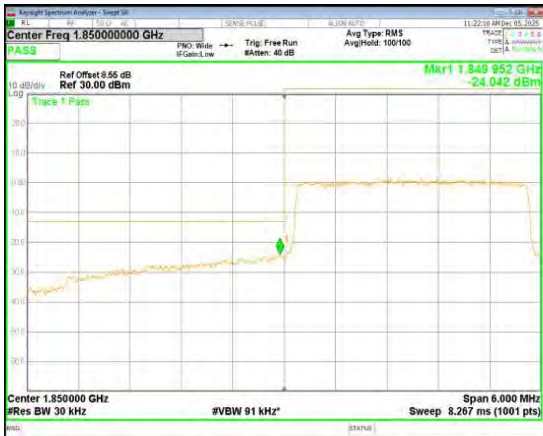
Band2 16QAM BW=3MHz Channel=19185 RB Size=15 Position=#0
