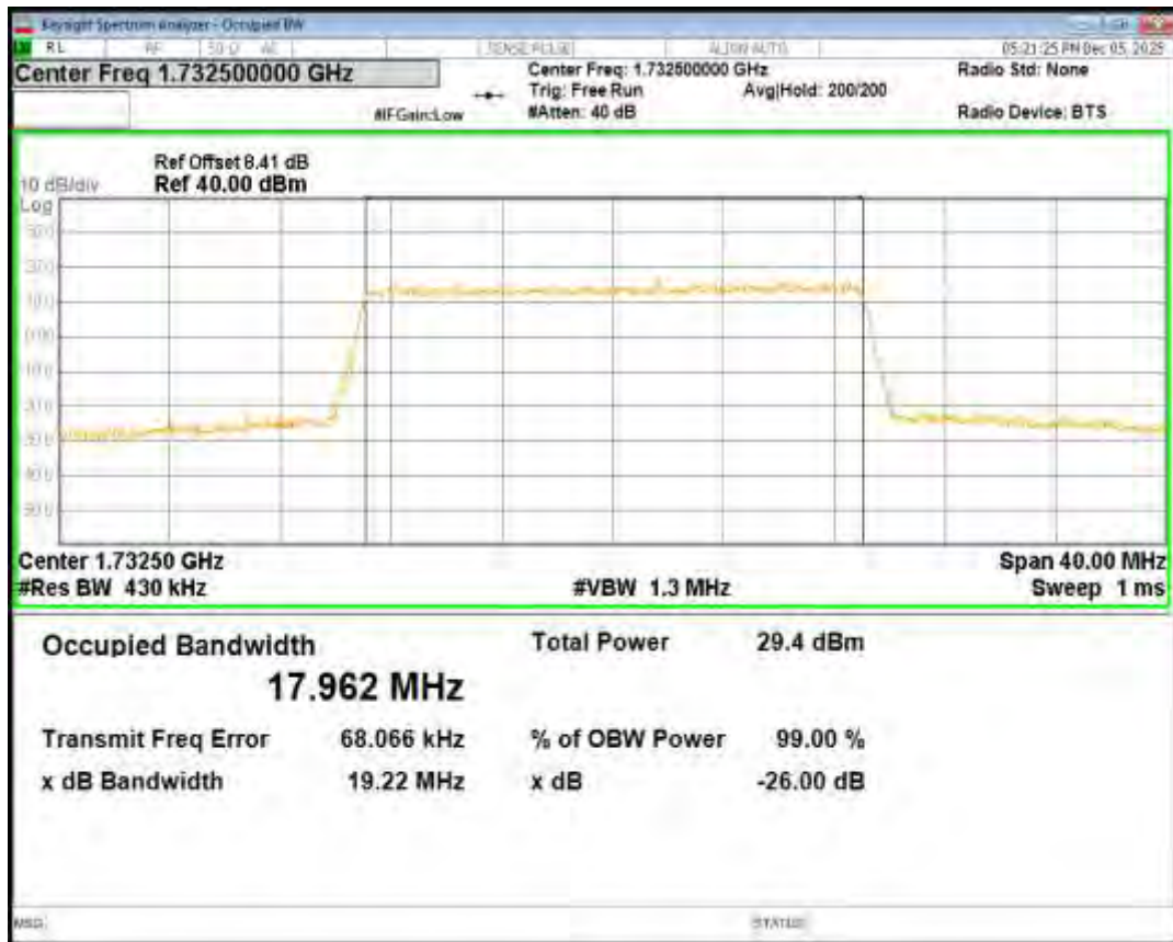
Band4 QPSK BW=20MHz Channel=20300 RB Size=100 Position=#0
