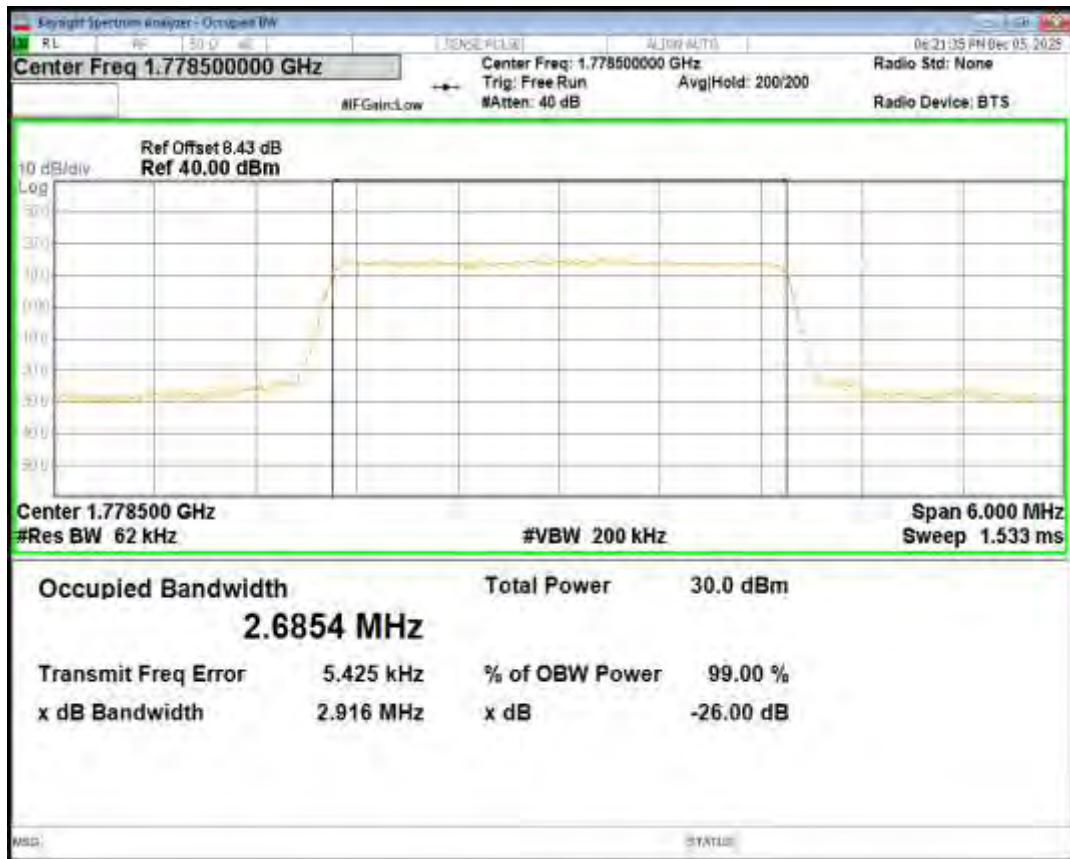
Band66 QPSK BW=5MHz Channel=131997 RB Size=25 Position=#0
