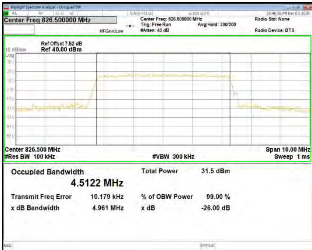
Band5 16QAM BW=5MHz Channel=20525 RB Size=25 Position=#0
