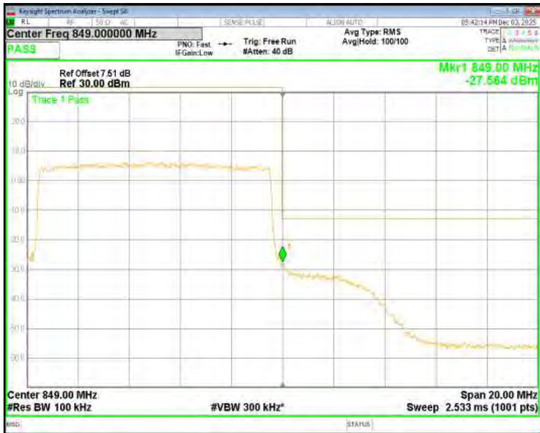
Band5 QPSK BW=3MHz Channel=20415 RB Size=15 Position=#0
