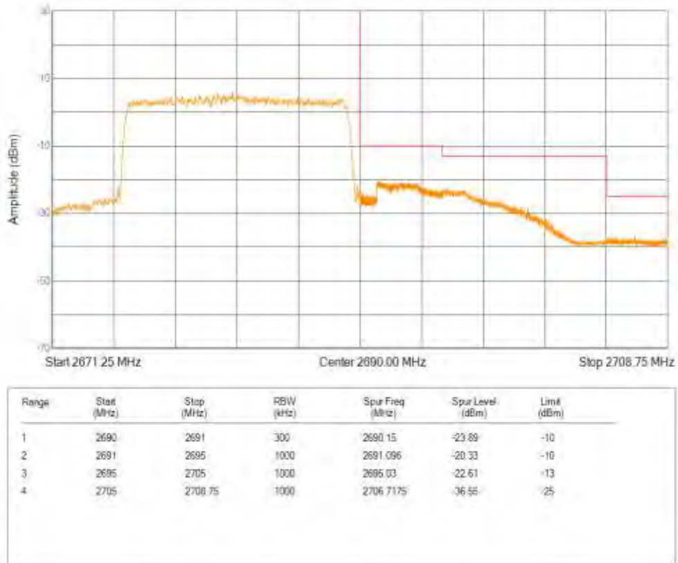
Band41 QPSK BW=20MHz Channel=39750 RB Size=100 Position=#0
