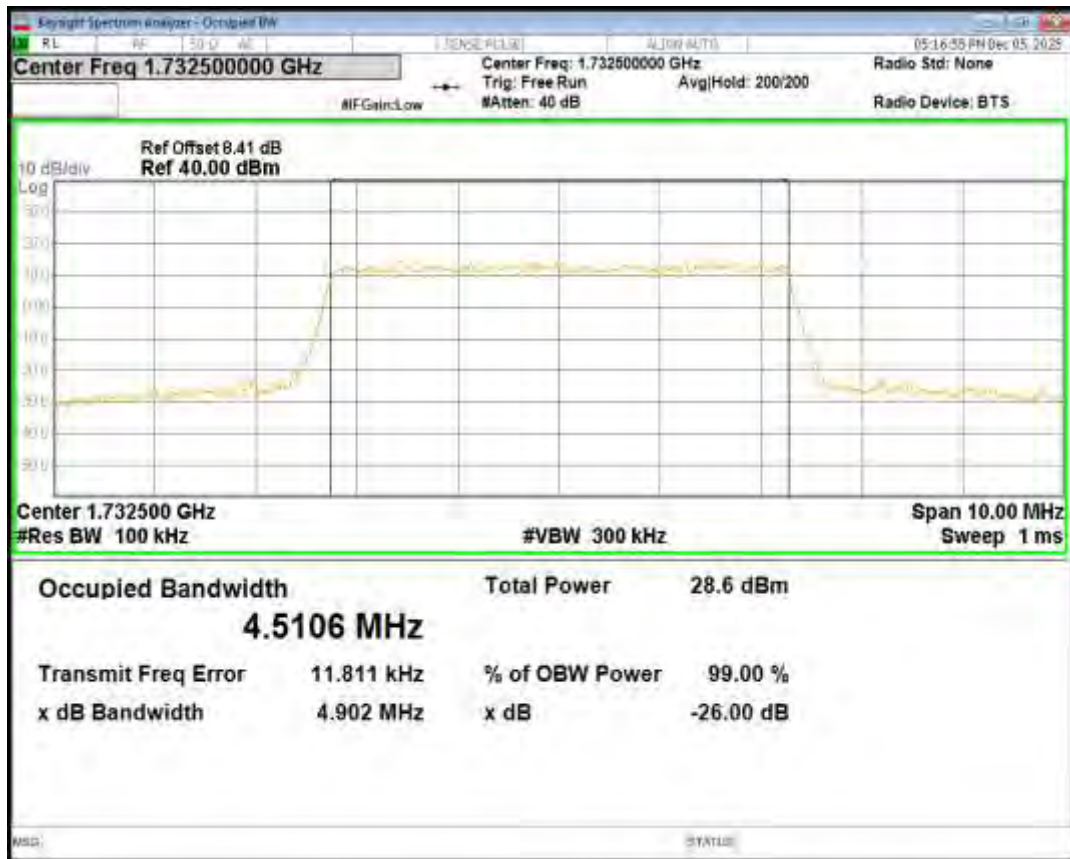
Band4 16QAM BW=5MHz Channel=20375 RB Size=25 Position=#0
