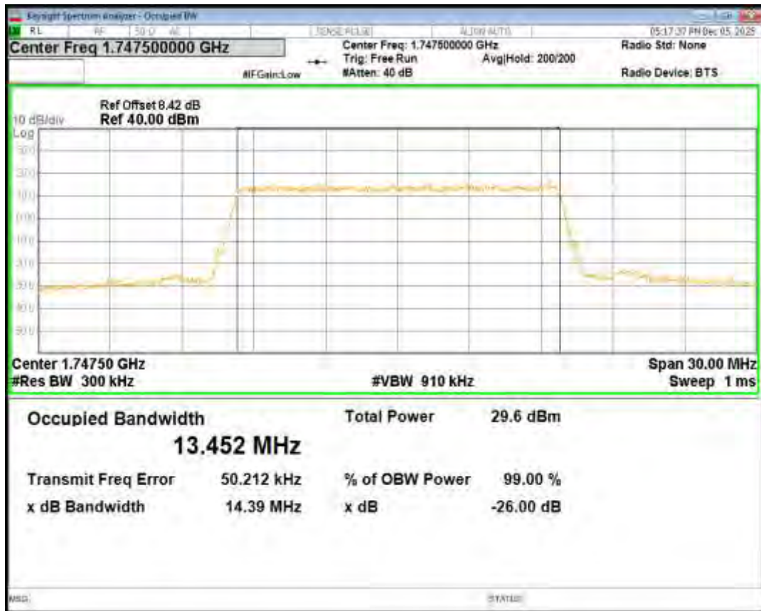
Band4 QPSK BW=20MHz Channel=20050 RB Size=100 Position=#0
