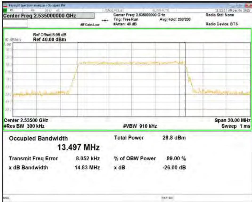
Band7 16QAM BW=15MHz Channel=21375 RB Size=75 Position=#0
