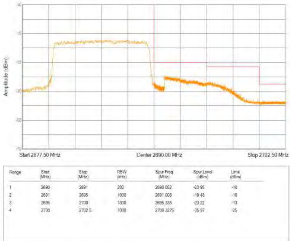
Band41 QPSK BW=15MHz Channel=39725 RB Size=75 Position=#0
