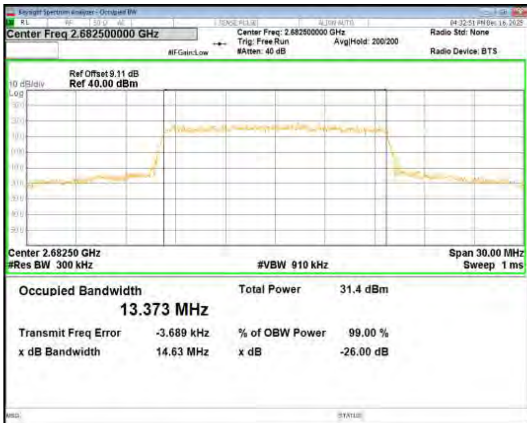
Band41 QPSK BW=20MHz Channel=39750 RB Size=100 Position=#0
