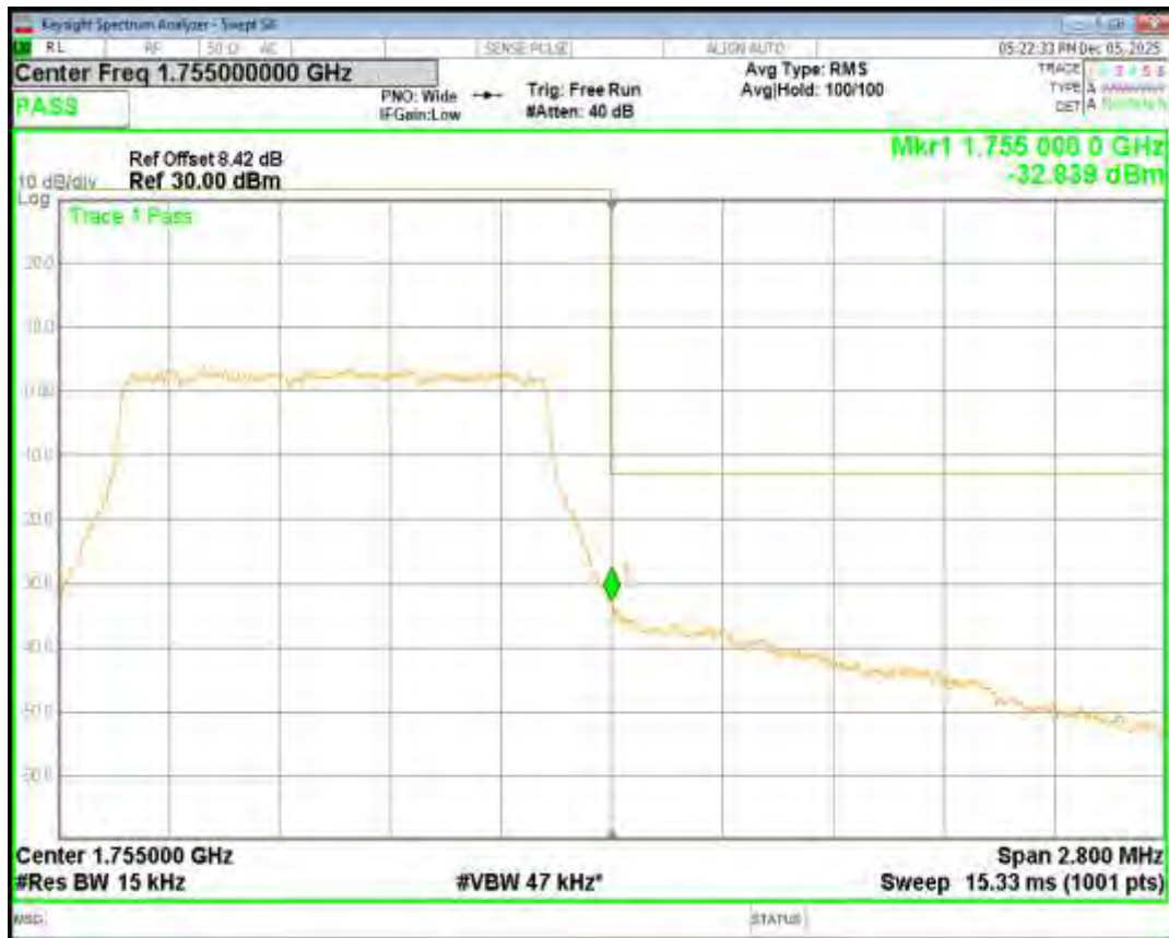
Band4 16QAM BW=10MHz Channel=20000 RB Size=50 Position=#0
