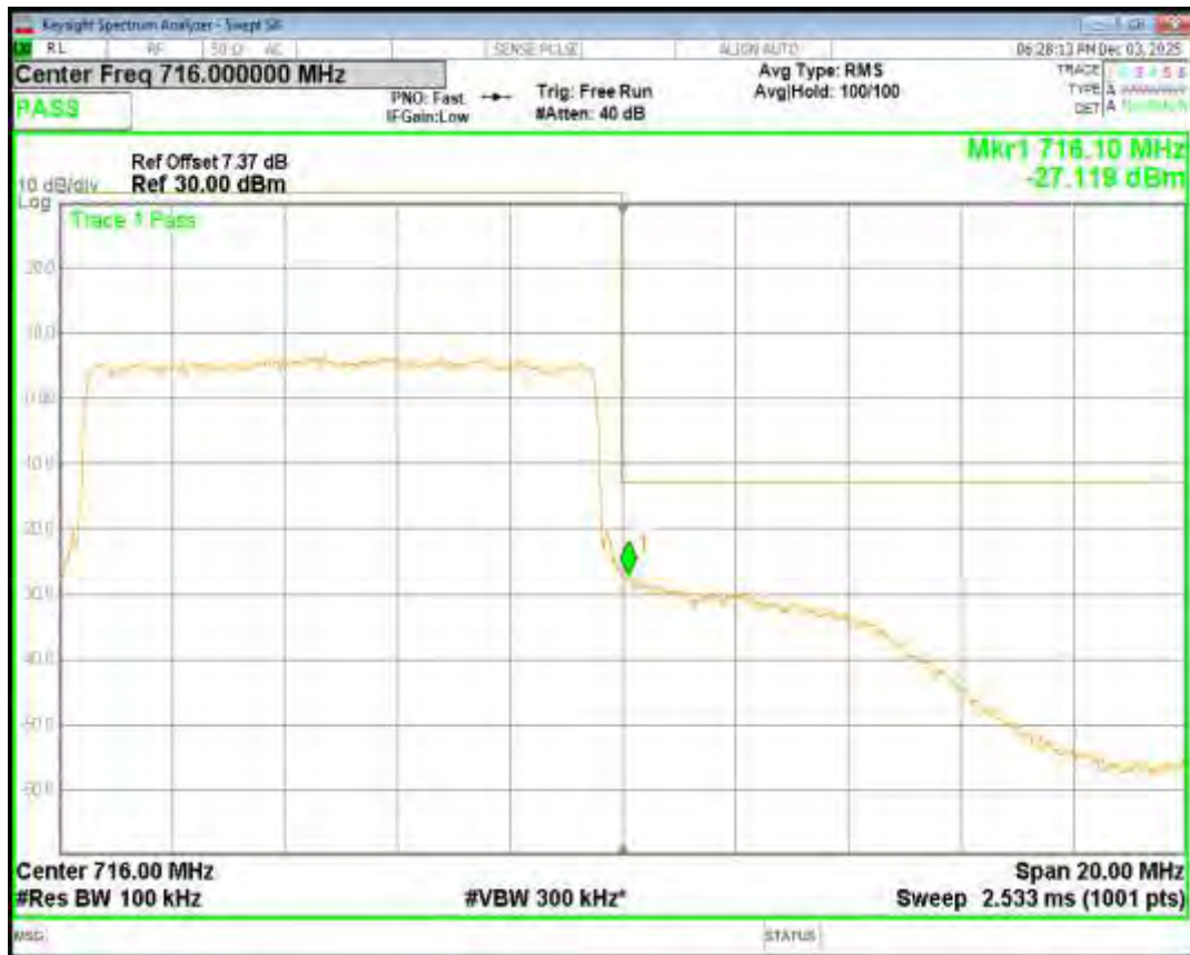
Band17 QPSK BW=5MHz Channel=23755 RB Size=25 Position=#0
