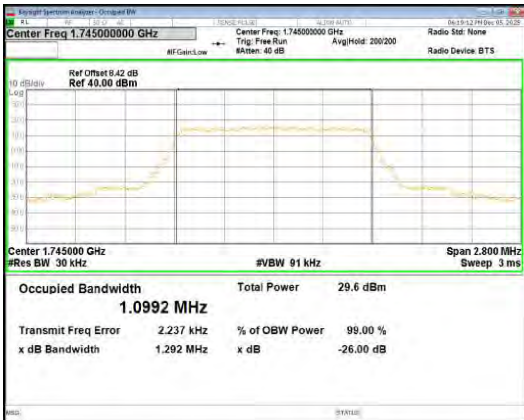
Band66 QPSK BW=1.4MHz Channel=132665 RB Size=6 Position=#0
