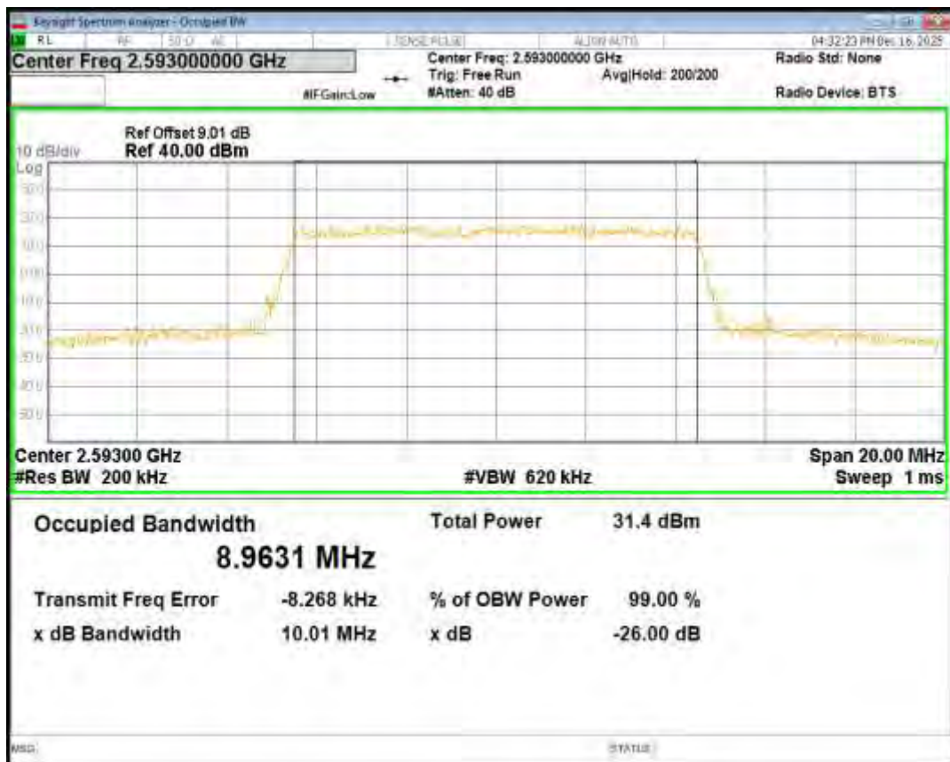
Band41 QPSK BW=10MHz Channel=41540 RB Size=50 Position=#0
