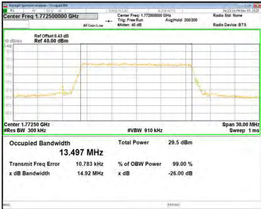
Band66 QPSK BW=20MHz Channel=132072 RB Size=100 Position=#0
