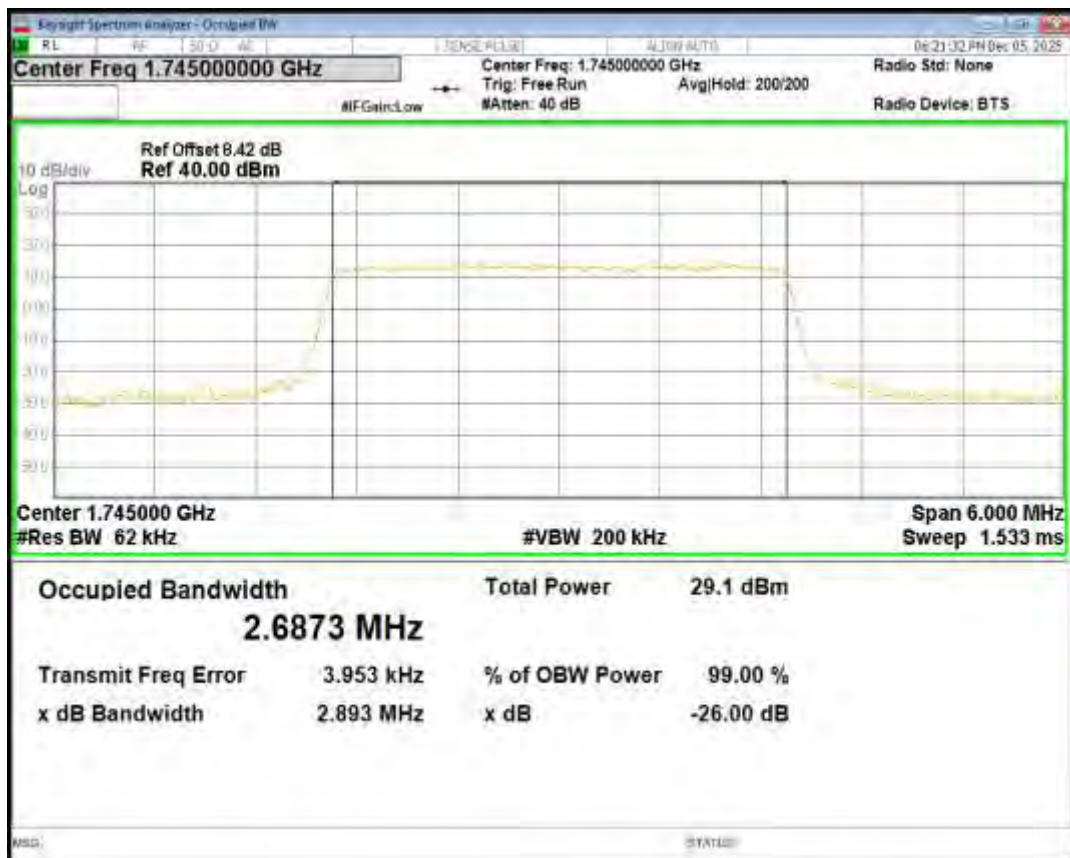
Band66 16QAM BW=3MHz Channel=132657 RB Size=15 Position=#0
