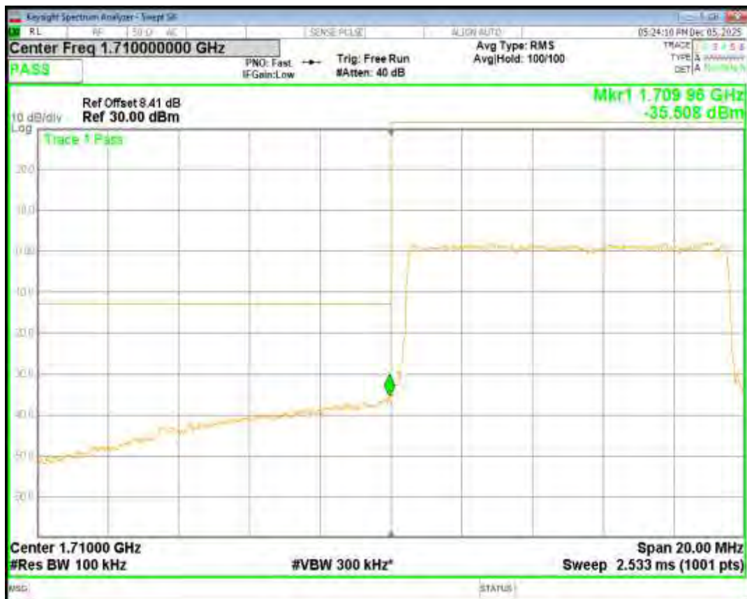
Band4 16QAM BW=10MHz Channel=20350 RB Size=50 Position=#0
