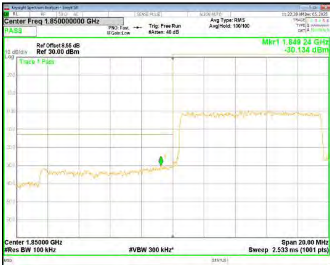
Band2 QPSK BW=10MHz Channel=19150 RB Size=50 Position=#0
