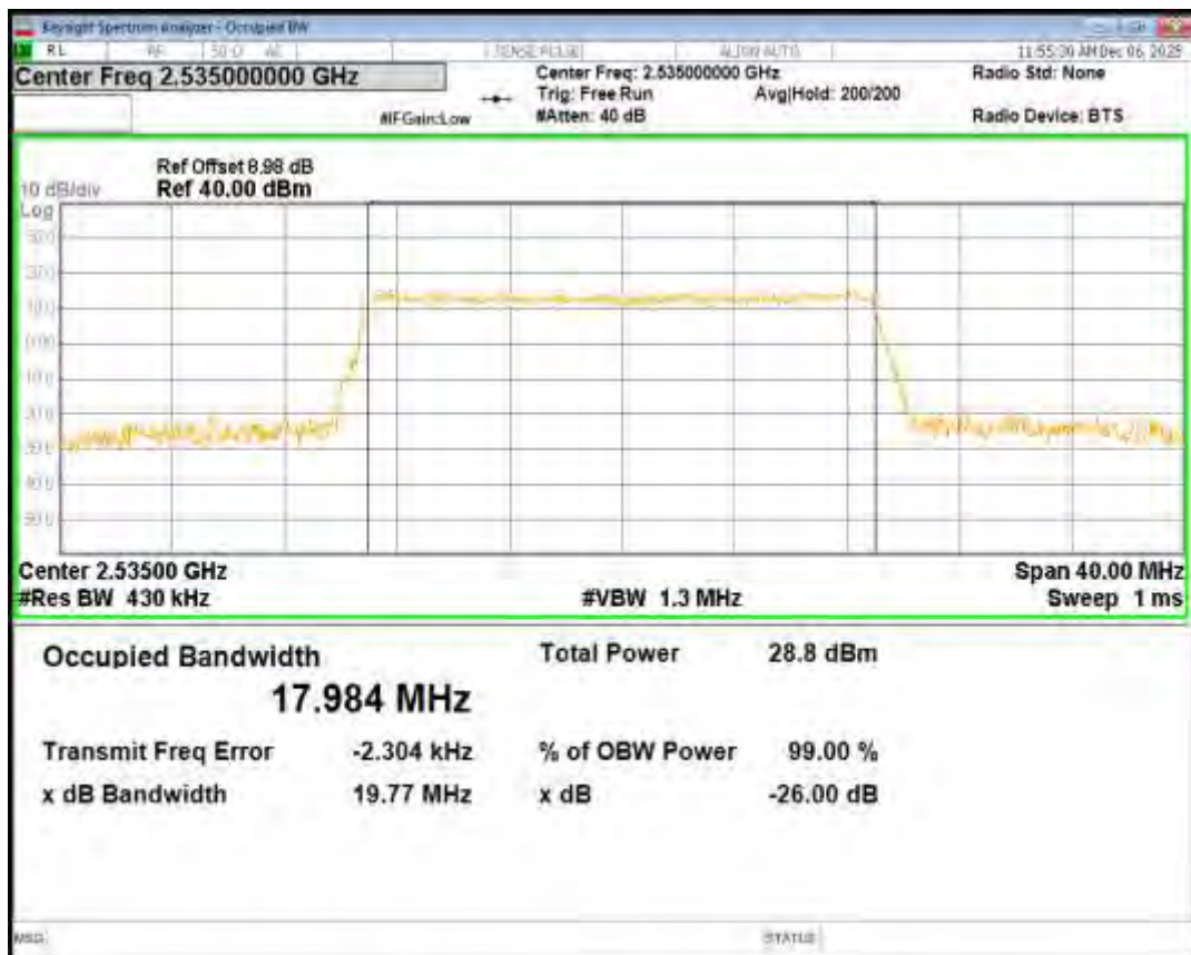
Band7 16QAM BW=20MHz Channel=21350 RB Size=100 Position=#0
