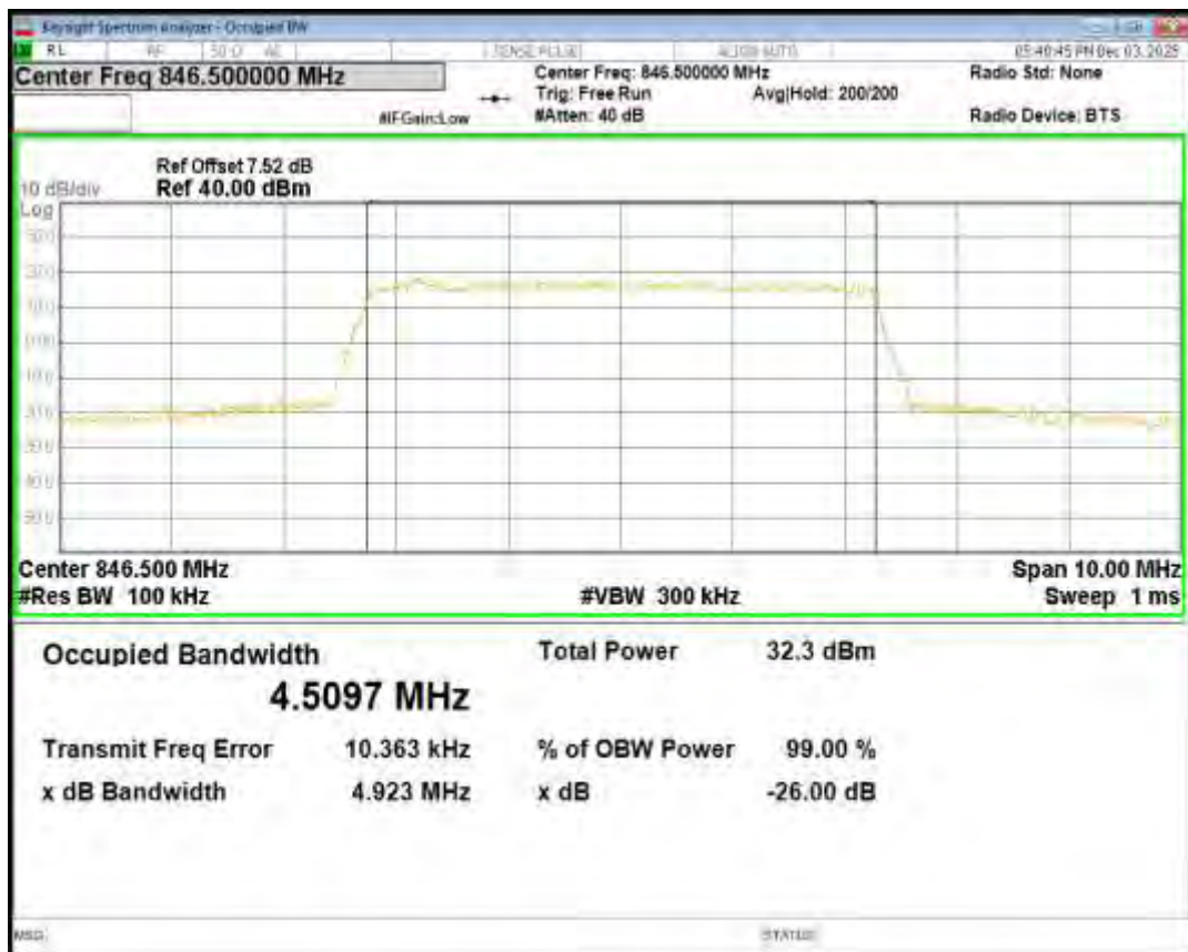
Band66 16QAM BW=1.4MHz Channel=131979 RB Size=6 Position=#0
