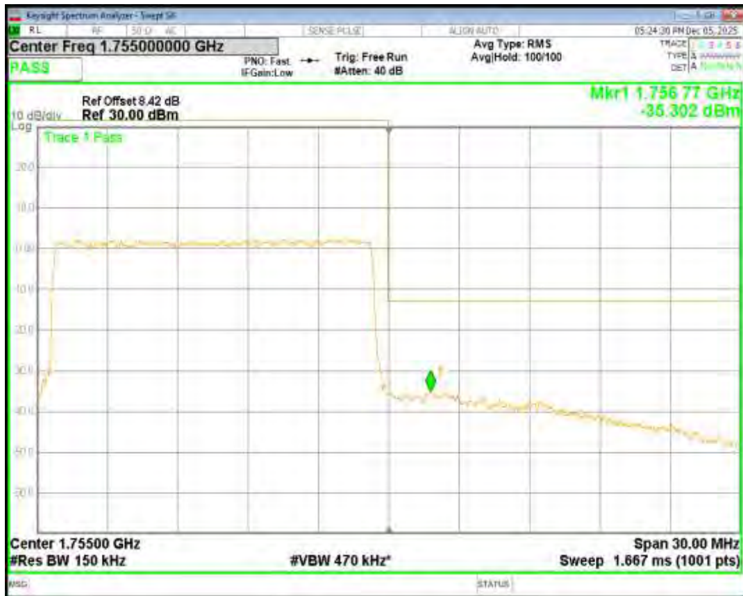
Band4 16QAM BW=20MHz Channel=20050 RB Size=100 Position=#0
