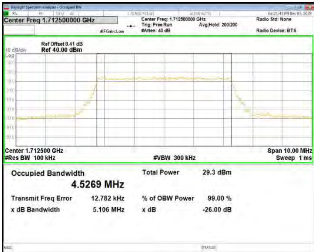
Band66 QPSK BW=5MHz Channel=132322 RB Size=25 Position=#0
