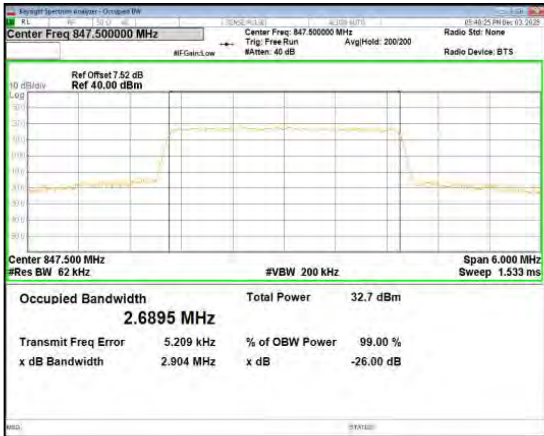
Band5 QPSK BW=5MHz Channel=20425 RB Size=25 Position=#0
