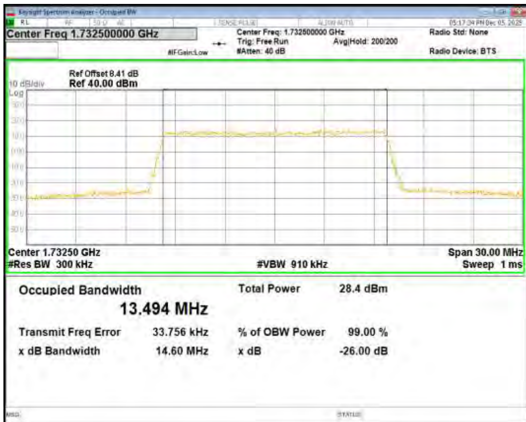
Band4 16QAM BW=15MHz Channel=20325 RB Size=75 Position=#0
