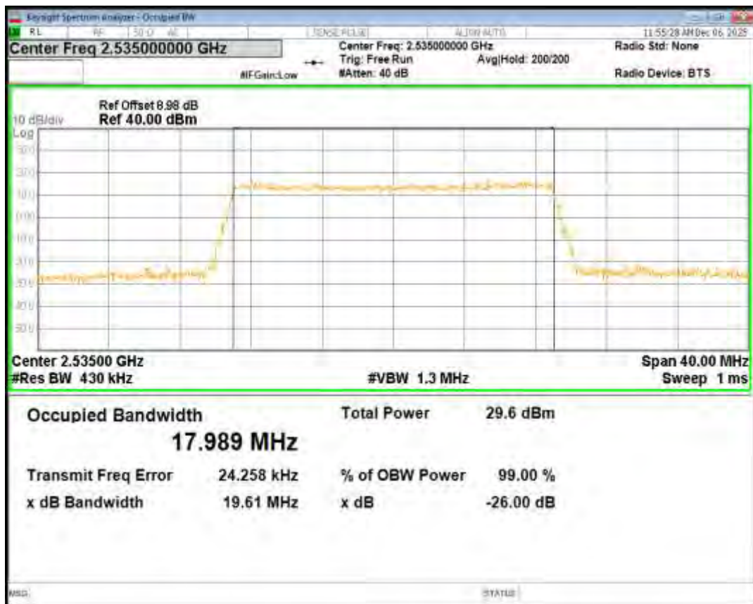
Band7 QPSK BW=20MHz Channel=21350 RB Size=100 Position=#0
