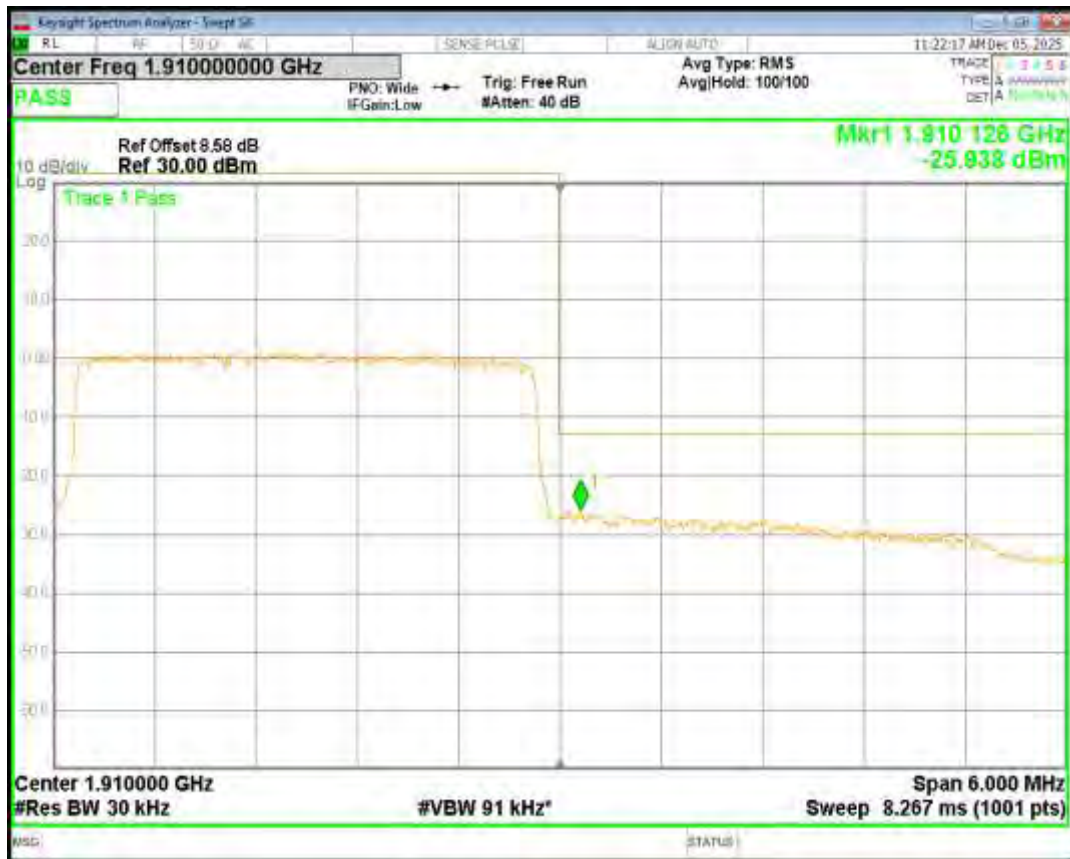
Band2 16QAM BW=5MHz Channel=18625 RB Size=25 Position=#0
