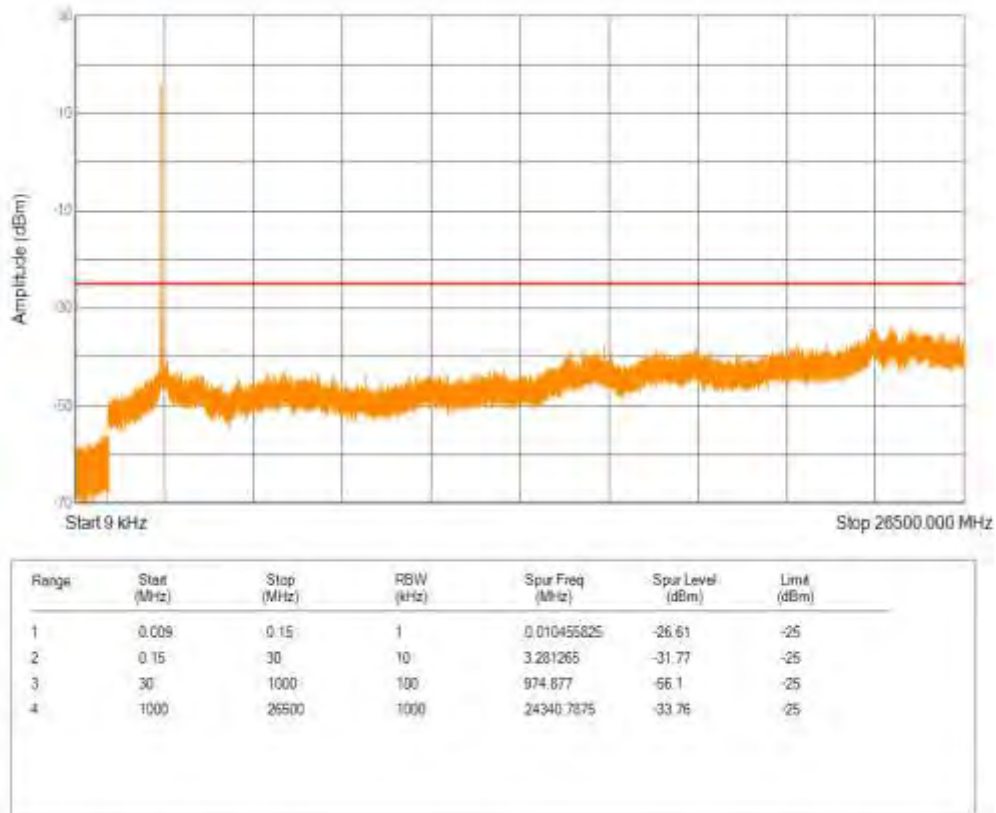
Band7 16QAM BW=20MHz Channel=20850 RB Size=100 Position=#0
