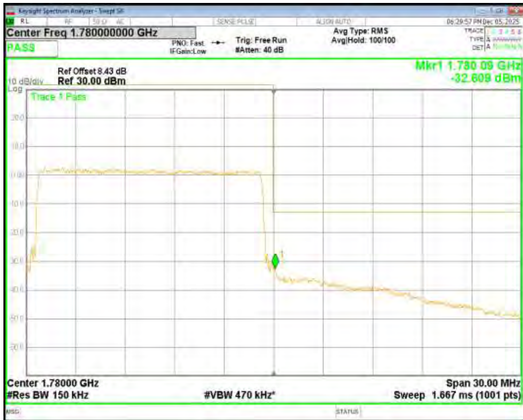
Band66 16QAM BW=20MHz Channel=132072 RB Size=100 Position=#0
