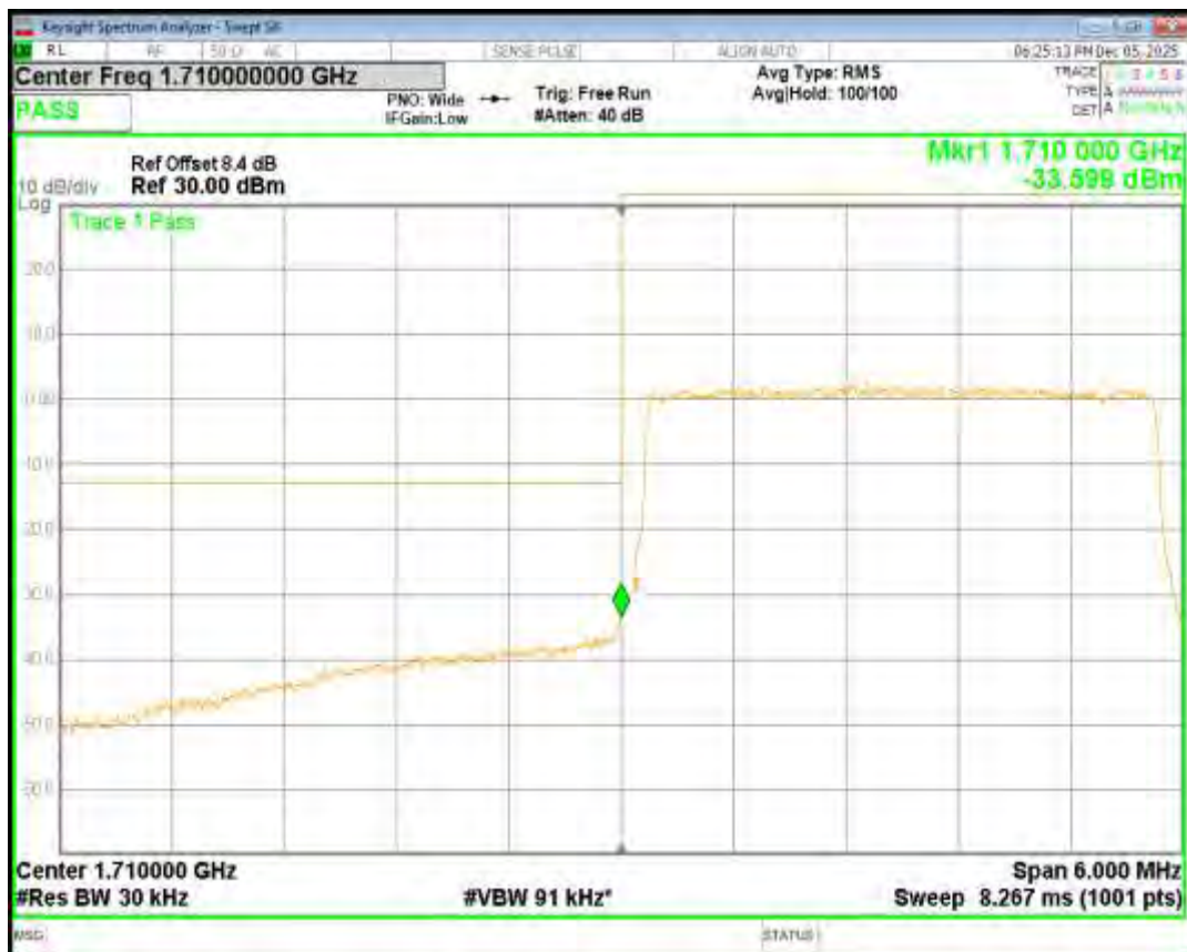
Band66 16QAM BW=3MHz Channel=132657 RB Size=15 Position=#0
