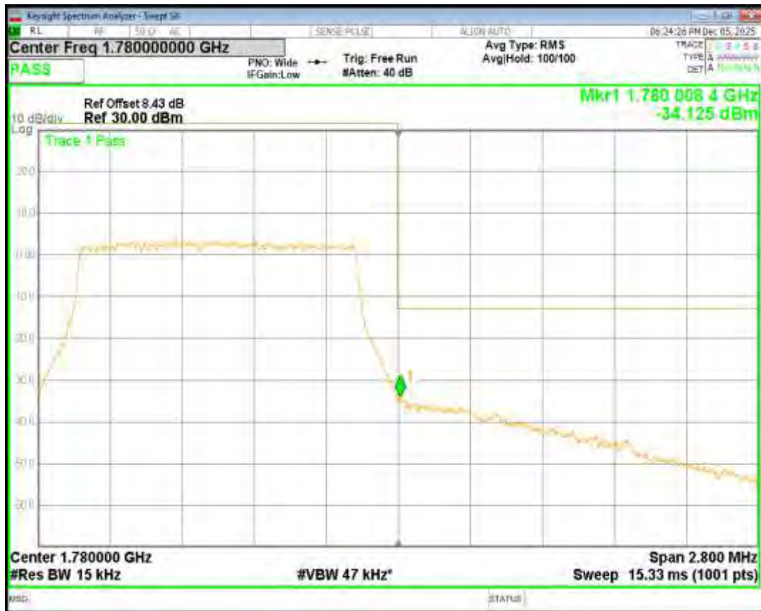
Band66 16QAM BW=10MHz Channel=132022 RB Size=50 Position=#0
