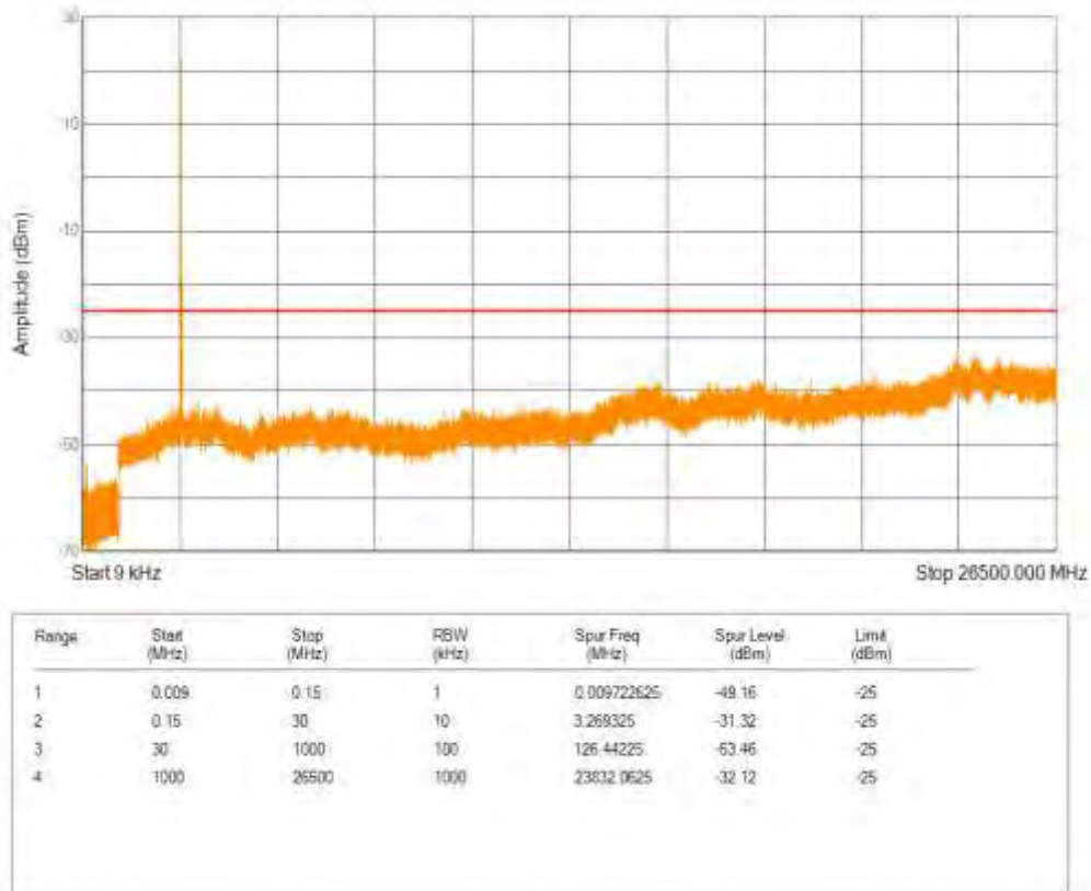
Band41 QPSK BW=10MHz Channel=39700 RB Size=50 Position=#0
