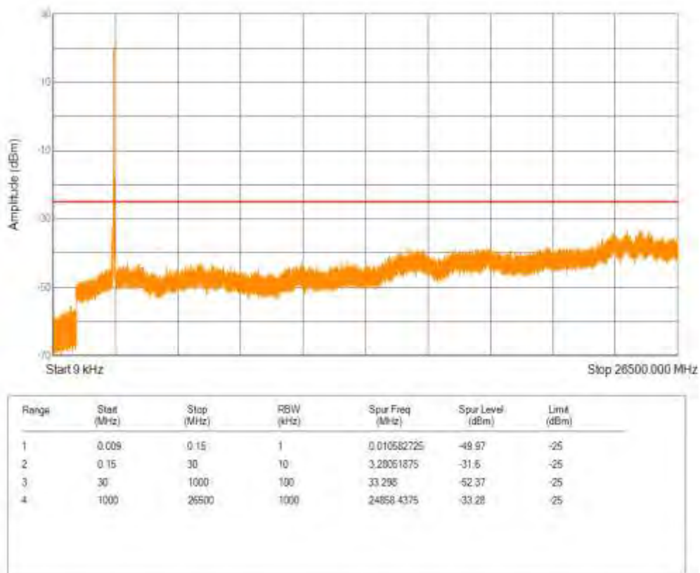
Band41 QPSK BW=15MHz Channel=41515 RB Size=75 Position=#0
