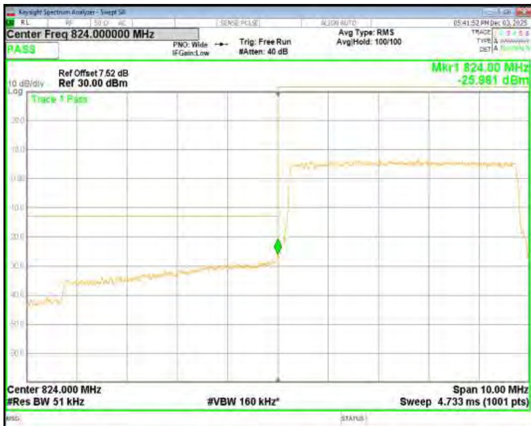
Band5 QPSK BW=5MHz Channel=20625 RB Size=25 Position=#0
