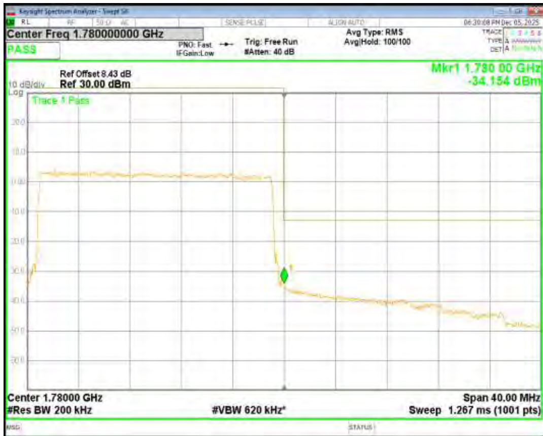
Band66 QPSK BW=3MHz Channel=131987 RB Size=15 Position=#0
