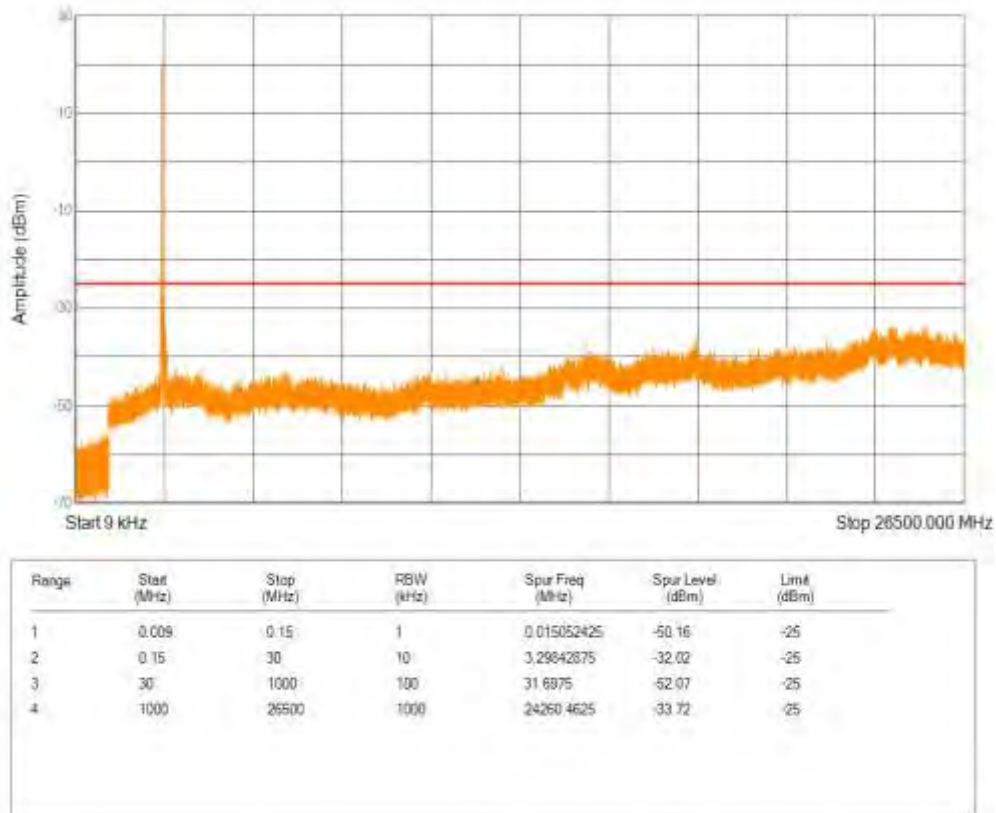
Band41 QPSK BW=10MHz Channel=41540 RB Size=50 Position=#0
