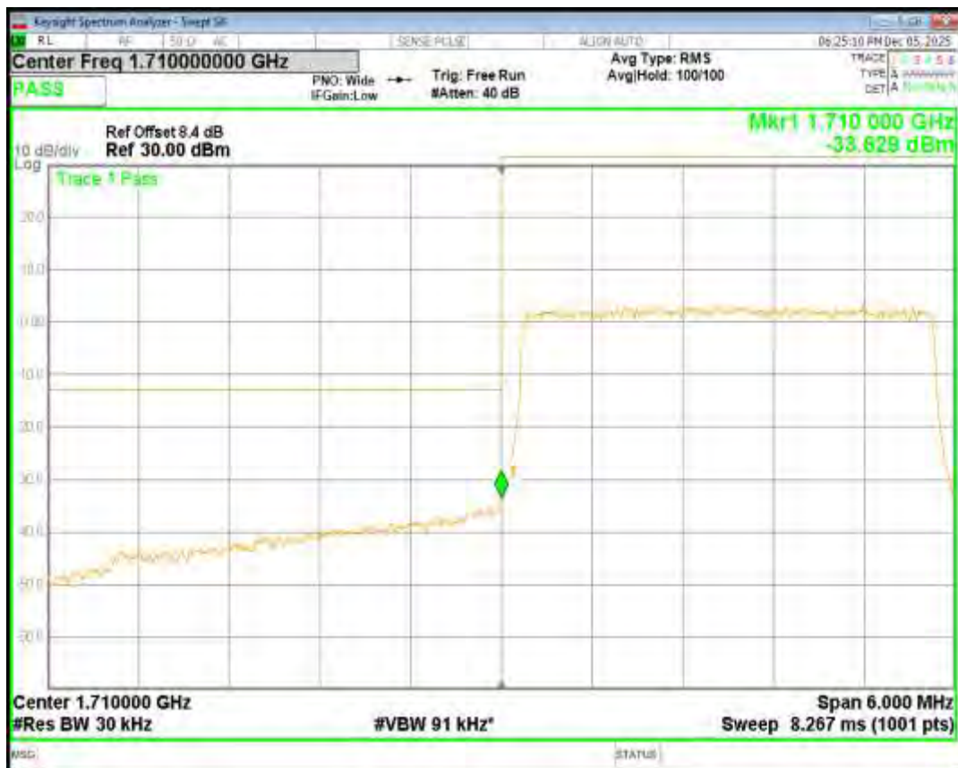
Band66 QPSK BW=3MHz Channel=132657 RB Size=15 Position=#0
