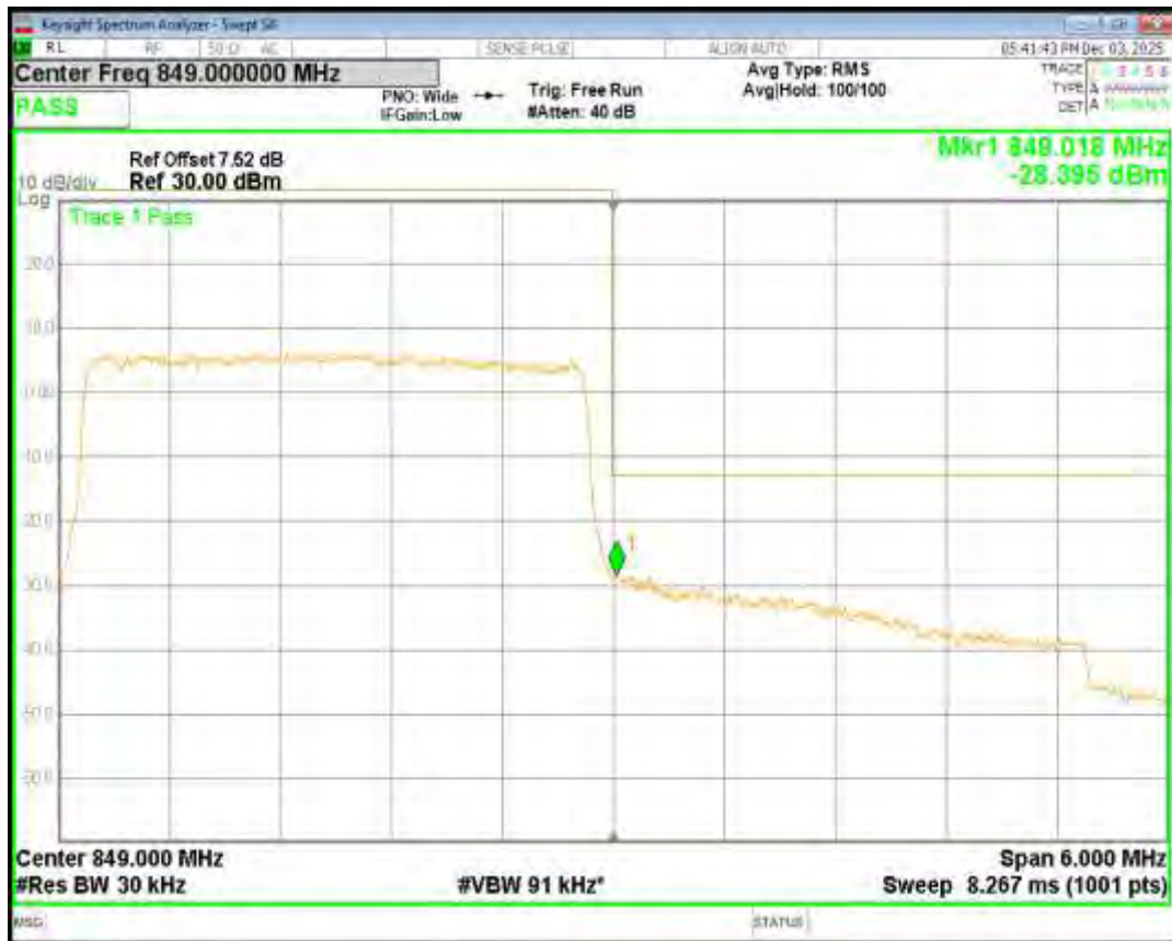
Band5 QPSK BW=5MHz Channel=20425 RB Size=25 Position=#0
