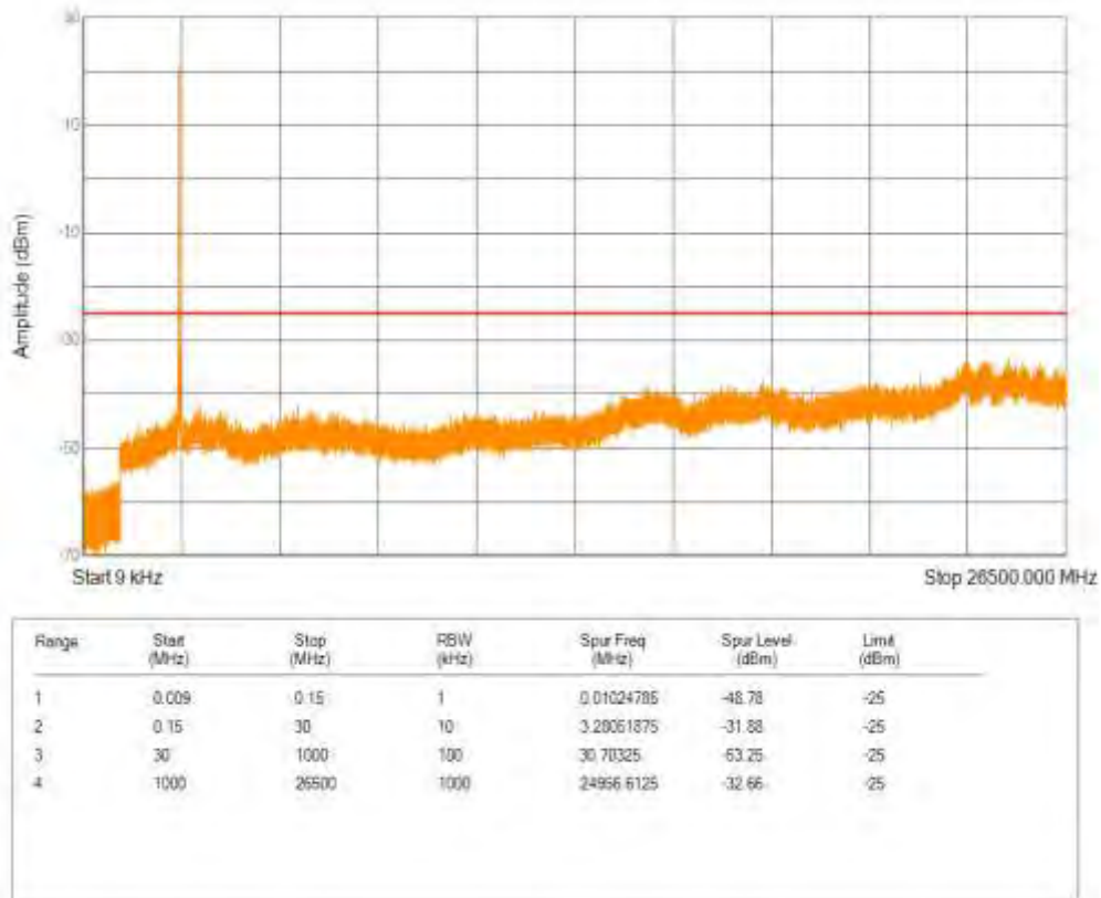
Band41 16QAM BW=10MHz Channel=41540 RB Size=50 Position=#0
