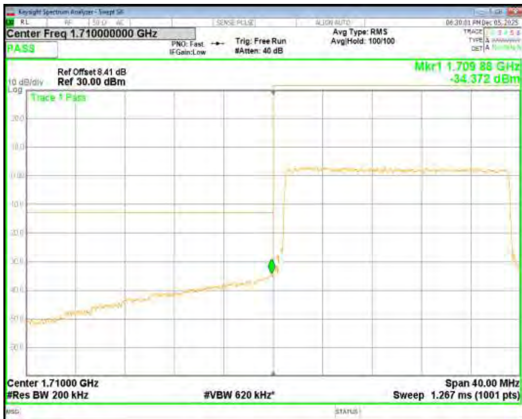
Band66 QPSK BW=20MHz Channel=132572 RB Size=100 Position=#0
