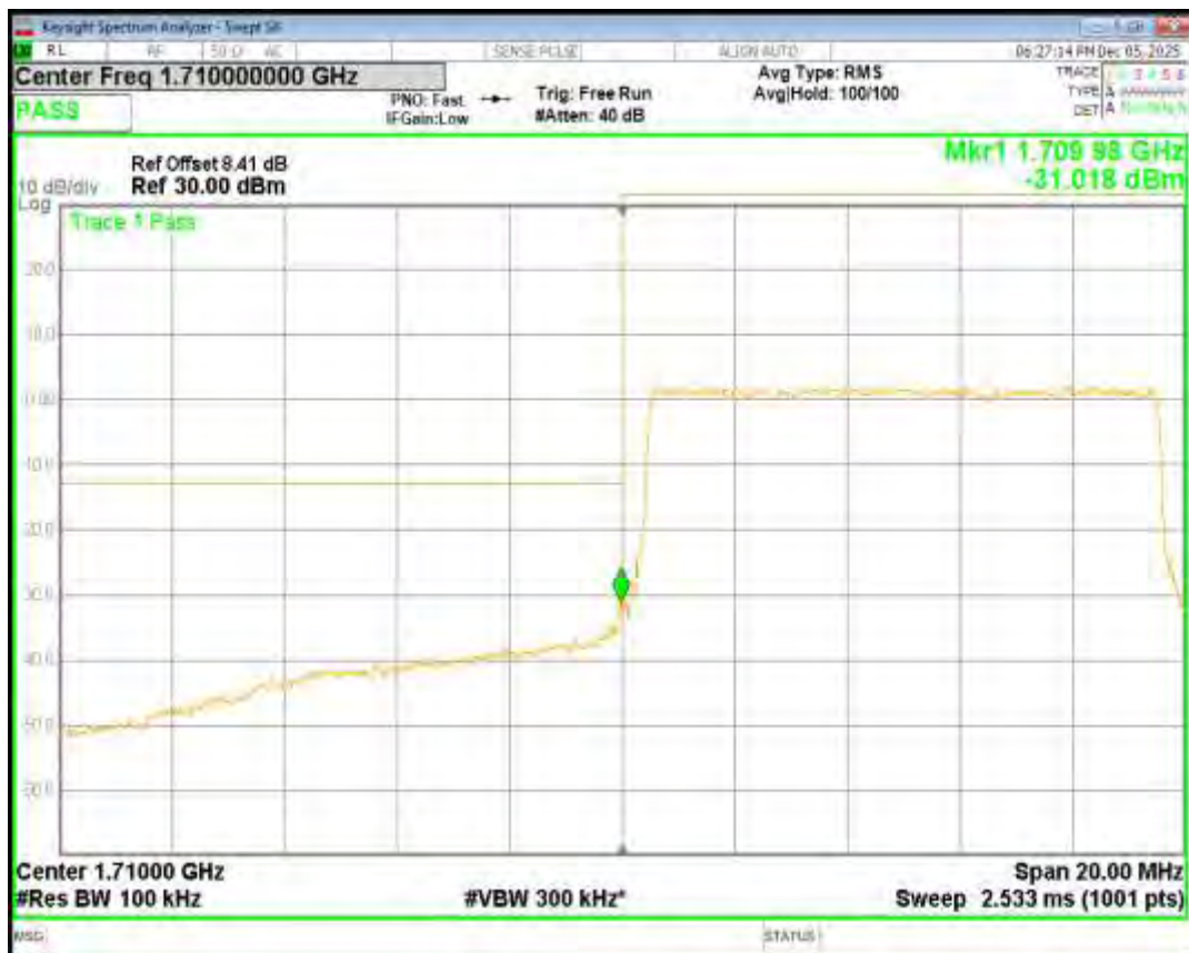
Band66 16QAM BW=10MHz Channel=132622 RB Size=50 Position=#0
