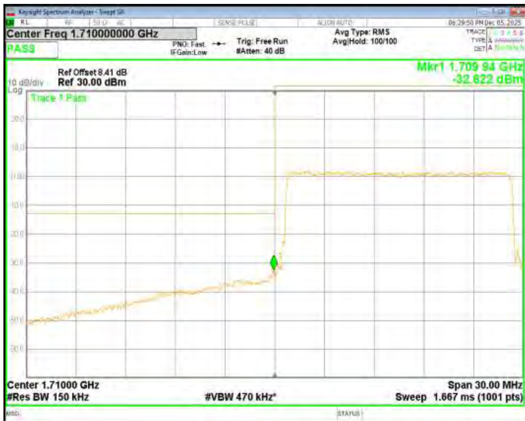
Band66 16QAM BW=15MHz Channel=132597 RB Size=75 Position=#0
