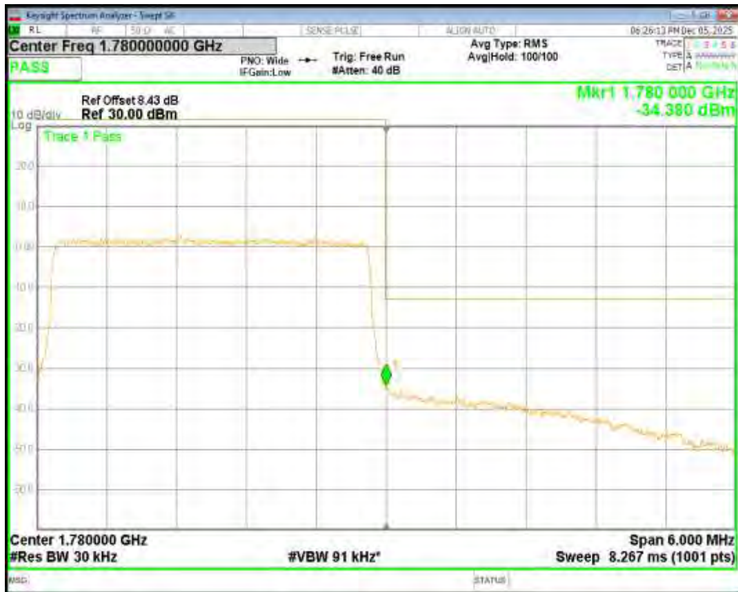
Band66 16QAM BW=5MHz Channel=131997 RB Size=25 Position=#0
