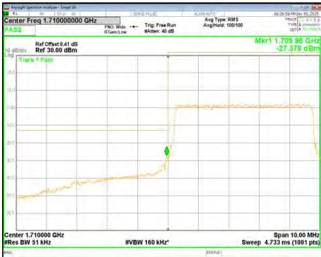
Band66 16QAM BW=5MHz Channel=132647 RB Size=25 Position=#0
