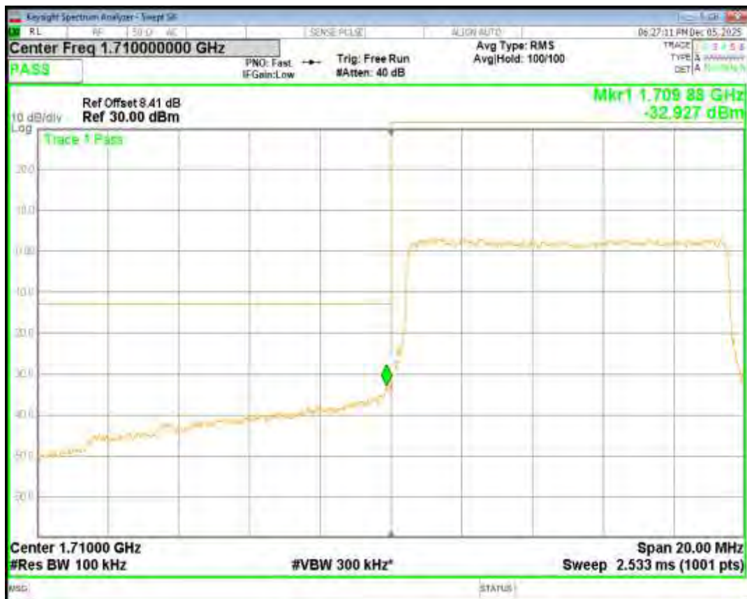
Band66 QPSK BW=10MHz Channel=132622 RB Size=50 Position=#0
