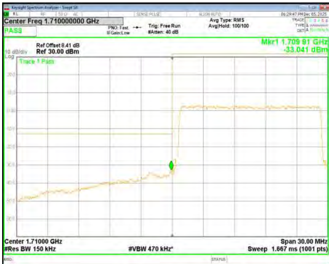
Band66 QPSK BW=15MHz Channel=132597 RB Size=75 Position=#0
