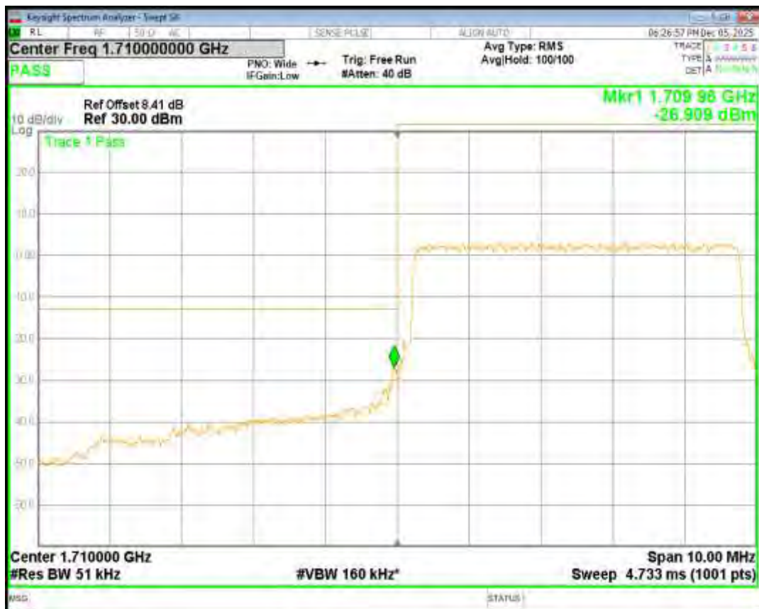
Band66 QPSK BW=5MHz Channel=132647 RB Size=25 Position=#0
