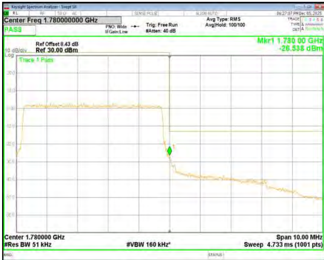
Band66 QPSK BW=1.4MHz Channel=131979 RB Size=6 Position=#0
