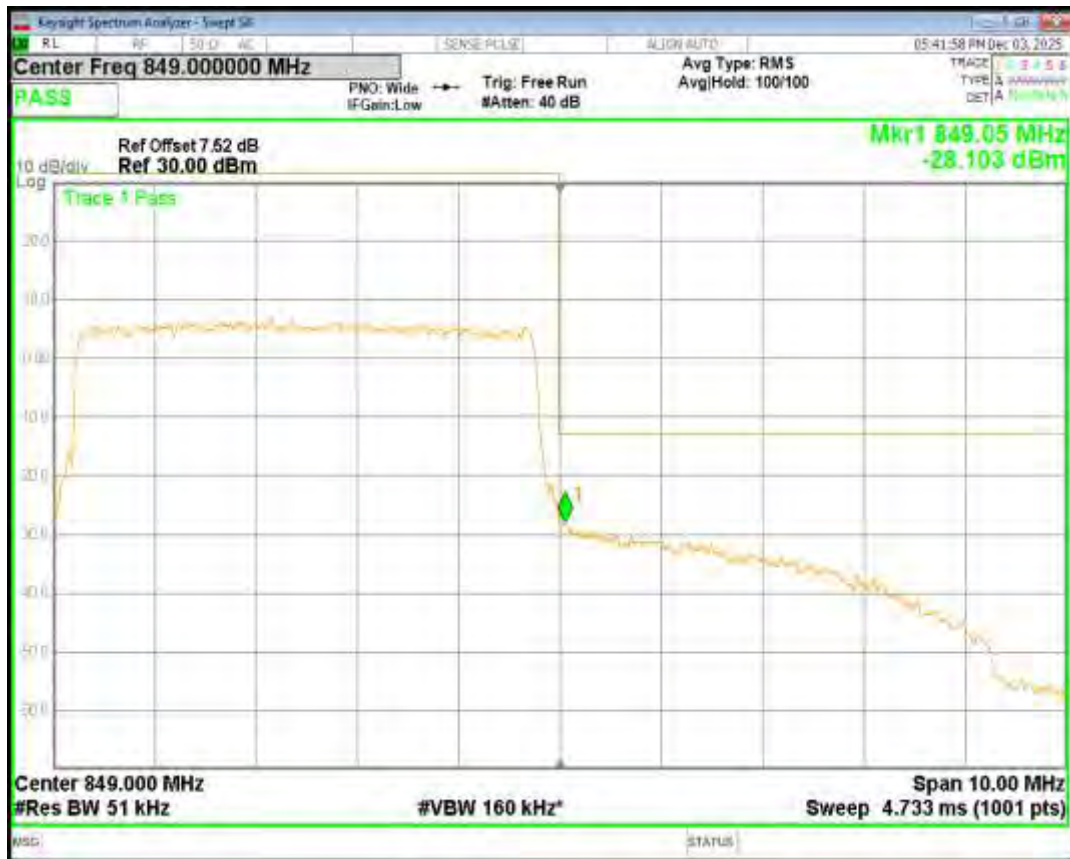
Band66 16QAM BW=1.4MHz Channel=131979 RB Size=6 Position=#0
