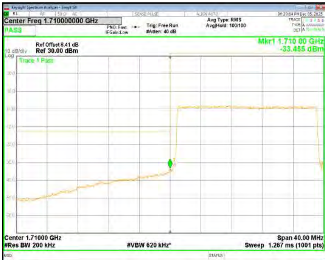
Band66 16QAM BW=20MHz Channel=132572 RB Size=100 Position=#0
