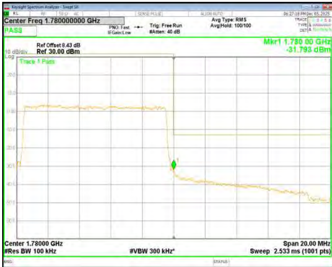
Band66 QPSK BW=15MHz Channel=132047 RB Size=75 Position=#0
