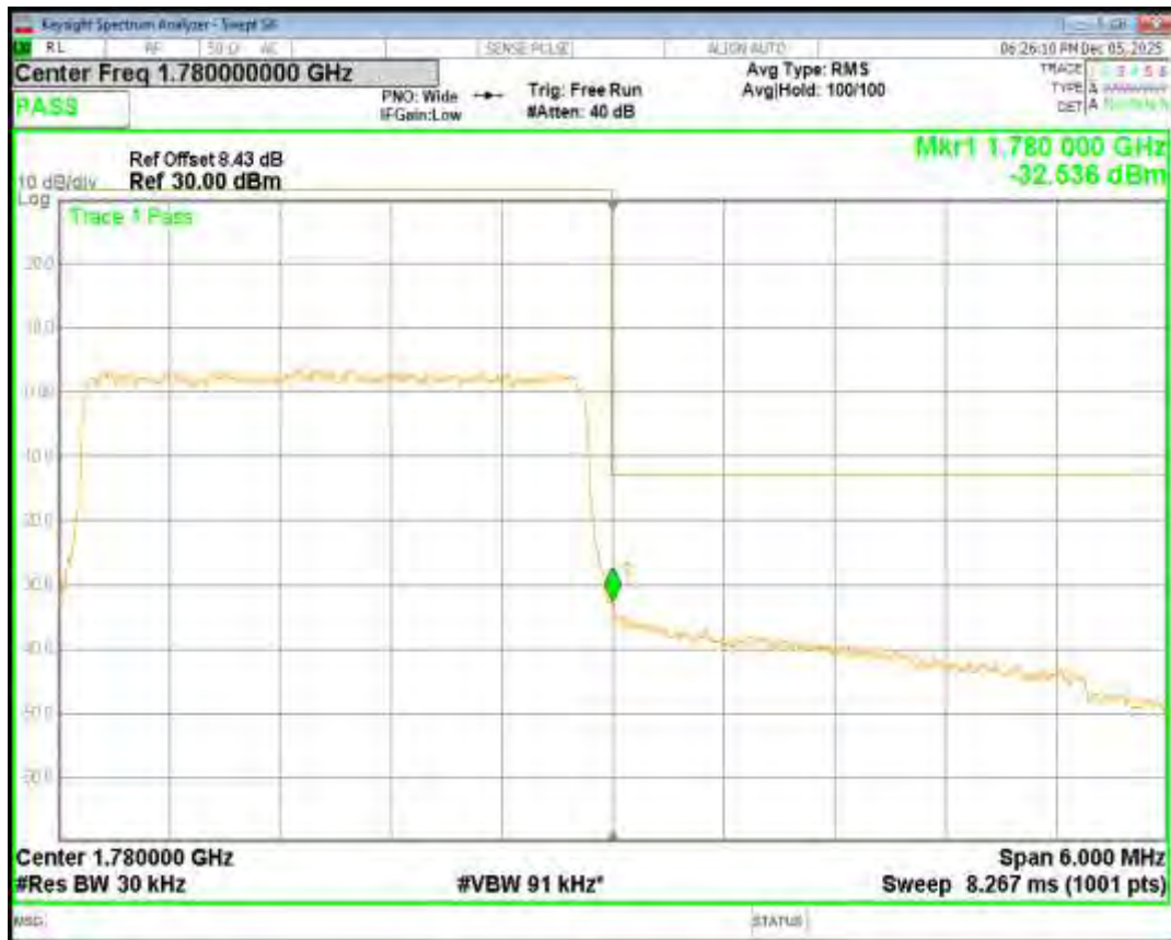
Band66 QPSK BW=5MHz Channel=131997 RB Size=25 Position=#0
