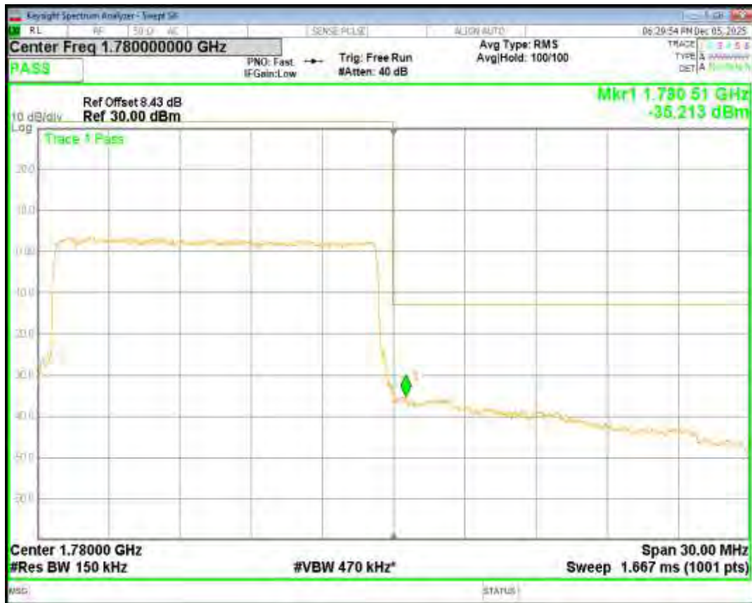
Band66 QPSK BW=20MHz Channel=132072 RB Size=100 Position=#0
