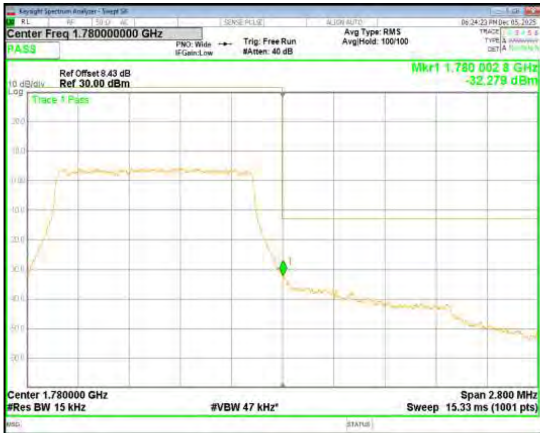
Band66 QPSK BW=10MHz Channel=132022 RB Size=50 Position=#0
