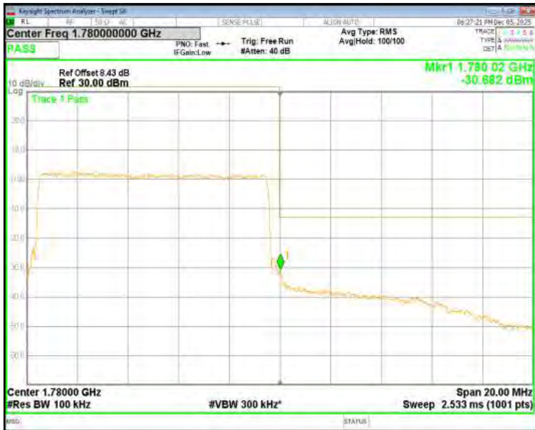
Band66 16QAM BW=15MHz Channel=132047 RB Size=75 Position=#0
