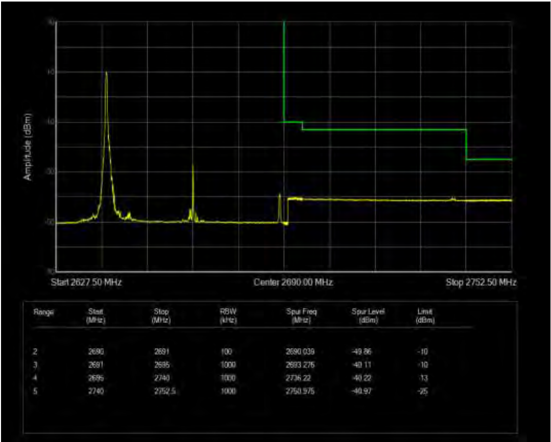
n41 SCS=30kHz CP QPSK BW=50MHz Channel=532998 RB=1@132
