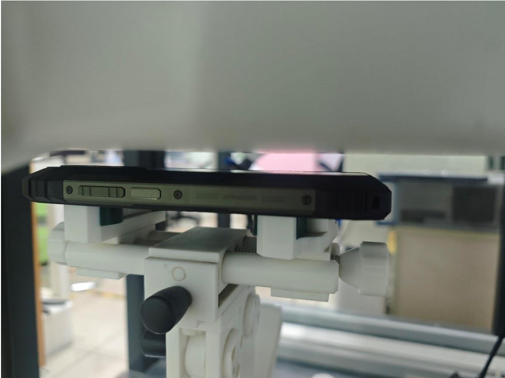
Body Back side(separation distance is 10mm)
