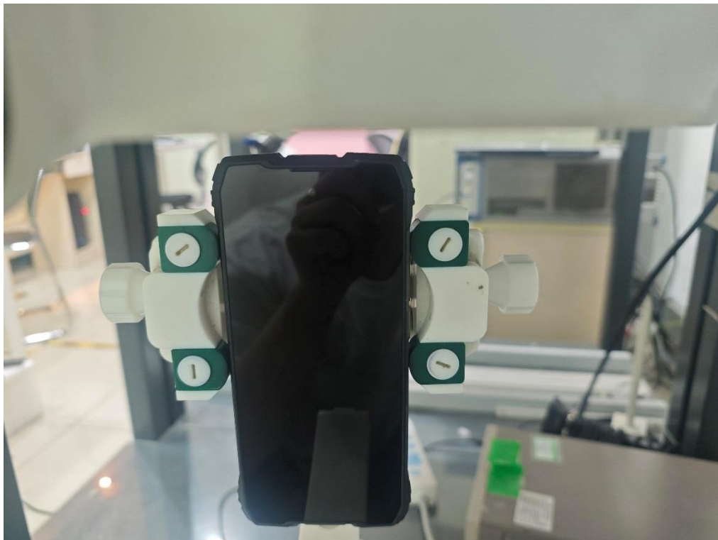
Body Top side(separation distance is 10mm)
