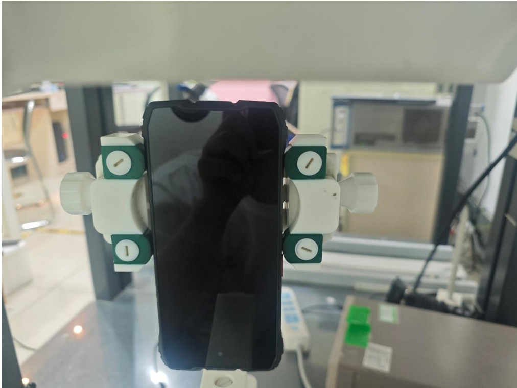
Body Bottom side(separation distance is 10mm)
