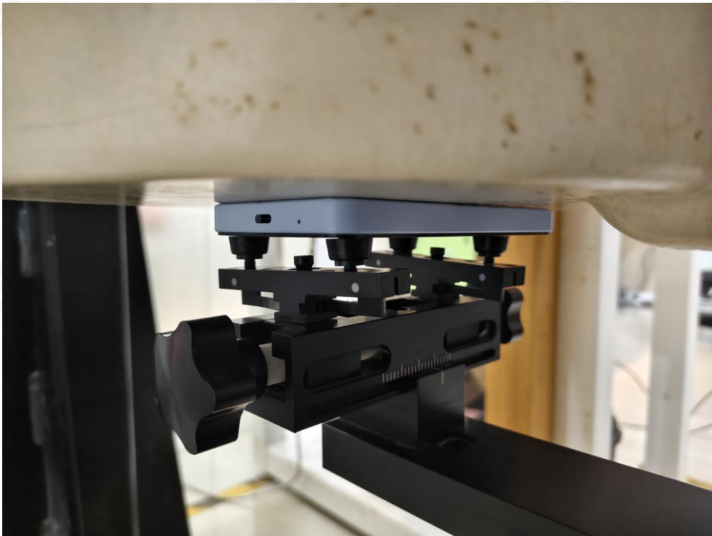
Limbs Back side(separation distance is 0mm)
