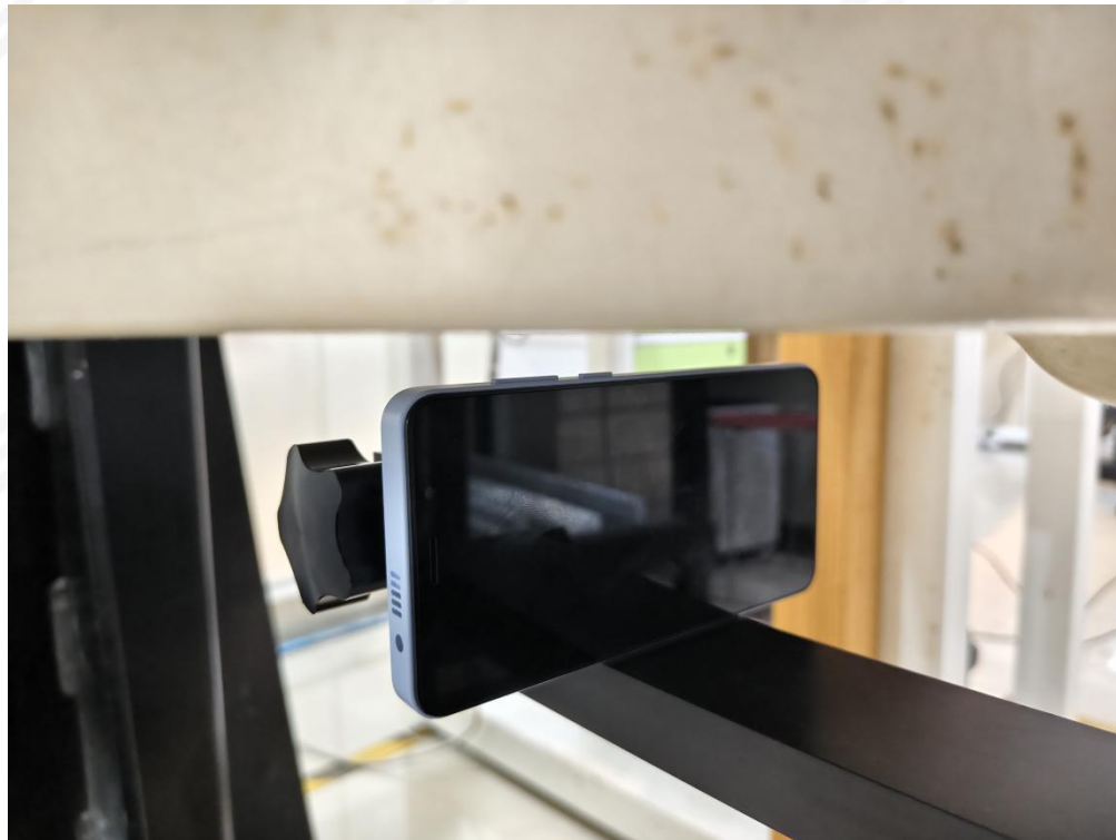
Body Right side(separation distance is 10mm)
