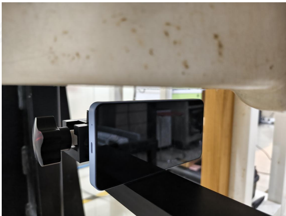
Body Left side(separation distance is 10mm)
