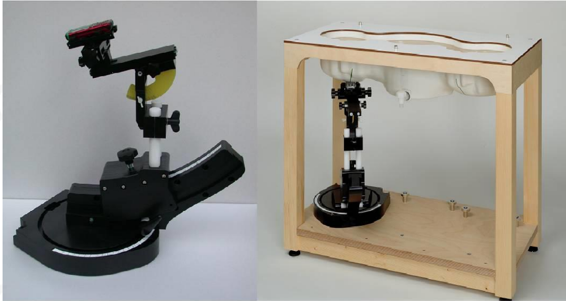
Device holder supplied by SPEAG
