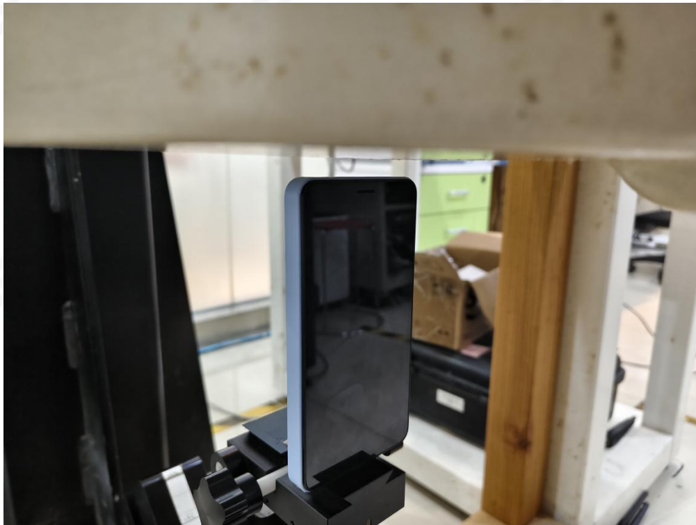
Body Top side(separation distance is 10mm)
