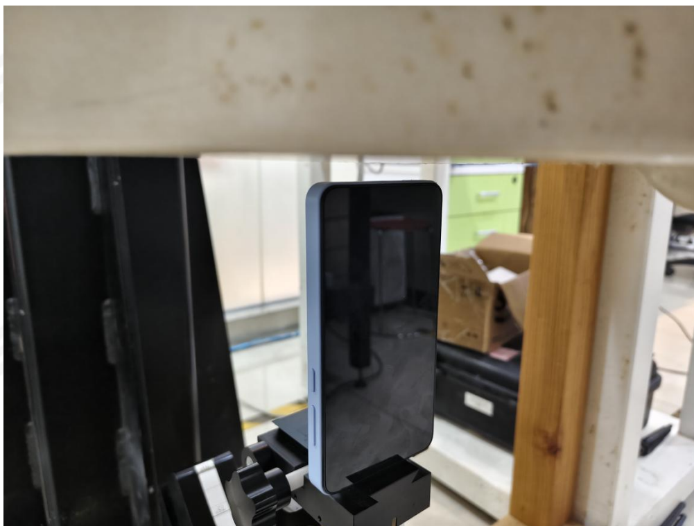
Body Bottom side(separation distance is 10mm)
