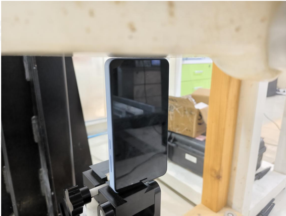
Limbs Bottom side(separation distance is 0mm)
