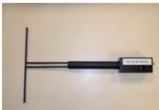
Figure 1 – MVG COMOSAR Validation Dipole
