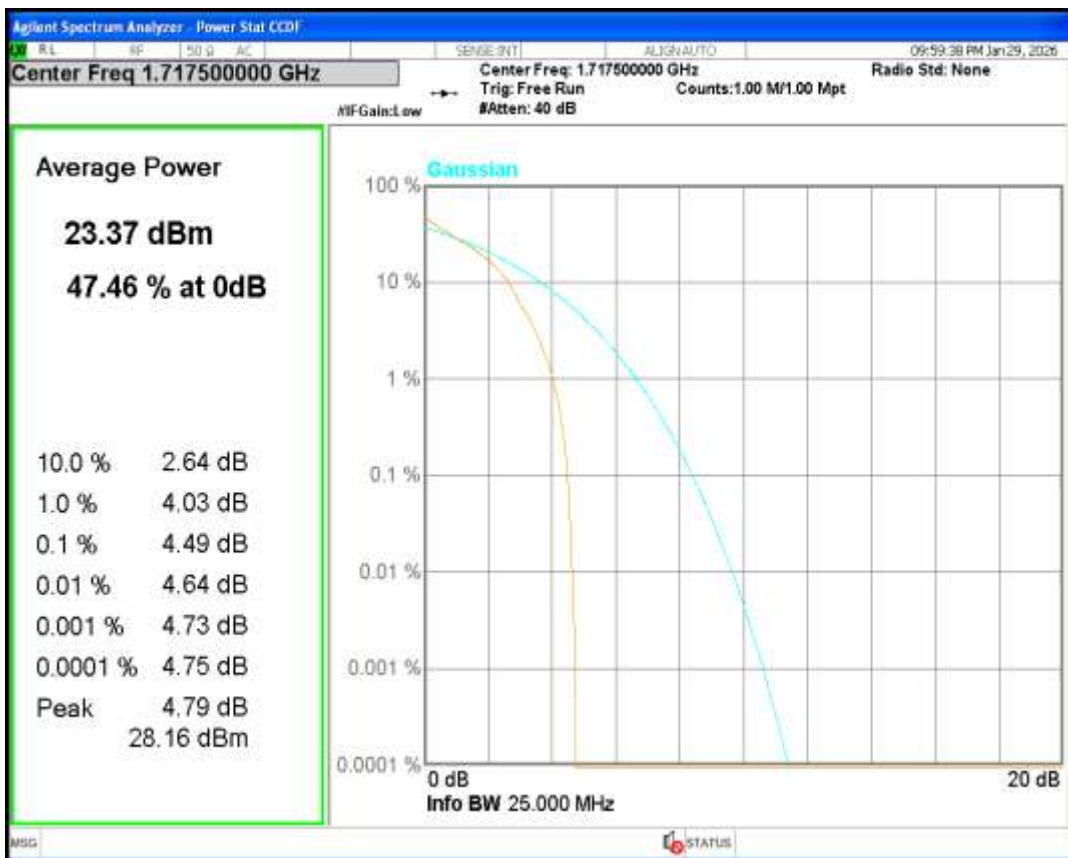
Band4 QPSK BW=20MHz Channel=20050 RB Size=1 Position=#0
