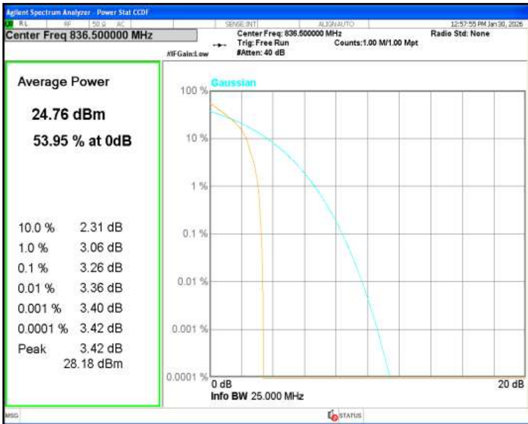
Band5 QPSK BW=3MHz Channel=20635 RB Size=1 Position=#0
