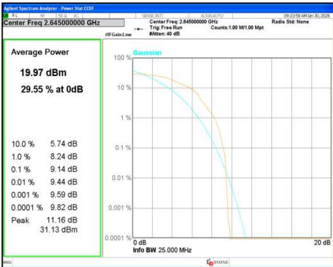
Band41(2555-2655) 16QAM BW=5MHz Channel=40265 RB Size=1 Position=#0
