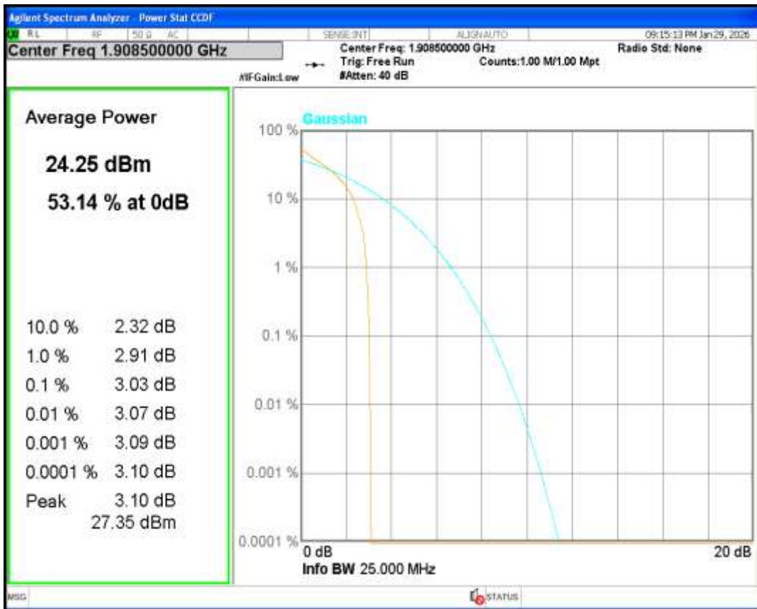
Band2 QPSK BW=5MHz Channel=18625 RB Size=1 Position=#0
