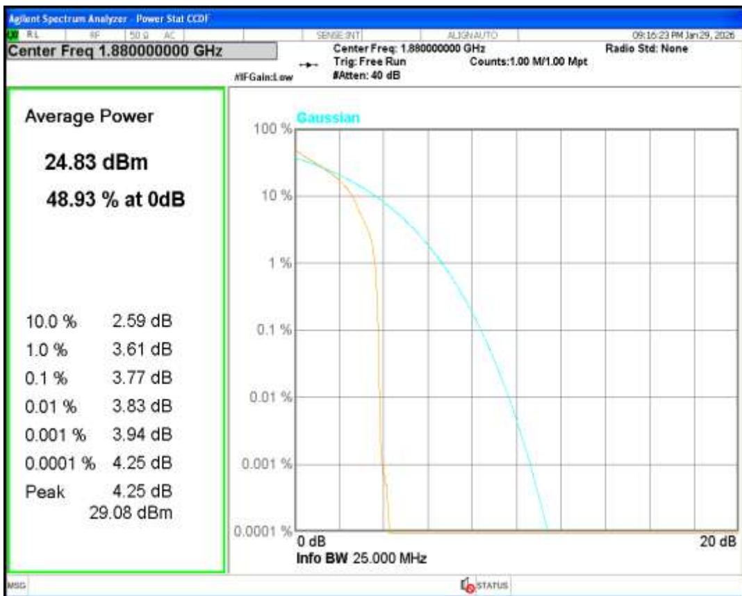
Band2 QPSK BW=20MHz Channel=19100 RB Size=1 Position=#0
