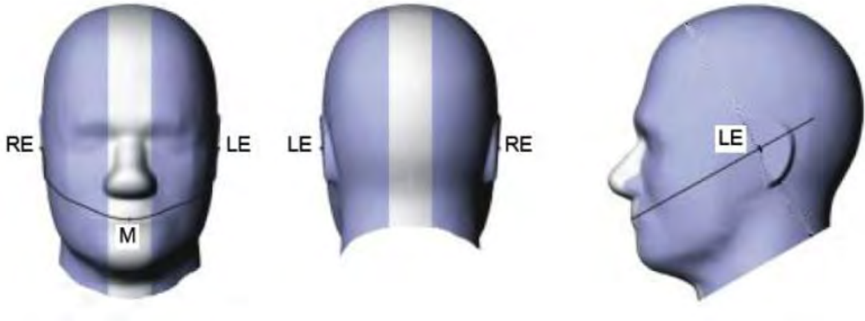
Fig 7.1.1 Front, back, and side views of SAM phantom
