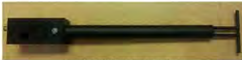
Figure 1 – MVG COMOSAR Validation Dipole
