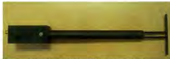
Figure 1 – MVG COMOSAR Validation Dipole
