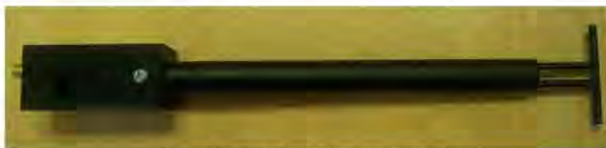
Figure 1 – MVG COMOSAR Validation Dipole
