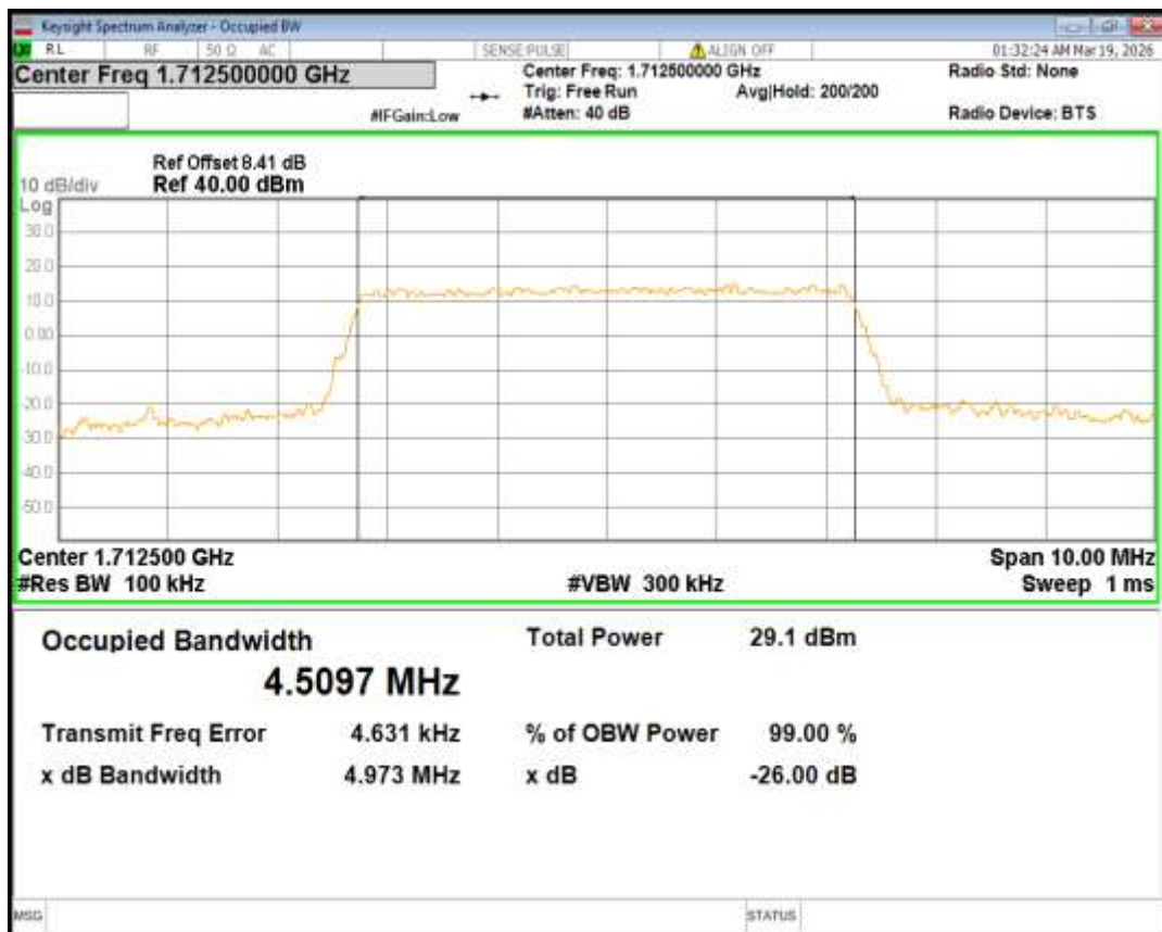
Band66 QPSK BW=5MHz Channel=132322 RB Size=25 Position=#0
