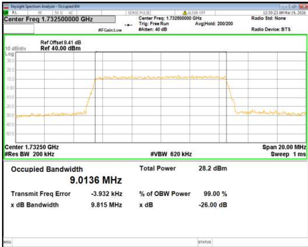
Band4 16QAM BW=10MHz Channel=20350 RB Size=50 Position=#0
