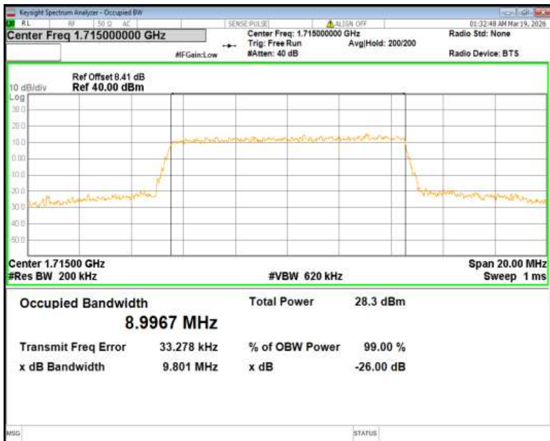
Band66 16QAM BW=10MHz Channel=132322 RB Size=50 Position=#0
