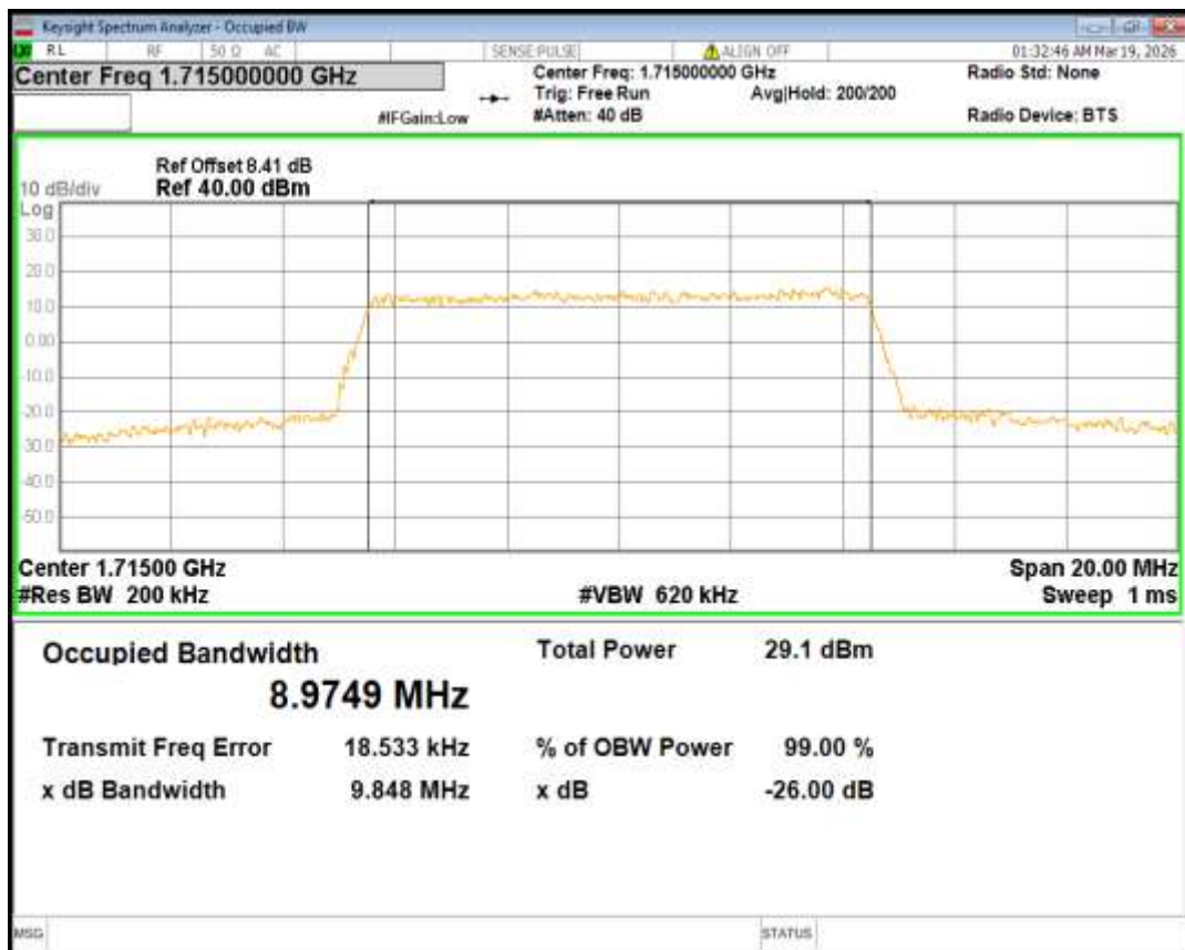
Band66 QPSK BW=10MHz Channel=132322 RB Size=50 Position=#0
