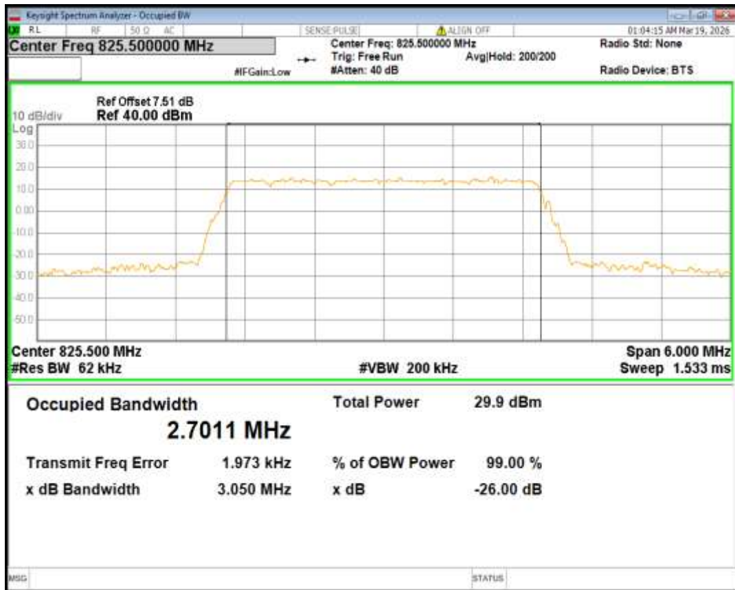
Band5 16QAM BW=3MHz Channel=20525 RB Size=15 Position=#0
