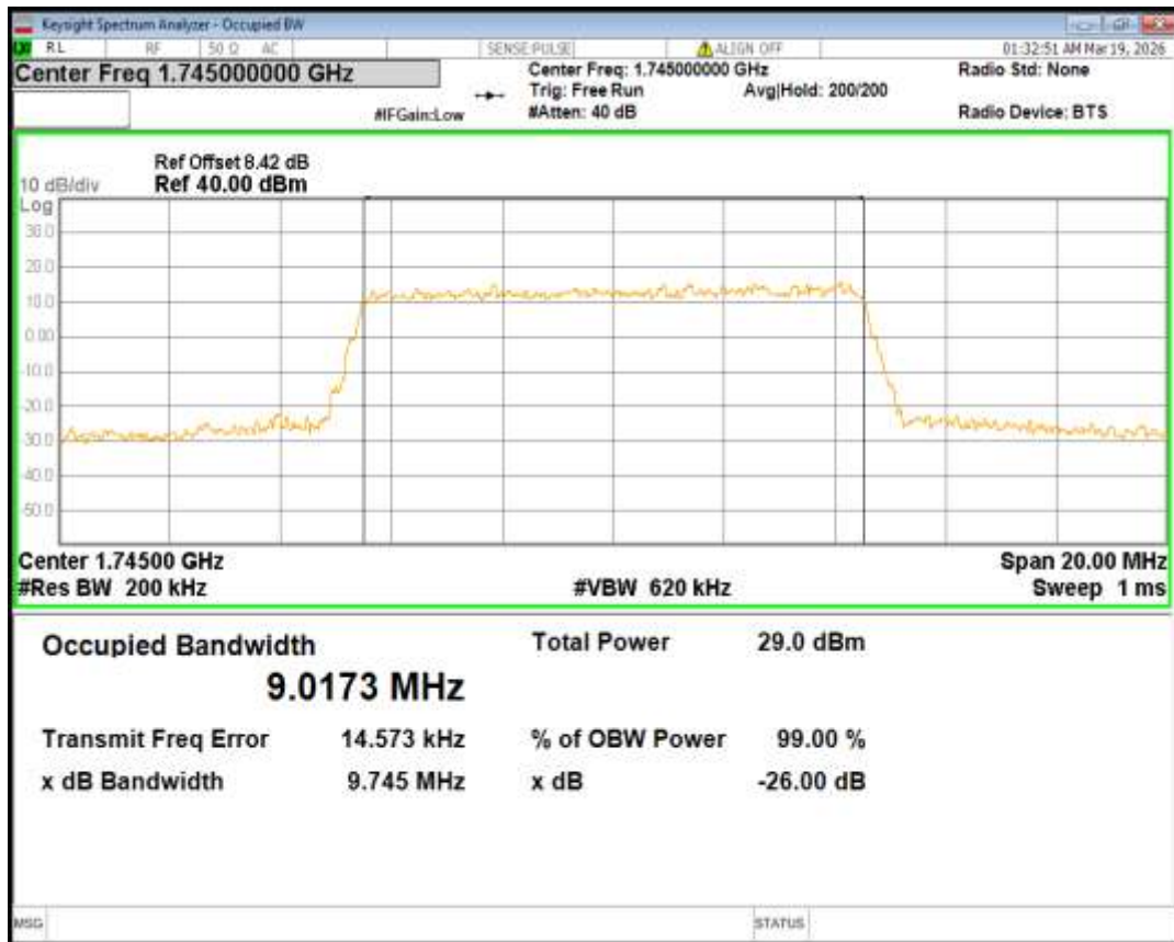
Band66 QPSK BW=10MHz Channel=132622 RB Size=50 Position=#0
