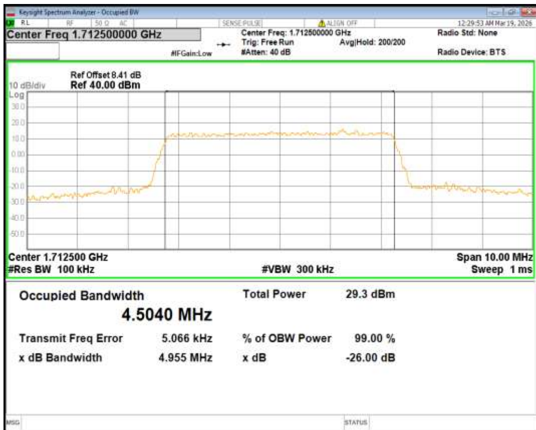
Band4 QPSK BW=5MHz Channel=20175 RB Size=25 Position=#0
