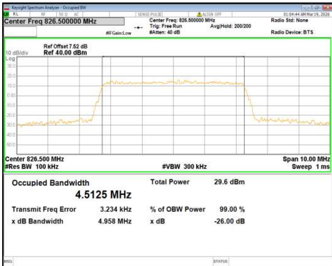
Band5 16QAM BW=5MHz Channel=20525 RB Size=25 Position=#0
