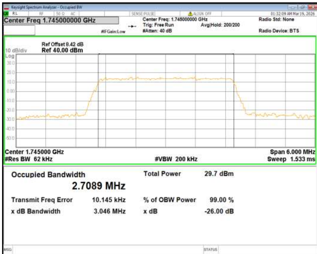
Band66 QPSK BW=3MHz Channel=132657 RB Size=15 Position=#0
