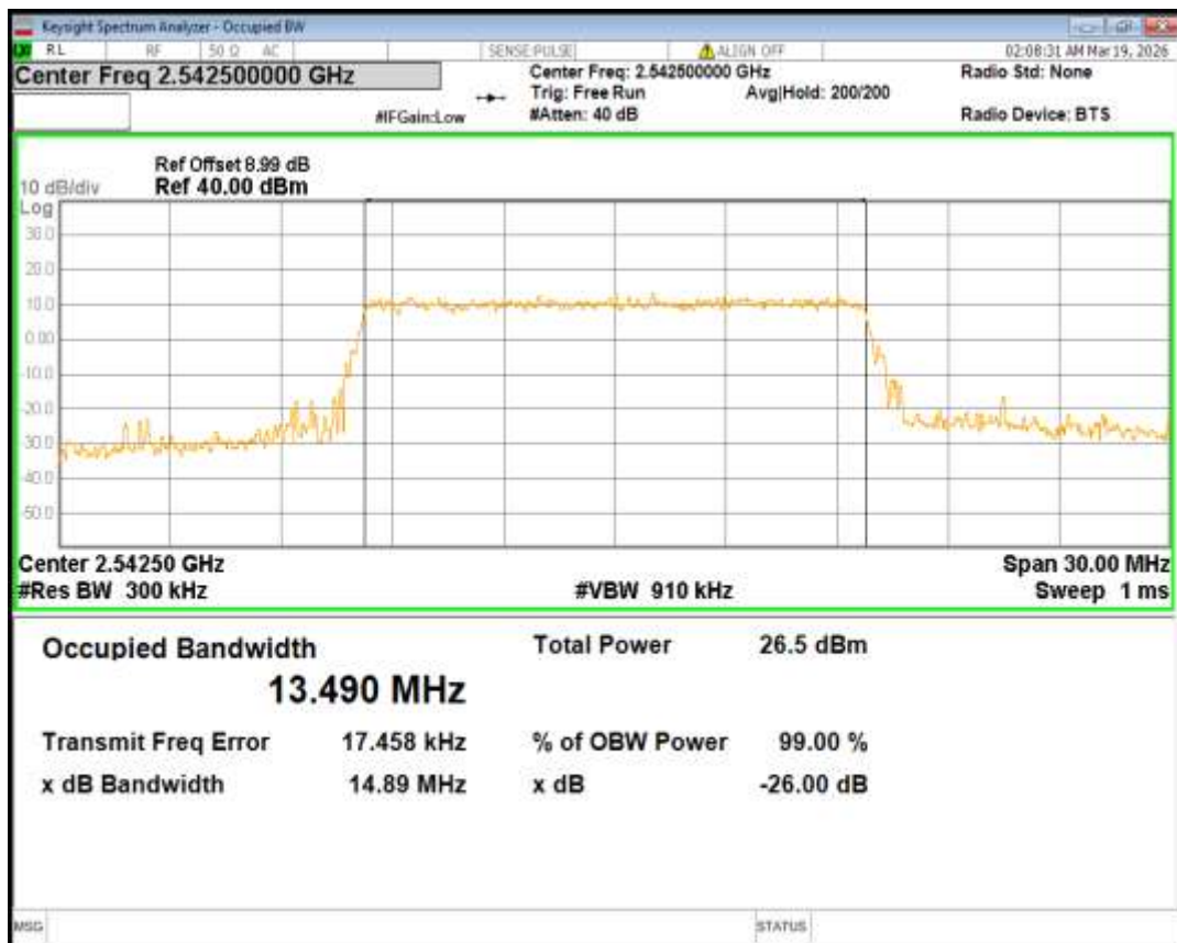
Band41(2535-2655) 16QAM BW=15MHz Channel=40640 RB Size=75 Position=#0
