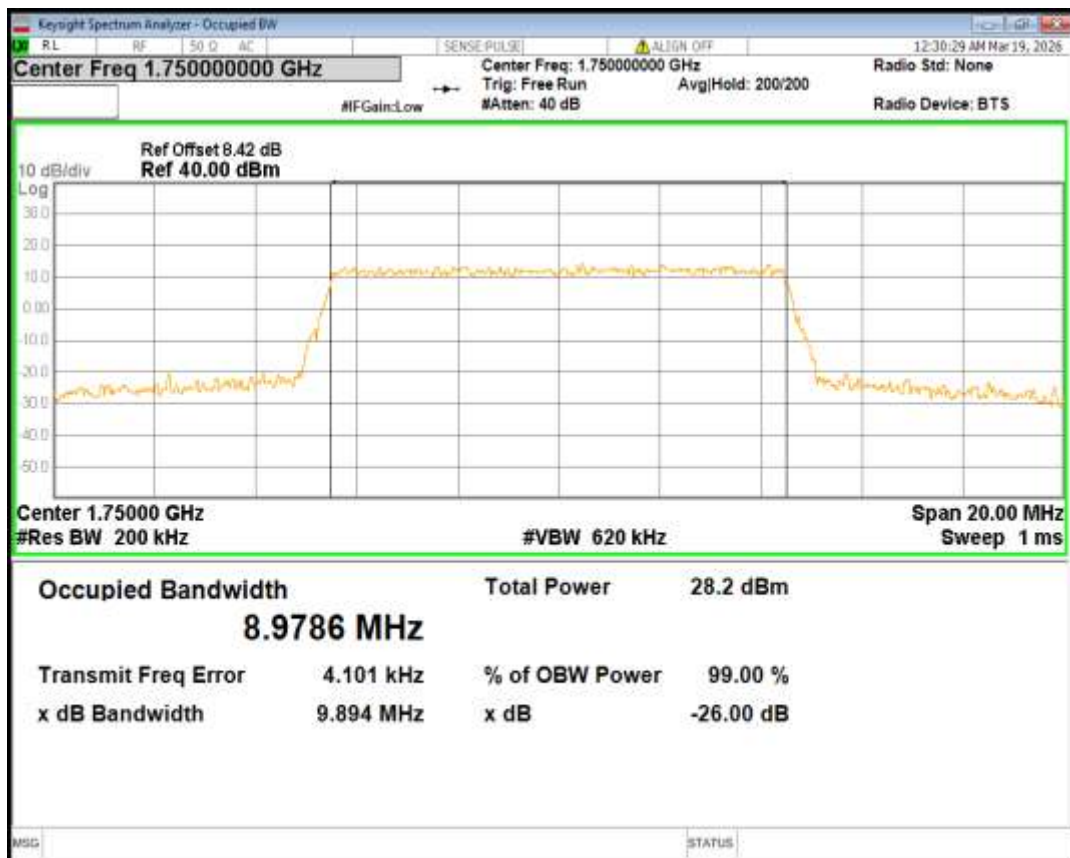
Band4 16QAM BW=15MHz Channel=20025 RB Size=75 Position=#0
