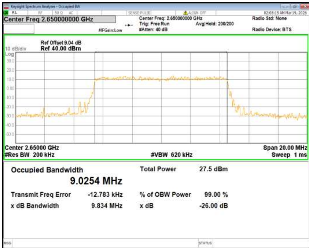
Band41(2535-2655) QPSK BW=15MHz Channel=40115 RB Size=75 Position=#0
