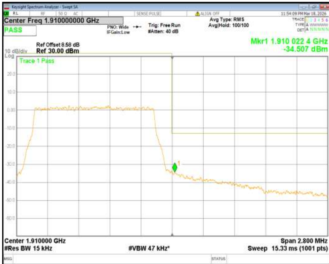
Band2 16QAM BW=10MHz Channel=18650 RB Size=50 Position=#0
