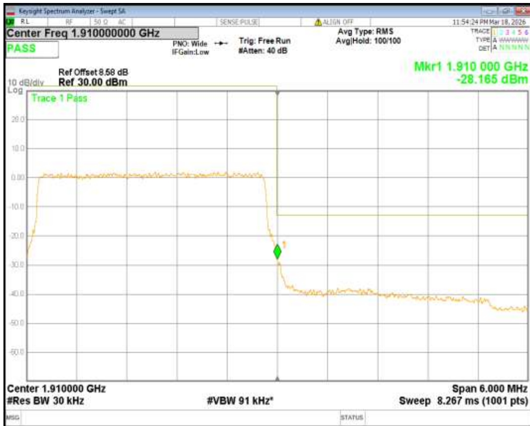
Band2 QPSK BW=5MHz Channel=18625 RB Size=25 Position=#0
