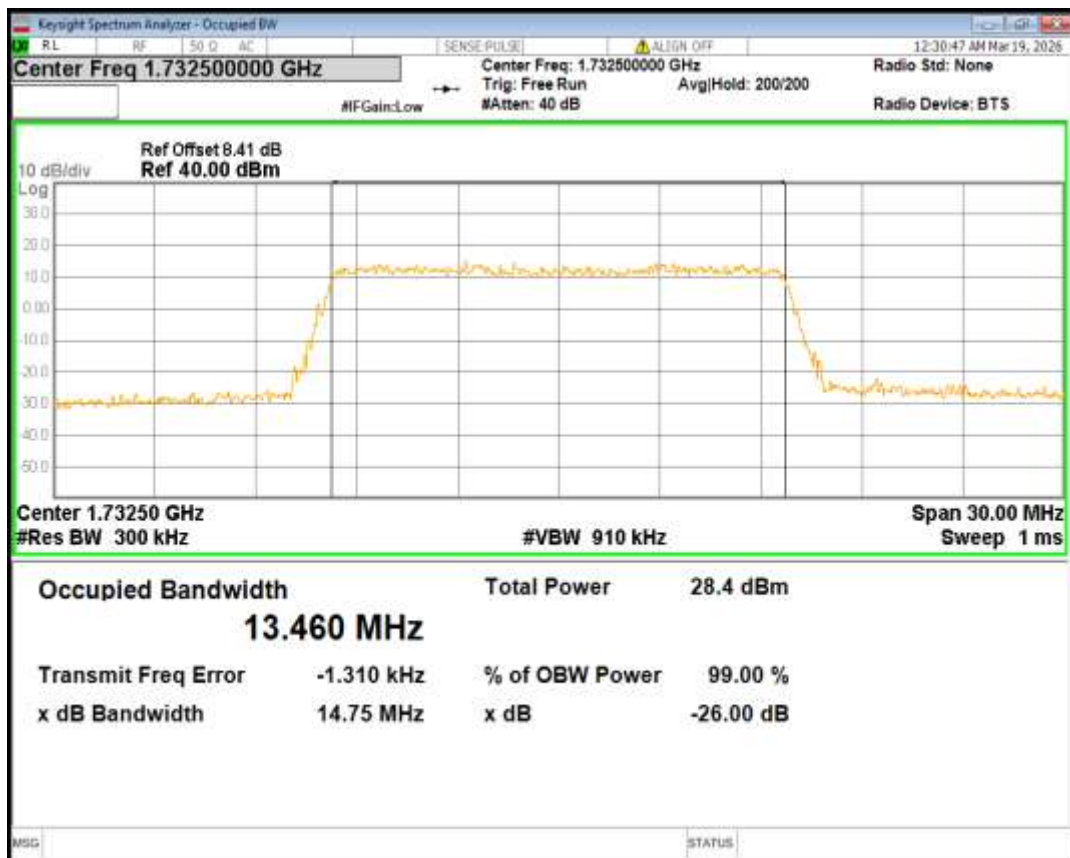
Band4 16QAM BW=15MHz Channel=20325 RB Size=75 Position=#0
