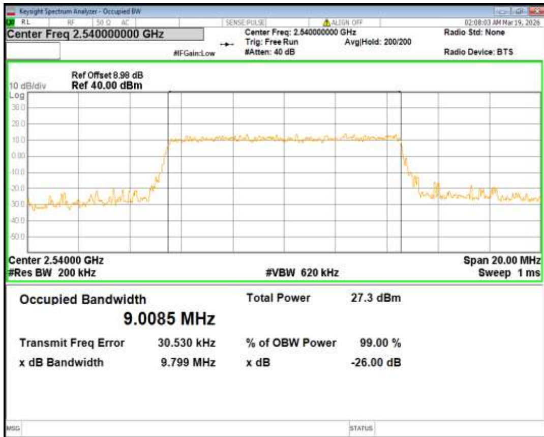
Band41(2535-2655) QPSK BW=10MHz Channel=40640 RB Size=50 Position=#0
