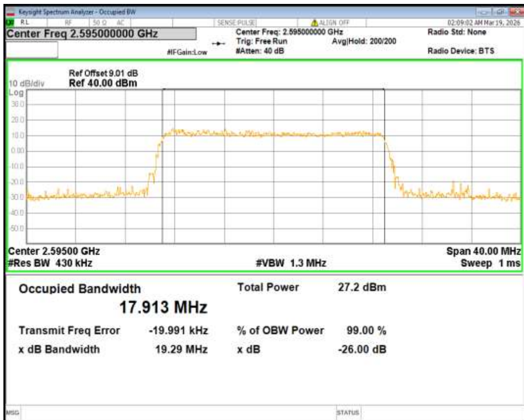
Band41(2535-2655) 16QAM BW=20MHz Channel=41140 RB Size=100 Position=#0
