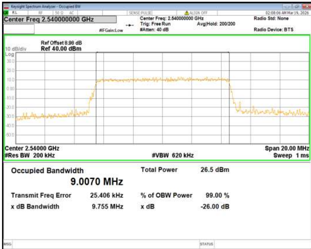
Band41(2535-2655) 16QAM BW=10MHz Channel=40640 RB Size=50 Position=#0
