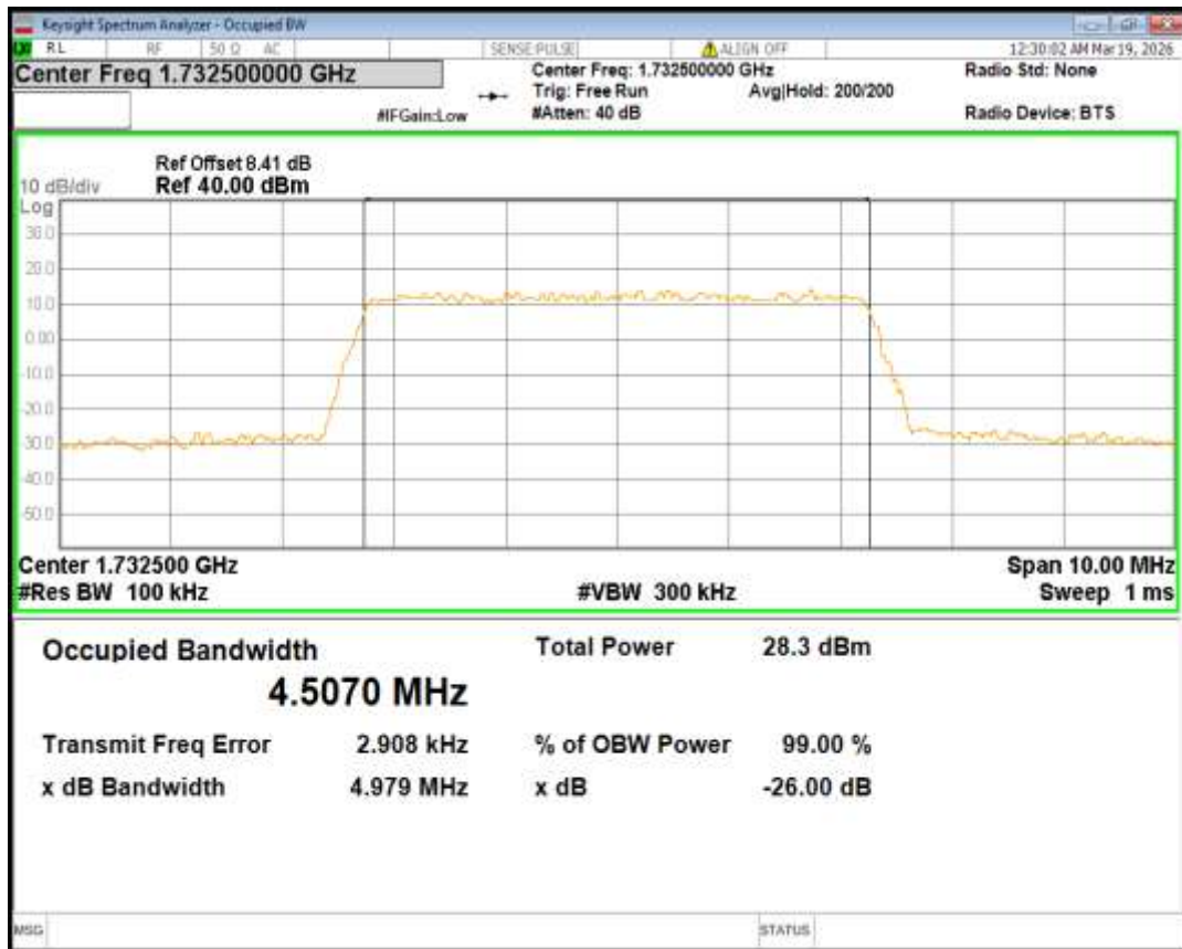
Band4 16QAM BW=5MHz Channel=20375 RB Size=25 Position=#0
