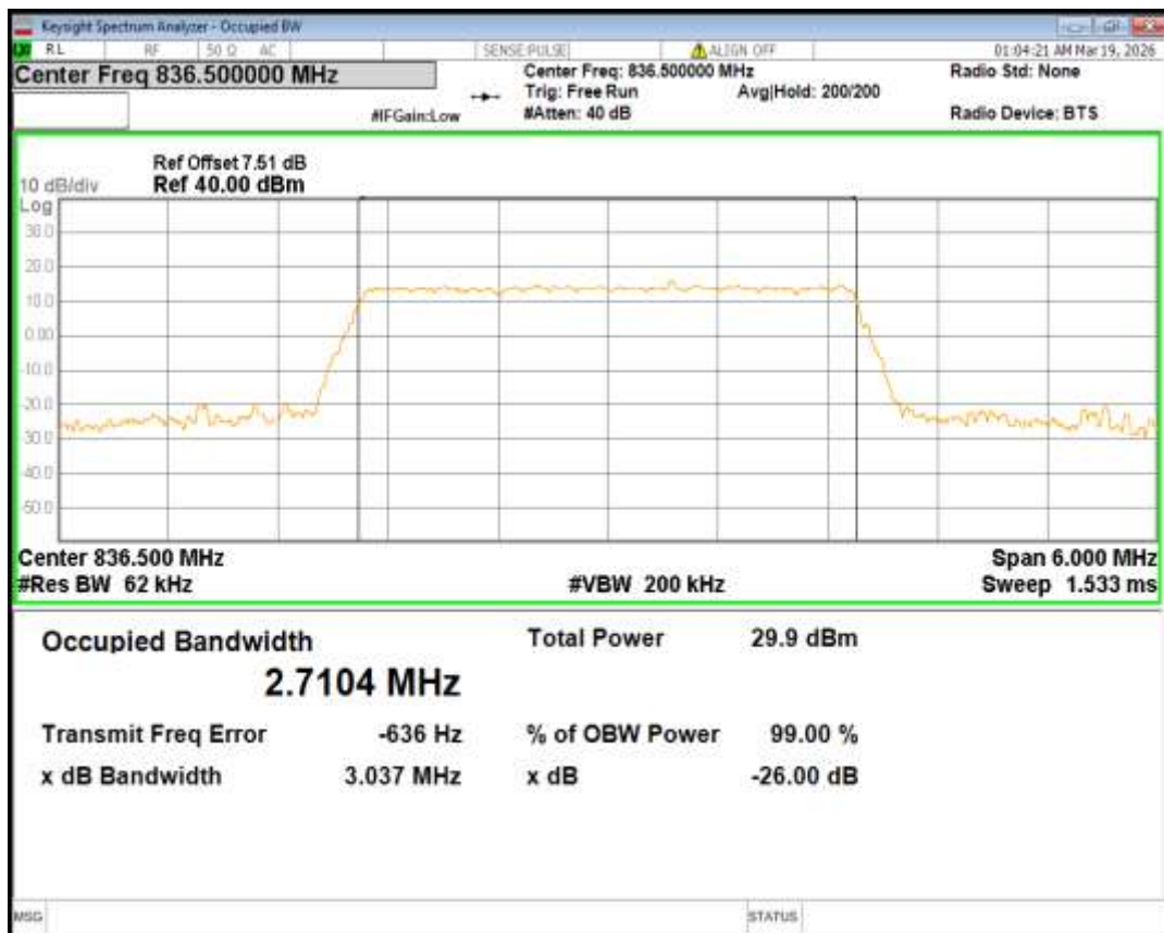
Band5 16QAM BW=3MHz Channel=20635 RB Size=15 Position=#0
