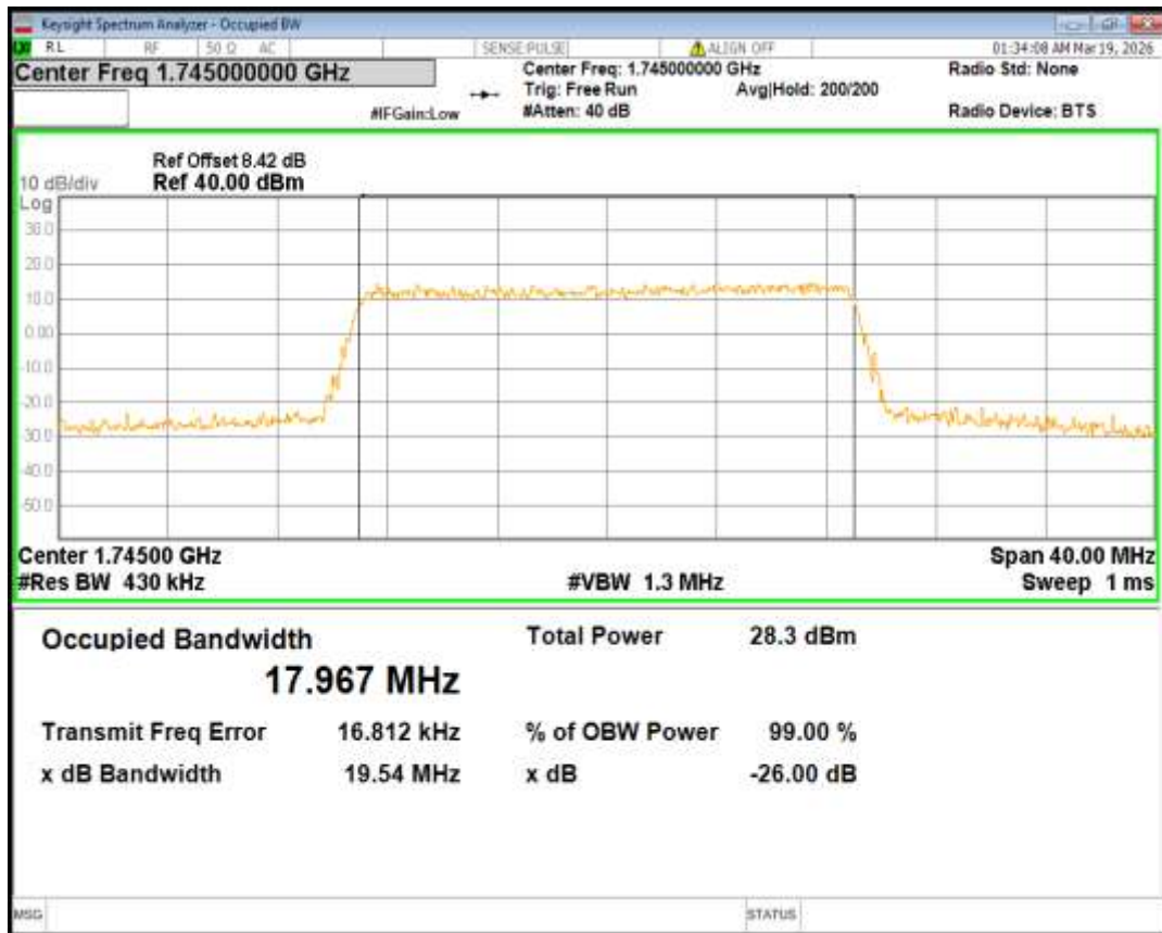
Band66 16QAM BW=20MHz Channel=132572 RB Size=100 Position=#0
