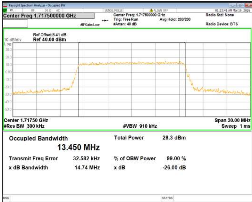
Band66 16QAM BW=15MHz Channel=132322 RB Size=75 Position=#0
