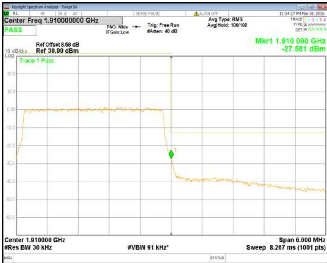
Band2 16QAM BW=5MHz Channel=18625 RB Size=25 Position=#0
