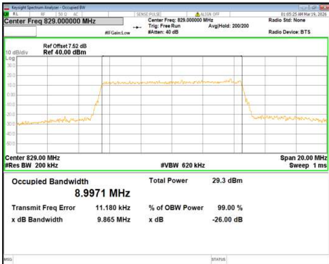
Band5 16QAM BW=10MHz Channel=20525 RB Size=50 Position=#0
