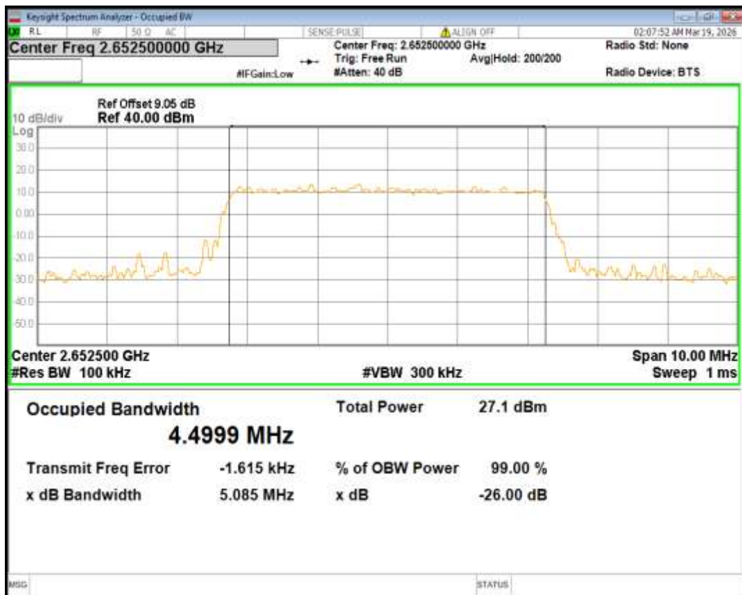
Band41(2535-2655) QPSK BW=10MHz Channel=40090 RB Size=50 Position=#0
