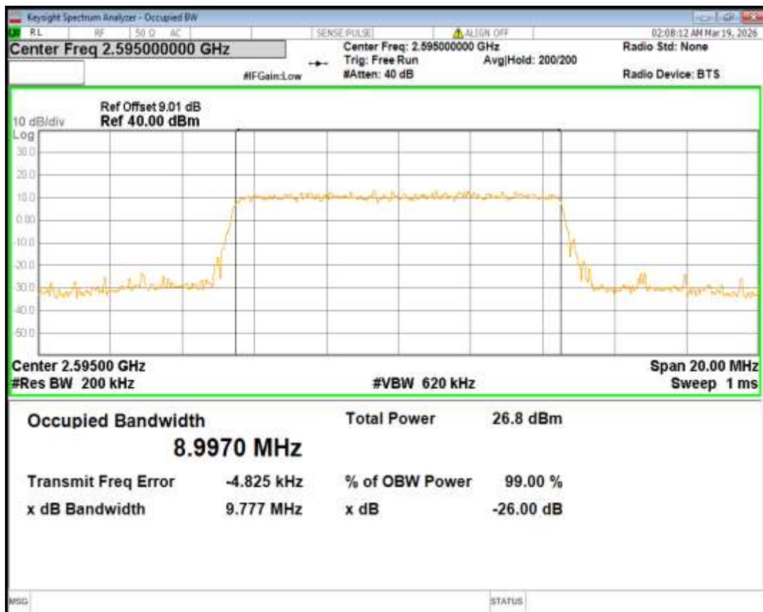
Band41(2535-2655) 16QAM BW=10MHz Channel=41190 RB Size=50 Position=#0
