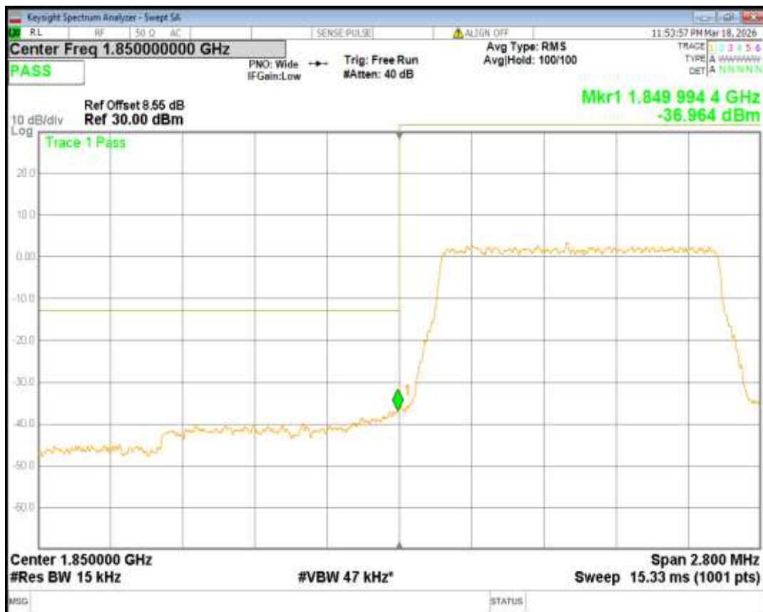
Band2 QPSK BW=1.4MHz Channel=19193 RB Size=6 Position=#0
