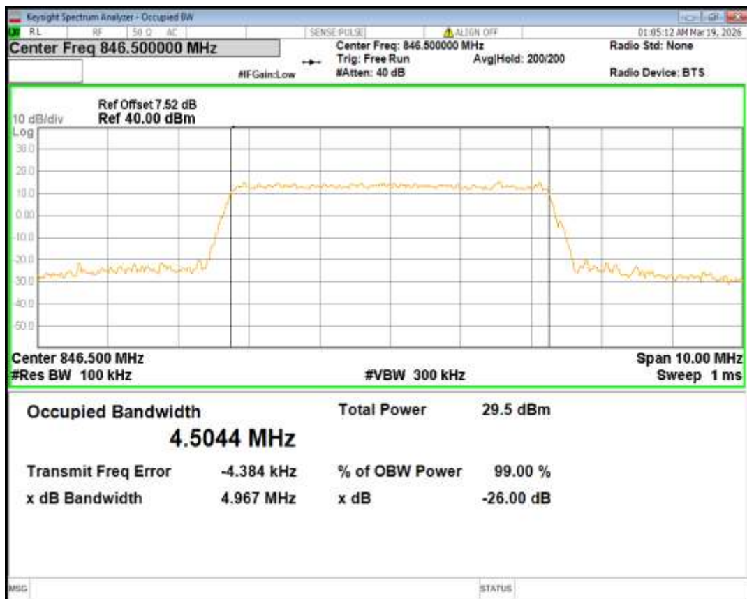
Band5 QPSK BW=1.4MHz Channel=20407 RB Size=6 Position=#0
