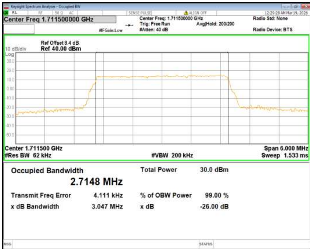
Band4 QPSK BW=3MHz Channel=20175 RB Size=15 Position=#0
