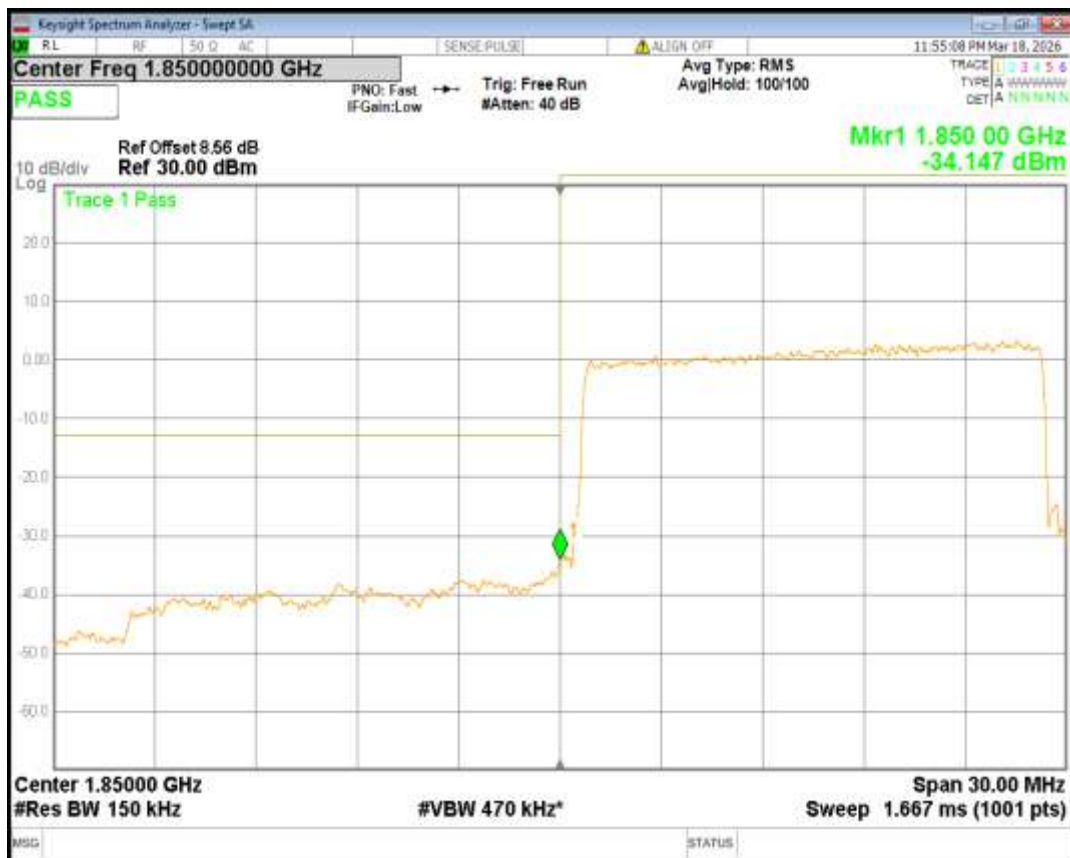
Band2 QPSK BW=15MHz Channel=19125 RB Size=75 Position=#0
