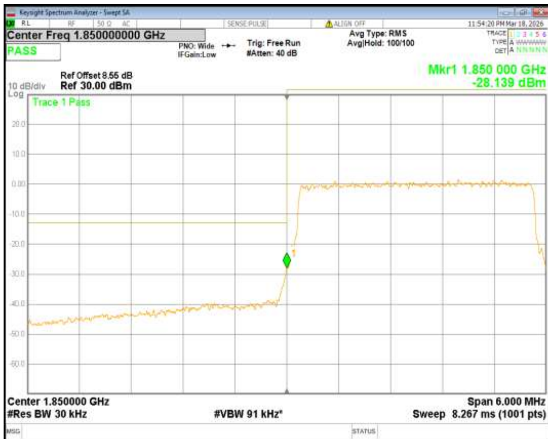
Band2 16QAM BW=3MHz Channel=19185 RB Size=15 Position=#0
