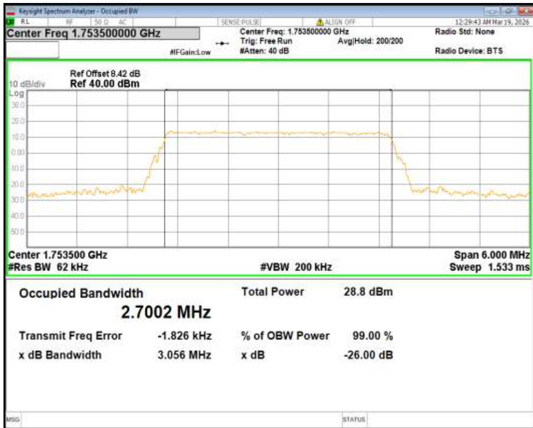
Band4 16QAM BW=5MHz Channel=19975 RB Size=25 Position=#0
