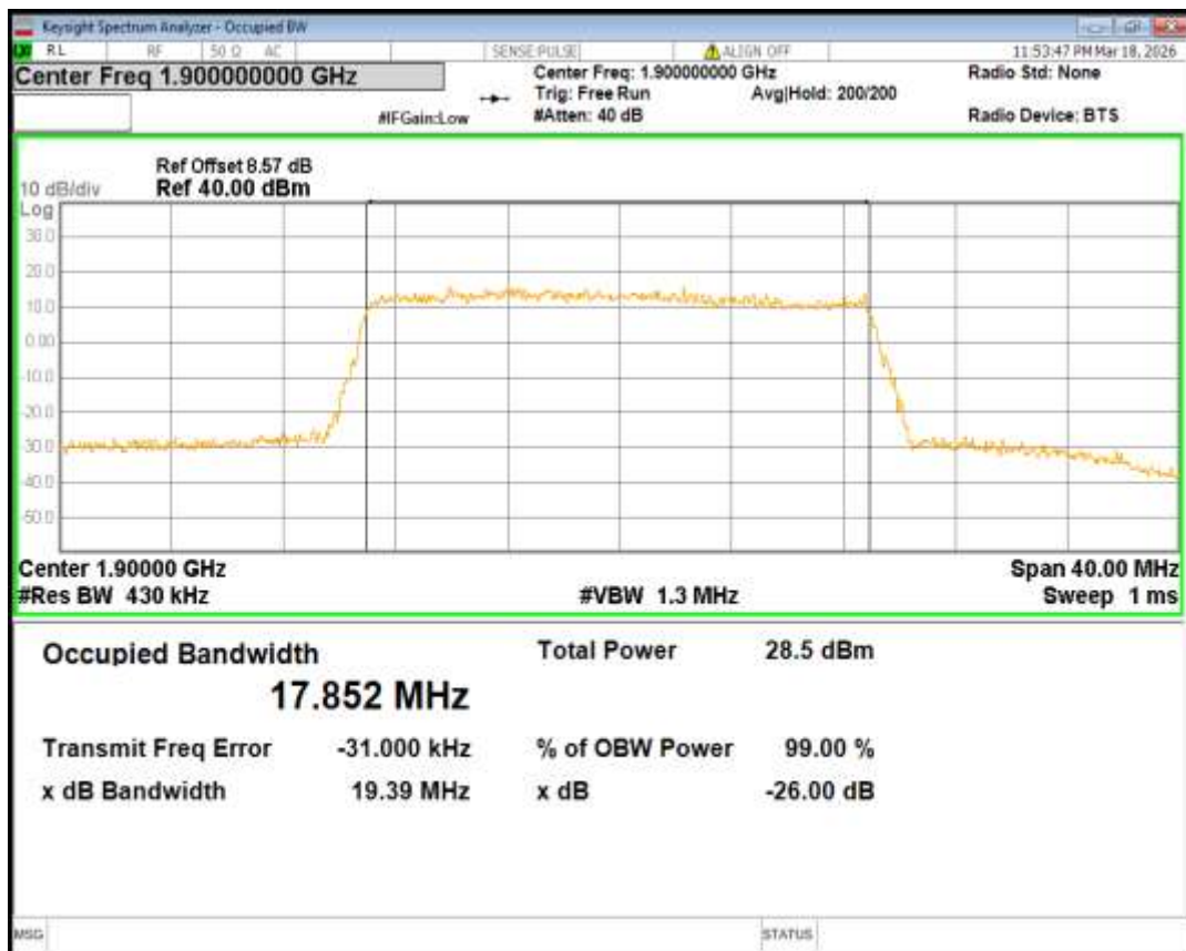
Band2 QPSK BW=3MHz Channel=18615 RB Size=15 Position=#0
