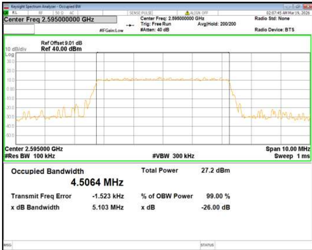
Band41(2535-2655) 16QAM BW=5MHz Channel=41215 RB Size=25 Position=#0
