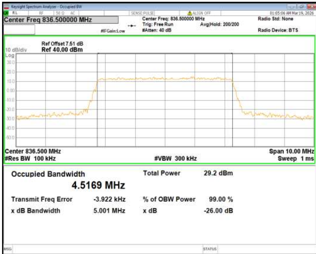
Band5 16QAM BW=5MHz Channel=20625 RB Size=25 Position=#0
