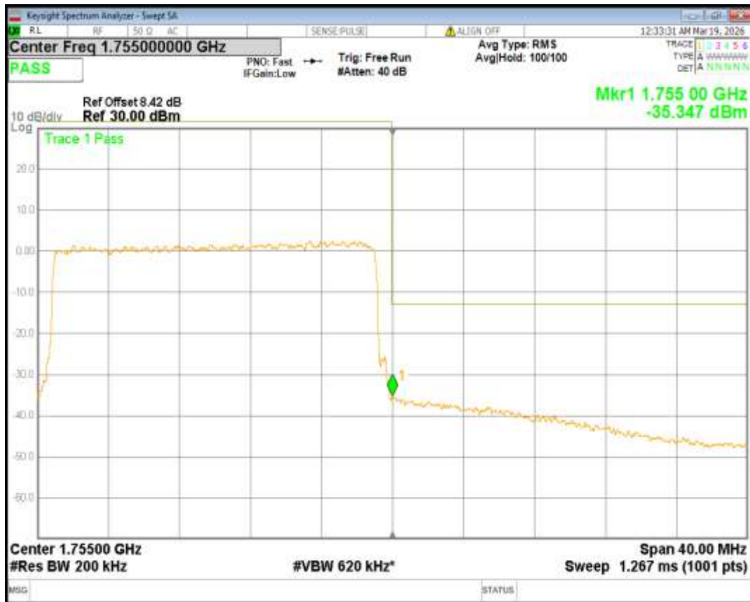
Band4 16QAM BW=3MHz Channel=19965 RB Size=15 Position=#0
