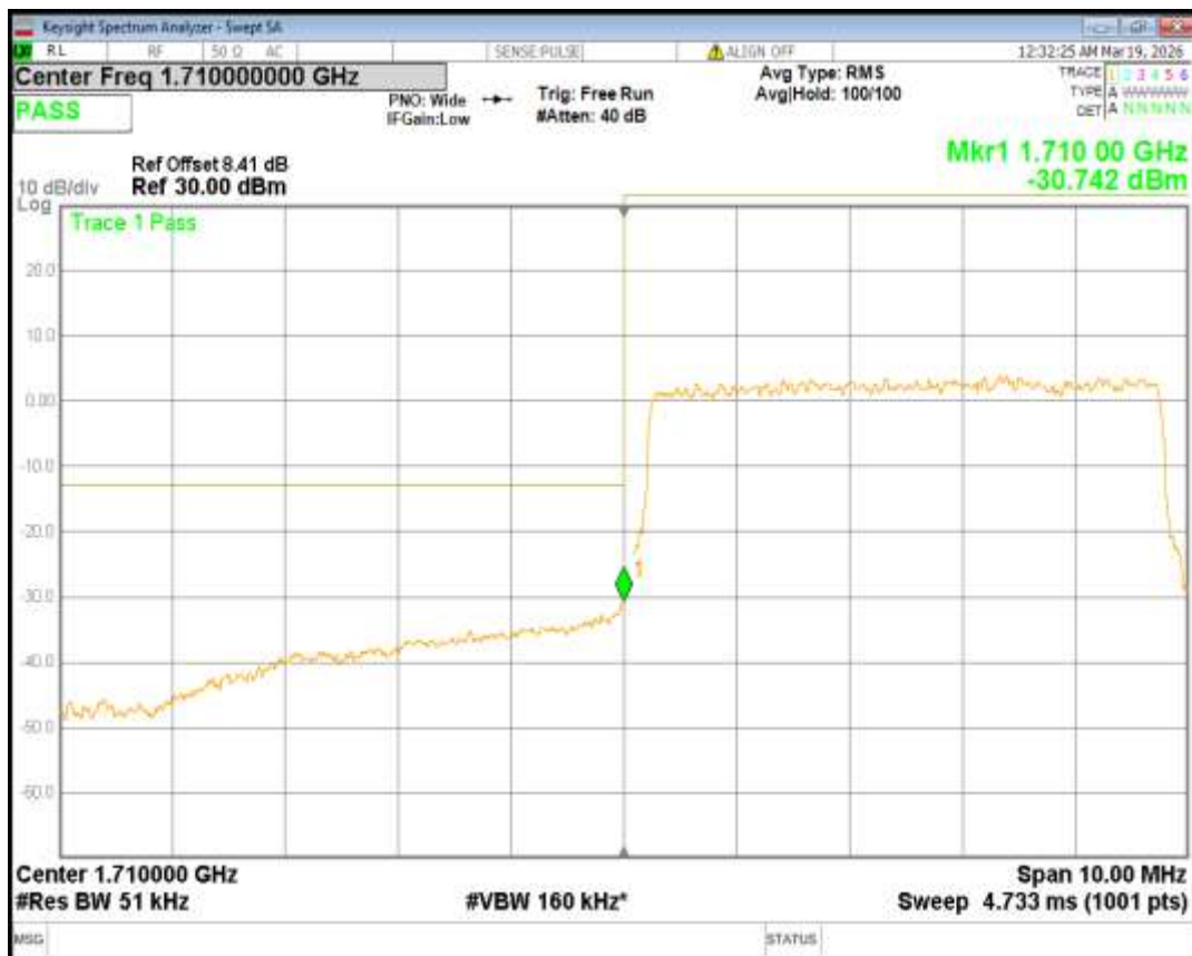
Band4 QPSK BW=5MHz Channel=20375 RB Size=25 Position=#0
