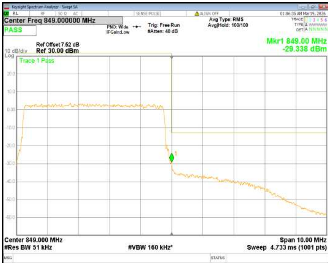
Band5 QPSK BW=1.4MHz Channel=20407 RB Size=6 Position=#0
