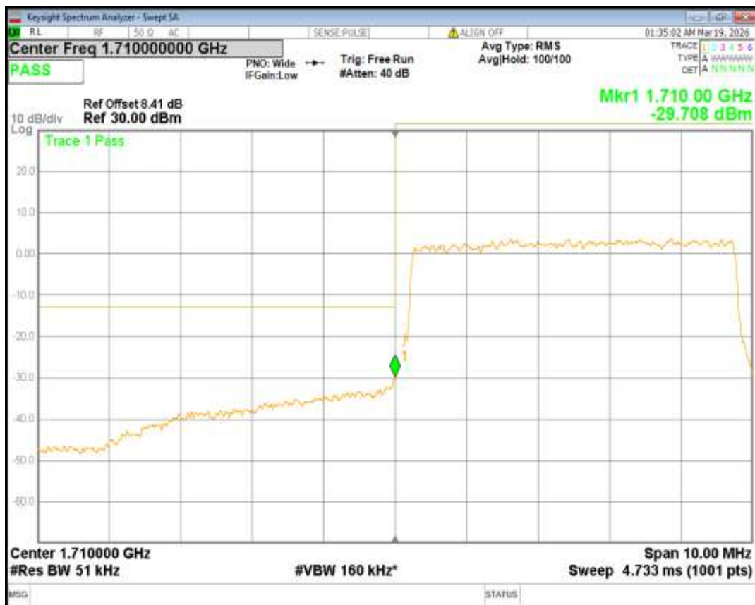
Band66 QPSK BW=5MHz Channel=132647 RB Size=25 Position=#0
