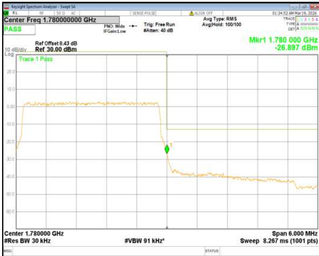
Band66 QPSK BW=5MHz Channel=131997 RB Size=25 Position=#0
