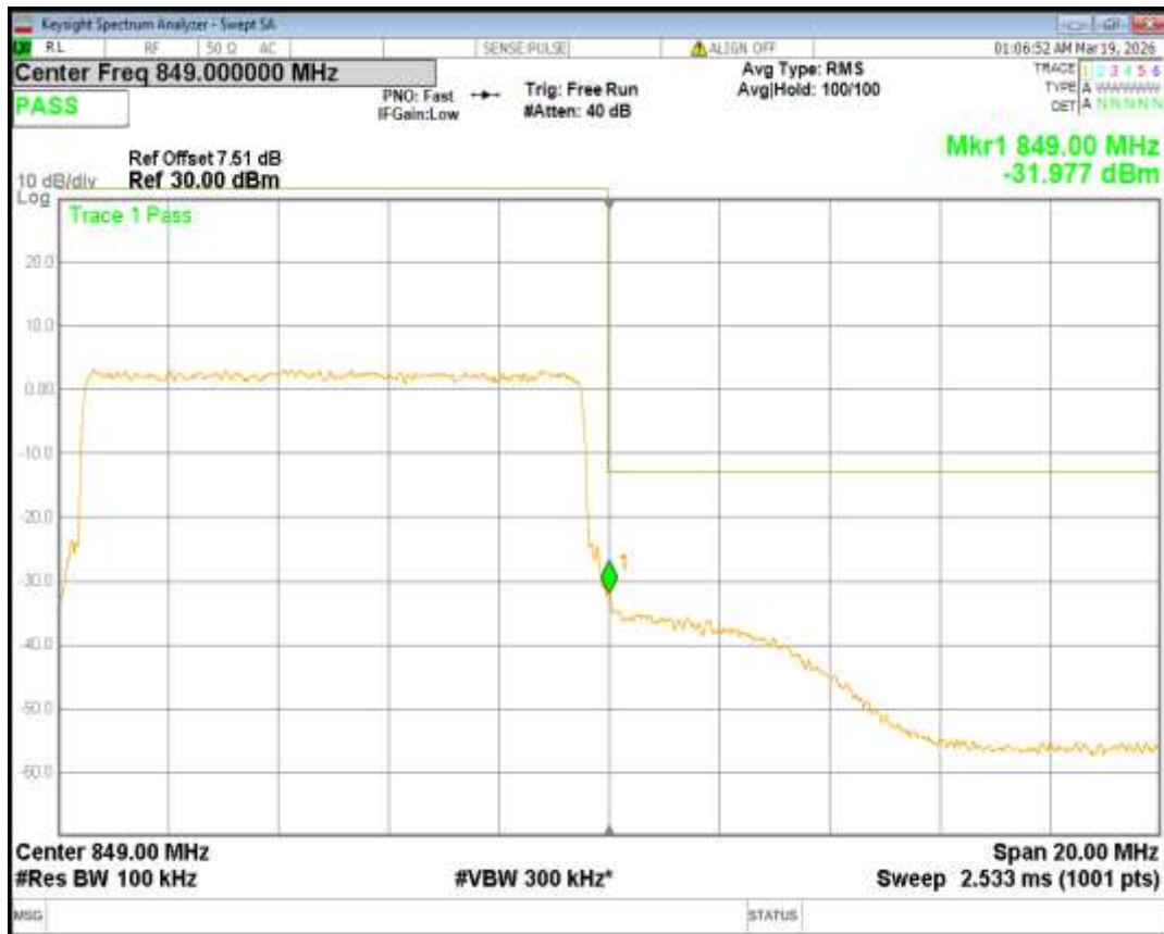
Band5 16QAM BW=3MHz Channel=20415 RB Size=15 Position=#0
