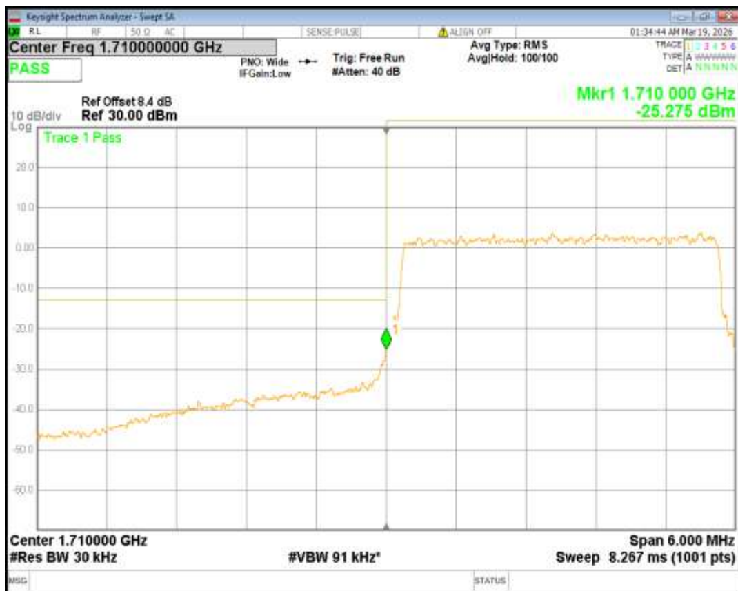
Band66 QPSK BW=3MHz Channel=132657 RB Size=15 Position=#0
