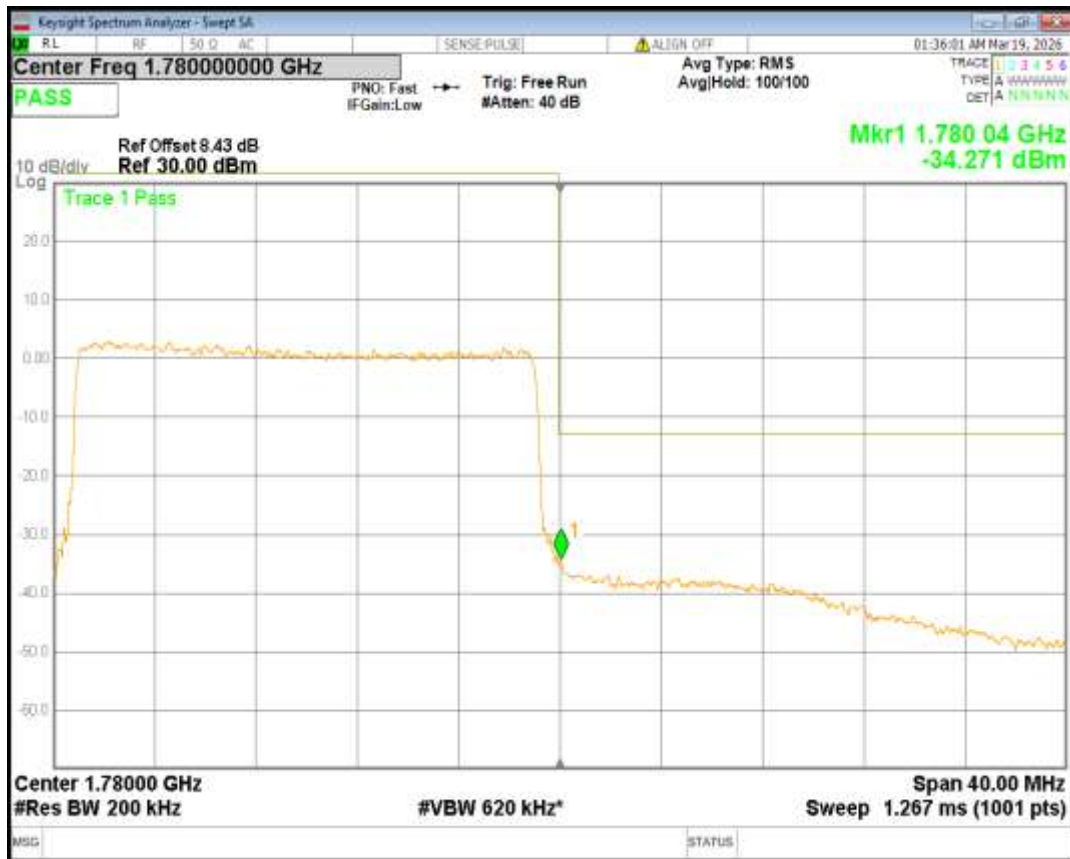
Band66 16QAM BW=3MHz Channel=131987 RB Size=15 Position=#0
