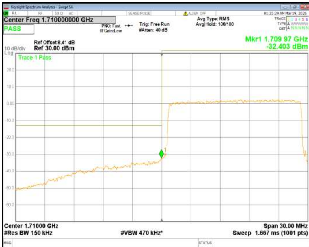
Band66 16QAM BW=15MHz Channel=132597 RB Size=75 Position=#0
