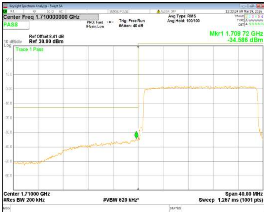
Band4 16QAM BW=20MHz Channel=20300 RB Size=100 Position=#0
