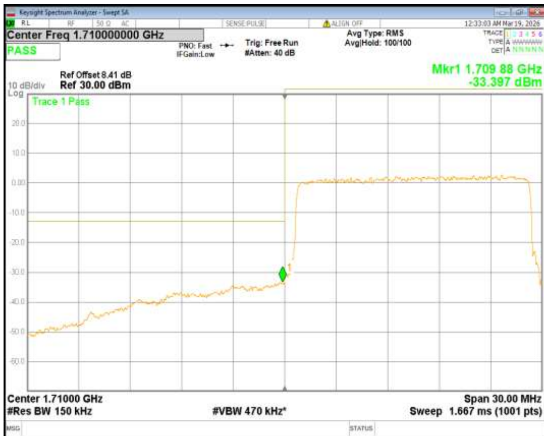
Band4 16QAM BW=15MHz Channel=20325 RB Size=75 Position=#0
