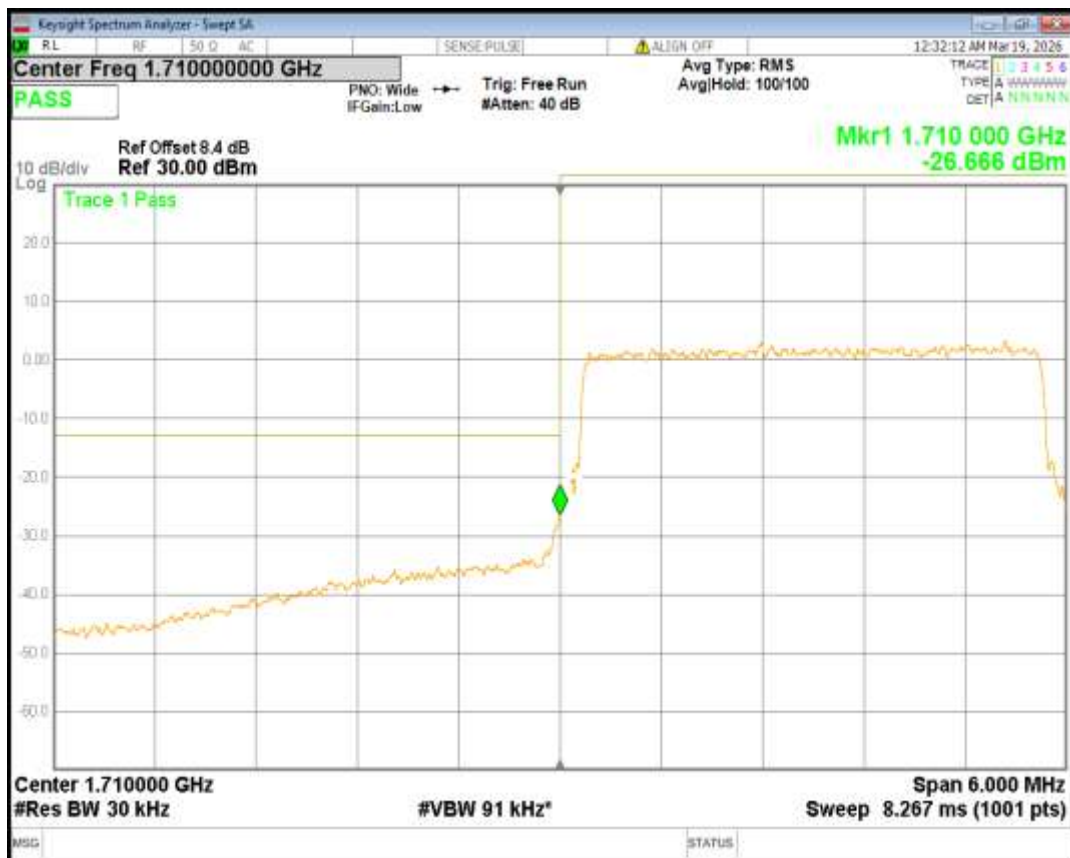
Band4 16QAM BW=3MHz Channel=20385 RB Size=15 Position=#0
