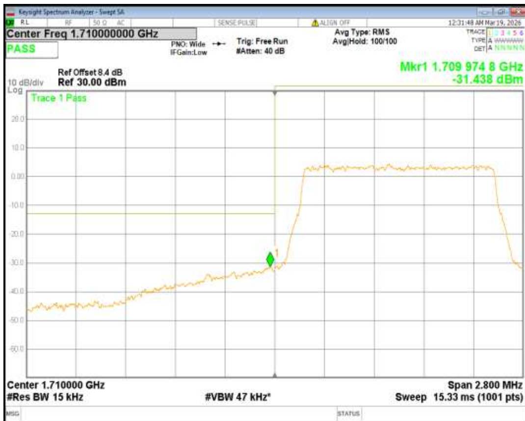
Band4 QPSK BW=1.4MHz Channel=20393 RB Size=6 Position=#0
