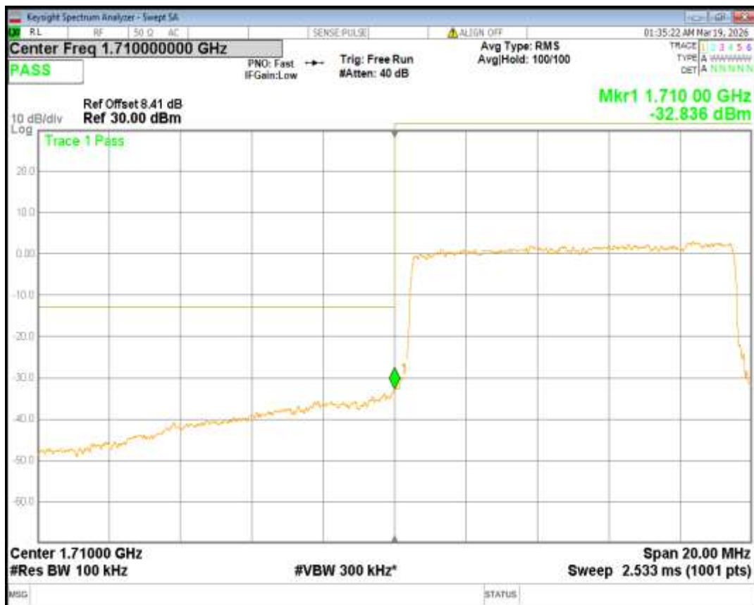
Band66 16QAM BW=10MHz Channel=132622 RB Size=50 Position=#0
