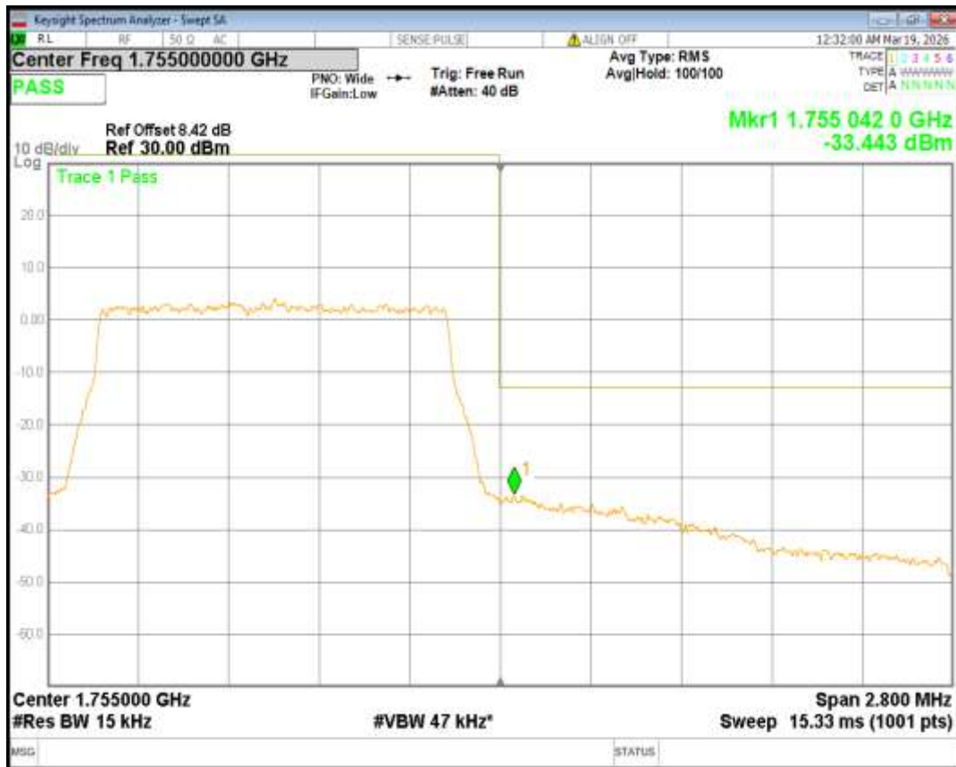
Band4 16QAM BW=10MHz Channel=20000 RB Size=50 Position=#0
