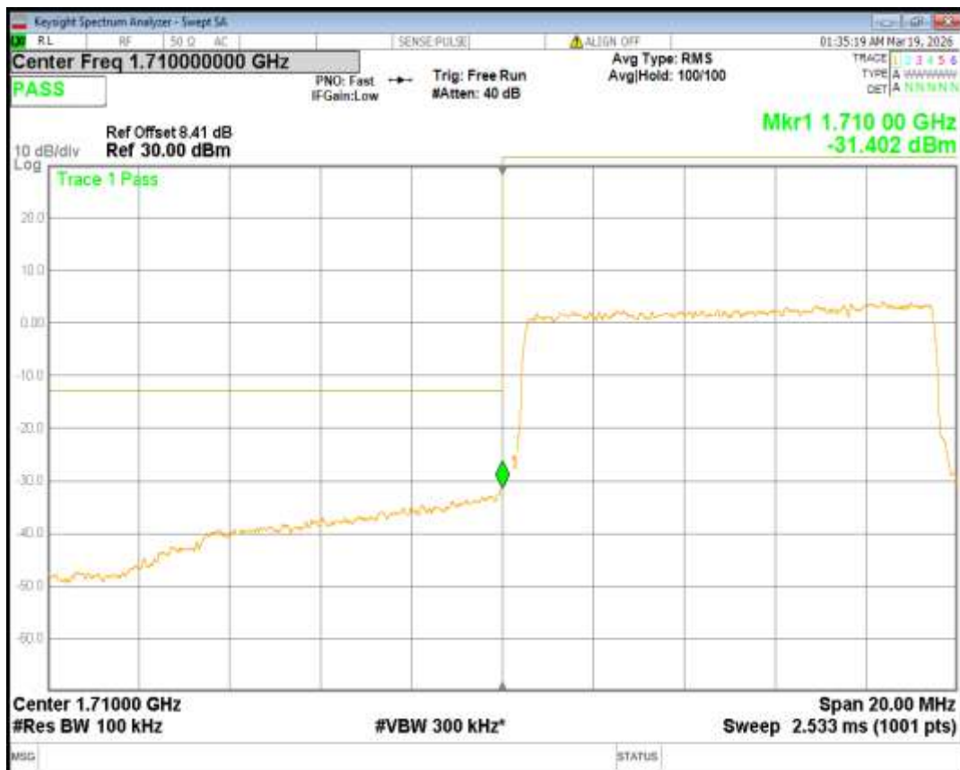
Band66 QPSK BW=10MHz Channel=132622 RB Size=50 Position=#0
