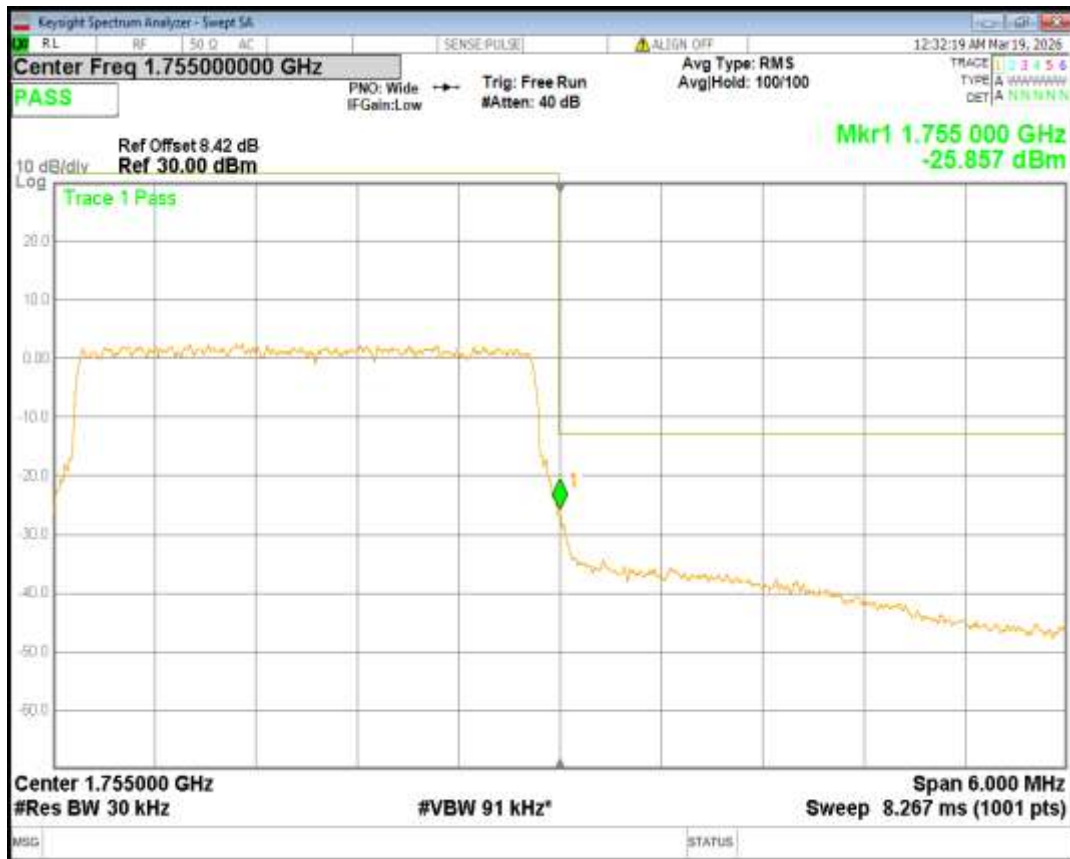
Band4 16QAM BW=5MHz Channel=19975 RB Size=25 Position=#0
