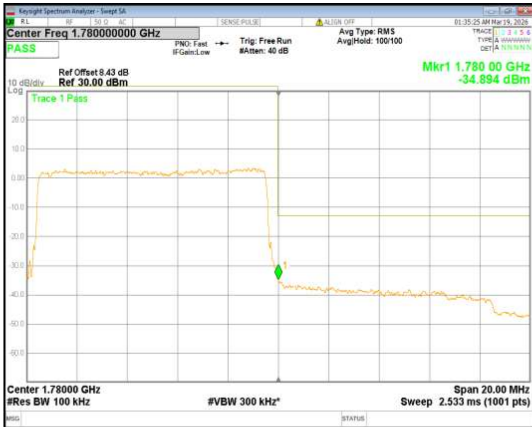
Band66 QPSK BW=15MHz Channel=132047 RB Size=75 Position=#0
