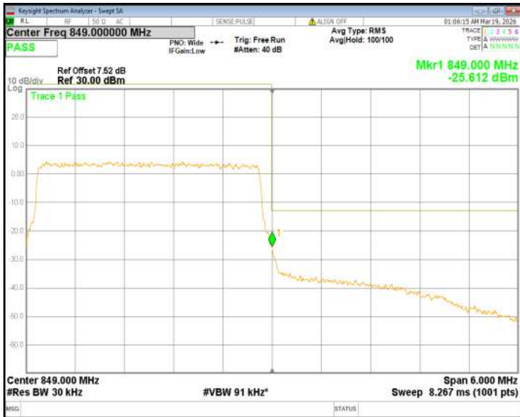
Band5 QPSK BW=5MHz Channel=20425 RB Size=25 Position=#0
