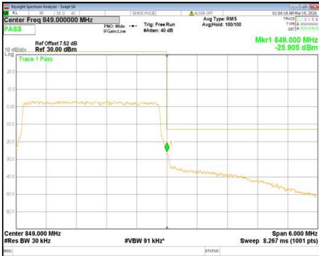
Band5 16QAM BW=5MHz Channel=20425 RB Size=25 Position=#0
