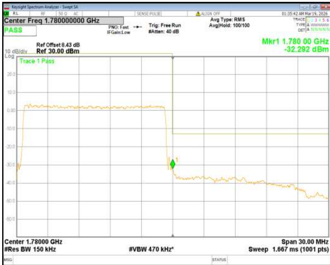
Band66 QPSK BW=20MHz Channel=132072 RB Size=100 Position=#0
