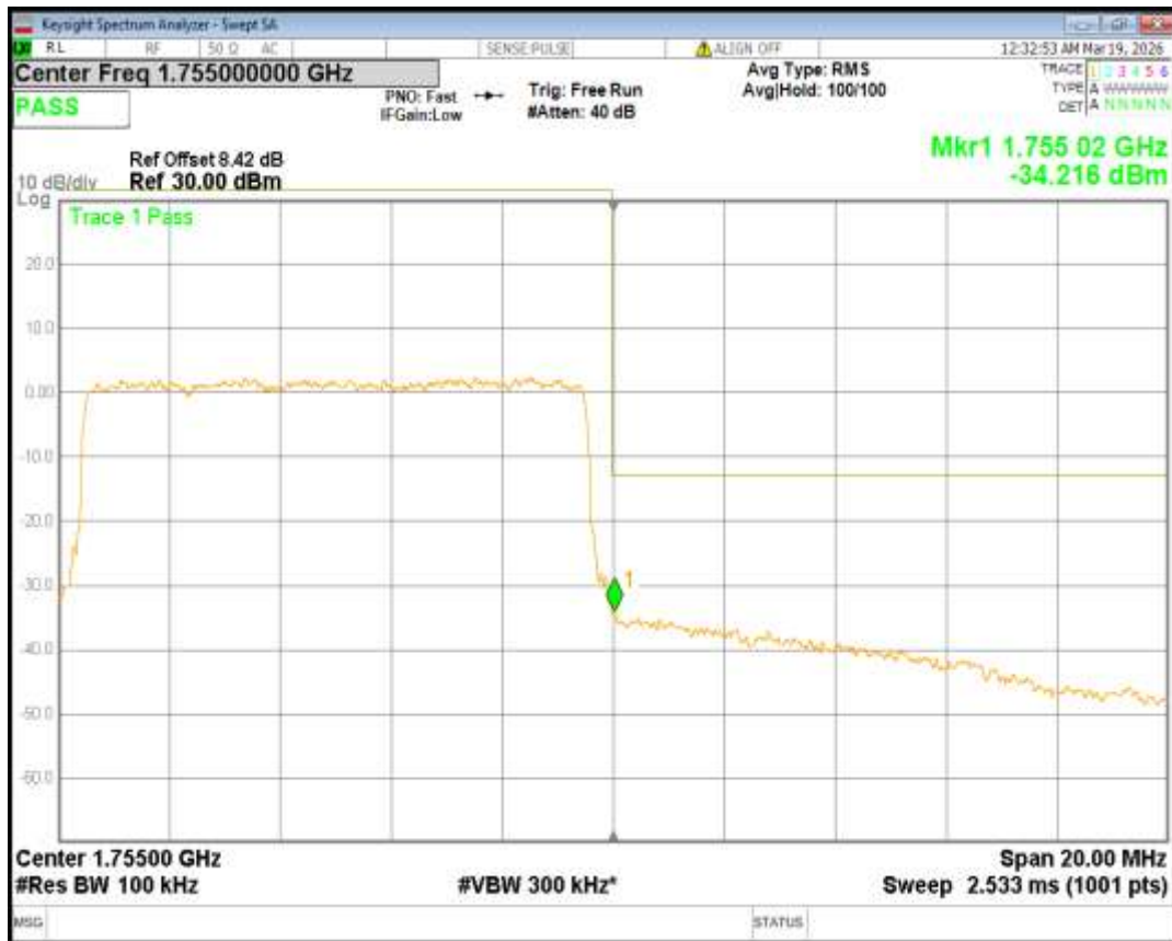
Band4 16QAM BW=15MHz Channel=20025 RB Size=75 Position=#0
