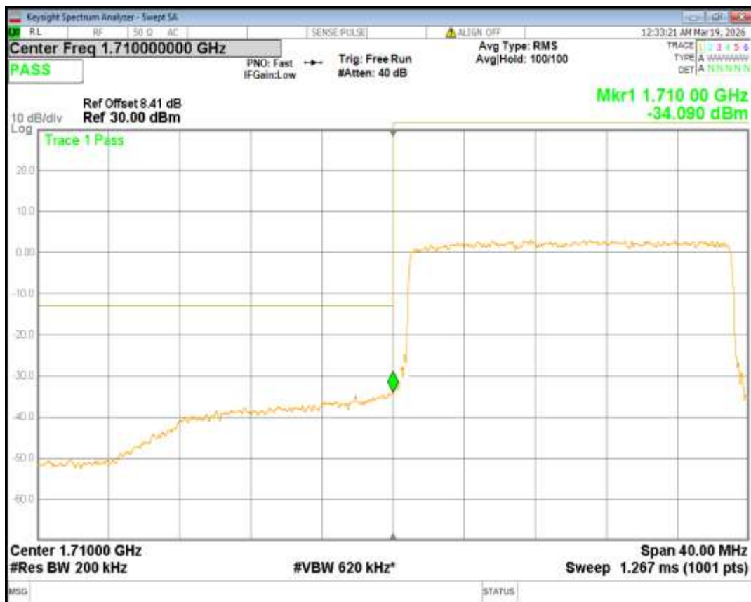
Band4 QPSK BW=20MHz Channel=20300 RB Size=100 Position=#0
