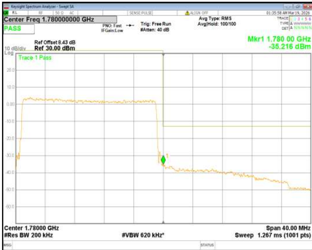
Band66 QPSK BW=3MHz Channel=131987 RB Size=15 Position=#0
