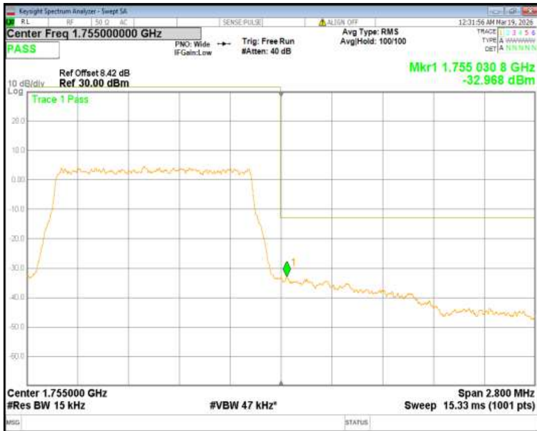
Band4 QPSK BW=10MHz Channel=20000 RB Size=50 Position=#0
