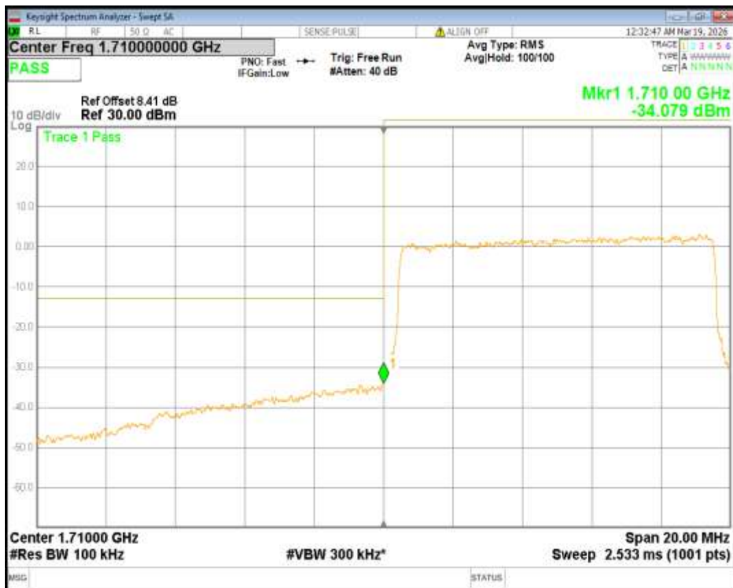
Band4 16QAM BW=10MHz Channel=20350 RB Size=50 Position=#0
