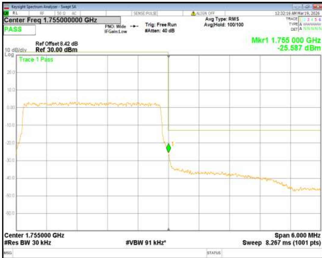
Band4 QPSK BW=5MHz Channel=19975 RB Size=25 Position=#0
