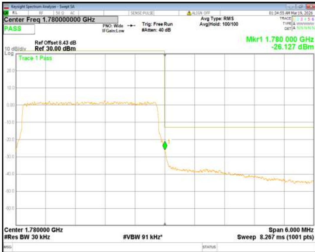
Band66 16QAM BW=5MHz Channel=131997 RB Size=25 Position=#0
