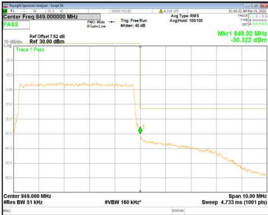
Band66 16QAM BW=1.4MHz Channel=131979 RB Size=6 Position=#0
