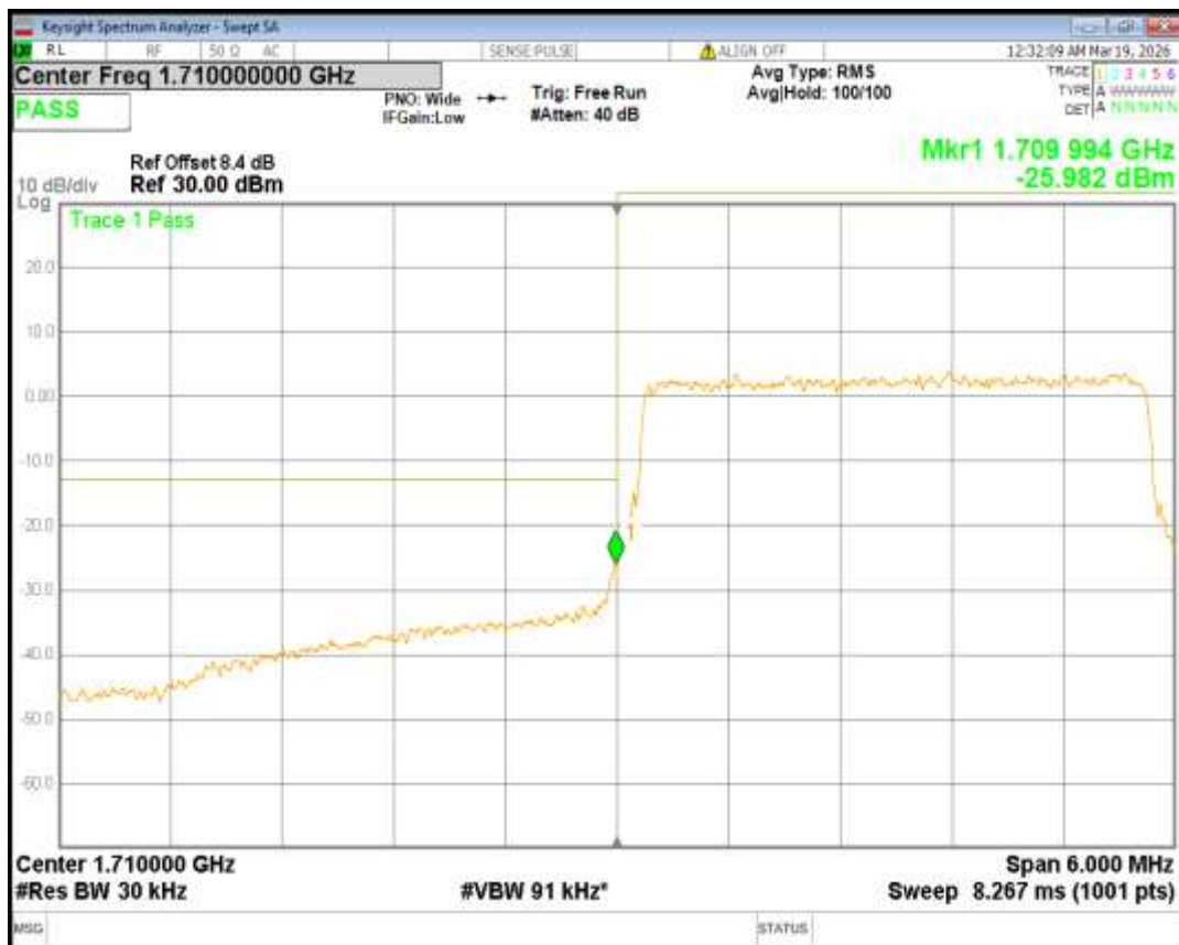
Band4 QPSK BW=3MHz Channel=20385 RB Size=15 Position=#0
