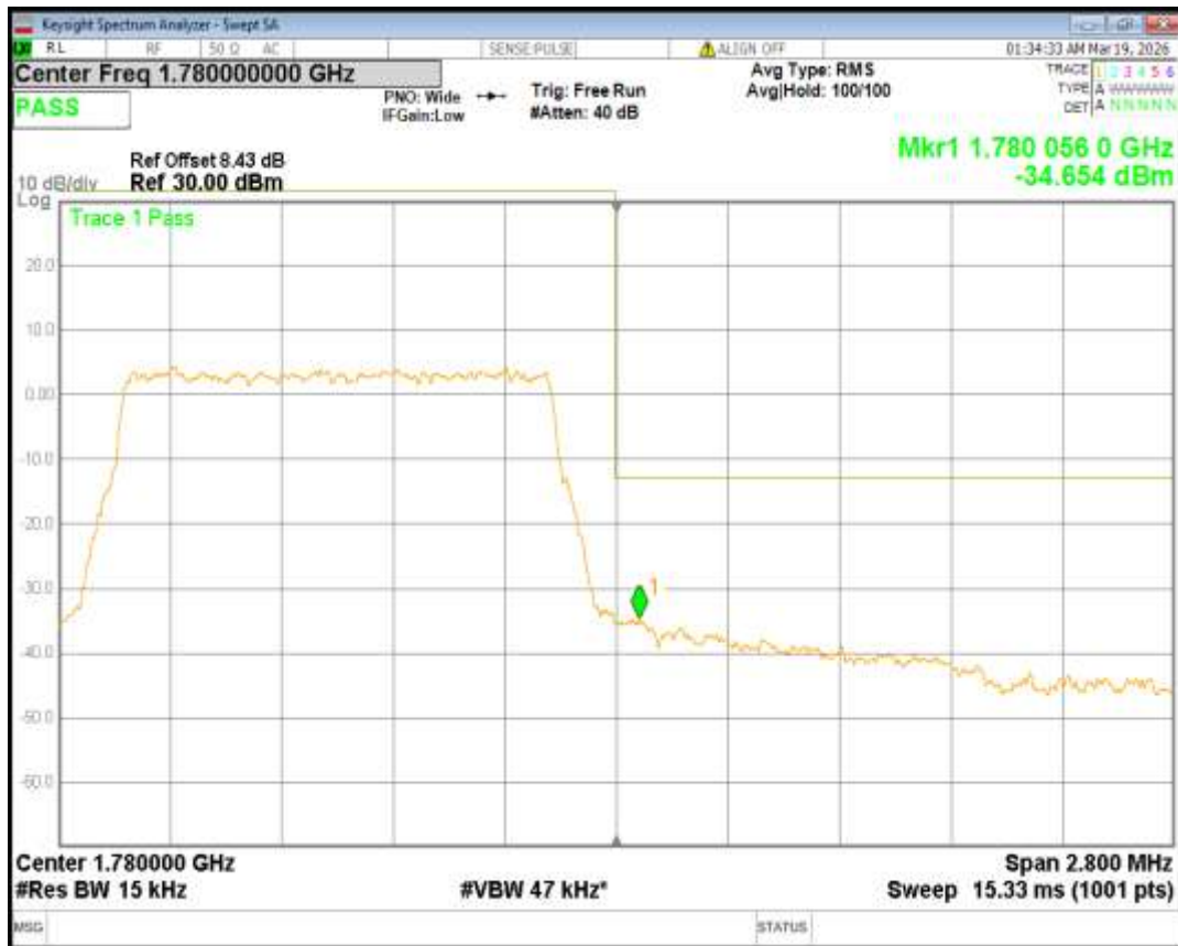
Band66 QPSK BW=10MHz Channel=132022 RB Size=50 Position=#0
