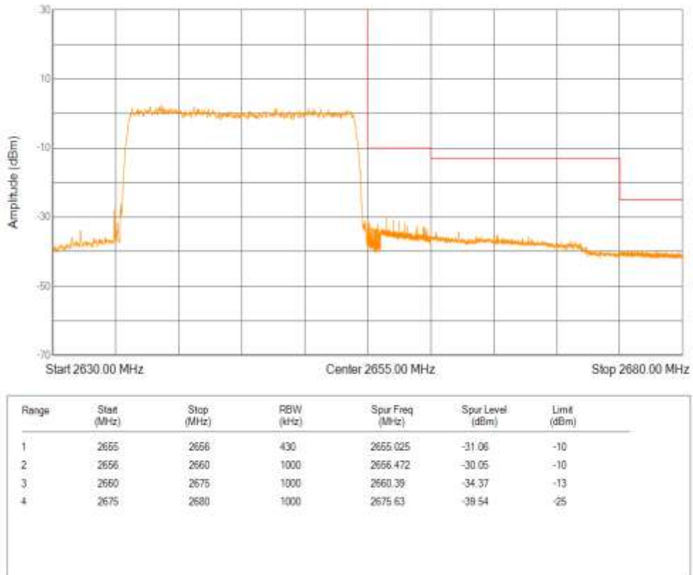
Band41(2535-2655) QPSK BW=5MHz Channel=40065 RB Size=25 Position=#0
