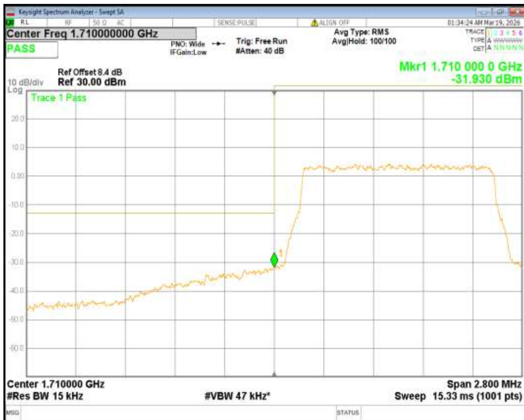
Band66 QPSK BW=1.4MHz Channel=132665 RB Size=6 Position=#0
