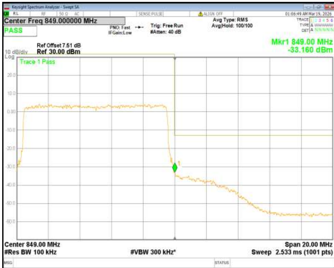
Band5 QPSK BW=3MHz Channel=20415 RB Size=15 Position=#0
