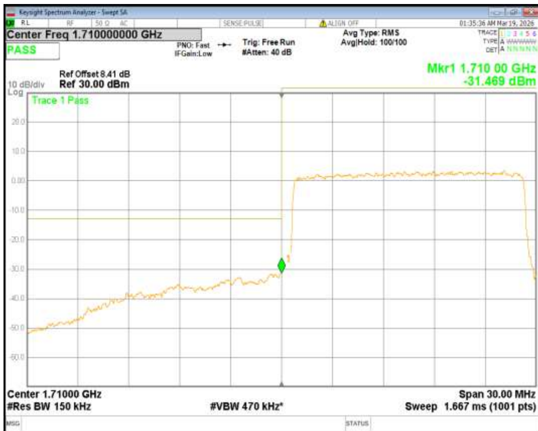
Band66 QPSK BW=15MHz Channel=132597 RB Size=75 Position=#0
