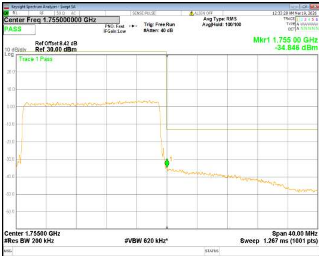
Band4 QPSK BW=3MHz Channel=19965 RB Size=15 Position=#0
