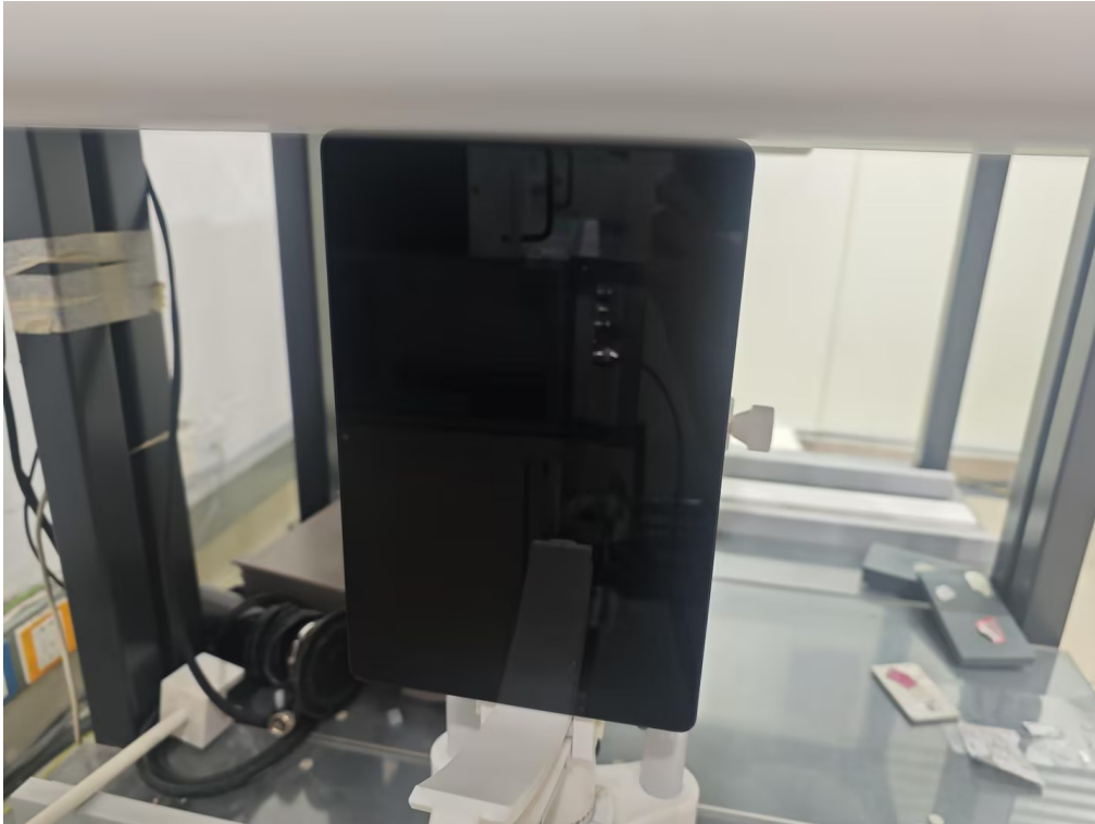
Body Right side(separation distance is 0mm)
