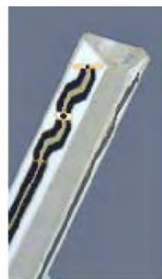
Figure 2.3 Probe Thick-Film Technique
