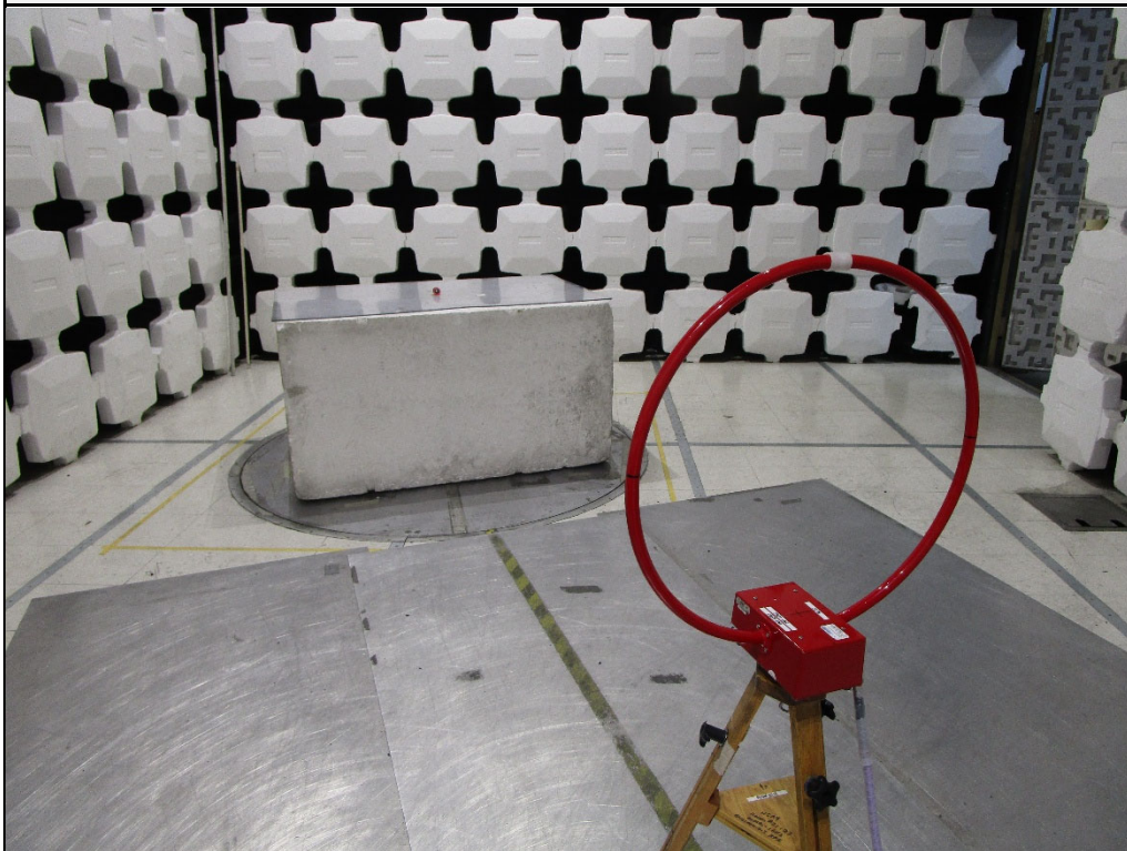
Test Setup for Spurious Radiated Emissions, 9kHz – 30MHz – Antenna Polarization Vertical
