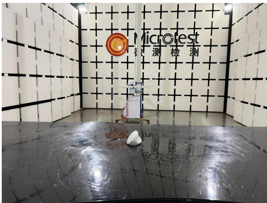
Radiated emissions (below 1GHz)
