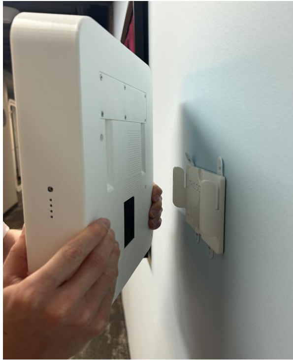
Figure III-3: Device Placement in Wall Mount
