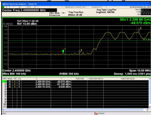
Out Of Band Emission(Left) GFSK_DH5_Channel Hopping
