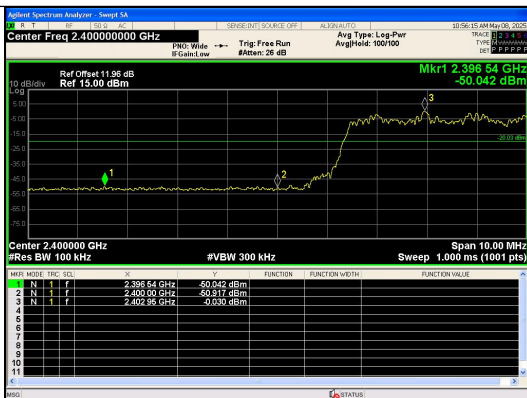
Out Of Band Emission(Left) 8DPSK_3-DH5_Channel Hopping
