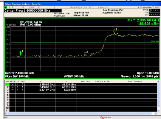
Out Of Band Emission(Left) \pi/4 DQPSK_2-DH5_Channel Hopping
