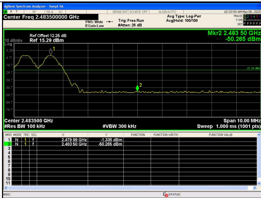
Out Of Band Emission(Right) GFSK_DH5_Channel Hopping
