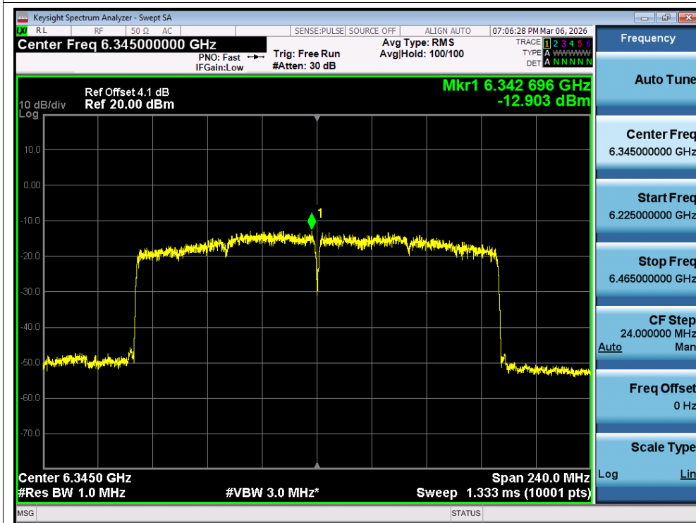
PSD NVNT ax160 6345MHz AntB
