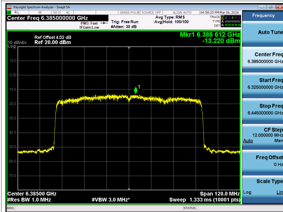
PSD NVNT ax80 6385MHz AntB
