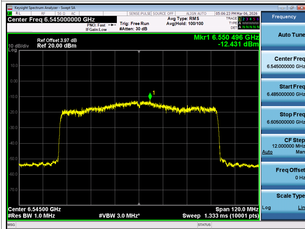
PSD NVNT ax80 6545MHz AntB
