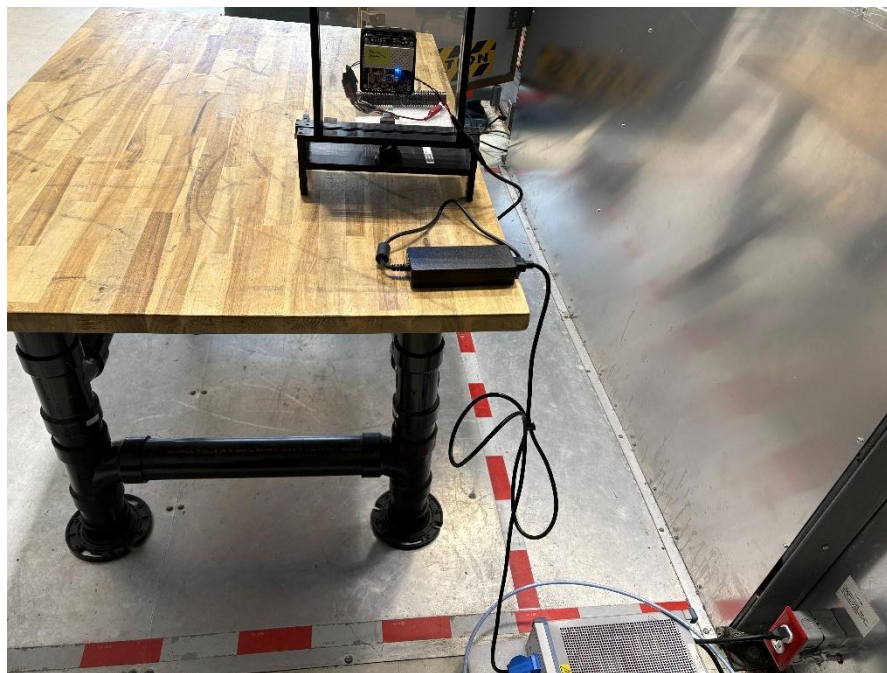
Figure 7.2-3: Conducted emissions – from AC mains power ports setup photo
