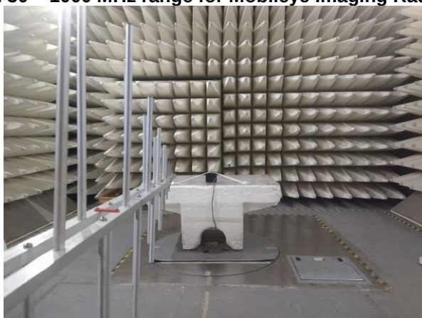
Photograph No.2 Setup for spurious emission field strength measurements in the anechoic chamber in 30 – 1000 MHz range for Mobileye Imaging Radar 1.0
