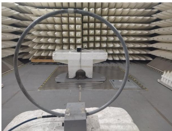
Photograph No.1 Setup for spurious emission field strength measurements in the anechoic chamber below 30 MHz for Mobileye Imaging Radar 1.0
