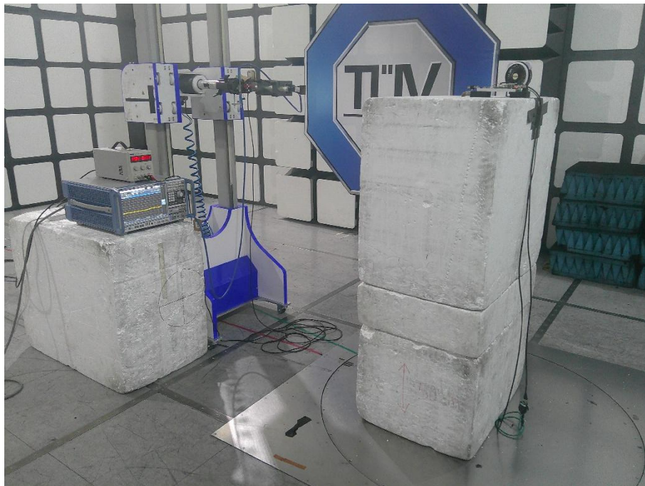
Figure 49 - Radiated test setup 18GHz to 26GHz
