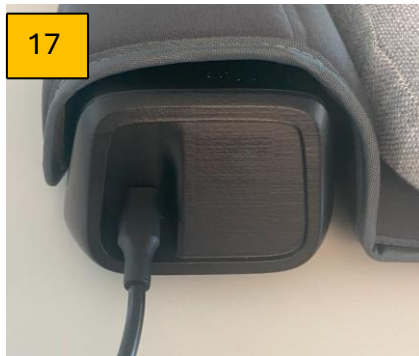
Figure 9: Rear view of the B-Control Dog (control unit) with the Power Supply Dog (charger) connector
