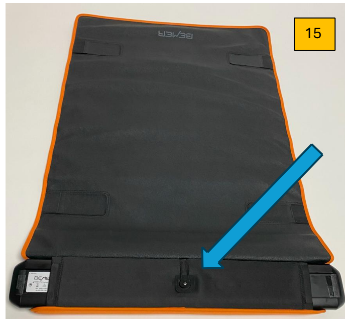
Figure 8: Bottom panel of the B-Control Dog (control device). The arrow-marked electronic contact can be detached to rotate the control device.
