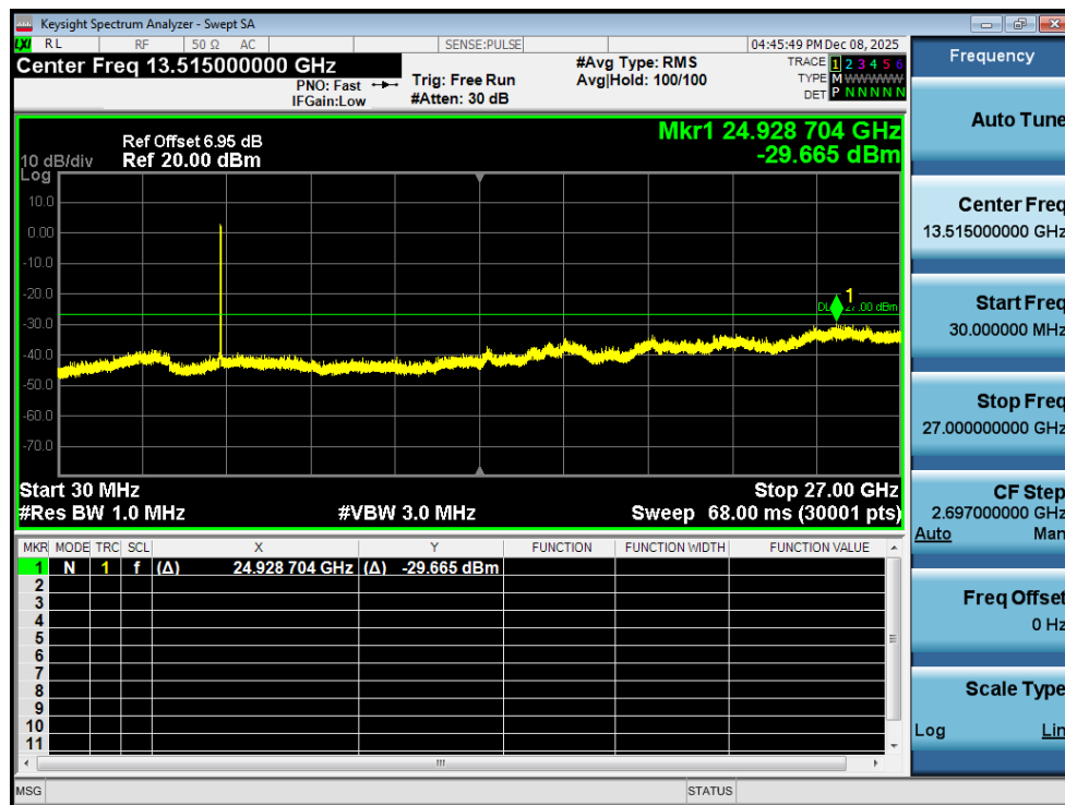
Tx. Spurious NVNT n40 5230MHz Ant1 Emission
