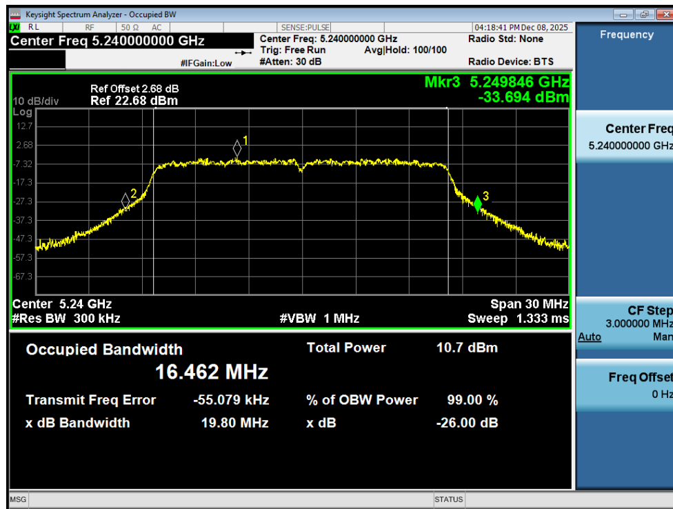
-26dB Bandwidth NVNT a 5240MHz Ant1
