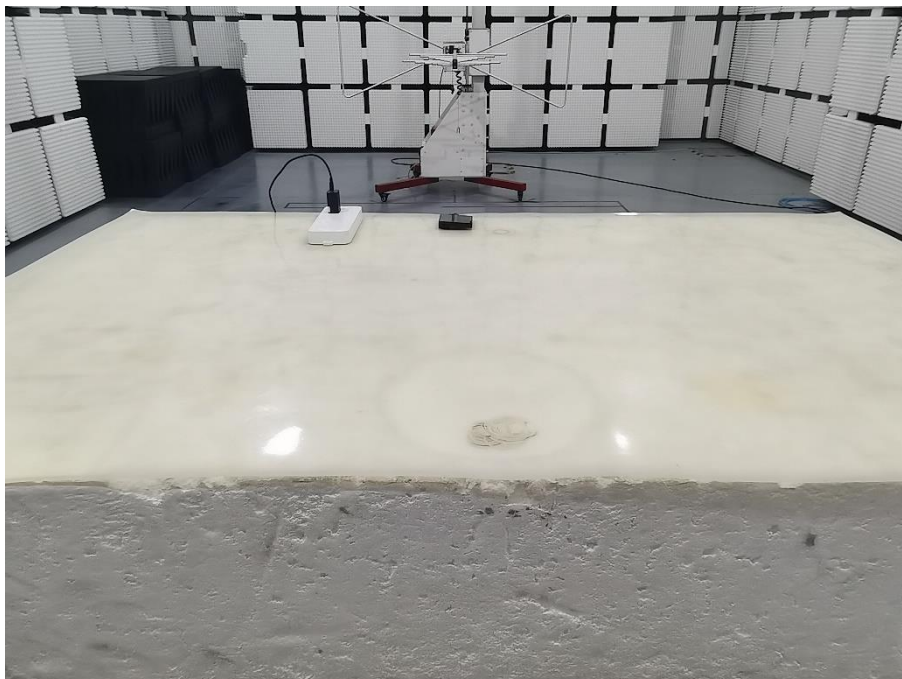
Set-up for Radiated Emission (RE), Below 1GHz
